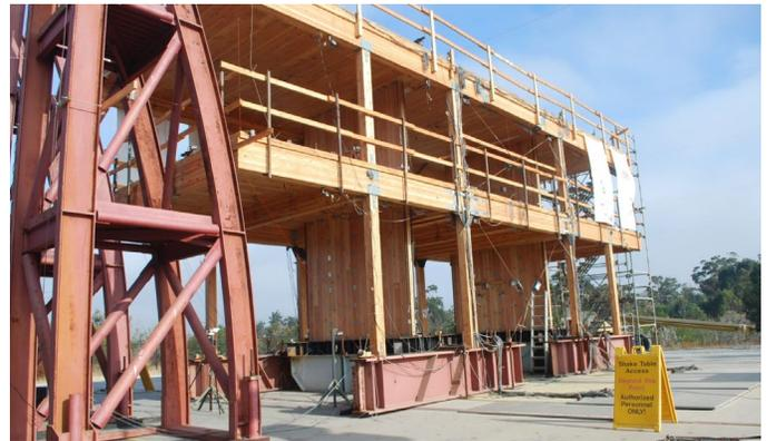
Oregon has allowed use of CLT shear walls since 2015. But the new SAM permits the use of smaller seismic design forces (Path 1) when CLT shear walls are designed in accordance with AWC’s 2021 SDPWS and ASCE 7-22. Path 2 provides design flexibility by allowing design teams to use CLT shear walls that vary from requirements of the 2021 SDPWS when designed for increased seismic forces.
