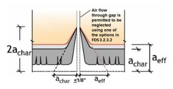
C3.2.3.3 Intersections and abutting edges of exposed members that are in contact or have gaps less than or equal to 1/8 inch but air flow through gaps is not permitted to be neglected (see Figure C3-4):
