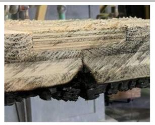
Because charring begins almost immediately when wood is exposed to combustion temperatures, there is insufficient time for an elevated temperature zone to form beyond the tip of the char penetration. As a result, the char penetration into the gap does not need to be increased by the 1.2 factor used for structural calculations. The inner boundary of the elevated temperature zone is depicted by the red line in FDS Figure 3.1.
