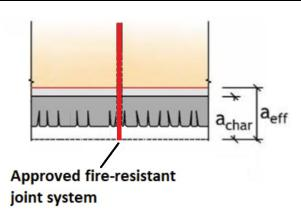
C3.2.3.2 Intersections and abutting edges of exposed members that are in contact or have gaps less than or equal to 1/8 inch and where air flow through gaps is permitted to be neglected using one of the options in FDS 3.2.3.2 (see Figure C3-3):
