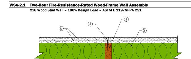
1. Framing: Nominal 2x6 wood studs, spaced 24 in. o.c., double top plates, single bottom plate.
