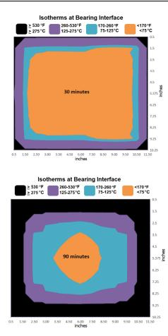
Based on this thermocouple data, a regression was developed to predict the depth of the  $212^{\circ}$ F isotherm relative to  $a_{char}$ . The depth of the  $212^{\circ}$ F isotherm was estimated to be at a depth of  $1.6a_{char}$  ahead of the char front.
