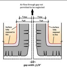
C3.2.3.4 Intersections and abutting edges of exposed members that have gaps greater than 1/8-inch (see Figure C3-5):
