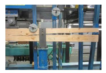
AWC funded testing to collect data to evaluate the end distance, edge distance, and shear design provisions applicable to bolted member connections in AWC's NDS standard.
