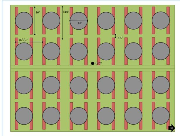
Figure 6. Loading configuration showing barrels placed on loaded bunks and LVDT location.
