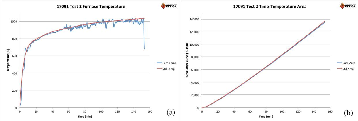
Figure 13. Test 2 (a) furnace temperature and (b) furnace area under the curve compared to the standard curve.
