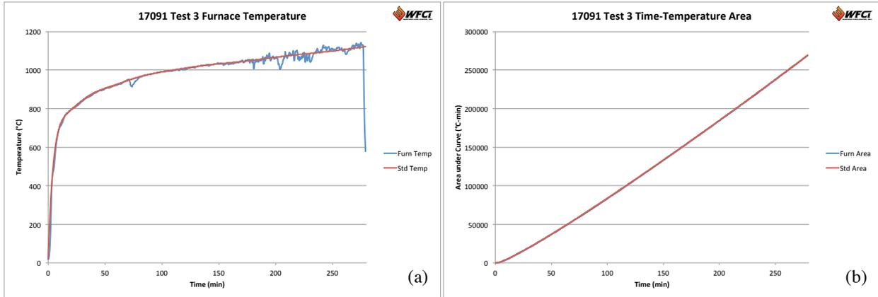
Figure 18. Test 3 (a) furnace temperature and (b) furnace area under the curve compared to the standard curve.
