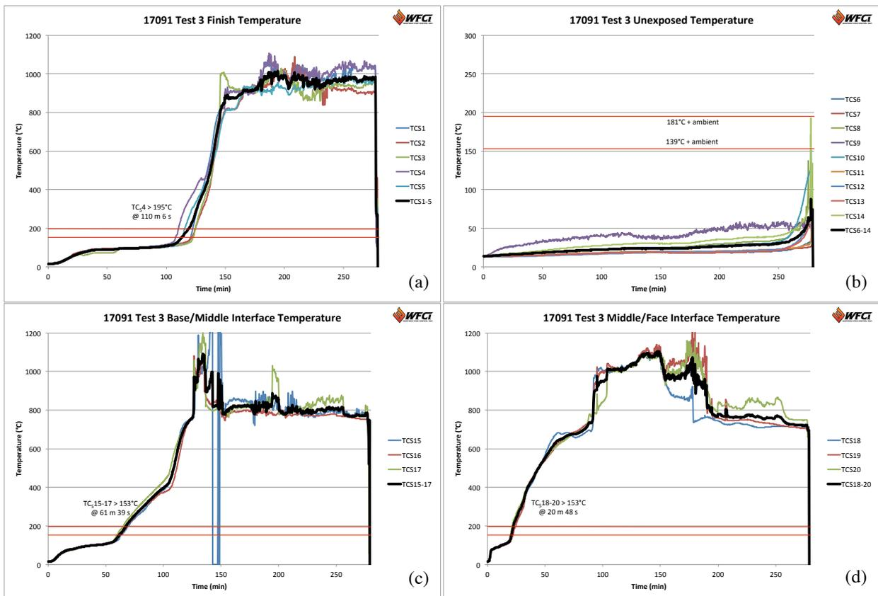
Figure 19. Test 3 sample thermocouples showing (a) finish, (b) unexposed, (c) base/middle, and (d) middle/face temperatures.
