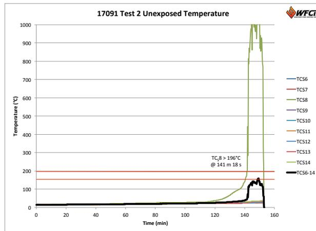
Figure 14. Test 2 sample thermocouples showing unexposed temperature.
