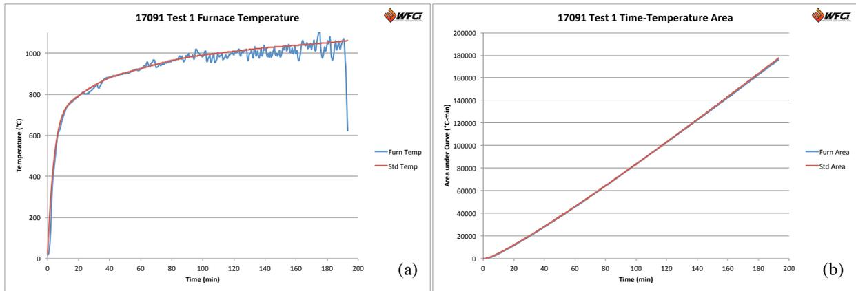
Figure 8. Test 1 (a) furnace temperature and (b) furnace area under the curve compared to the standard curve.
