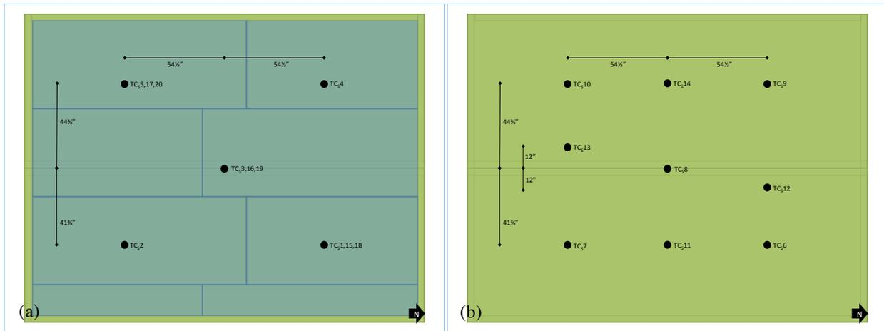
Figure 5. Thermocouple (TC<sub>S</sub>) placement on assembly showing (a) finish and gypsum interface layer temperature and (b) unexposed temperature.
