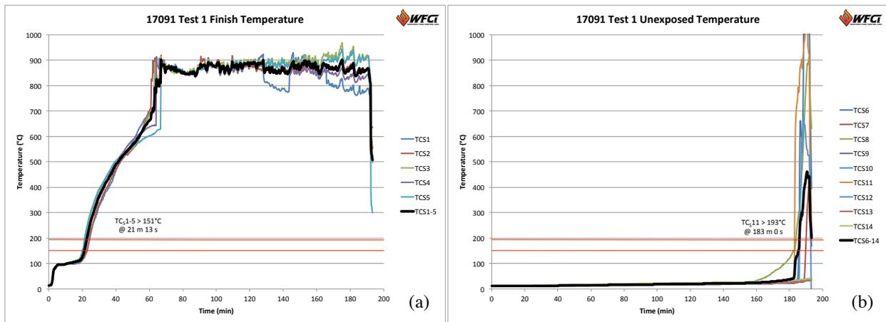
Figure 9. Test 1 sample thermocouples showing (a) finish and (b) unexposed temperature.
