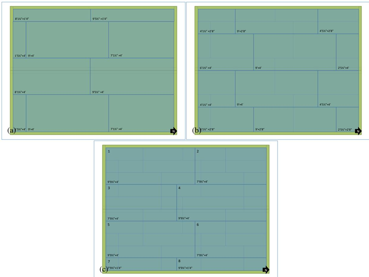
Figure 4. Gypsum layout for Test 3 showing (a) base layer, (b) middle layer, and (c) face layer.
