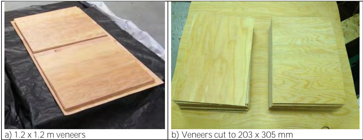
Figure 75: Douglas-Fir veneers for PS 1 testing
