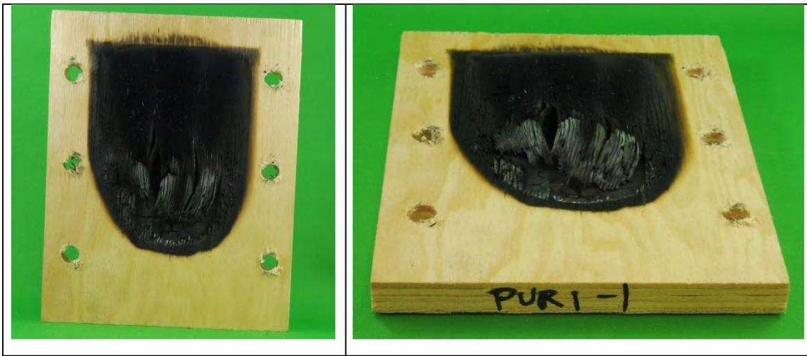
Figure 55: PU1-1 specimen after PS 1 flame testing
