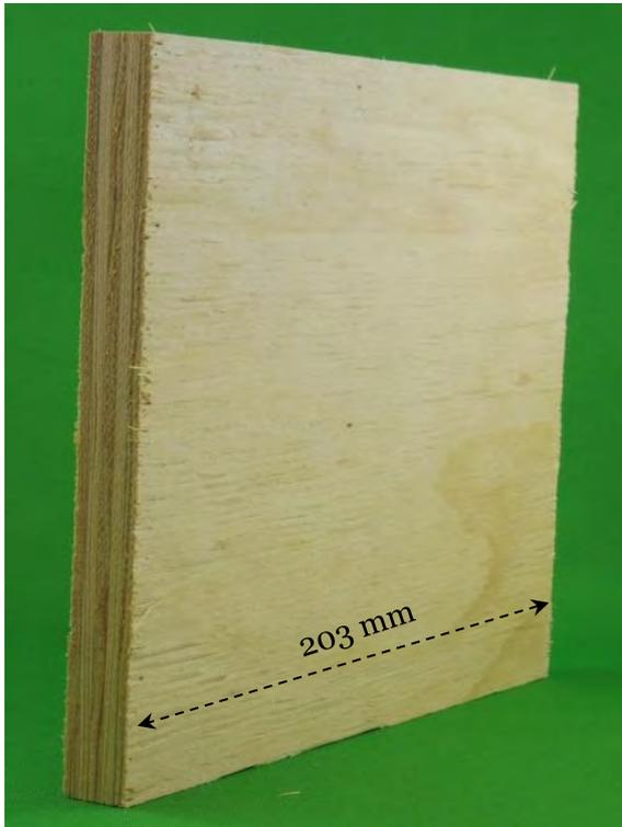
Figure 52: Plywood specimen (PU1-1) prior to flame testing
