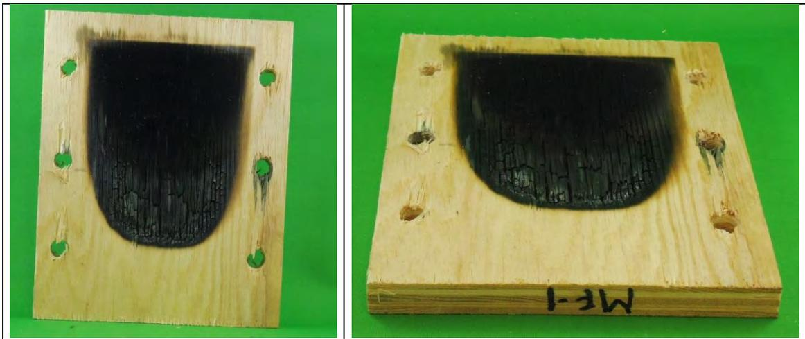
Figure 58: MF-1 specimen after PS 1 flame testing
