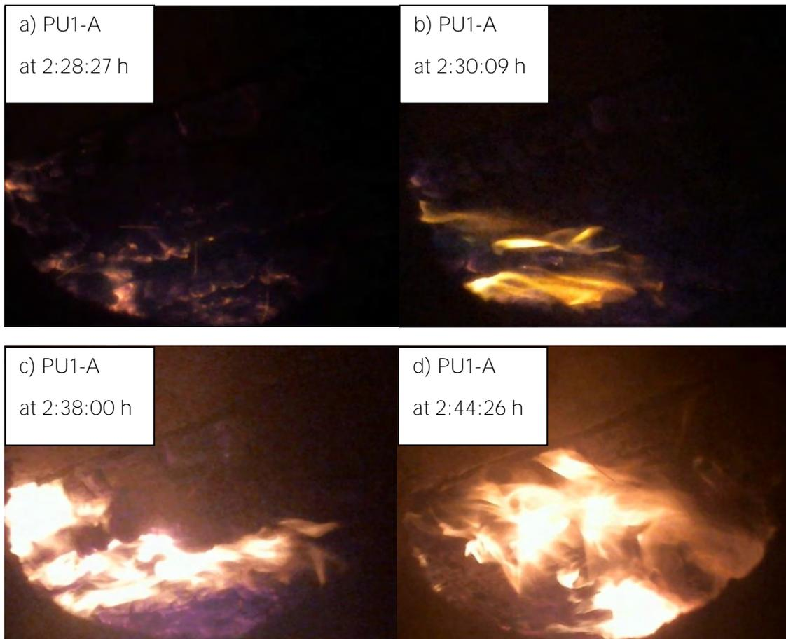
**Figure 30: Photos of the exposed surface in test PU1-A during delamination of the second ply**
