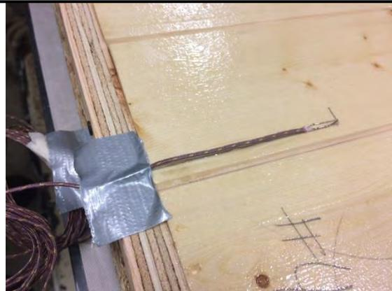
d) Thermocouple placed at a glue line
