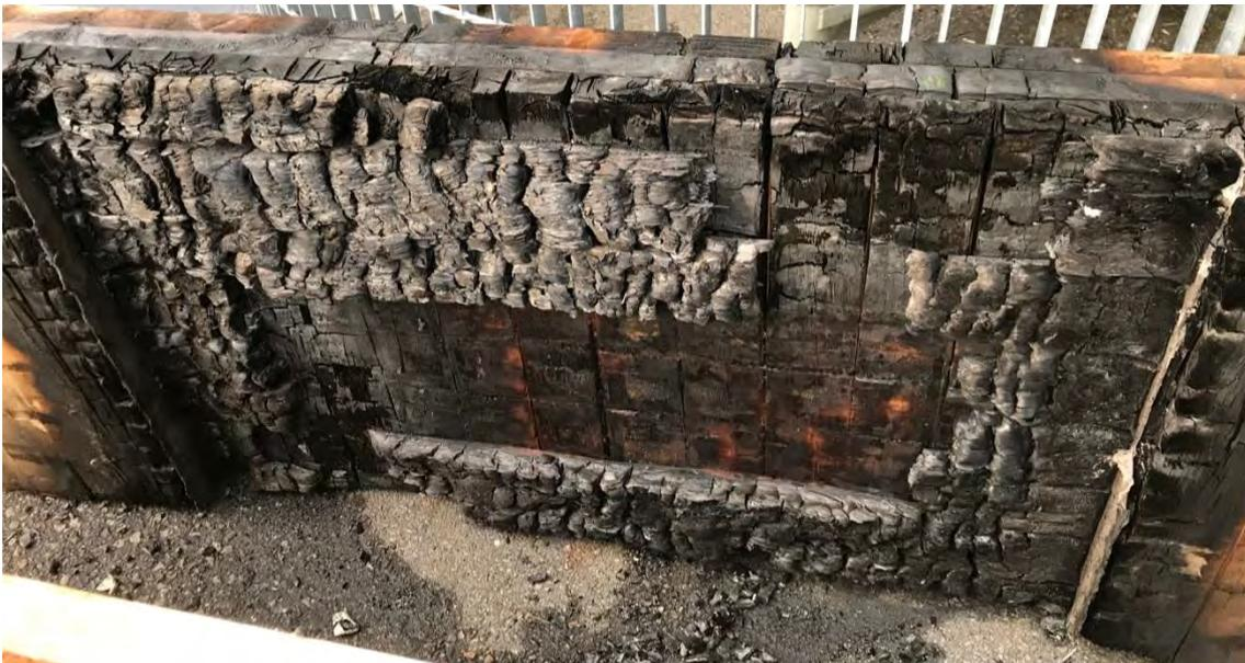
Figure 44: Specimen of test PU1-B after the test.
