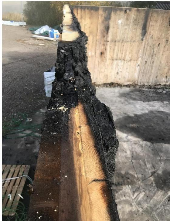
87 - Test 3. Area where resilient profile failed (likely due to lack of airtight seal) to provide protection at wall top.
