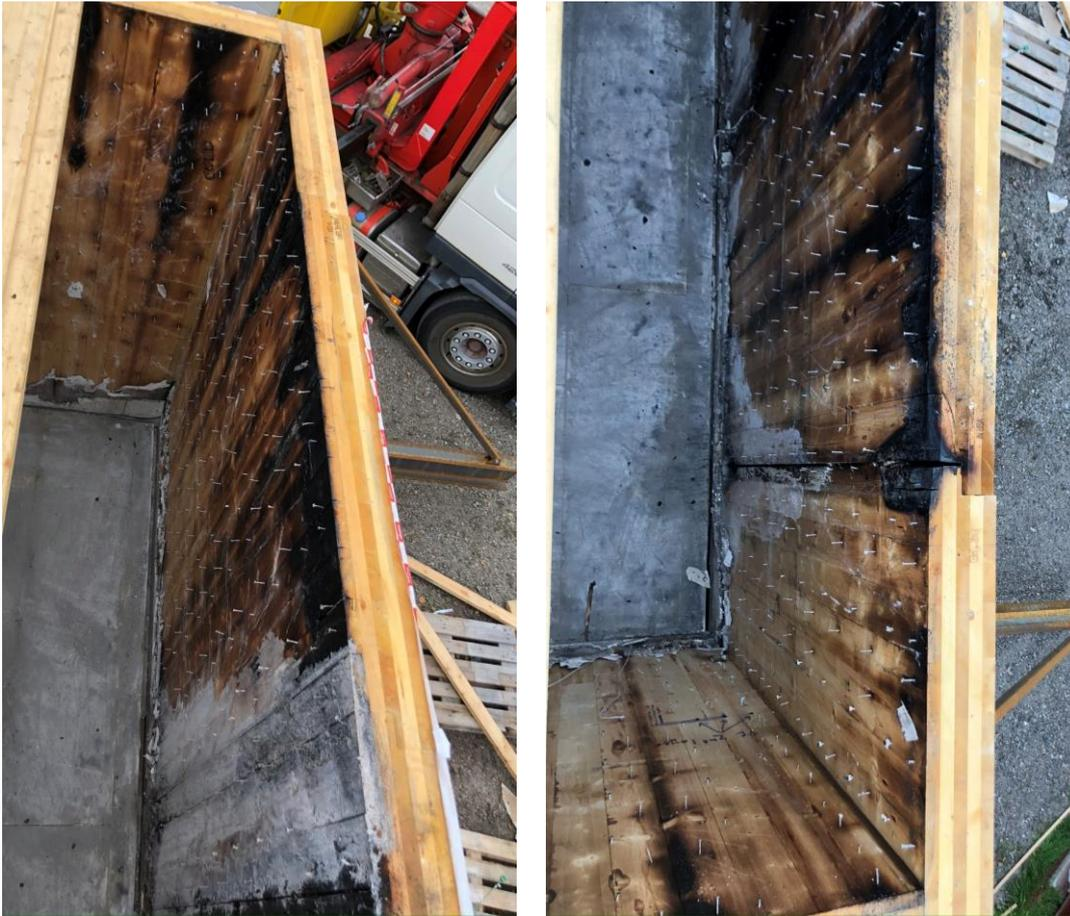
Figure 64: **Test 1**, Top of back wall after removal of ceiling.
