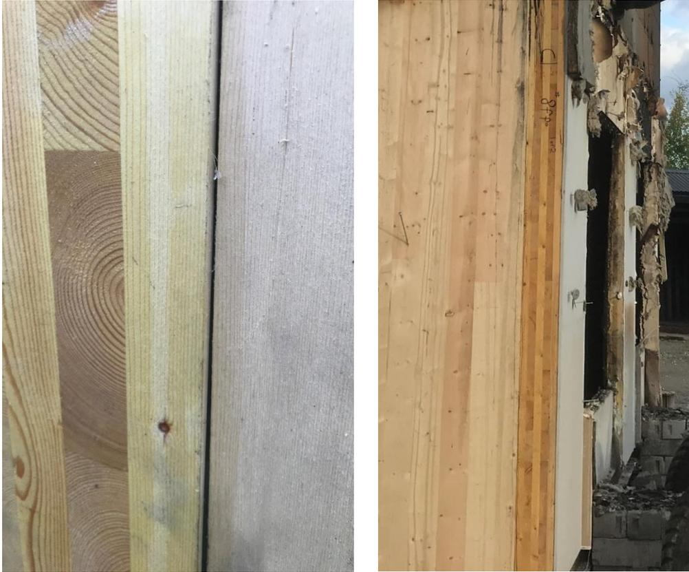
Figure 94: Typical wall-wall butt joint with construction sealing after the test.
