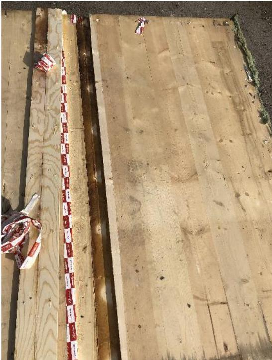
59 - Test 2. Ceiling spline board joint post fire.
