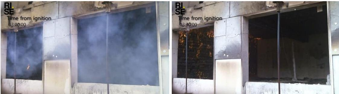
Figure 31: Test 3 - Video snapshots at 3 hours (left) and 3.5 hours (right) after ignition
