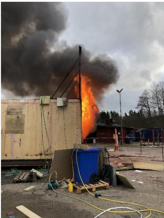
113 - Test 5. Fully developed fire from the side showing flame extension.
