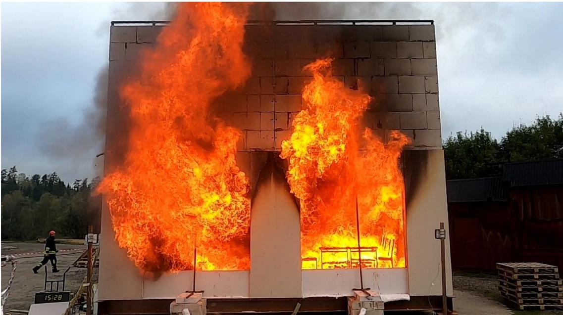
Figure F.1 Test 1 15min 28s after ignition
