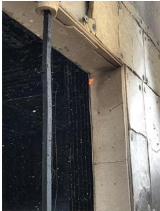
77 - Test 3. Small flame showing from behind gypsum board around opening.
