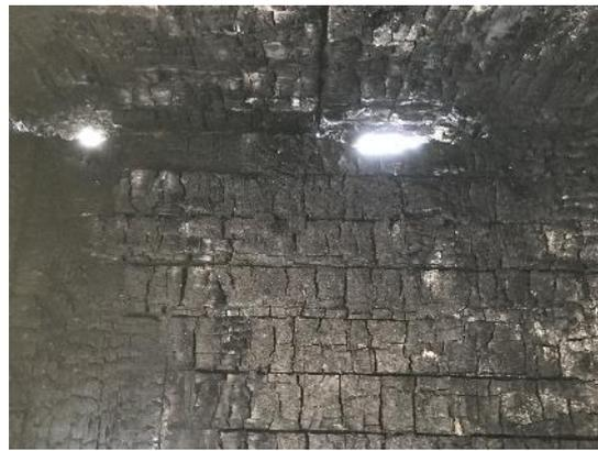
79 - Test 3. gaps visible at wall - ceiling interface post fire.
