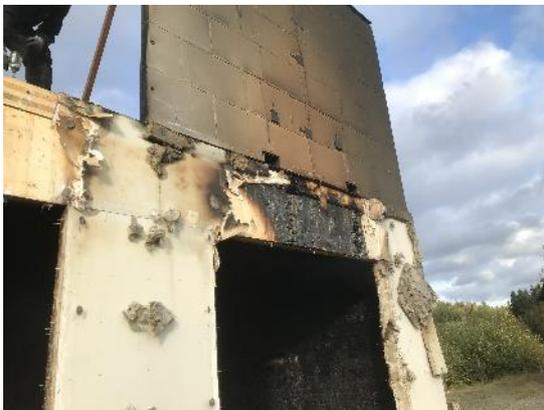
82 - Test 3. Charring of external CLT face above opening visible after protection removed.
