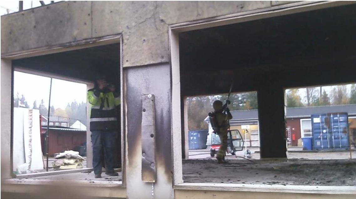
Figure L.5: Cooling down/extinguishing local identified hot spots, directly after Test 4
