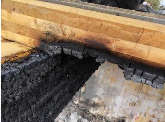
53 – Test 2. Post fire wall-ceiling interface.
