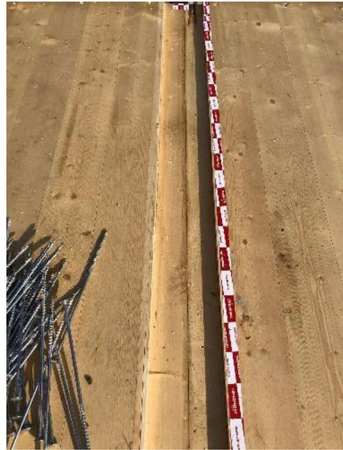
22 - Test 1. Roof joint post fire, no visible charring on unexposed surface at joint.
