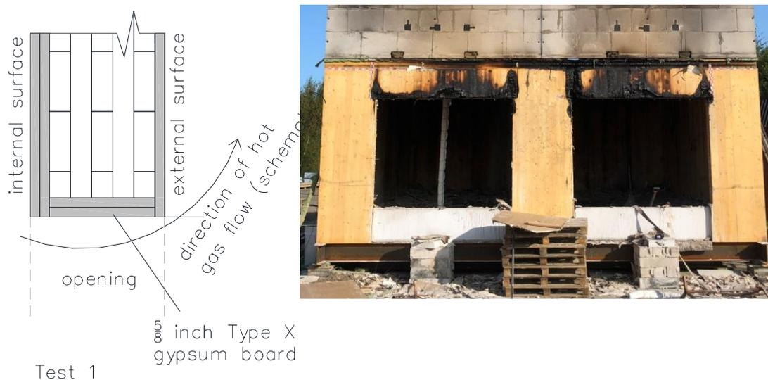
Figure 96: Test 1 - Detail above opening (left) and front façade after removal of gypsum boards (right)
