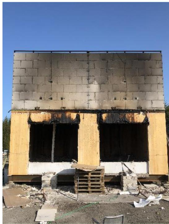
28 - Test 1. Front of the compartment posttest. Some charring directly above the openings. Especially, in the lap-joints which had no sealant applied.
