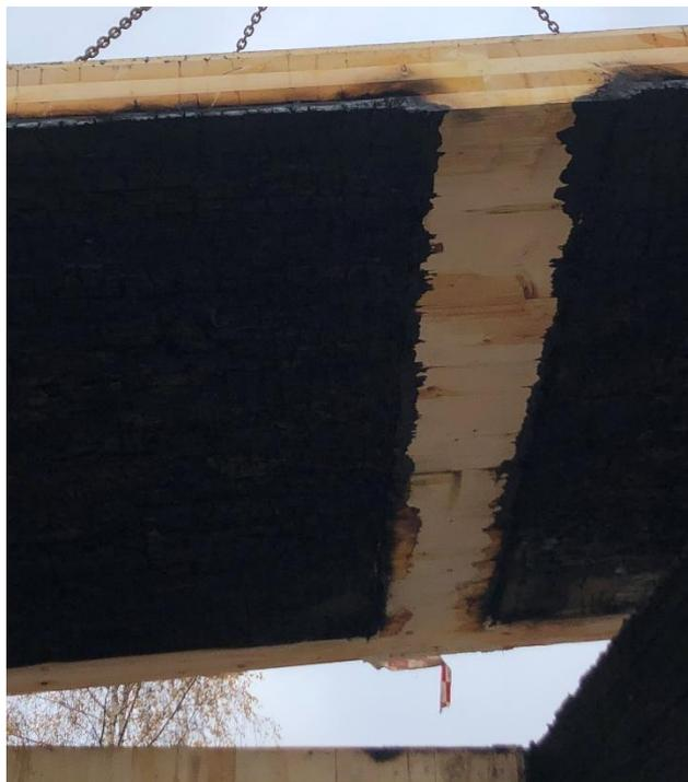
103 - Test 4. Lifting the back wall panel. The uncharred part is the position of the beam and the charring depth in the first lamella is clear.
