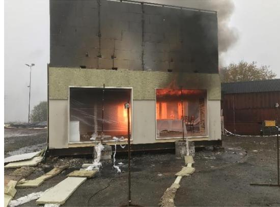
93 - Test 4. Fire shortly before flashover, flames visible along ceiling and small flame extension out of front opening.
