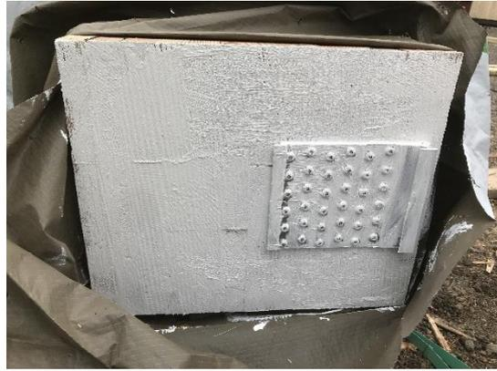
89 - Test 4. Beam end protected with intumescent paint.
