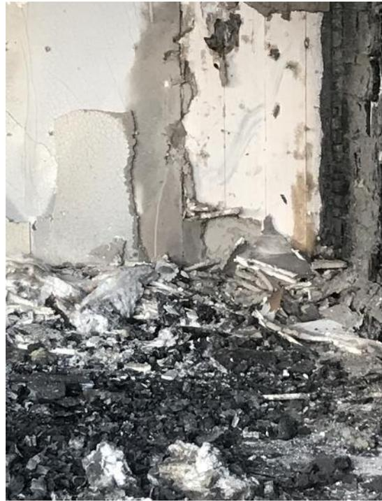
54 – Test 2. Post fire gypsum board condition.
