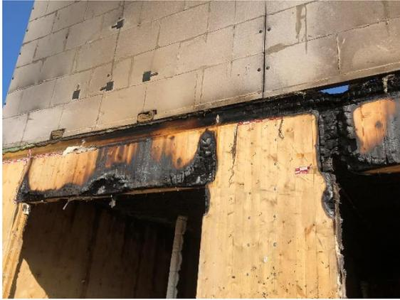
25 Test 1. Damage above the openings after Test 1. Highest damage occurred above the left corner of the right opening. The lap joints above the corners were not sealed in Test 1.
