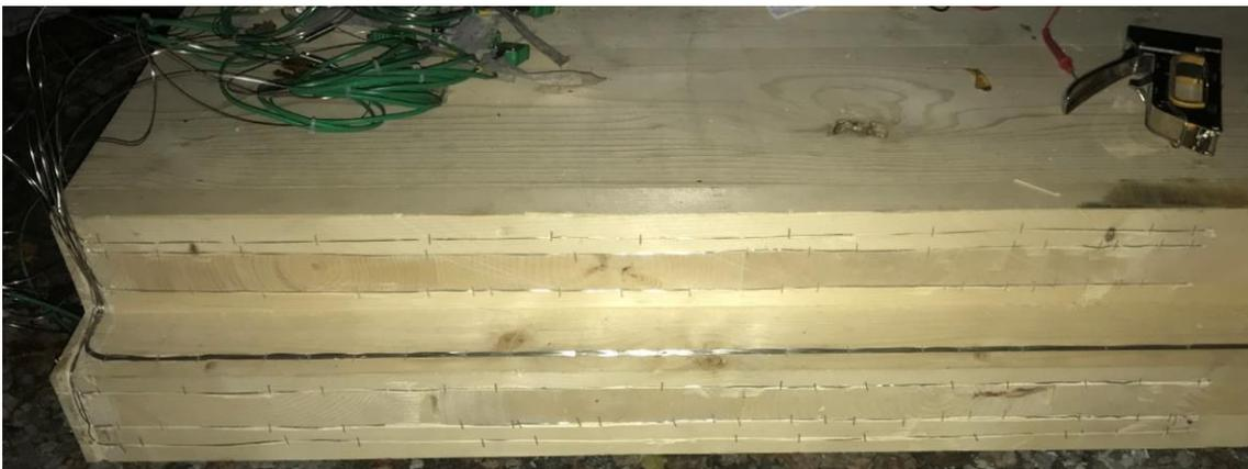
Figure 14: Thermocouples installed at lap-joint of a wall. The thermocouple tip is located at a depth of 75 mm from the visible surface.
