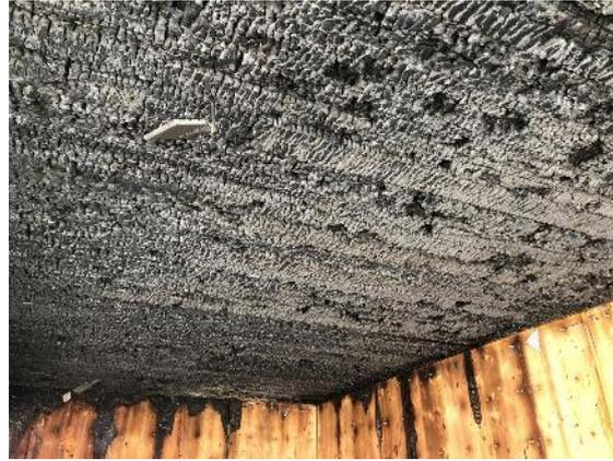
26 - Test 1. Exposed ceiling and unexposed walls (after gypsum removal). Right back corner visible.
