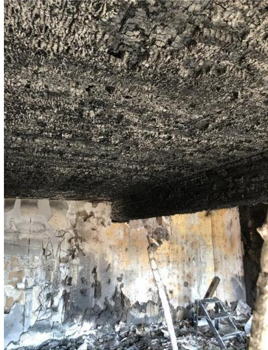
62 - Test 2. Ceiling underside post fire
