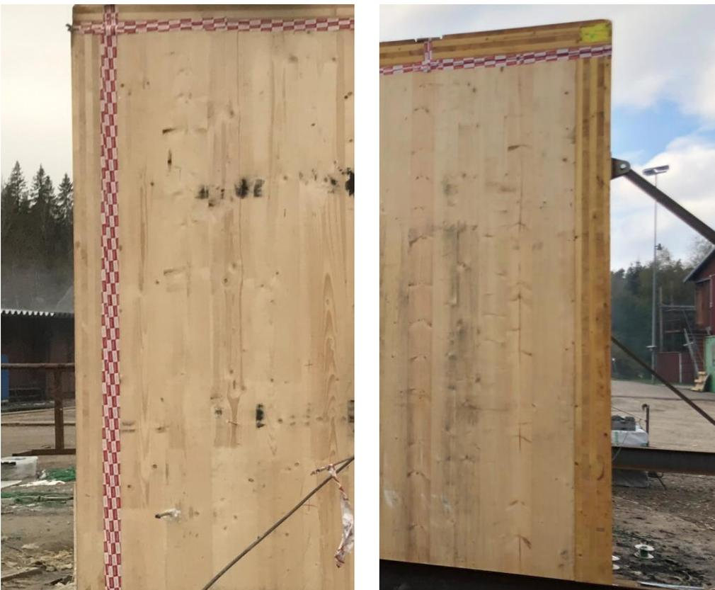
Figure 95: Typical wall-wall butt joint with construction tape (left) and expanding tape (right) after the test.
