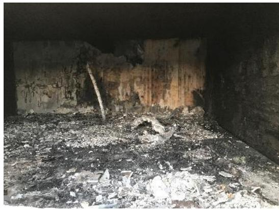
56 – Test 2. Back wall after gypsum removal
