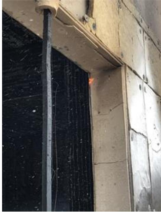
77 - Test 3. Small flame showing from behind gypsum board around opening.
