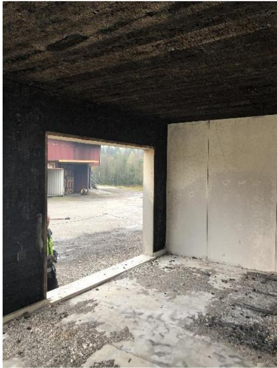
100 - Test 4. Unprotected surfaces after test
