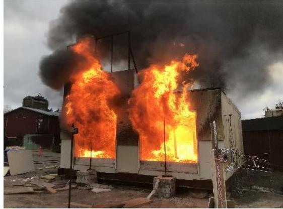
112 - Test 5. Fully developed fire.
