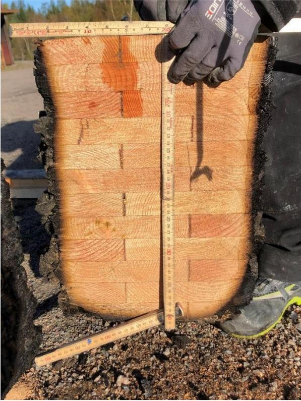
Figure G.3: Post-test beam cross section, Test 3.
