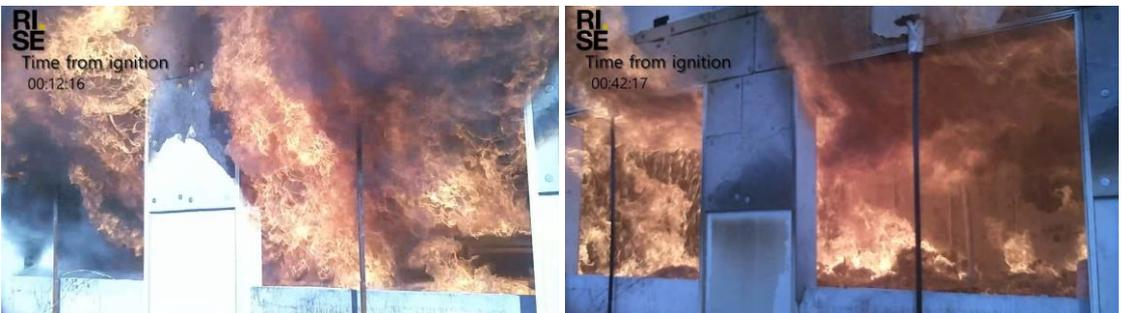
Figure 29: Test 3 - Video snapshots at flashover (left) and 30 minutes after flashover (right)
