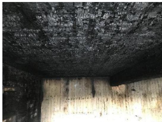
83 - Test 3. Rear wall condition after protection removed.
