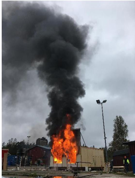
42 - Test 2. Fully developed phase.
