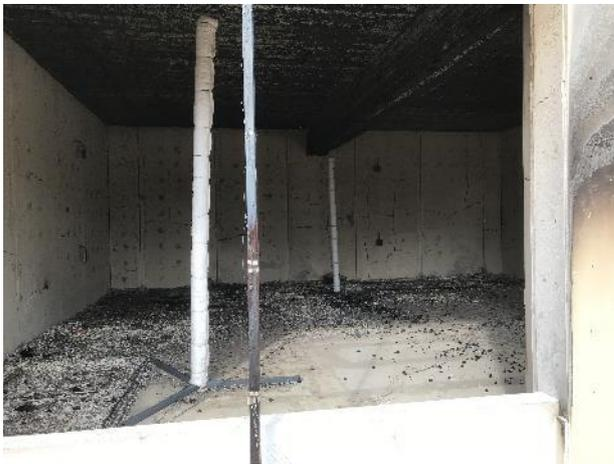
19 - Test 1. Interior post fire (gypsum still attached)
