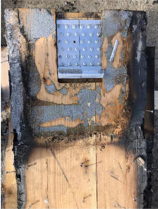
57 - Test 2. Column - beam (on column) connection post fire.
