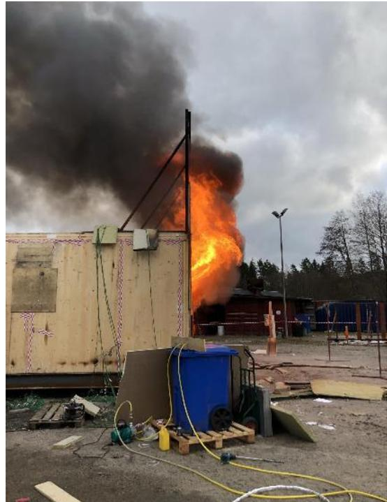
114 - Test 5. Fully developed fire from the side showing flame extension
