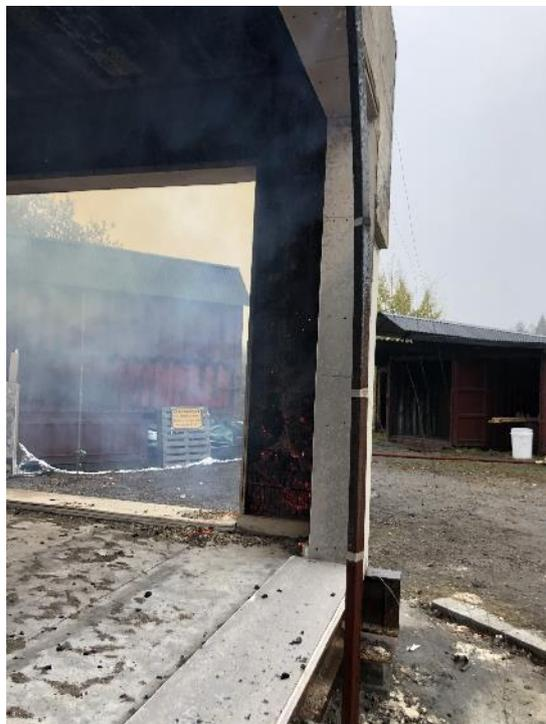
98 - Test 4. Smoldering ongoing in corner after fire stopped elsewhere.
