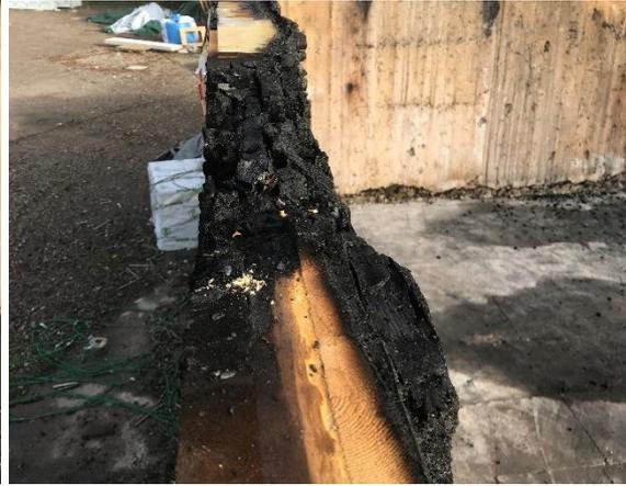
Figure 87: Top of the wall after removal of the ceiling and the resilient profile. Location of flame spread through intersection (front side of left wall) - Sealing method: resilient profile only (Test 3).
