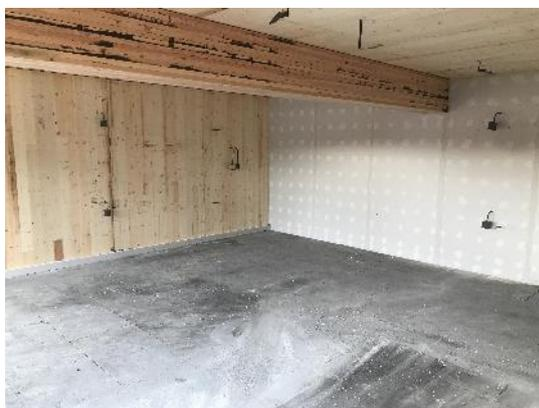
65 - Test 3. Interior of compartment after gypsum applied.
