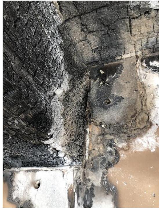
101 - Test 4. Beam wall connection post fire.
