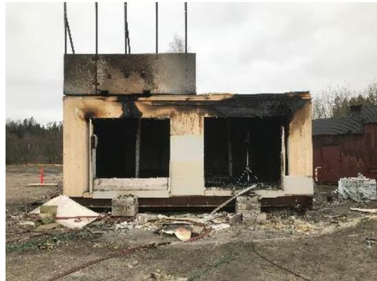
122 - Front of the compartment after protection removed. Areas where fire penetrated the void behind the gypsum boards clearly visible.
