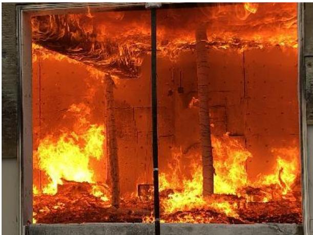
117 - Test 5. Late in the fully developed phase
