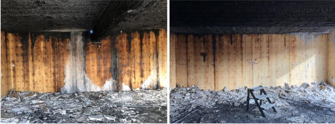
Figure 62: **Test 1**, Back wall (left) and right wall (right) after removal of the 2 gypsum board layers.
