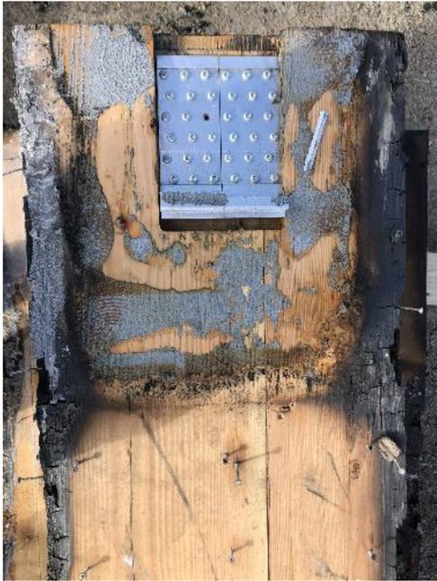
17 - Test 1. Column to beam connection post fire.
