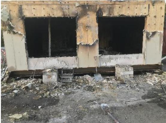
55 – Test 2. Façade after gypsum removal.
