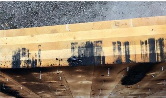
Figure 88: Top of the wall after removal of the ceiling. Typical location. Sealing method: construction tape only (Test 1).
