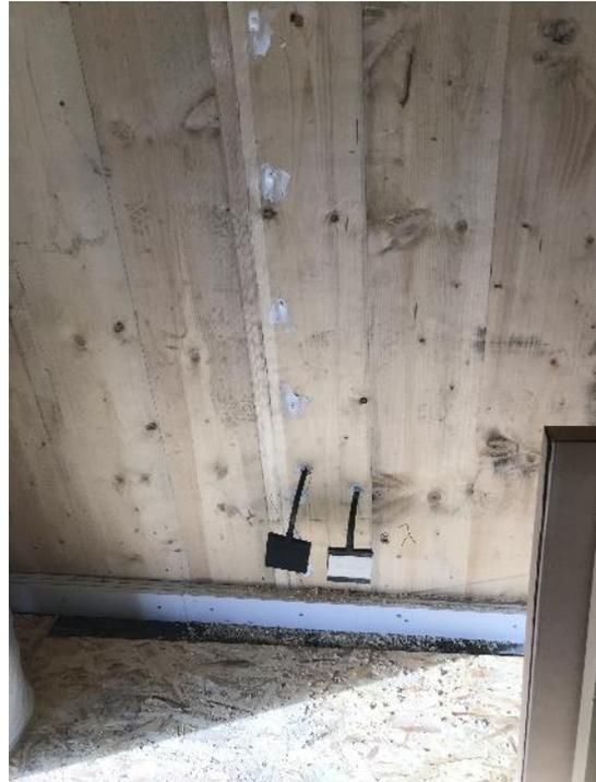
108 - Test 5. Installation of plate thermometers low on the left wall
