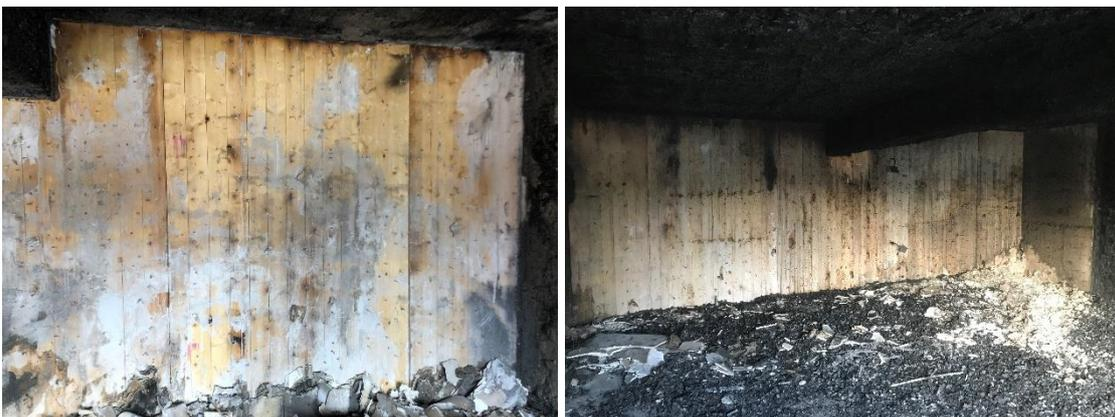
Figure 65: Protected walls of **Test 2** (left) and **Test 3** (right) of left wall after removal of the 3 gypsum board layers.
