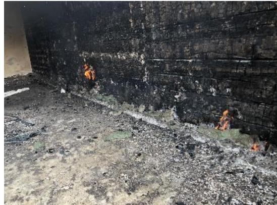
50 - Test 2. Small smoldering areas at end of fire.
