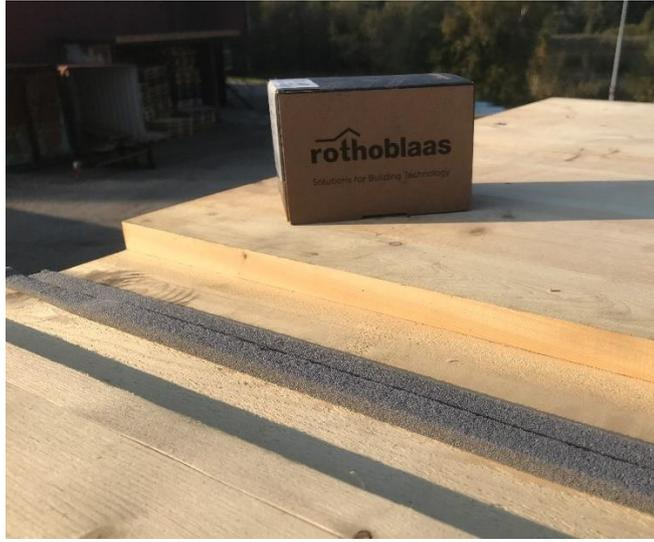
34 - Test 2. Expanding foam tape on the ceiling joint.
