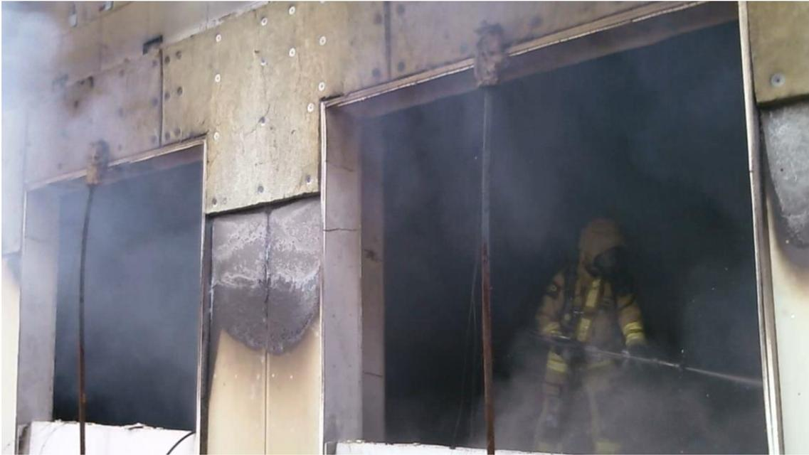
Figure L.6: Systematically cooling all exposed surfaces after directly after Test 2
