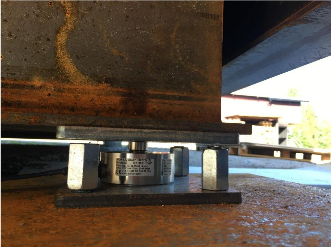
Figure 20: Load cell underneath one of the steel frames
