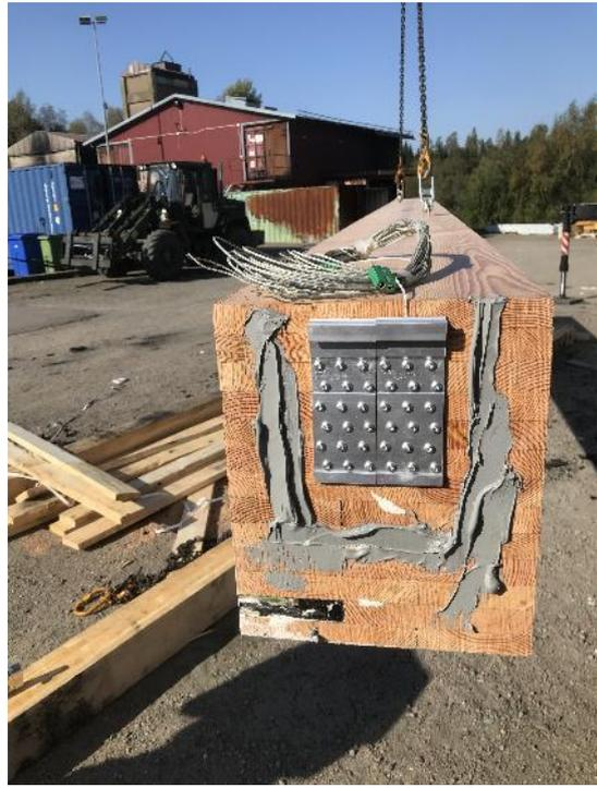
30 - Test 2. Fire sealing on the beam end by column connection.
