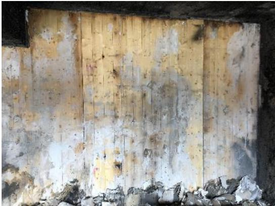
63 - Test 2. Back wall after gypsum removal.
