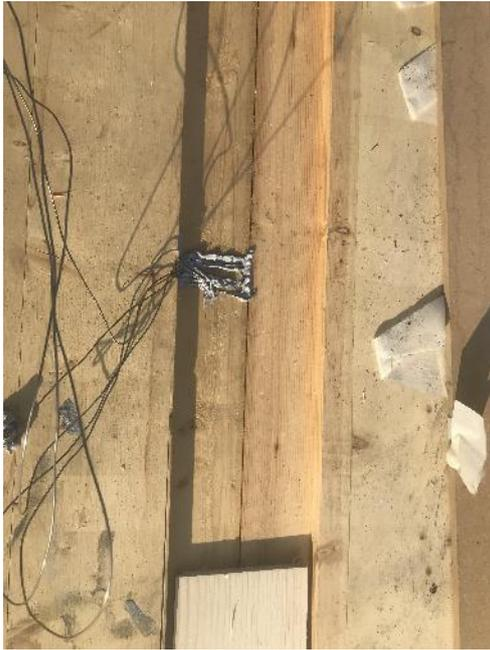
5 - Test 1. Spline board connection additionally sealed at thermocouple locations
