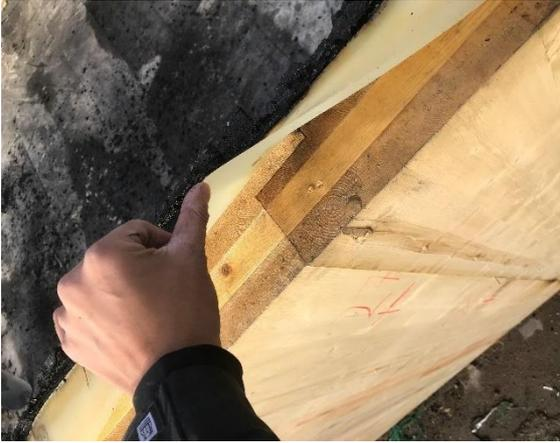
Figure 86: Top of the wall lap joint after removal of the ceiling. Typical location without flame spread. Sealing method: resilient profile only (Test 3).
