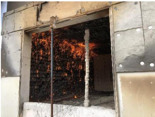
74 - Test 3. Flaming on the left wall late in the decay
