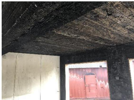
99 - Test 4. Unprotected surfaces after test.
