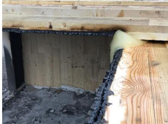
108- Test 4. Rear wall after removal of gypsum.
