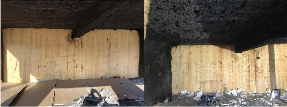
Figure 66: Protected walls of Test 4 (left, 2 GB layers) and Test 5 (right, 3 GB layers) after removal of gypsum boards.
