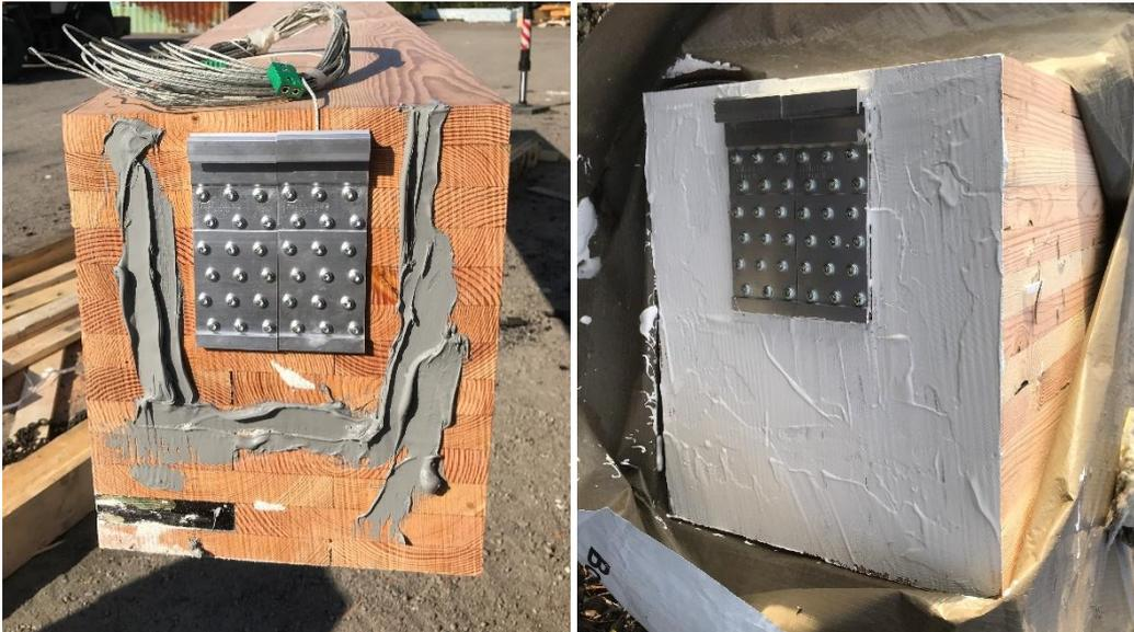
Figure 10: Fire sealant applied on the beam for Test 1 and 2 (left) intumescent paint applied on the beam for Test 3, 4 and 5 (right)
