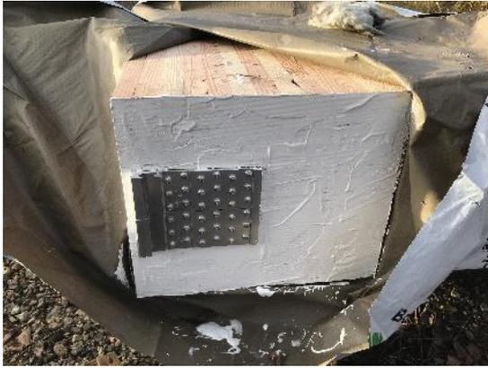
107 - Test 5. Beam end protected with intumescent paint.
