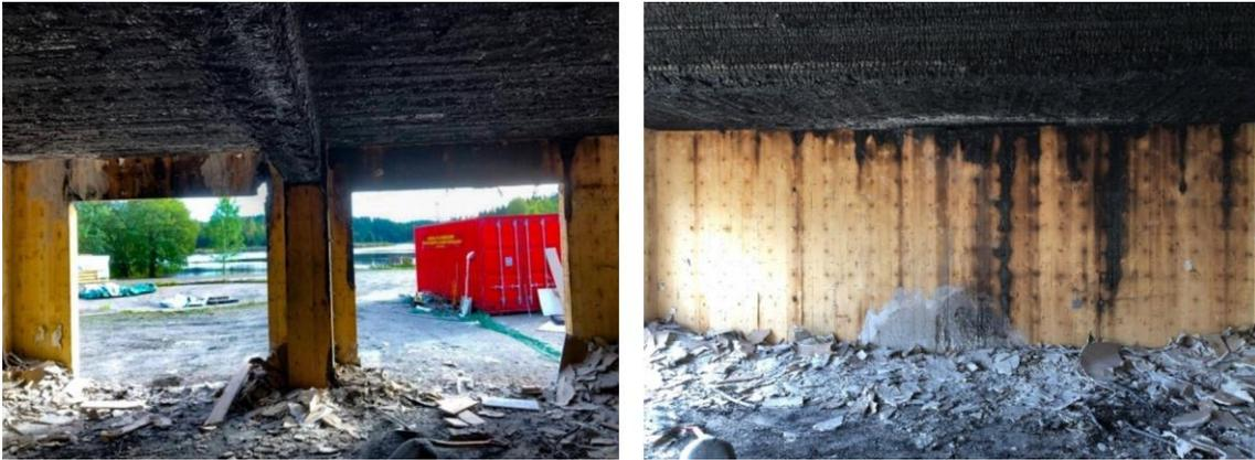
Figure 63: **Test 1**, Front wall (left) and left wall (right) after removal of the 2 gypsum board layers.
