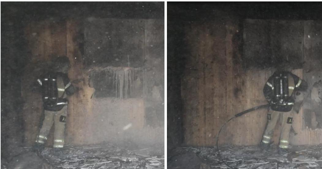
Figure L.8: Applying water mist behind the boards for a few seconds, separating the board from the wall (left), removing the board by hand (right).
