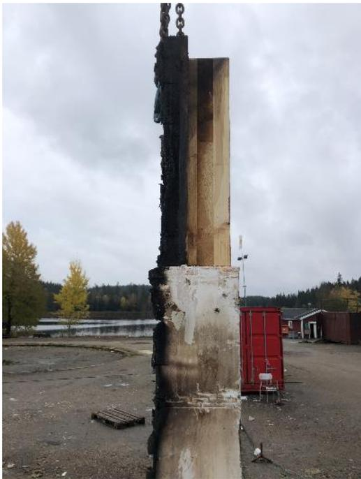
109 - Test 4. Beam after partial removal of the roof showing the resilient profile.
