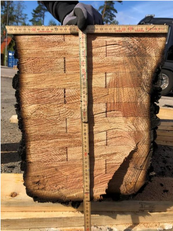
Figure G.1: Post-test beam cross section, **Test 1**.
