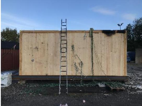
84 - Test 3. Area of charring visible from outside post test.
