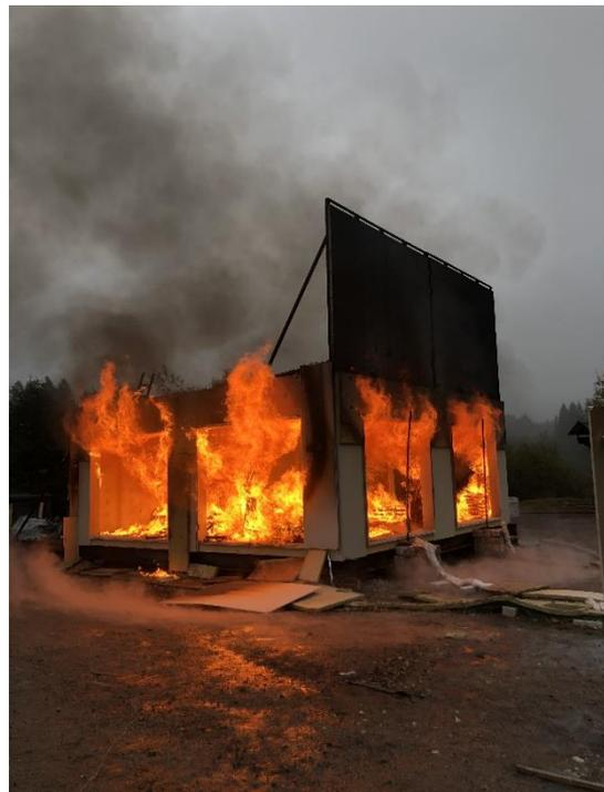
95 - Test 4. Fully developed fire.
