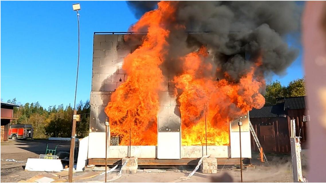
Figure F.5 Test 3 17min 45s after ignition
