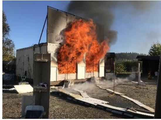
69 – Test 3. Fully developed fire.
