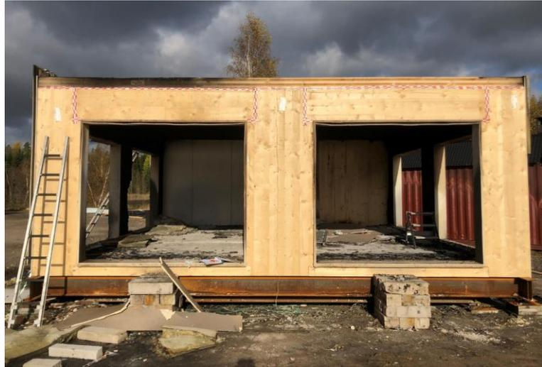
Figure 99: Test 4 - Detail above opening (left) and front façade after removal of gypsum boards.
