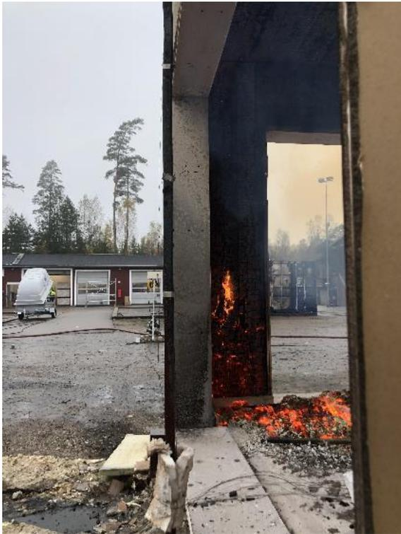
96 - Test 4. Smoldering in front left corner of compartment.
