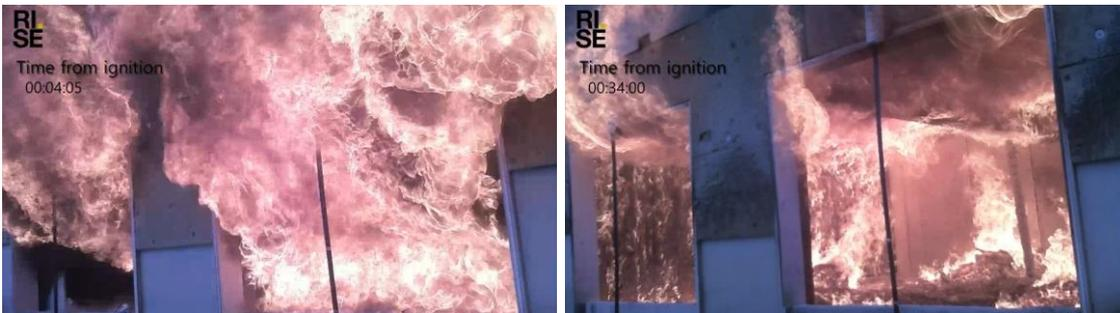
Figure 35: Test 5 - Video snapshots at flashover (left) and 30 minutes after flashover (right)
