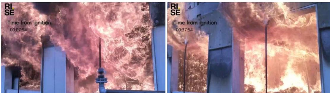
Figure 26: Test 2 - Video snapshots at flashover (left) and 30 min after flashover (right)
