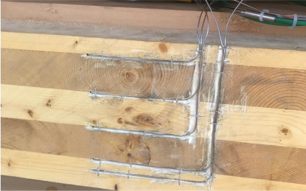
Figure 15: Thermocouples installed at the spline board joint of the ceiling. The thermocouple tip is located at a depth of 75 mm from the visible surface.
