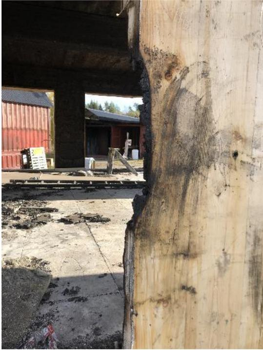
104 - Test 4. Wall section from outside. (same as photo 100 but from the outside and after removal of GB and char due to a local smoldering fire at the position of inserted thermocouples)
