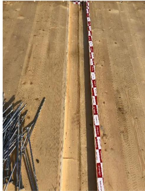
22 - Test 1. Roof joint post fire, no visible charring on unexposed surface at joint.
