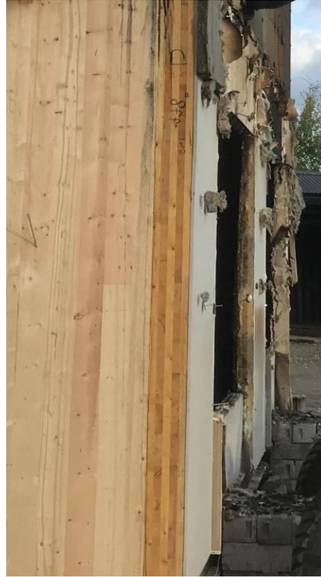
Figure 94: Typical wall-wall butt joint with construction sealing after the test.
