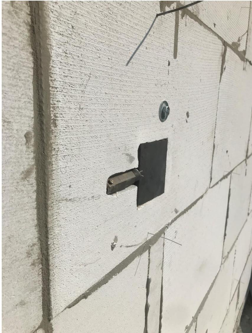
Figure 18: PT 4 embedded flush to the façade surface. Under the PT a 1 mm diameter TC (TC 7) extrudes 5 cm and above a 3 mm diameter TC extrudes 10 cm.
