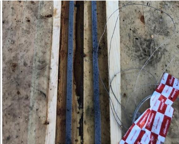
Figure 93: Photo after removal of spline board. Sealing method: 2x expanding tape at center of lap (Test 3). Note: the rain after the test cause additional discoloration
