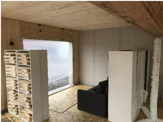
90 - Test 4. Light plastic sheeting covering openings to prevent wind for blowing out fire in very early stages.
