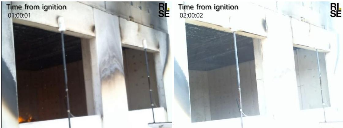
Figure 24: Test 1 - Video snapshots at 1 hour (left) and 2 hours (right) after ignition
