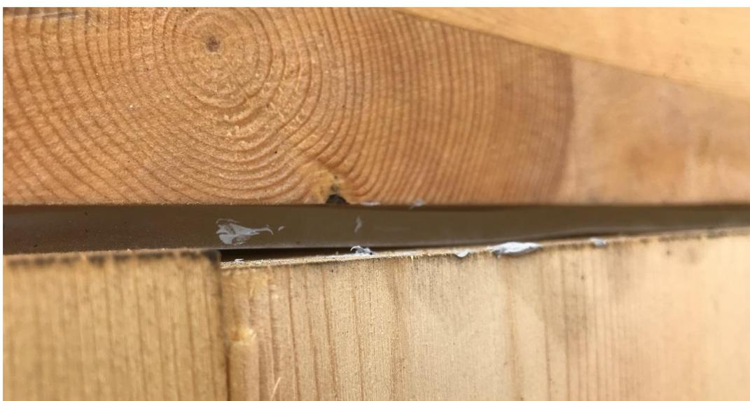
Figure 85: Location of imperfect detail at wall-ceiling joint with a resilient profile identified before the test
