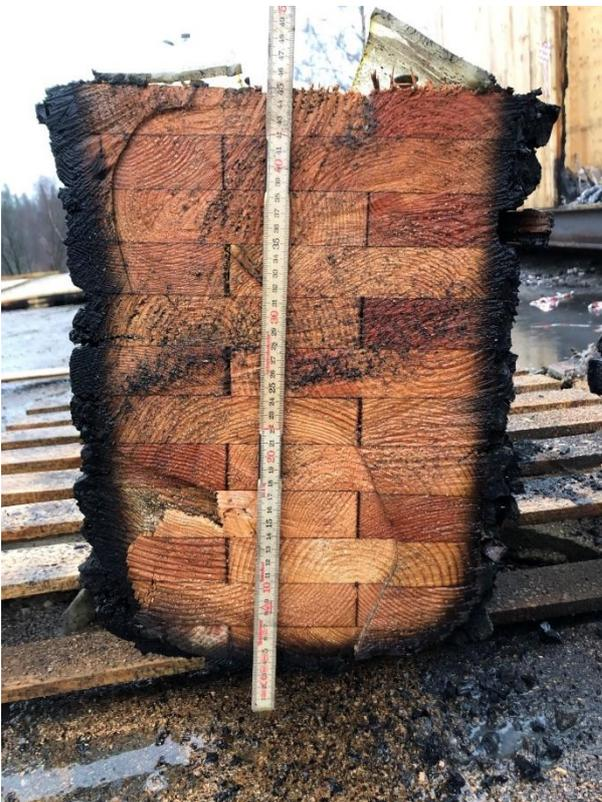
Figure G.4: Post-test beam cross section, Test 5.
