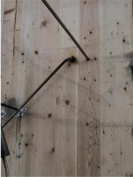
76 - Test 3. Small amount of discoloration visible on the unexposed side of the back wall around pipe penetration (for oxygen measurements)
