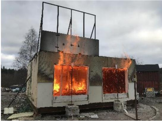
115 - Test 5. Late in the fully developed phase
