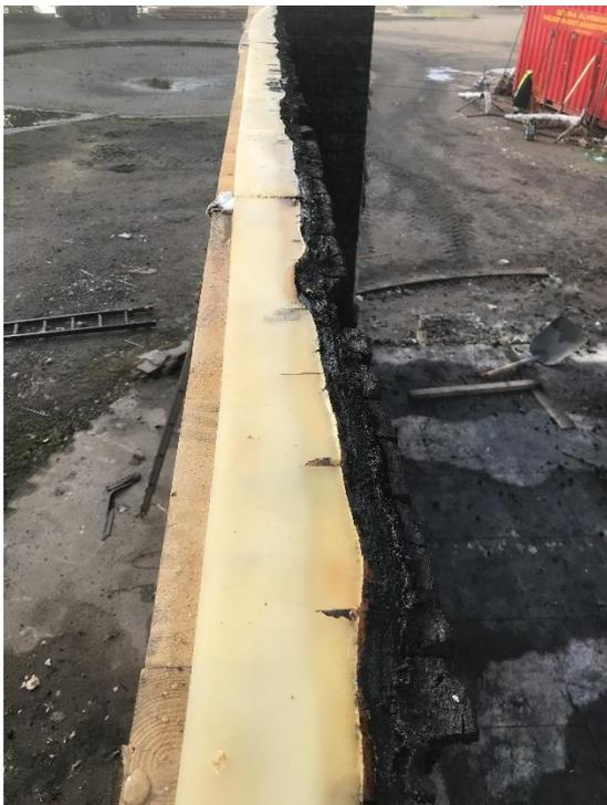
86 - Test 3. Demonstration of resilient profile providing protection at the wall-ceiling interface.
