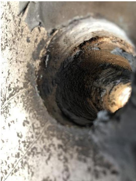
23 - Test 1. Penetration for instrumentation in wall, no visible charring within the hole.
