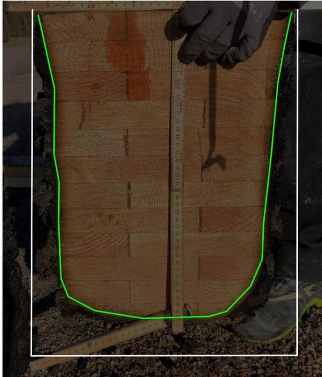
Figure 79: Example sketch of how the charred cross-sectional shape is established from a photo. Green line shows the char boundary and the white the original beam cross-section.
