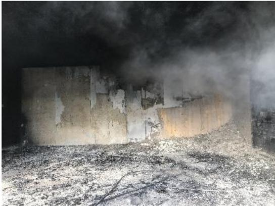
78 - Test 3. Post fire gypsum removal from rear wall.
