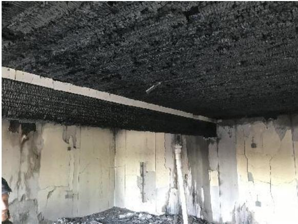
21 - Test 1. Exposed roof and beam post fire.
