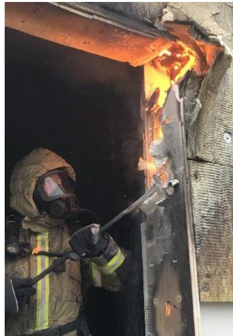
118 - Fire fighter removing gypsum around opening showing penetration of fire into the cavity behind the protection. This cavity was only present in Test 5.
