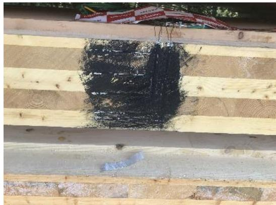
32 - Test 2. Sealant over TCs installed in CLT.
