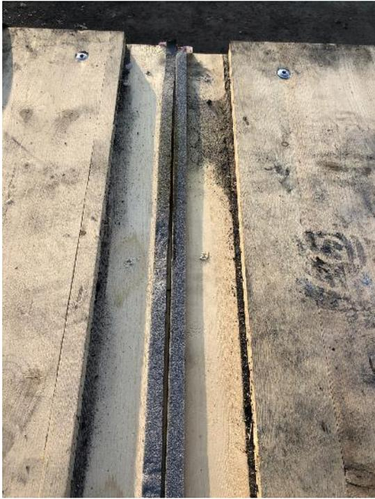
61 - Test 2. Ceiling spline board joint post fire.
