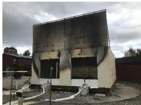
20 - Test 1. Exterior post fire (protection still attached)
