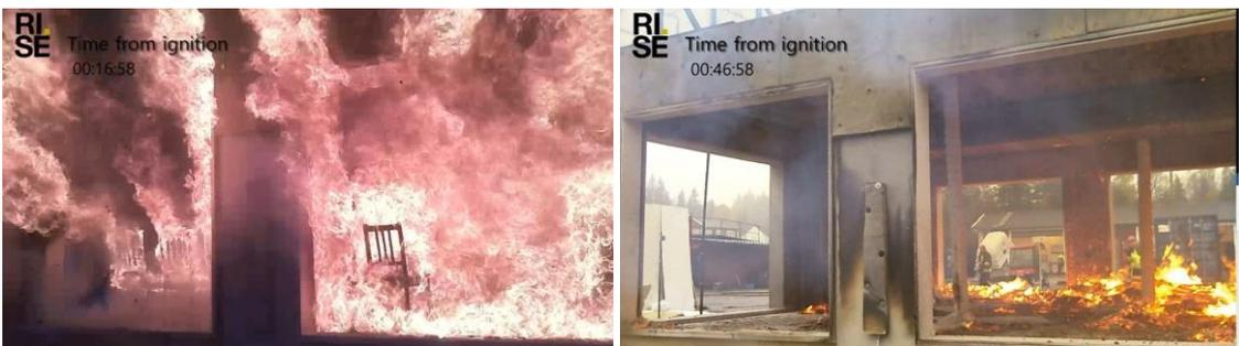
Figure 32: Test 4 - Video snapshots at flashover (left) and 30 minutes after flashover (right)
