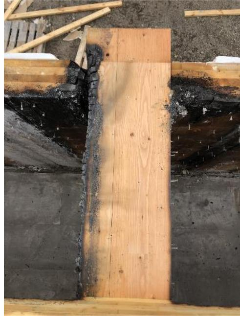
18 - Test 1. Post fire, beam penetrating through rear wall. Charring visible on the left where gap wasn't sufficiently sealed (see Section, 6.15), none visible on the right.
