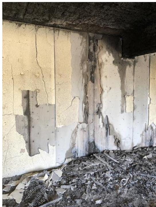
24 - Test 1. Gypsum post fire after using a water mist extinguisher to extinguish local smoldering.
