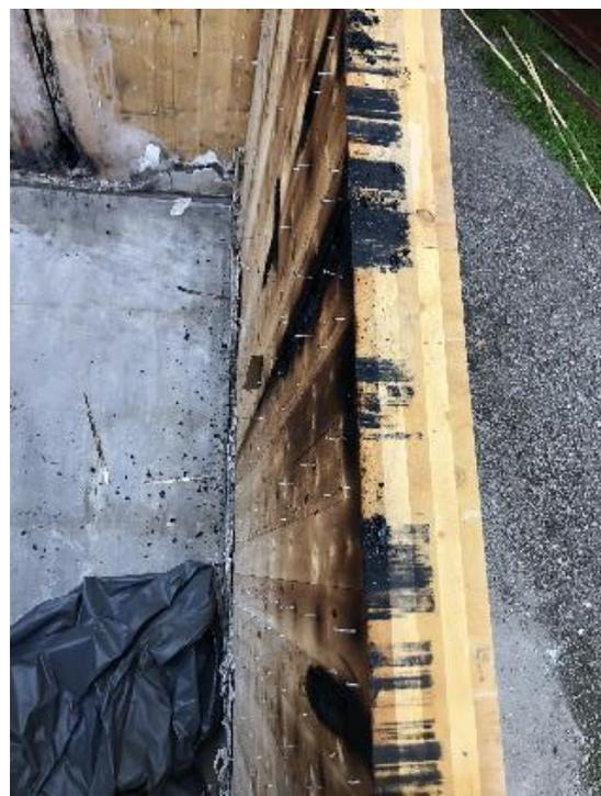
60 - Test 2. Protected wall post fire and gypsum removal.
