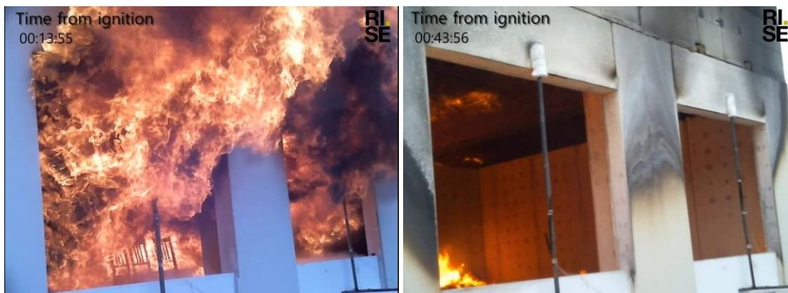
Figure 23: Test 1 - Video snapshots at flashover (left) and 30 minutes after flashover (right)
