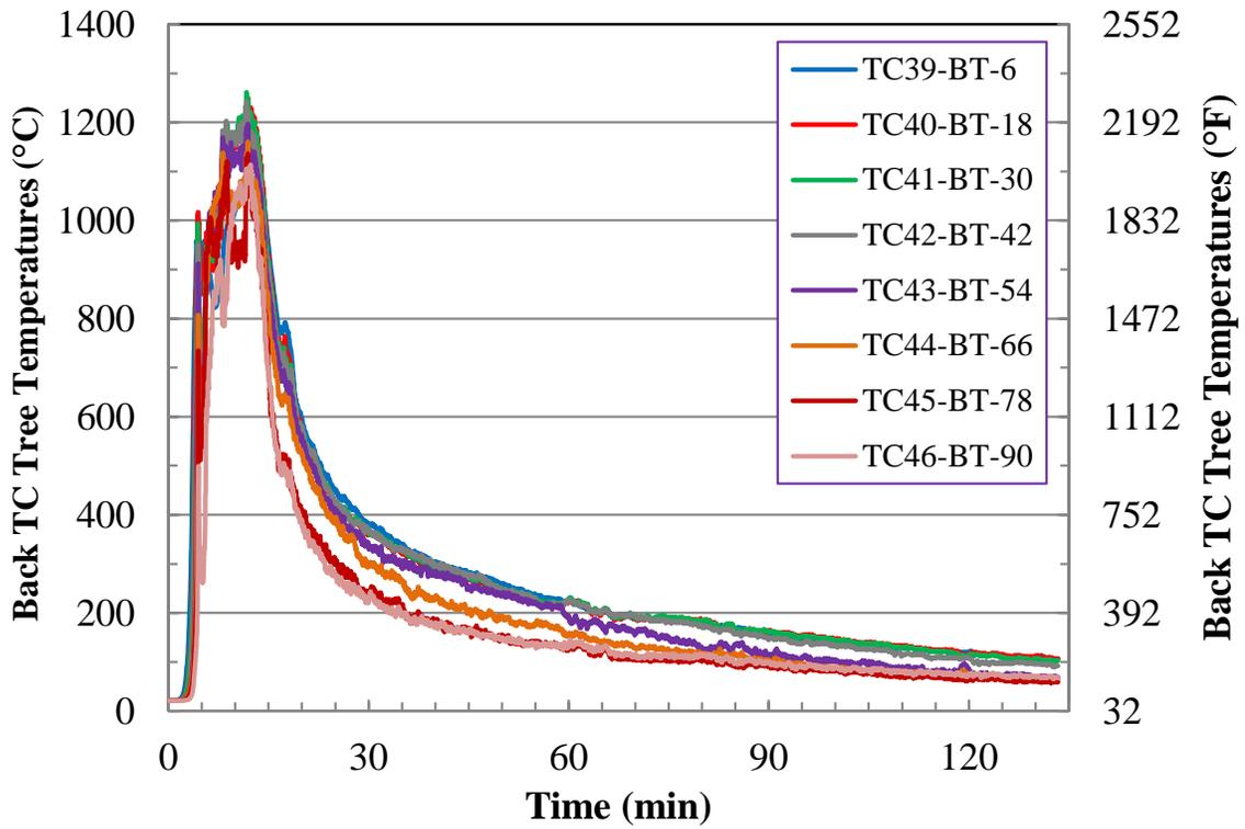
Figure E-16. Test 2 Back Interior TC Tree Temperatures.
