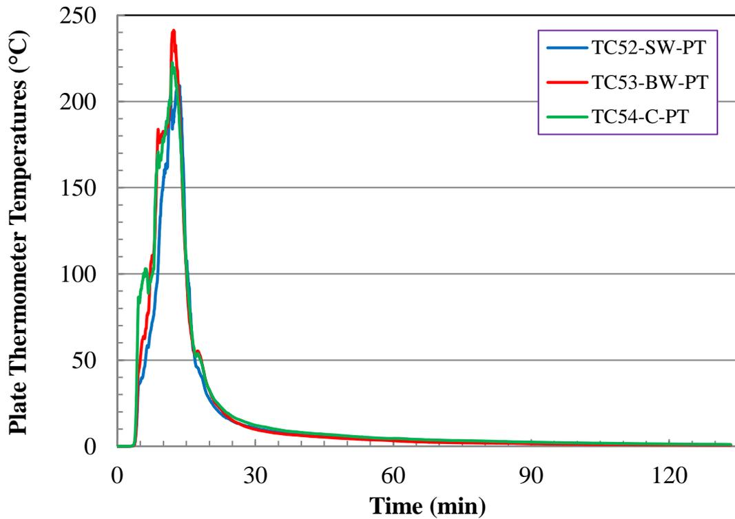
Figure E-22. Test 1 Plate Thermometer Heat Fluxes.
