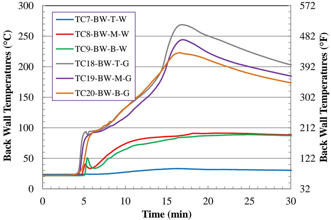
Figure C-7. Test 1 Back Wall Temperatures (First 30 min).
