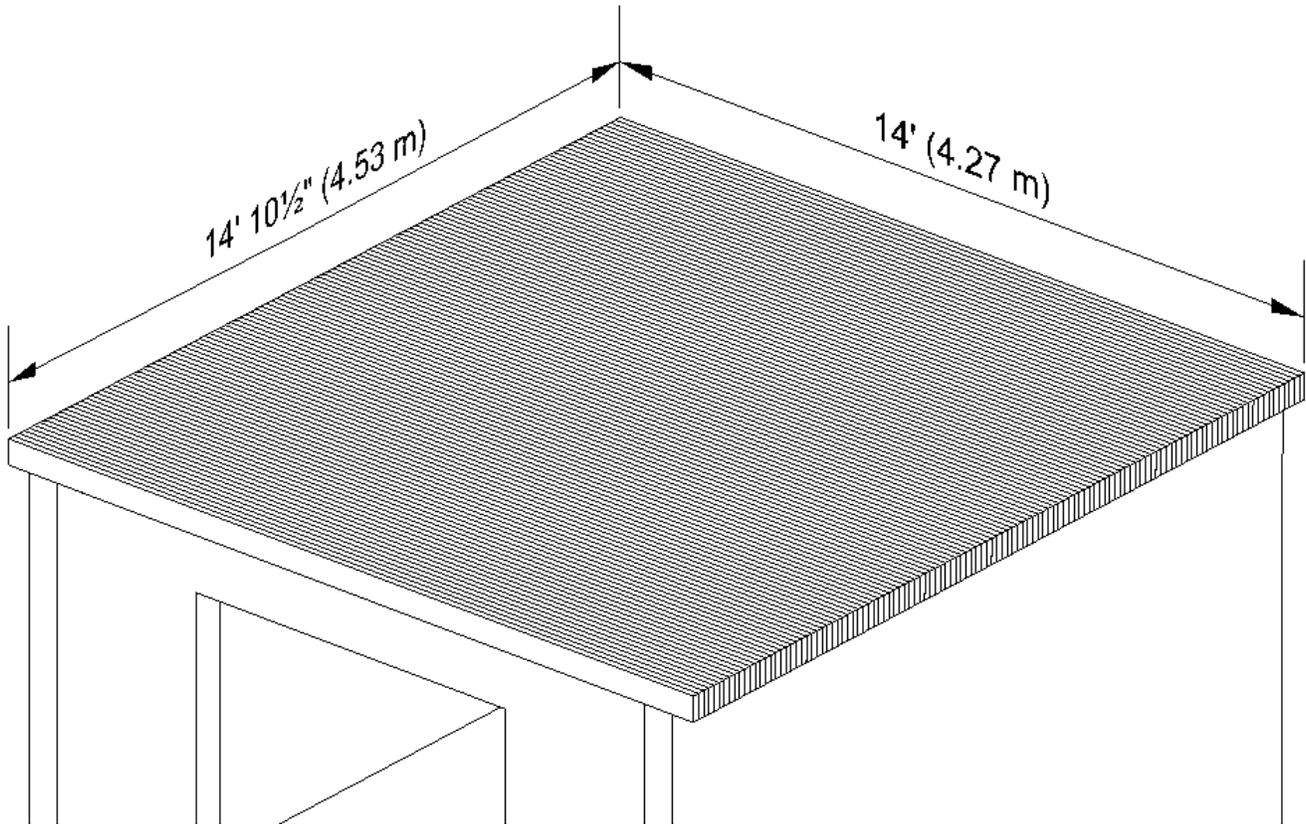
**Figure 3. NLT Ceiling for Test 1 Compartment.**
