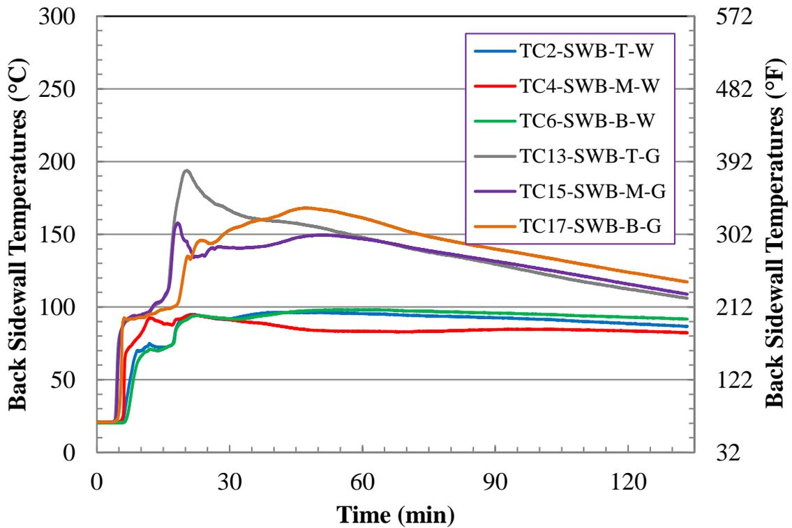
Figure E-6. Test 2 Back Sidewall Temperatures.
