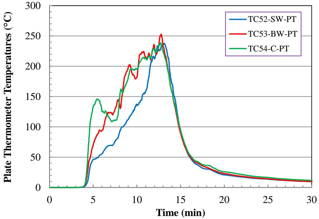
Figure C-21. Test 1 Plate Thermometer Heat Fluxes (First 30 min).
