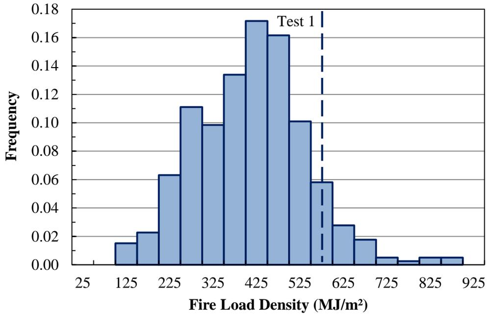
**Figure 6. Test 1 vs. Fire Load Density Frequency Distribution from Canadian Survey.**
