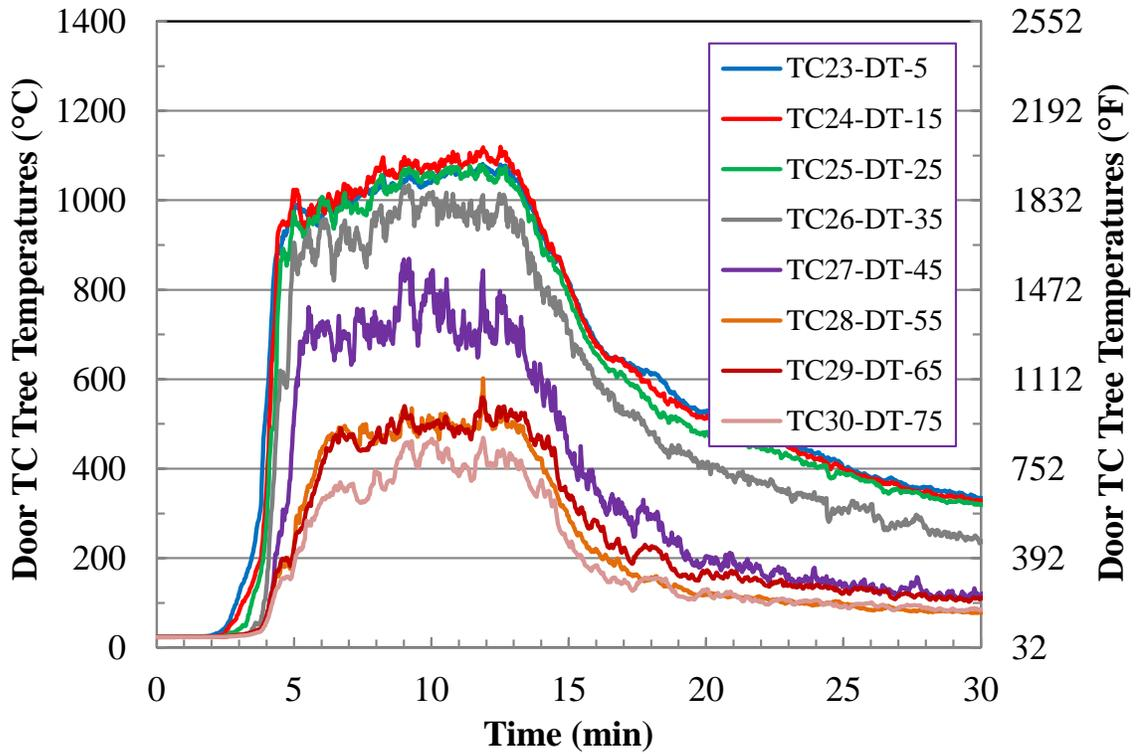
Figure C-11. Test 1 Door TC Tree Temperatures (First 30 min).
