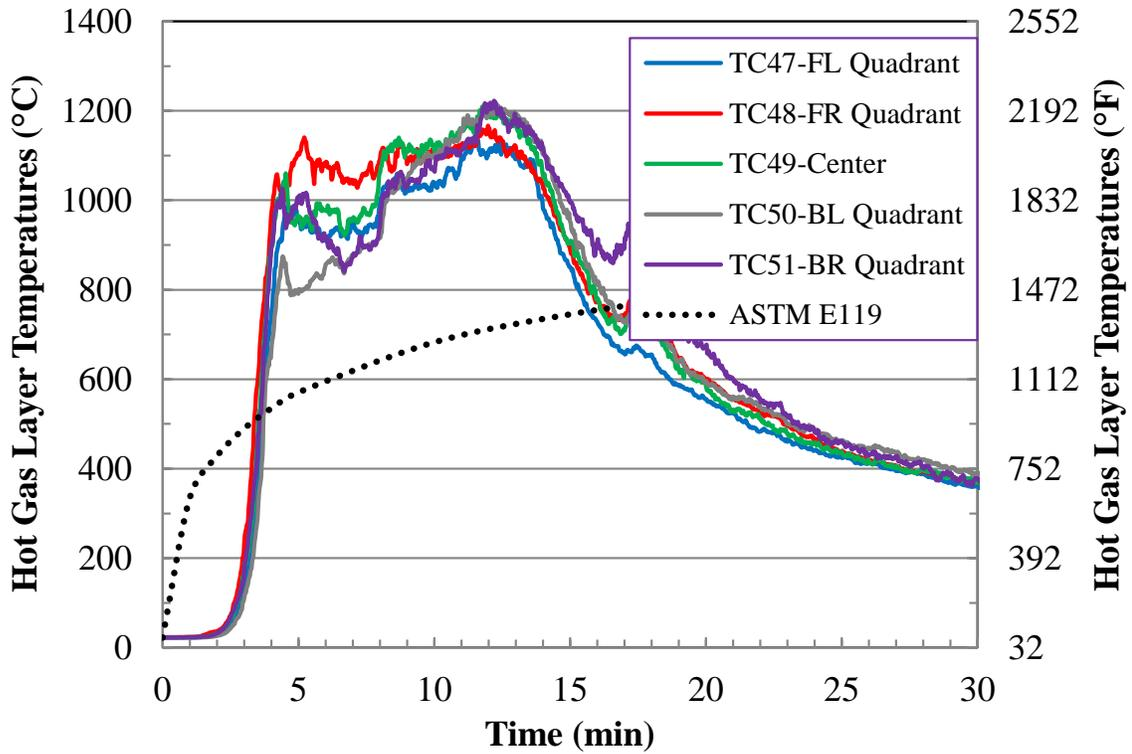
Figure E-17. Test 2 Hot Gas Layer Temperatures (First 30 min).
