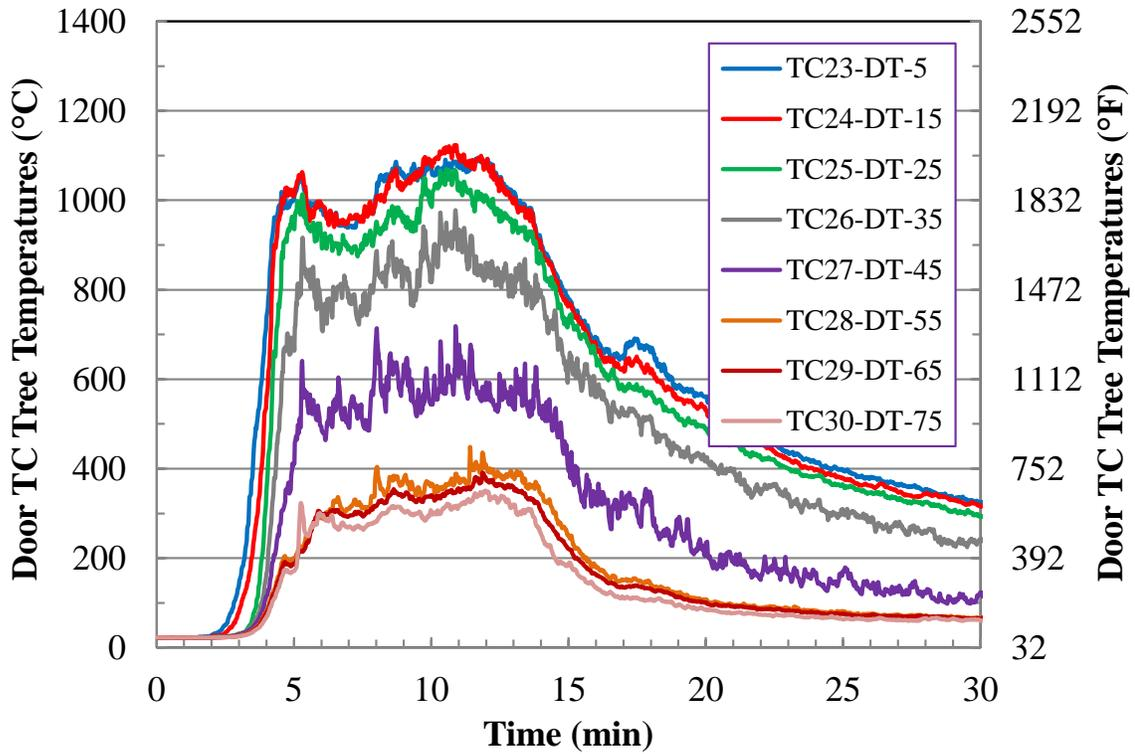
Figure E-11. Test 2 Door TC Tree Temperatures (First 30 min).
