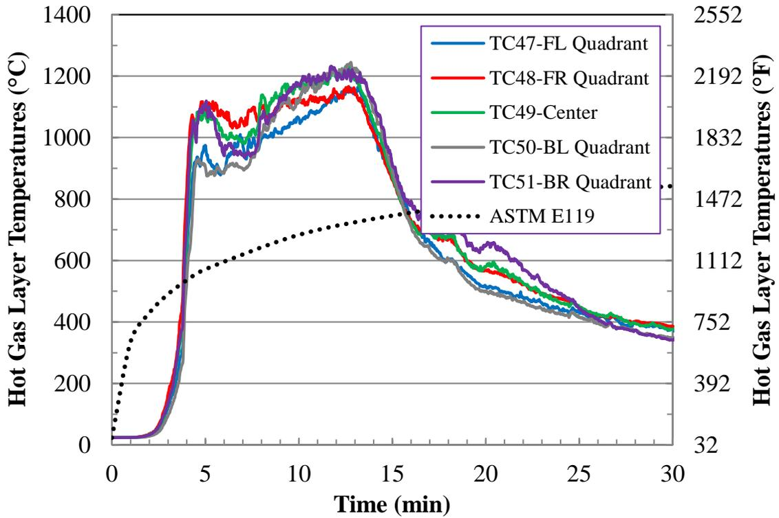
Figure C-17. Test 1 Hot Gas Layer Temperatures (First 30 min).
