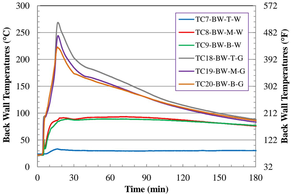
Figure C-8. Test 1 Back Wall Temperatures.
