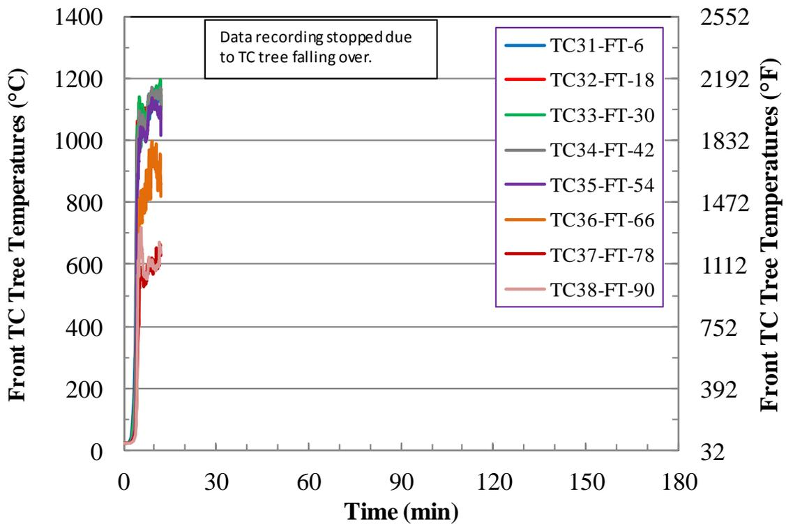
Figure C-14. Test 1 Front Interior TC Tree Temperatures.
