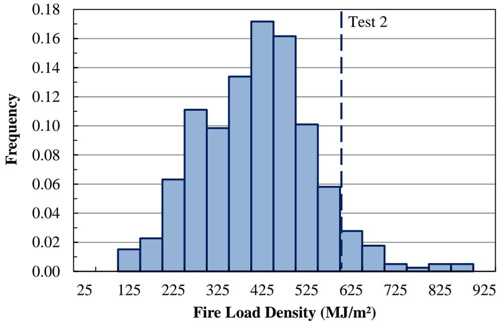
**Figure 9. Test 2 vs. Fire Load Density Frequency Distribution from Canadian Survey.**
