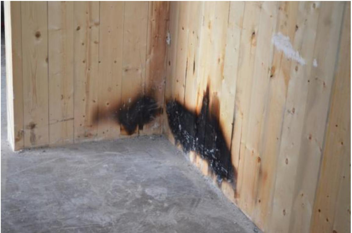
**Figure B-36. Charring in Front Left Corner Post-Test.**
