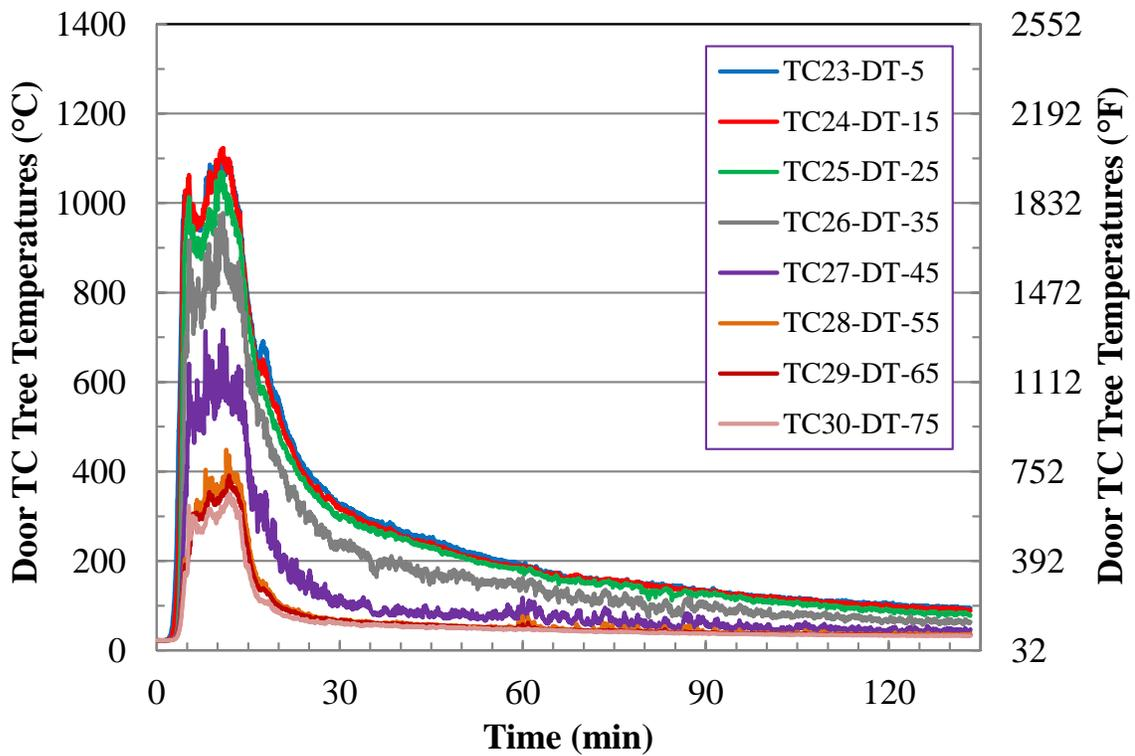
Figure E-12. Test 2 Door TC Tree Temperatures.
