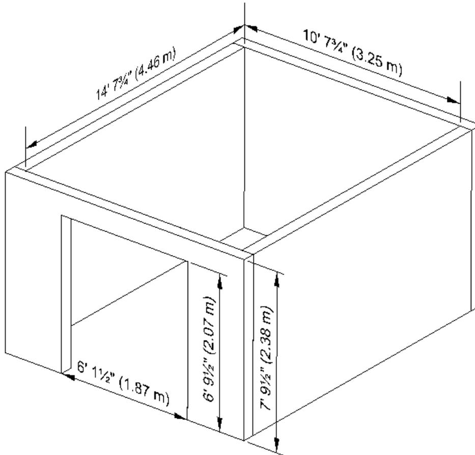
**Figure 8. CLT Wall Panel Assembly for Test 2 Compartment.**
