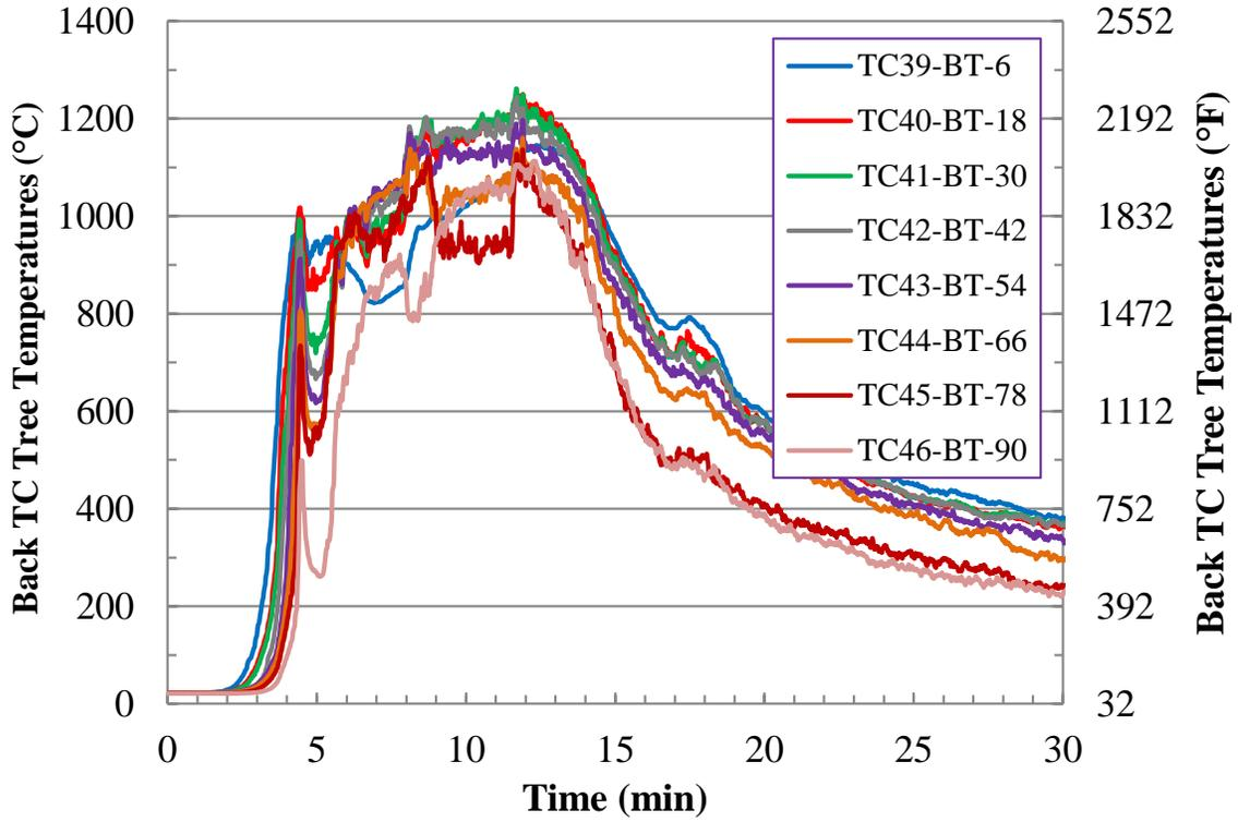
Figure E-15. Test 2 Back Interior TC Tree Temperatures (First 30 min).
