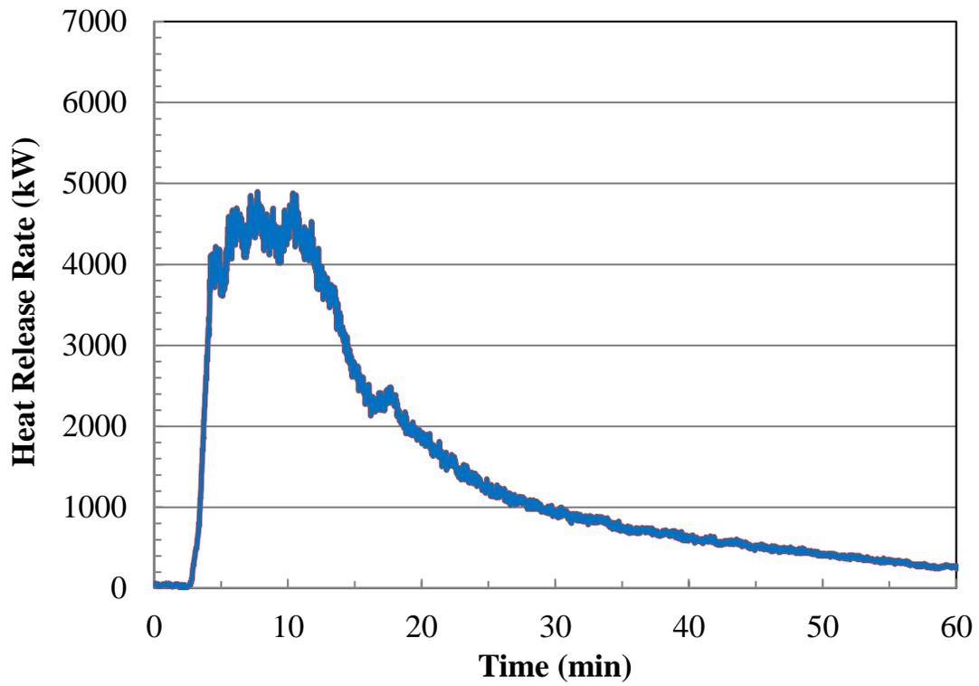
**Figure E-2. Test 2 Heat Release Rate (First 30 min).**
