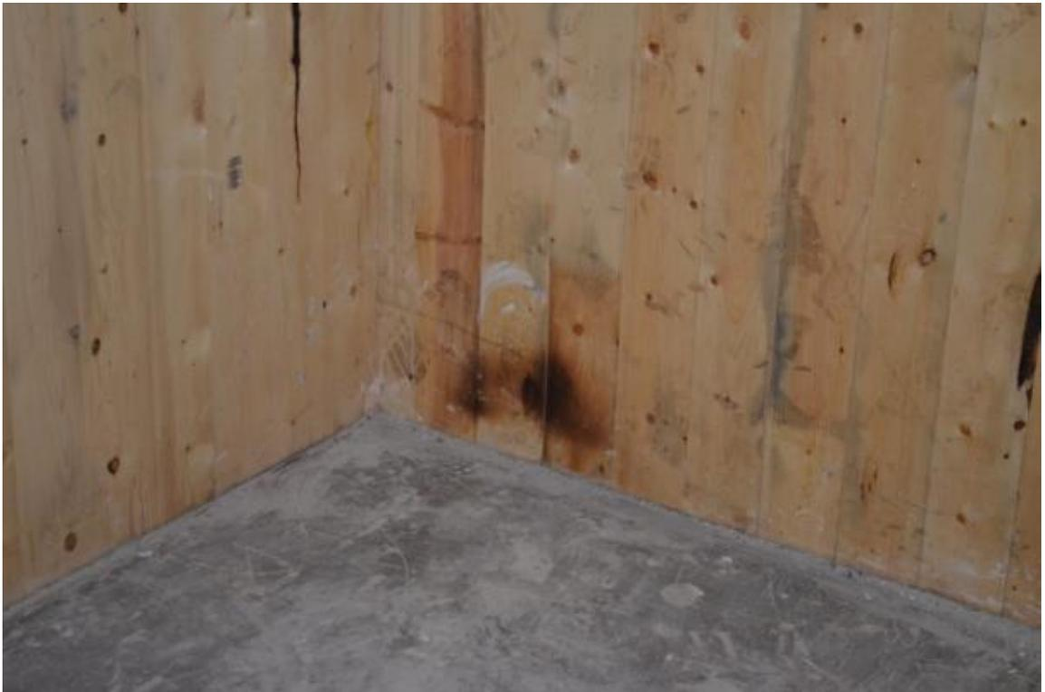
**Figure B-36. Charring in Back Right Corner Post-Test.**
