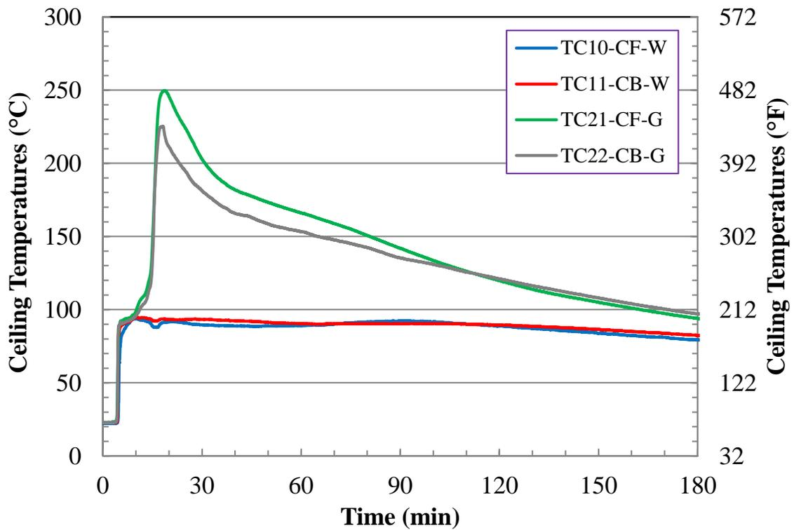
Figure C-10. Test 1 Ceiling Temperatures.
