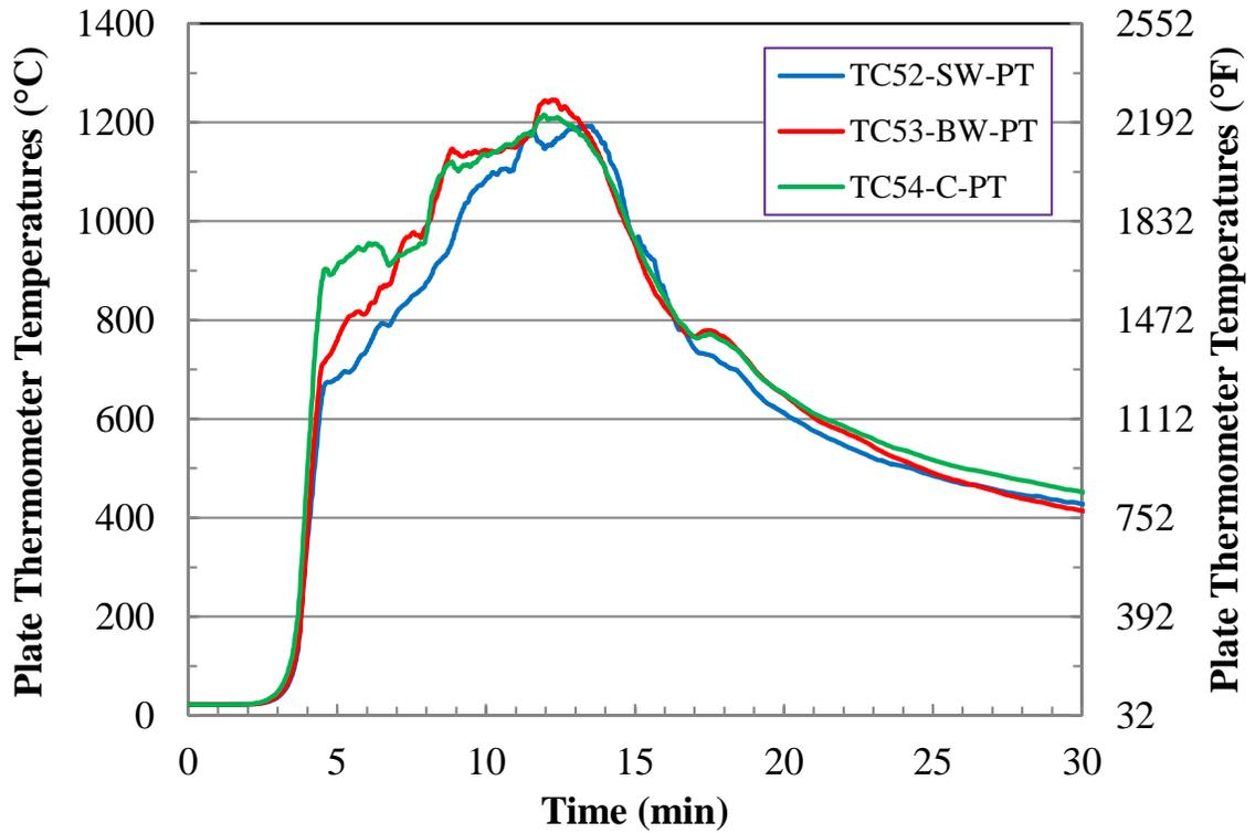
Figure E-19. Test 2 Plate Thermometer Temperatures (First 30 min).
