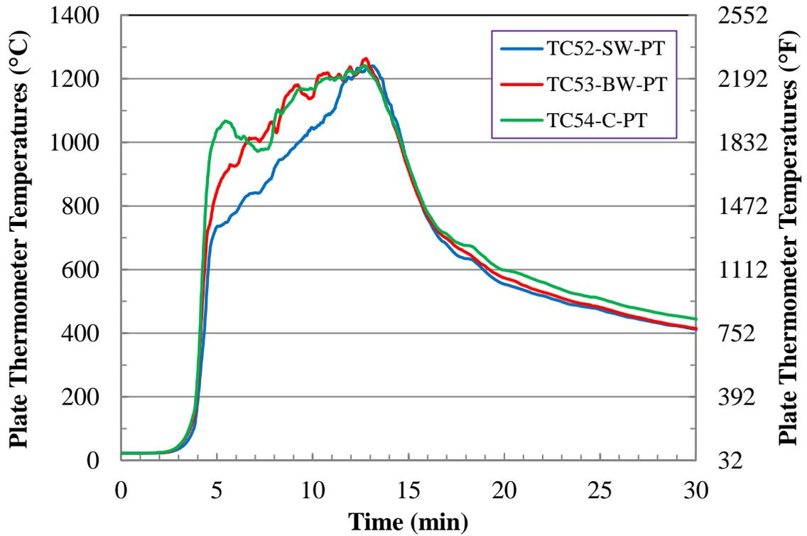
Figure C-19. Test 1 Plate Thermometer Temperatures (First 30 min).
