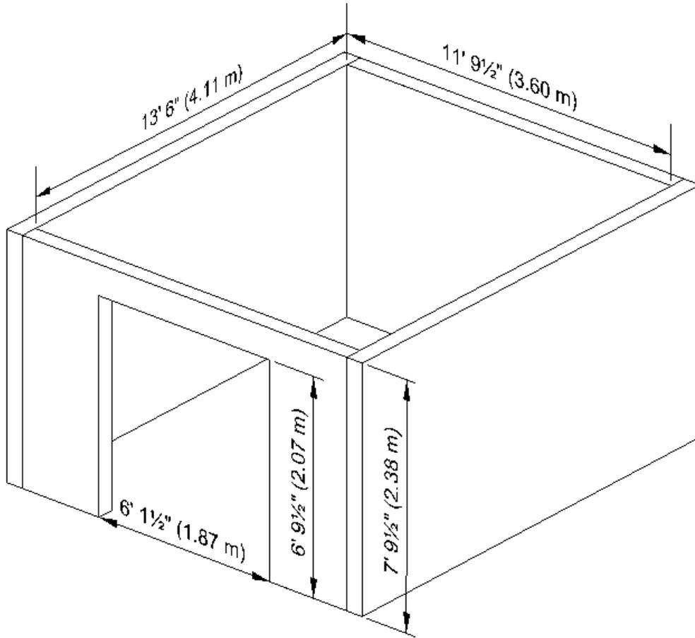
**Figure 1. CLT Wall Panel Assembly for Test 1 Compartment.**
