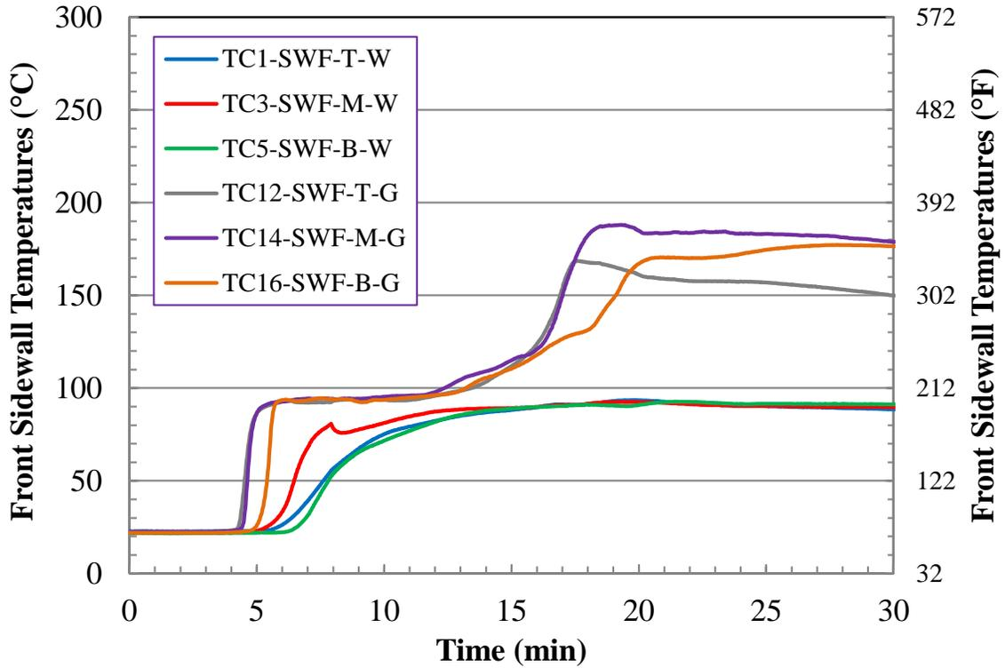
Figure C-3. Test 1 Front Sidewall Temperatures (First 30 min).
