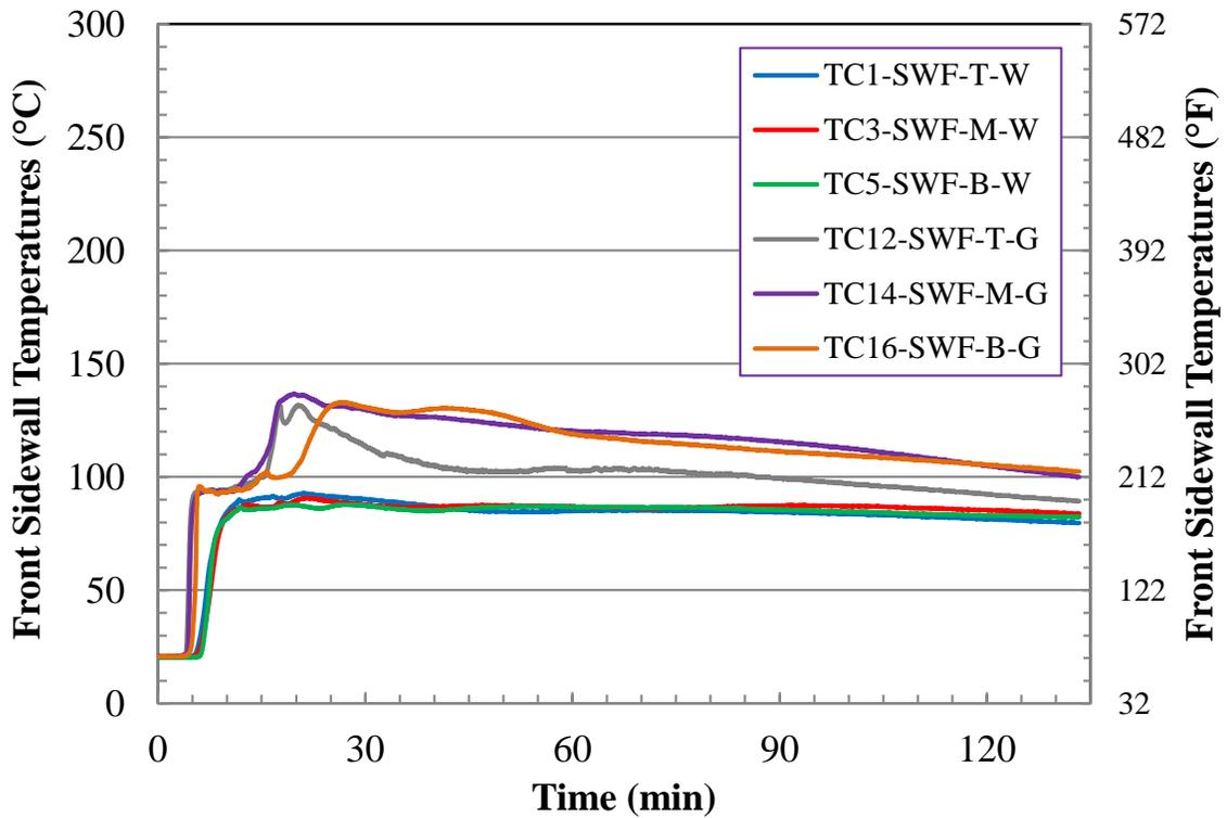
Figure E-4. Test 2 Front Sidewall Temperatures.
