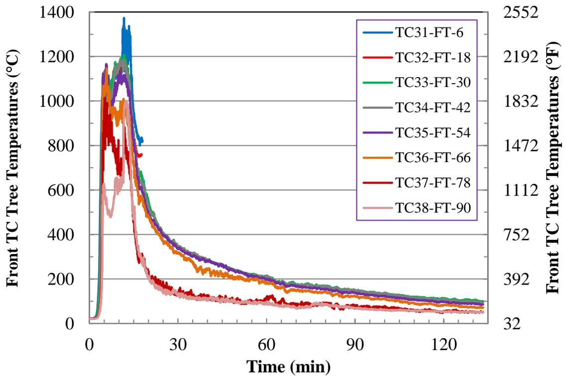
Figure E-14. Test 2 Front Interior TC Tree Temperatures.
