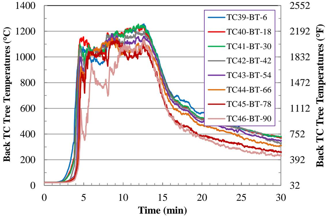
Figure C-15. Test 1 Back Interior TC Tree Temperatures (First 30 min).
