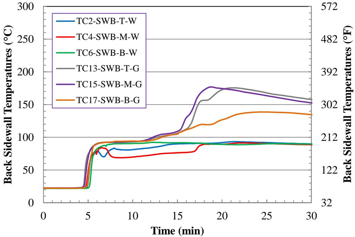
Figure C-5. Test 1 Back Sidewall Temperatures (First 30 min).
