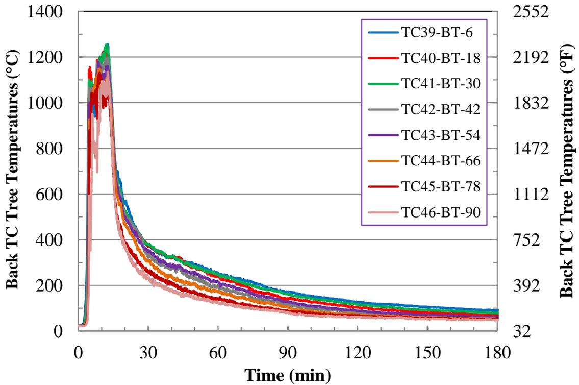
Figure C-16. Test 1 Back Interior TC Tree Temperatures.
