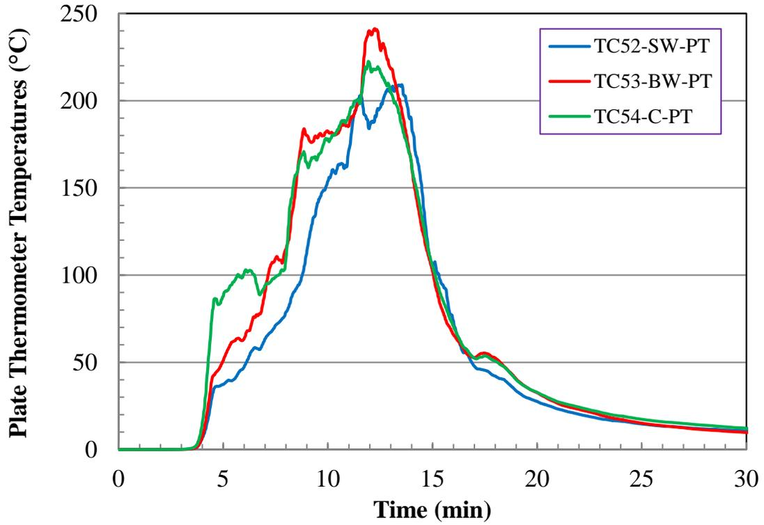
Figure E-21. Test 2 Plate Thermometer Heat Fluxes (First 30 min).
