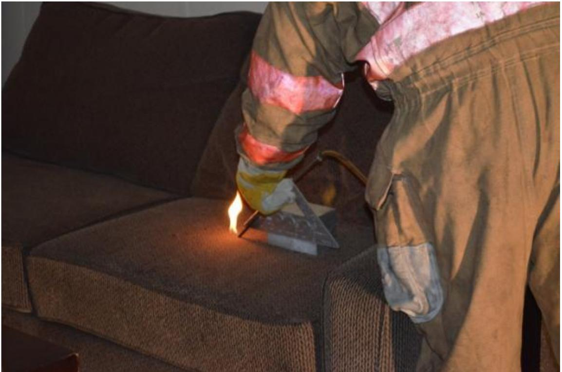
**Figure B-16. Start of Test (Application of BS5852 Ignition Source 2).**
