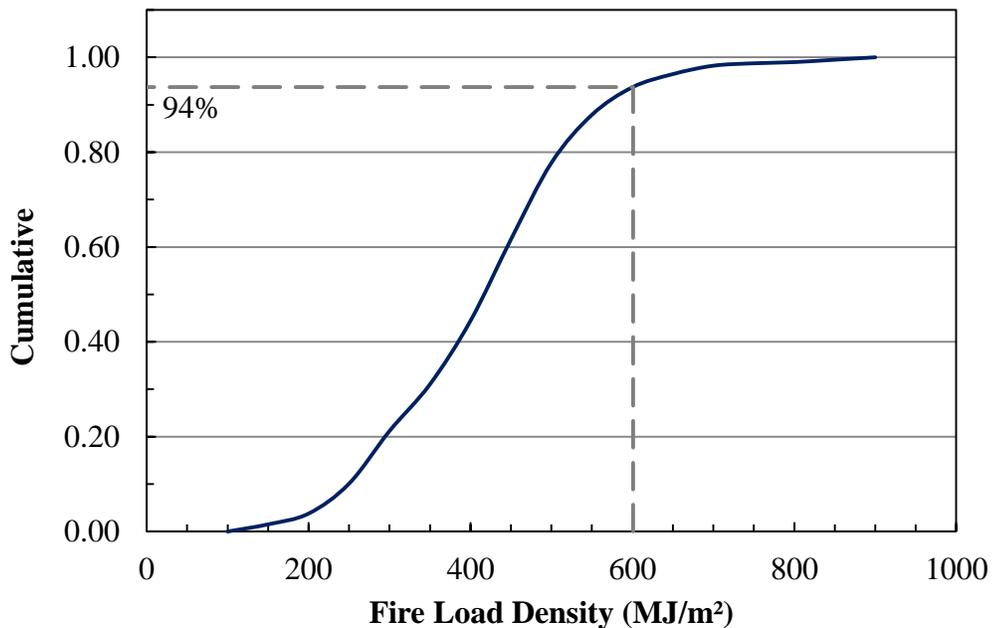
**Figure 10. Test 2 vs. Cumulative Fire Load Density Distribution from Canadian Survey.**
