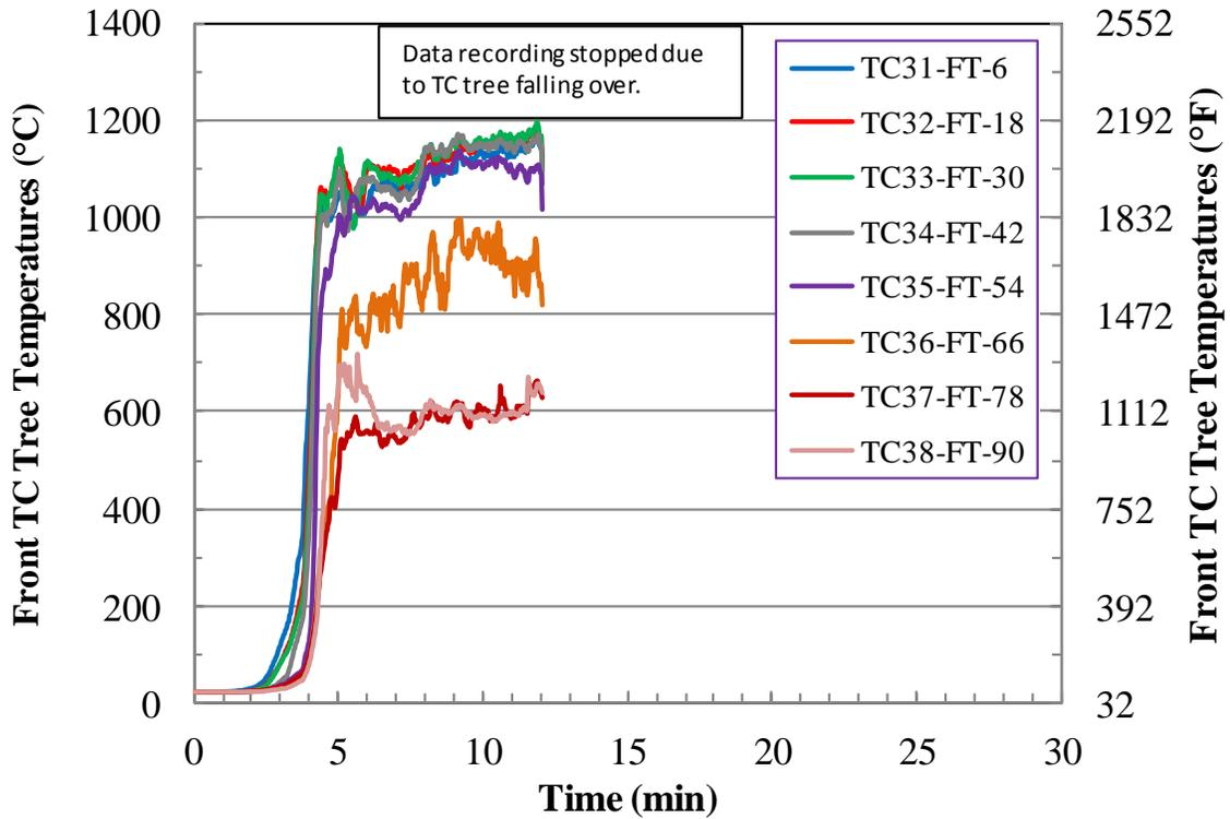
Figure C-13. Test 1 Front Interior TC Tree Temperatures (First 30 min).
