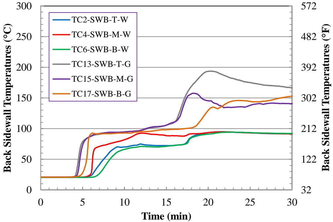
Figure E-5. Test 2 Back Sidewall Temperatures (First 30 min).
