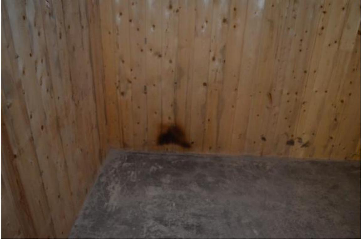
**Figure B-35. Charring in Back Left Corner Post-Test.**
