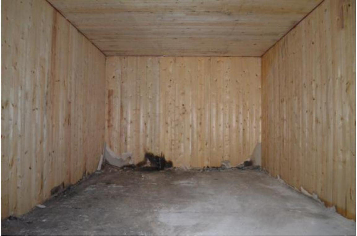
**Figure D-31. CLT Structure Post-Test.**
