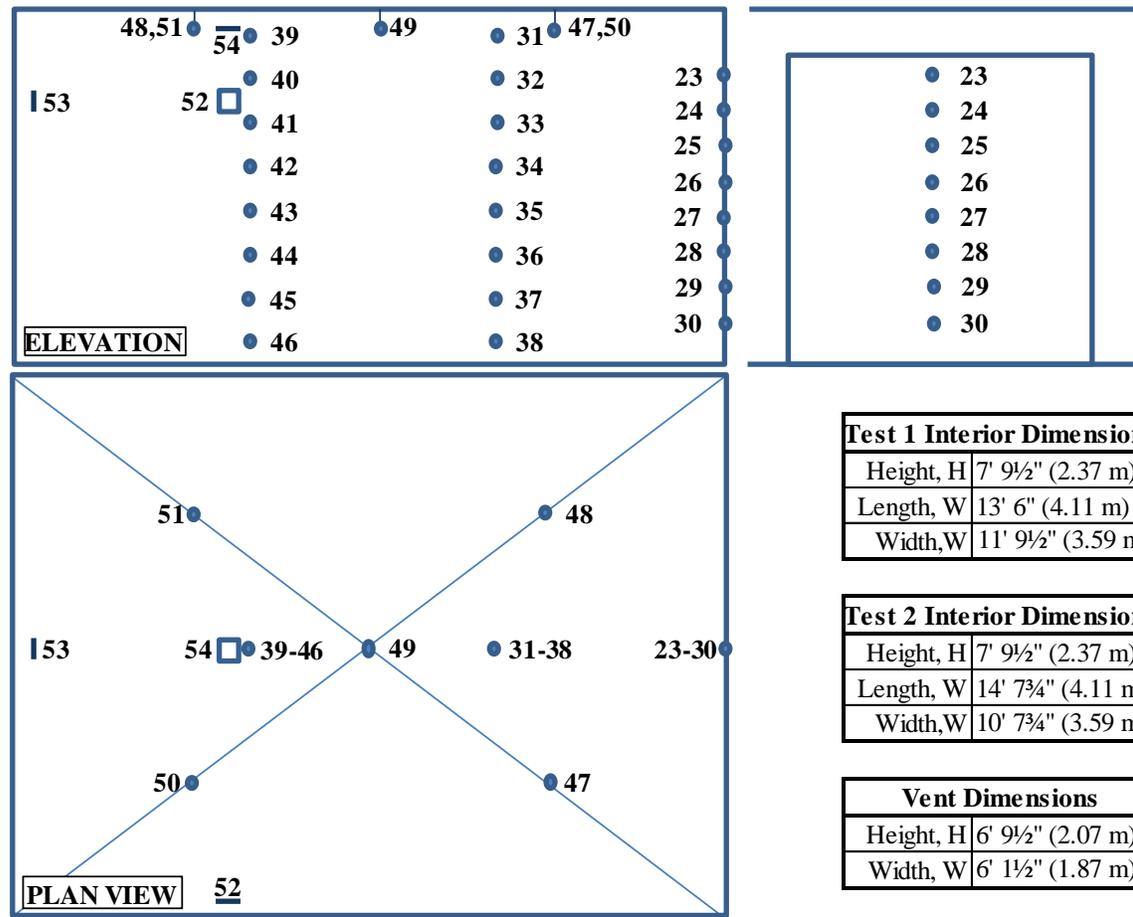
Figure 5. Room Interior Thermocouple Layout.
