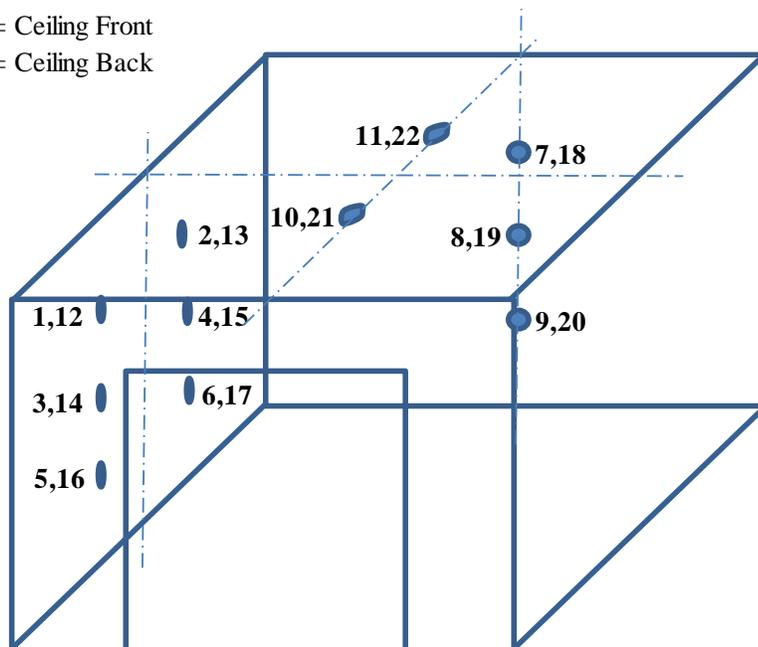
Figure 4. Wall and Ceiling Thermocouple Layout.
