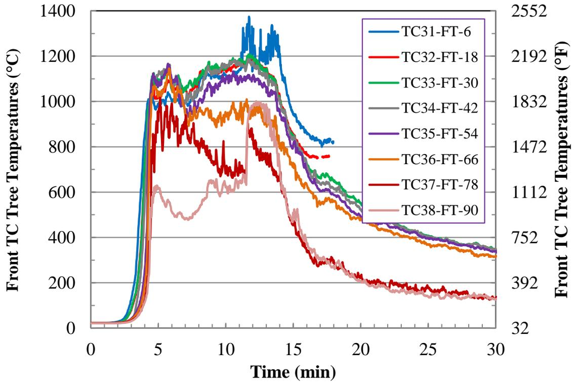
Figure E-13. Test 2 Front Interior TC Tree Temperatures (First 30 min).
