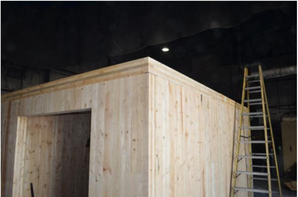
**Figure D-4. Assembled CLT Compartment for Test 2.**
