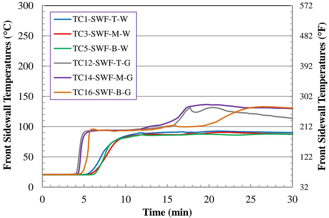
Figure E-3. Test 2 Front Sidewall Temperatures (First 30 min).
