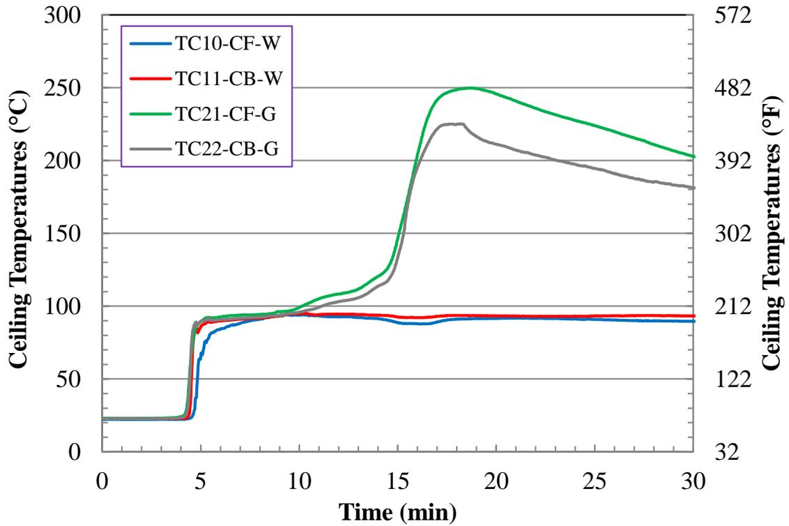
Figure C-9. Test 1 Ceiling Temperatures (First 30 min).
