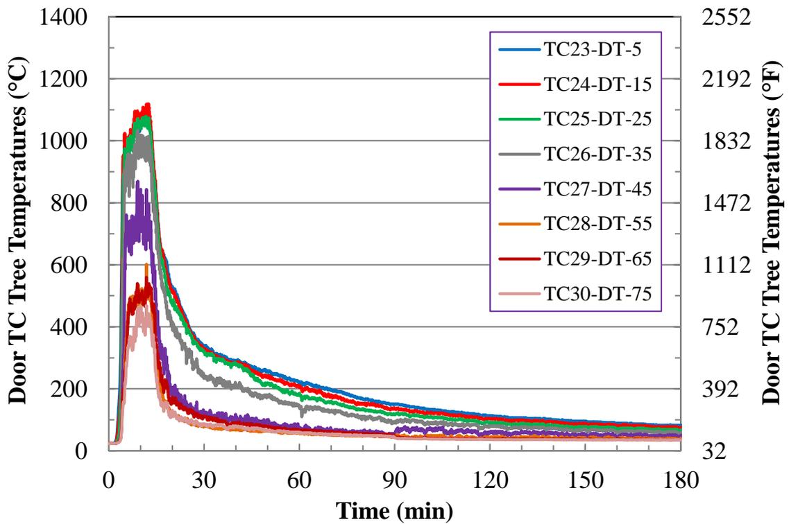
Figure C-12. Test 1 Door TC Tree Temperatures.
