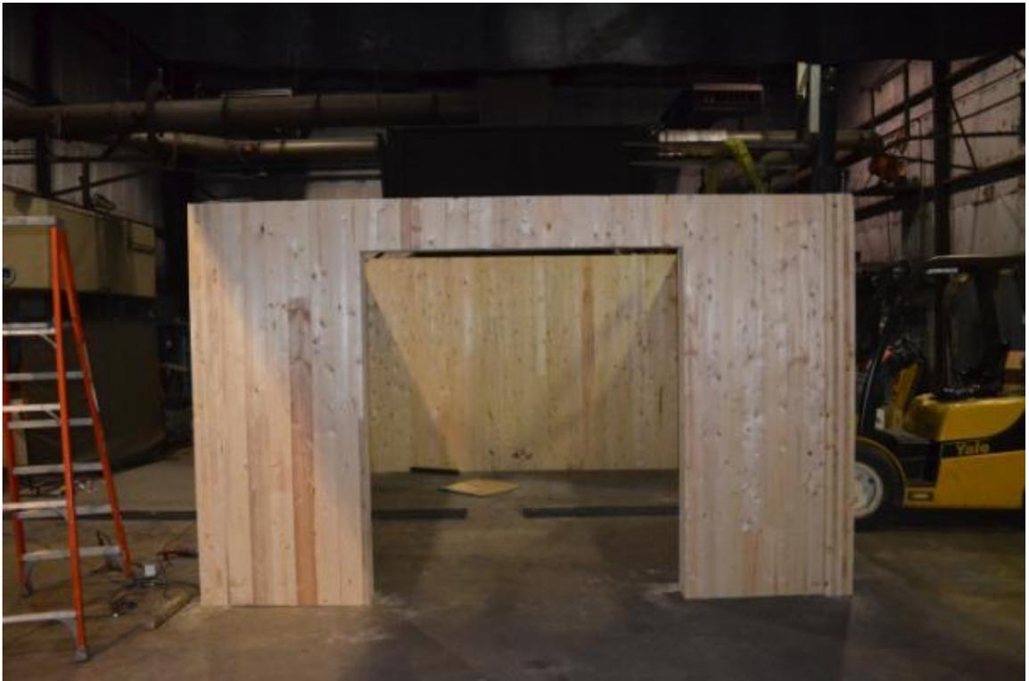
**Figure B-2. Assembled CLT Walls.**
