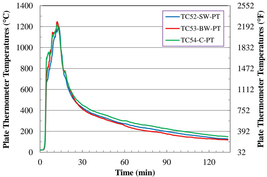
Figure E-20. Test 1 Plate Thermometer Temperatures.
