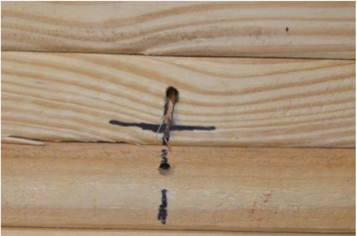
**Figure B-12. Thermocouple on Floor Joist.**
