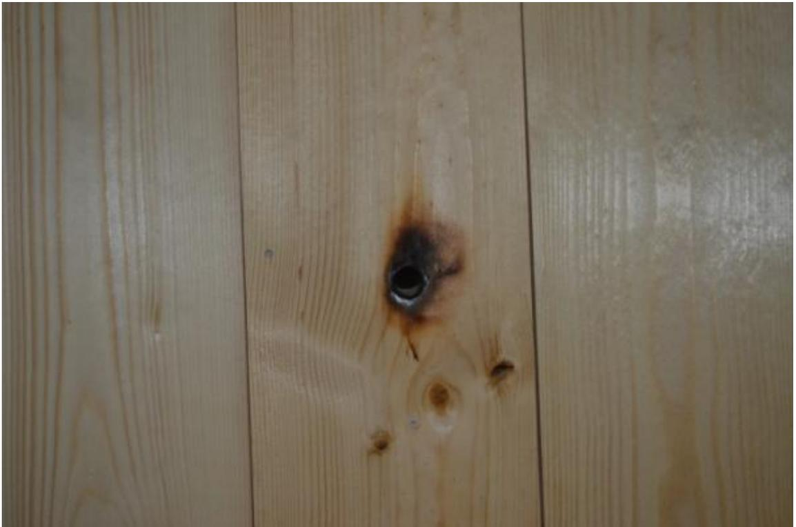
**Figure D-32. Charring around Plate Thermometer Conduit.**
