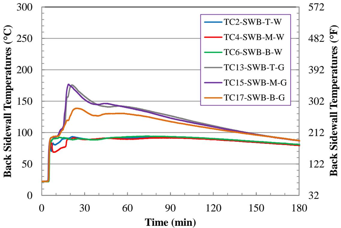
Figure C-6. Test 1 Back Sidewall Temperatures.
