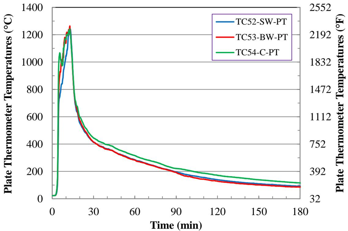
Figure C-20. Test 1 Plate Thermometer Temperatures.
