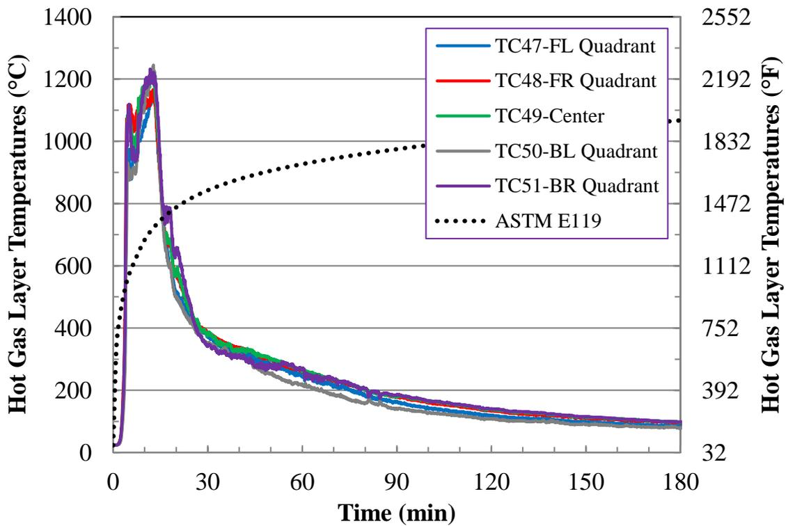
Figure C-18. Test 1 Hot Gas Layer Temperatures.
