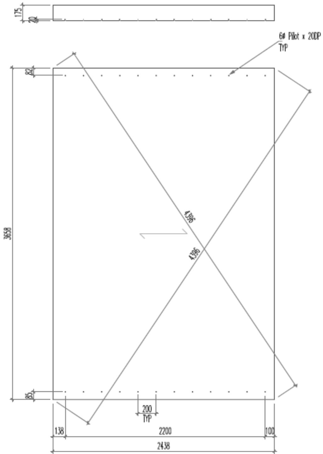
Figure A-2. Back Wall (Tests 1 and 2).
