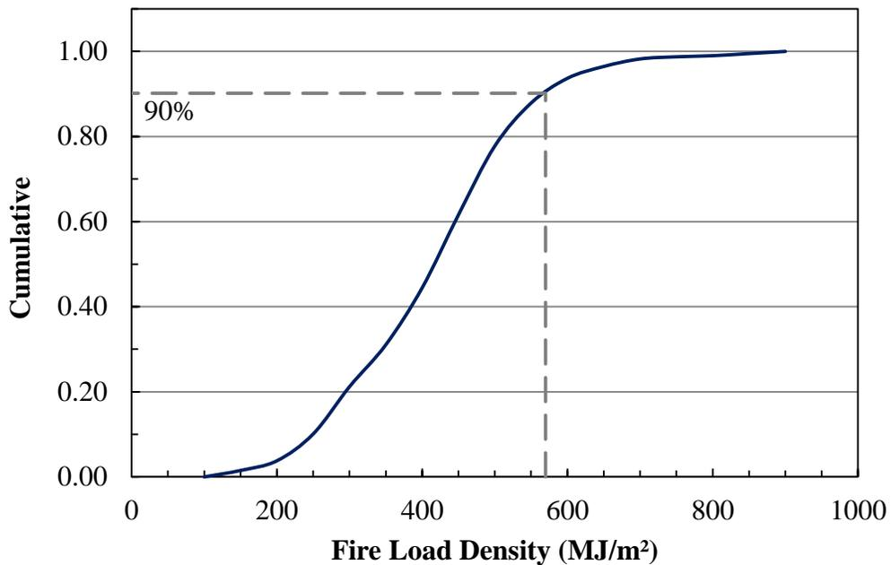
**Figure 7. Test 1 vs. Cumulative Fire Load Density Distribution from Canadian Survey.**
