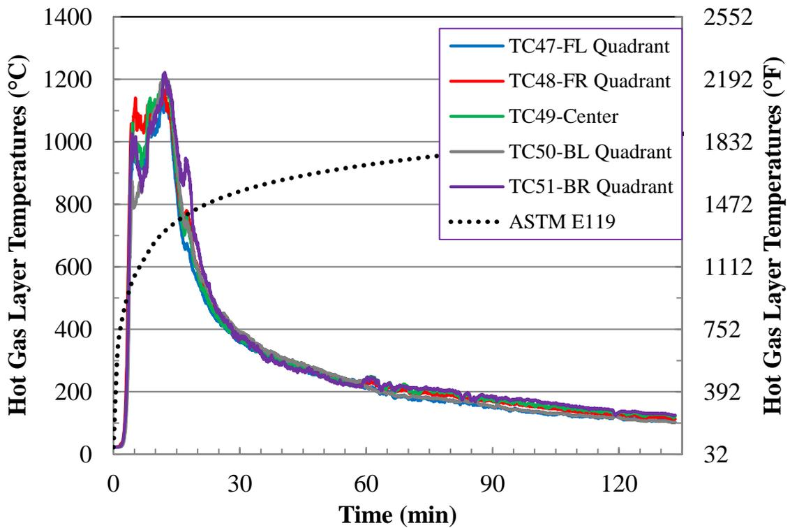
Figure E-18. Test 2 Hot Gas Layer Temperatures.
