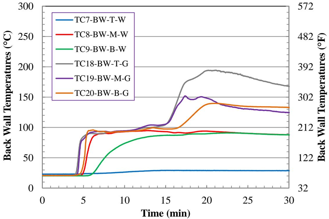
Figure E-7. Test 2 Back Wall Temperatures (First 30 min).
