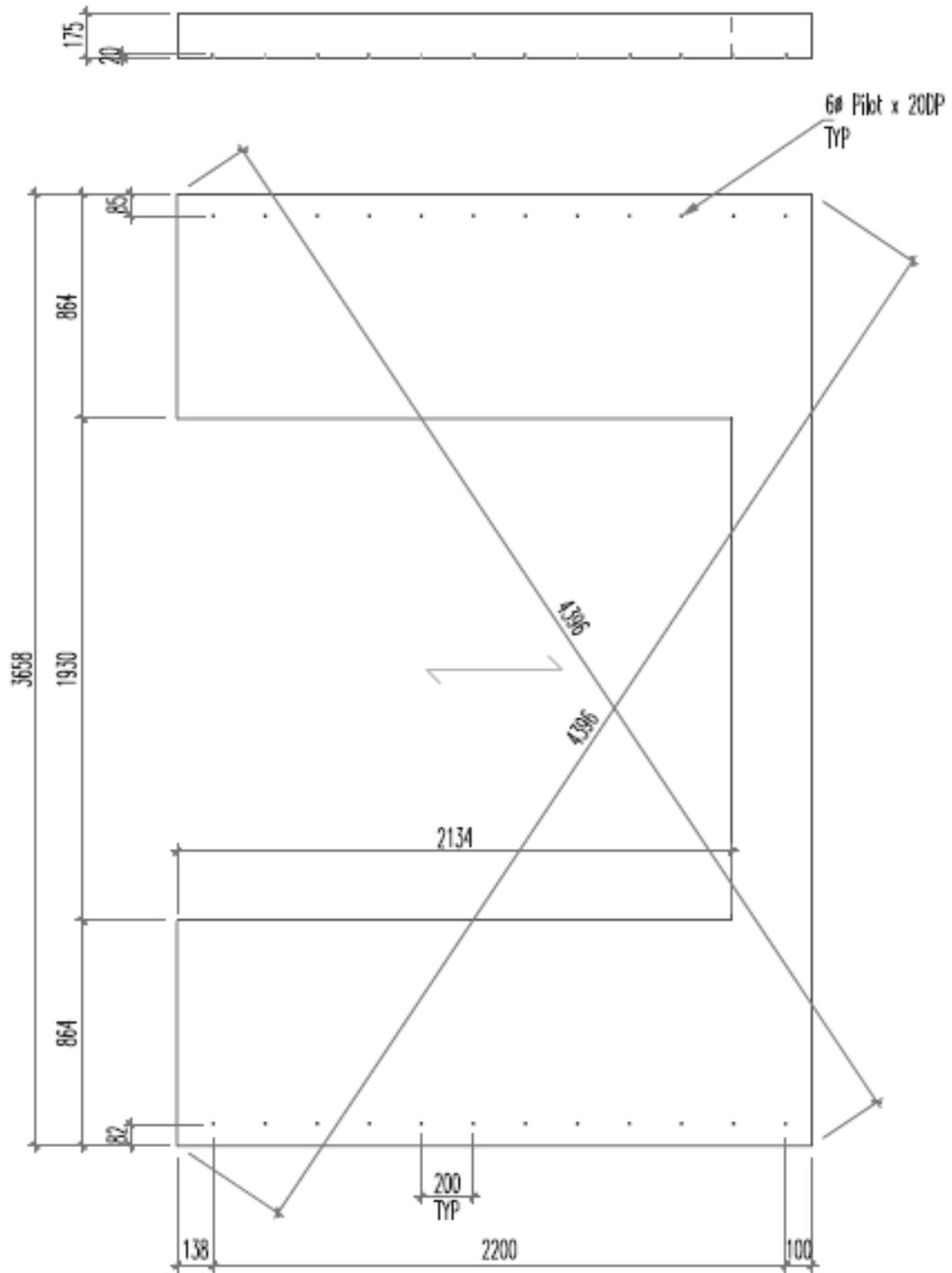
**Figure A-1. Front Wall (Tests 1 and 2).**
