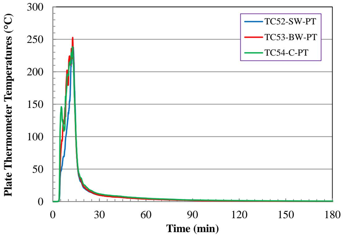
Figure C-22. Test 1 Plate Thermometer Heat Fluxes.
