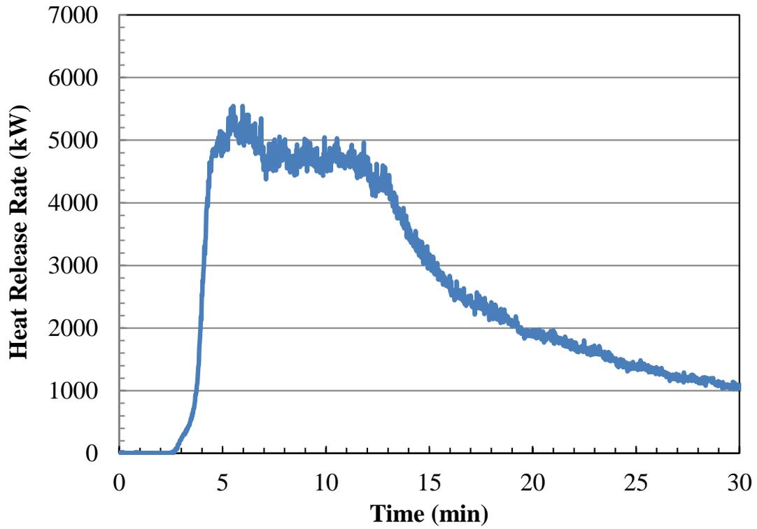
**Figure C-1. Test 1 Heat Release Rate (First 30 min).**
