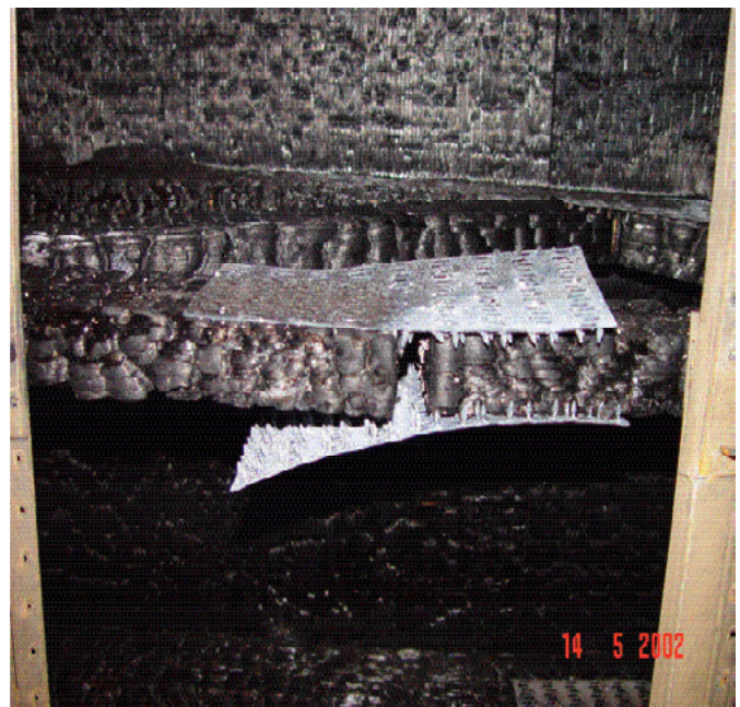
Figure 1: Metal Connector Plates After Fire Test
