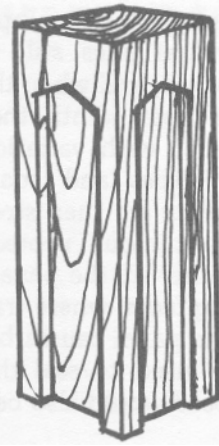
Figure 47.--Dado relief reduces visible checking.
