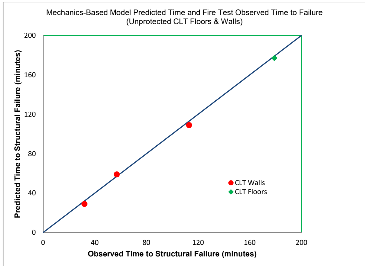
Figure 2-8 Comparison of Predicted to Observed Time to Failure (CLT tests)
