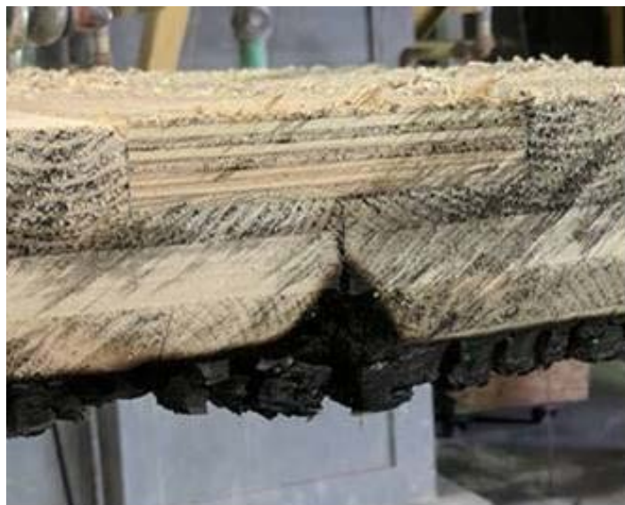
Figure C3-2. Example of char contraction at abutting edges of CLT floor panels (photo courtesy of Katerra)
