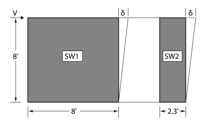
Figure 5. Distribution of shear to shear walls in a line to produce equal deflection in each shear wall is the underlying basis of the familiar 2b,/h factor.
