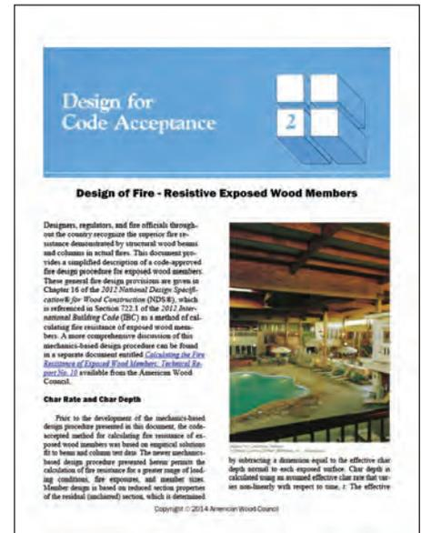
*Design of Fire-Resistive Exposed Wood Members* (DCA2) replaces the empirical design equations in the 2012 IBC with simplified design information developed in accordance with the NDS for exposed wood members, and is available for free download at [www.awc.org](http://www.awc.org).
