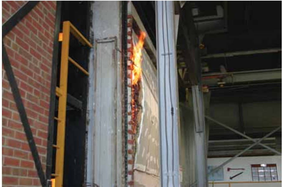
The American Wood Council (AWC) conducted a successful ASTM E119 fire resistance test on a CLT wall last year at NGC Testing Services in Buffalo, NY.
