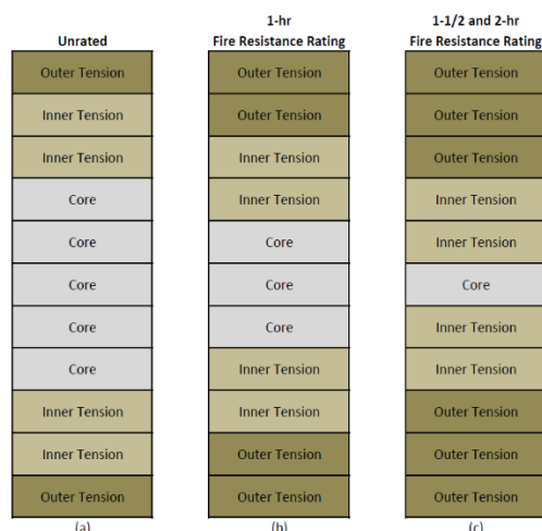
Figure 4-2 Typical Balanced Beam Layout
