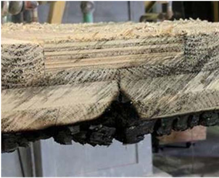
Figure 1-4. Example of char contraction at abutting edges of CLT floor panels (photo courtesy of Katerra).
