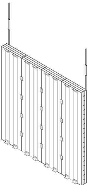
Figure 4. Cross-laminated timber shear wall, multi-panel configuration.
