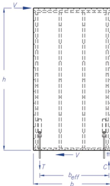
Figure 3. Wood-frame shear wall notations (hold-down on the inside face of post shown).
