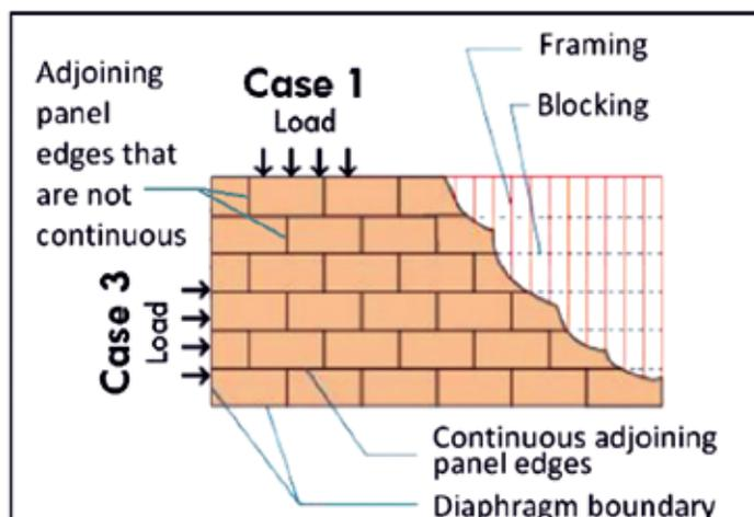
Figure 2. Adjoining panel edge locations, sheathed woodframe diaphragm (select cases).
