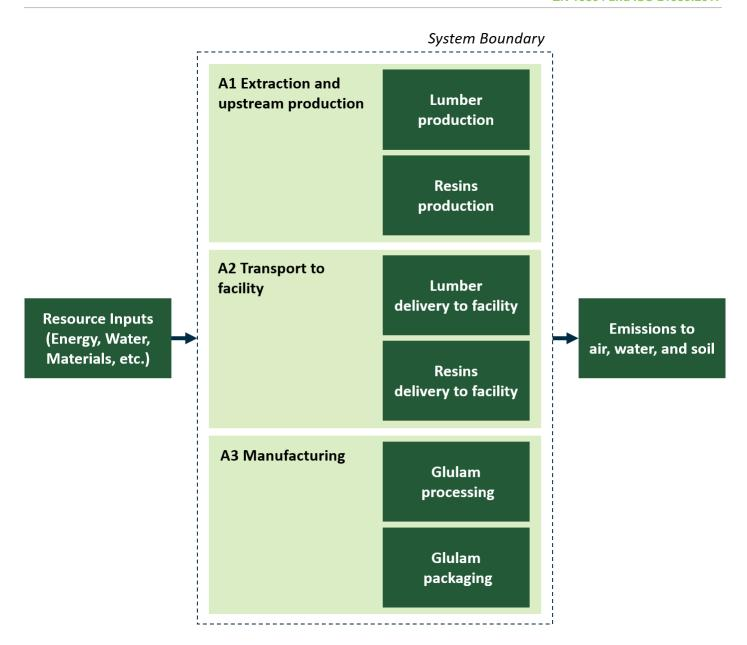
Figure 1. Cradle-to-gate glulam production flow diagram
