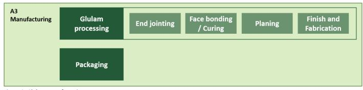
Figure 2. Glulam manufacturing process
