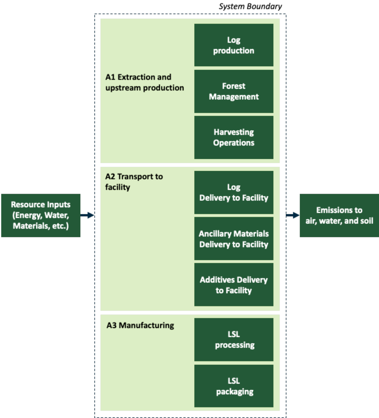
Figure 1. Cradle-to-Gate LSL production flow diagram
