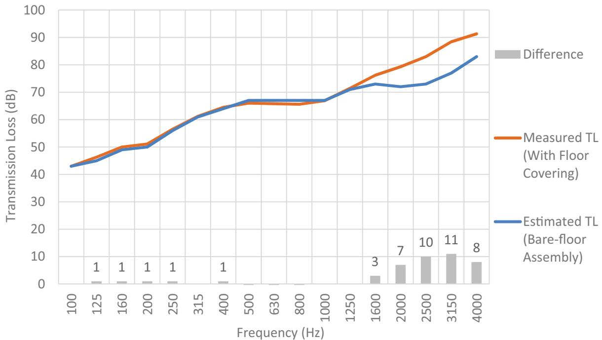
the difference between the actual measured TL contour of the tested floor-covered assembly (test TLF-17-060), versus the estimated  $TL_a(f)$ , which neglects the influence of the floating wood laminate floor covering. As illustrated
