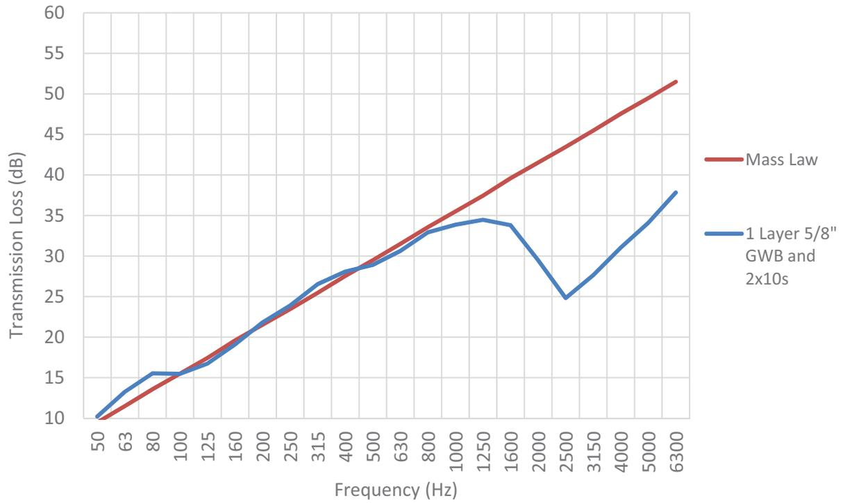
**Figure 1.2.3b Comparison of Measured TL and Mass Law Prediction for Typical Floor Layer**
