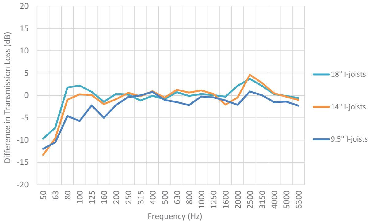
increase at the lower end affects frequencies (63 Hz to 125 Hz) that partially overlap the governing frequencies of the STC range (starting at 125 Hz), this translates into a positive correlation between joist depth and STC. However, the overall effect of joist depth typically only amounts to a 1 dB or 2 dB difference in STC.
