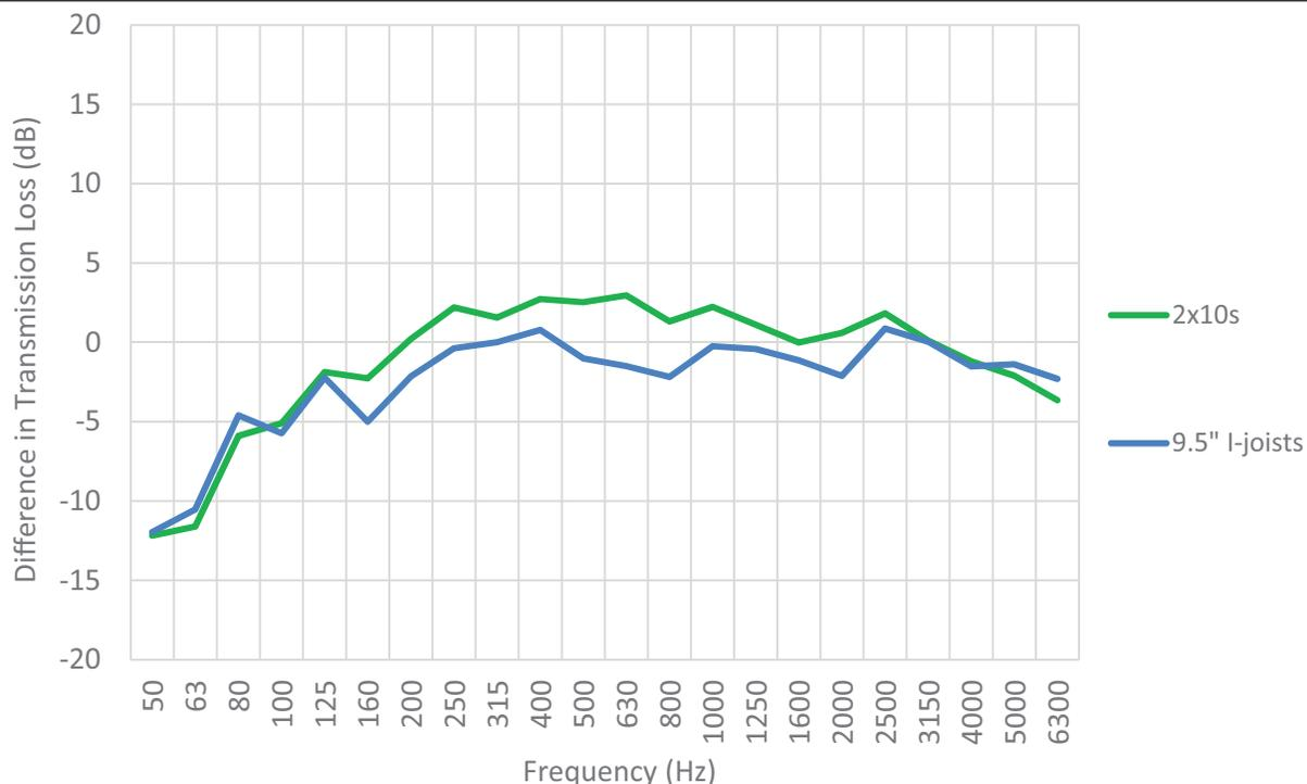
**Figure 1.2.5.4b System Effects Associated with Variations in Joist Depth**
