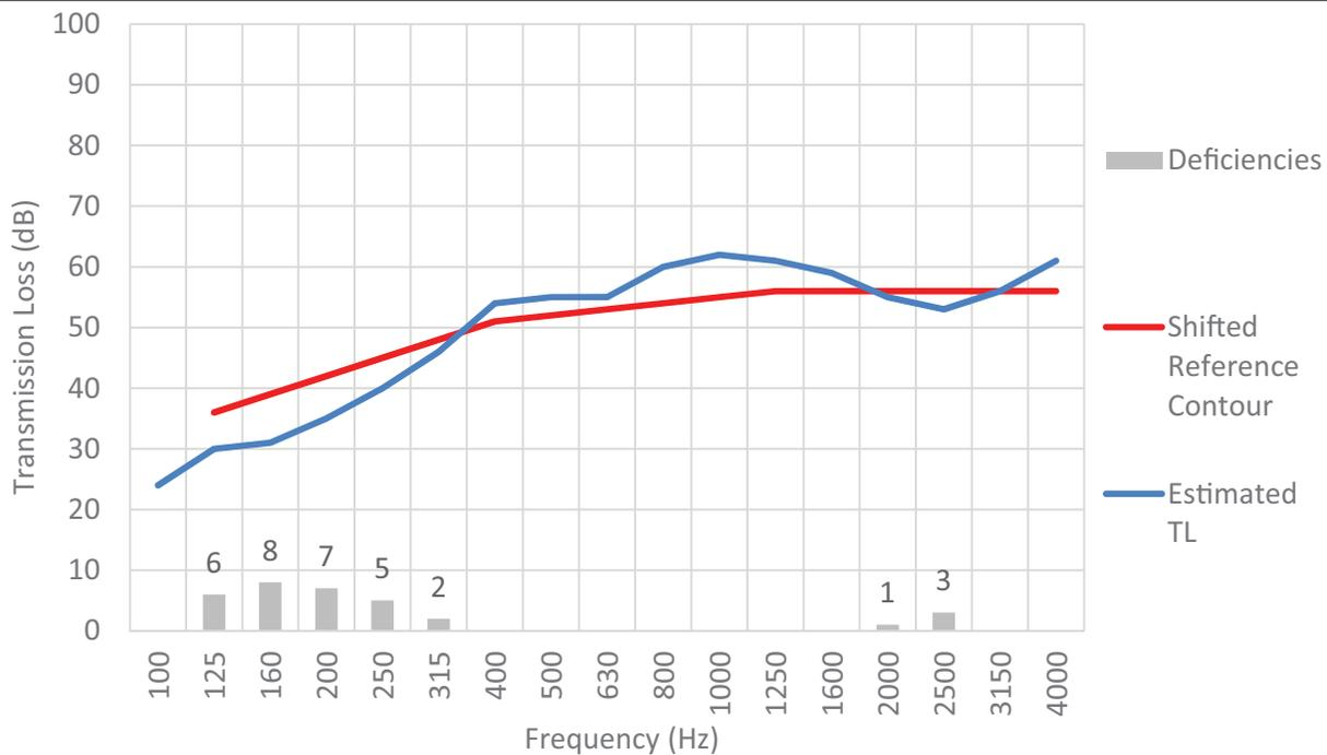
while still satisfying both of the conditions specified in Section 1.3.1.1 (i.e., sum of deficiencies  $\leq 32$ ; maximum deficiency  $\leq 8$  dB). In this example, the estimated STC is controlled both by the sum-of-deficiencies limit of 32, as well as the single-point-deficiency limit of 8 dB at 160 Hz.
