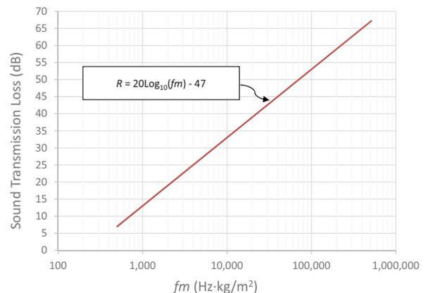
This idealized relationship between sound transmission loss and layer mass provides a useful tool in acoustical analysis of assemblies. As will be discussed in following sections, however, there are often significant differences between these idealized values and actual measured values.
