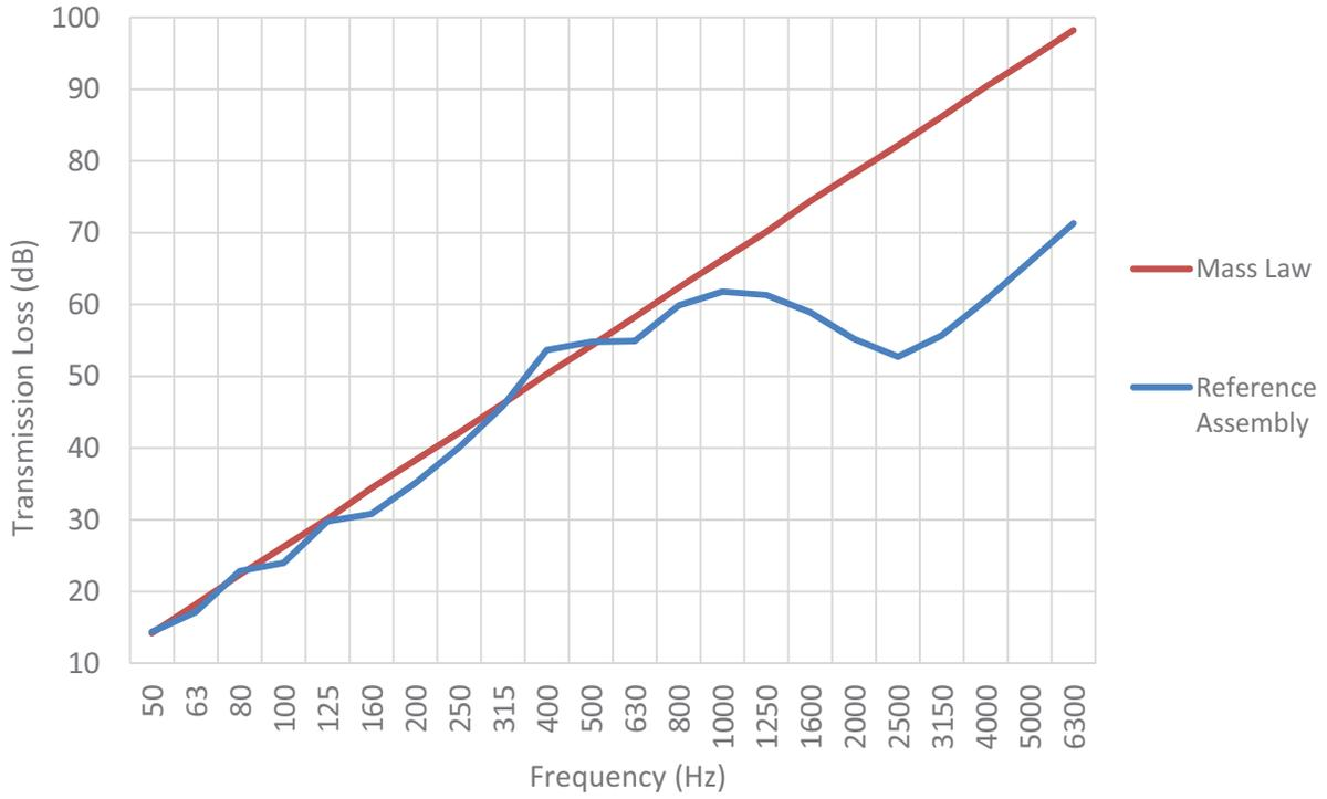
**Figure 1.2.4b Comparison of the Sum of Layer TLs to the Measured TL of the Reference Assembly**
