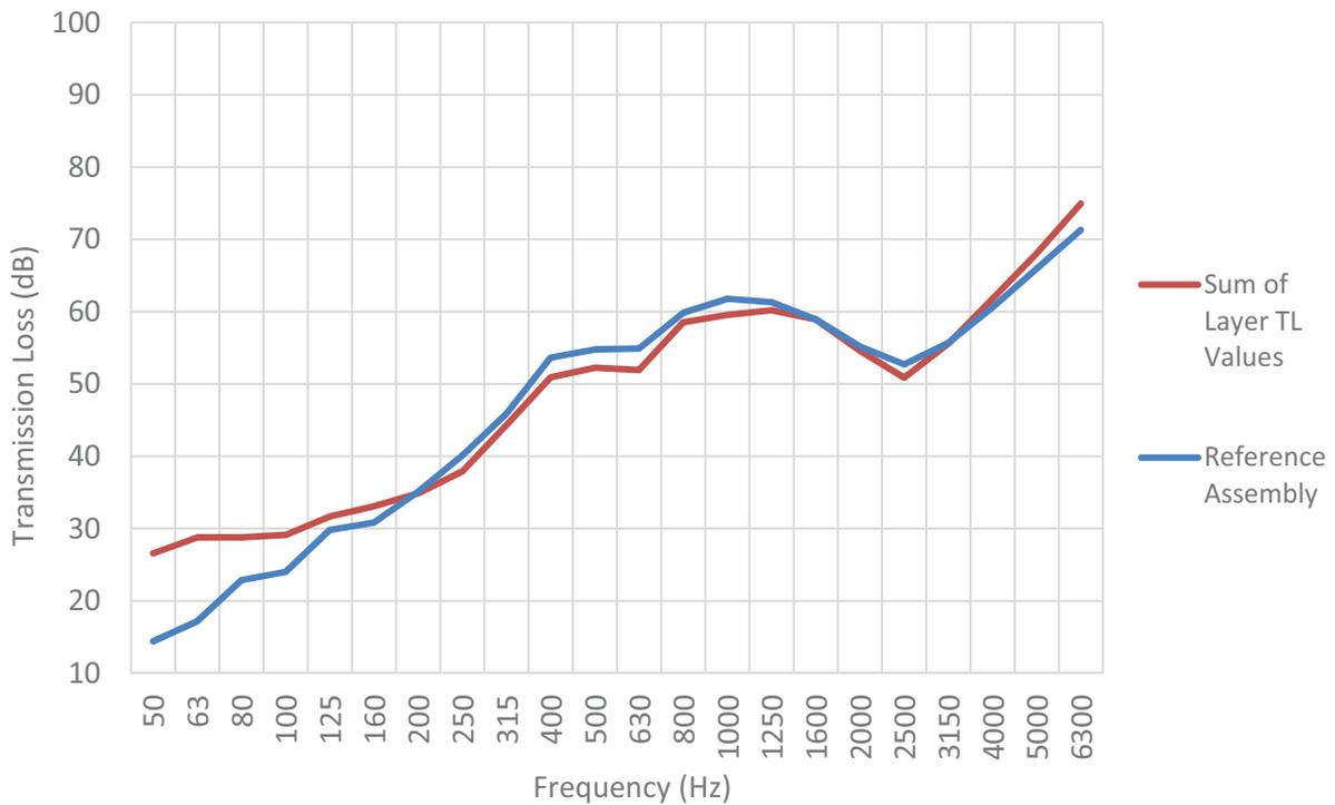
**Figure 1.2.4c System Effect of the Reference Assembly**
