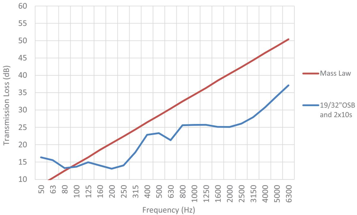
**Figure 1.2.4a Comparison of Measured TL and Mass law Prediction for the Reference Assembly**
