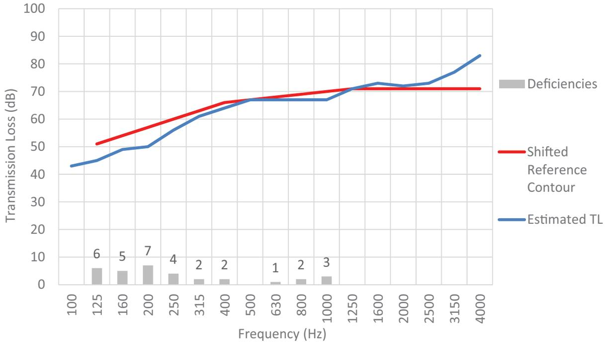
**Figure 3.3.1b** Example 2: Estimated TL of Bare-floor Assembly and Measured TL of Floor-Covered Assembly
