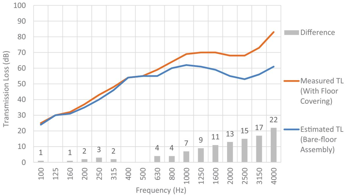
At the high end of the frequency spectrum (4000 Hz), the difference between the measured TL of the assembly having the floor covering versus the estimated TL of the bare-floor assembly was as great as 22 dB. This difference, shown in Figure 3.2.1b, is directly attributable to the influence of the thin carpet floor covering.
