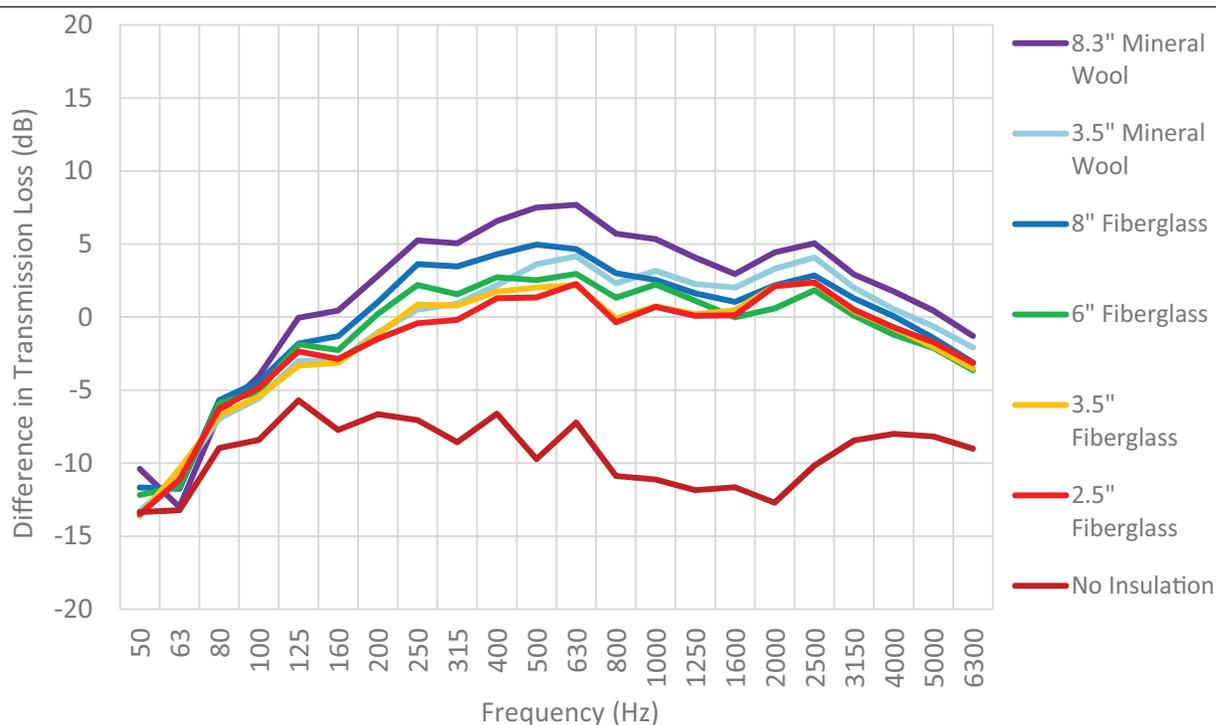
**Figure 1.2.5.2 System Effects Associated with Variations in the GWB Ceiling Layer**
