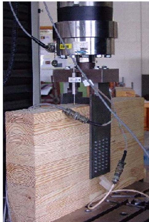
Figure 7—Test of rivets loaded perpendicular to grain.
