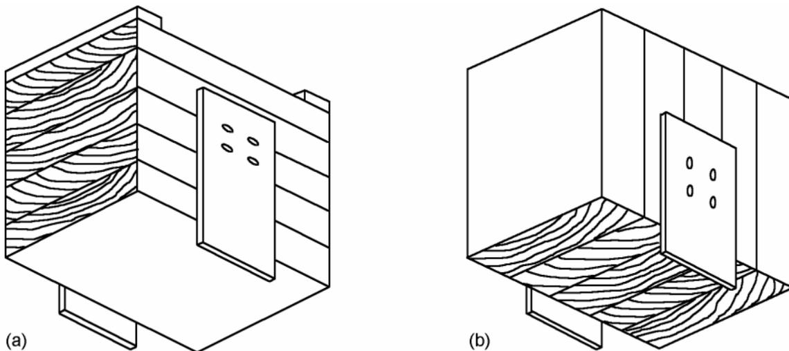
Figure 2—Small specimens for (a) perpendicular-to-grain and (b) parallel-to-grain loadings.
