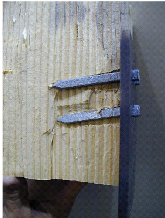
**Figure 11—Yield mode III<sub>m</sub> is characterized by single curvature of rivet below head (solid-sawn Southern Pine, 65-mm rivets).**
