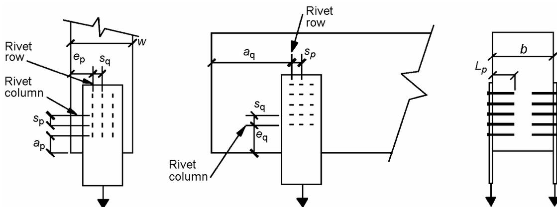
**Figure 1—Connection geometry variables: (from left) parallel-to-grain connection, perpendicular-to-grain connection, and view through thickness of connection.**
