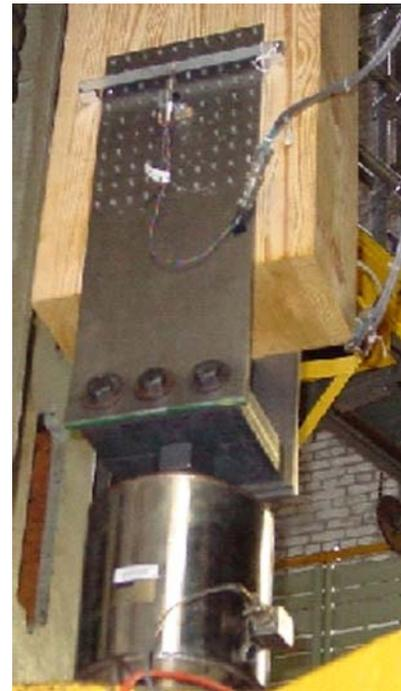
Figure 5—Measurement of displacement parallel to grain.
