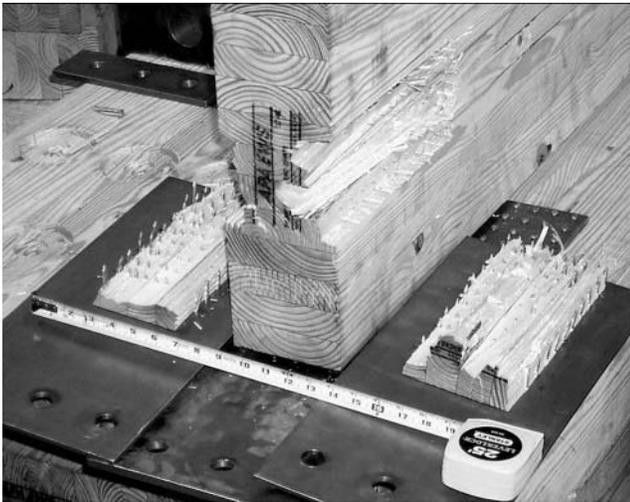
**Figure 13—Typical failure mode for large parallel-to-grain specimens.**
