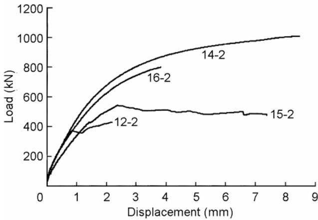
**Figure 12—Typical load–displacement plots for large parallel-to-grain specimens. See Appendix for description of test specimens.**
