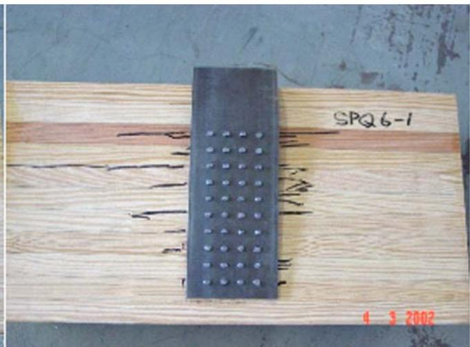
**Figure 14—Typical failure modes for large perpendicular-to-grain tests.**
