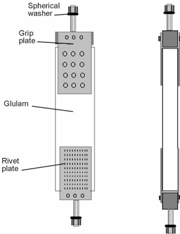
Figure 4—Setup for tension parallel-to-grain test.
