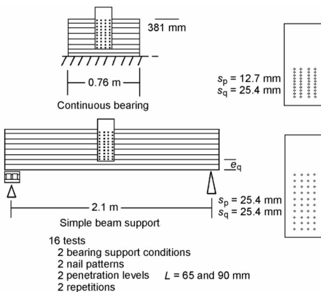
Figure 6—Specimens for perpendicular-to-grain tests.
