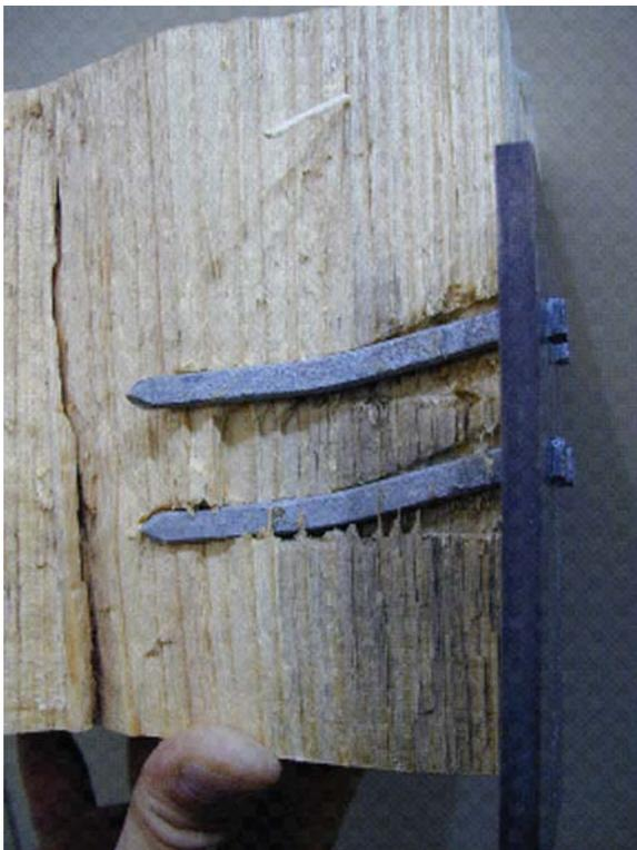
**Figure 10—Yield mode IV is characterized by reverse curvature of rivet between tip and head (solid-sawn Southern Pine, 90-mm rivets).**
