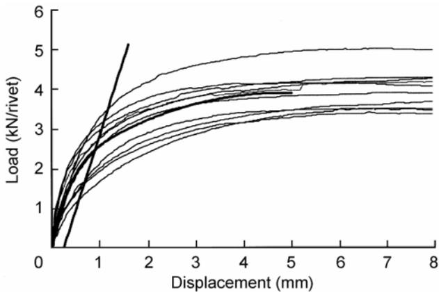
**Figure 8—Typical results for small specimens loaded parallel to grain. Ten replicates of solid-sawn Southern Pine, 65-mm rivets. Fitted curve and 5% offset line used for analysis.**
