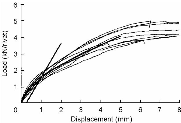
**Figure 9—Typical results for small specimens loaded perpendicular to grain. Ten replicates of solid-sawn Southern Pine, 65-mm rivets. Fitted curve and 5% offset line used for analysis.**
