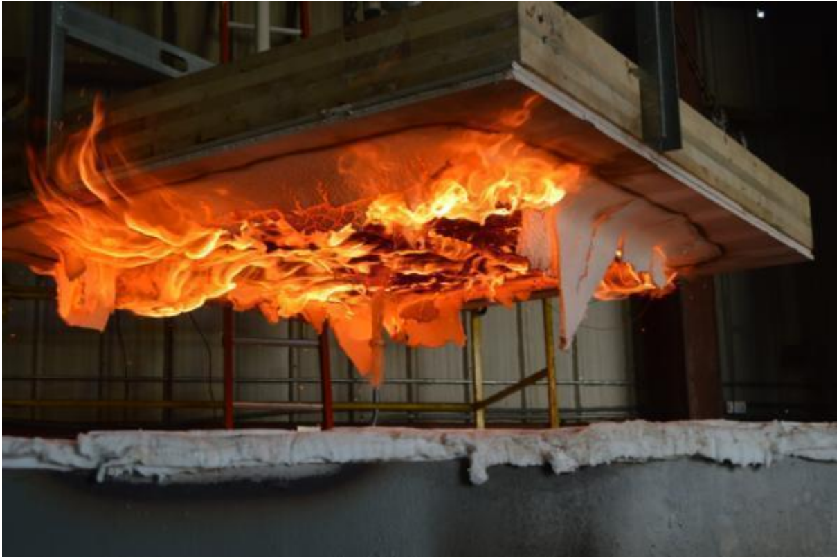
Figure B-3. Sample after 2-h Exposure.
