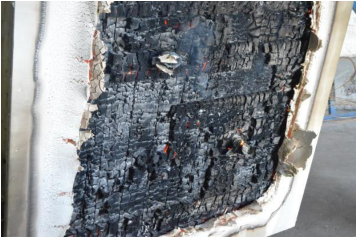
Figure B-4. Sample before the Hose Stream Test.
