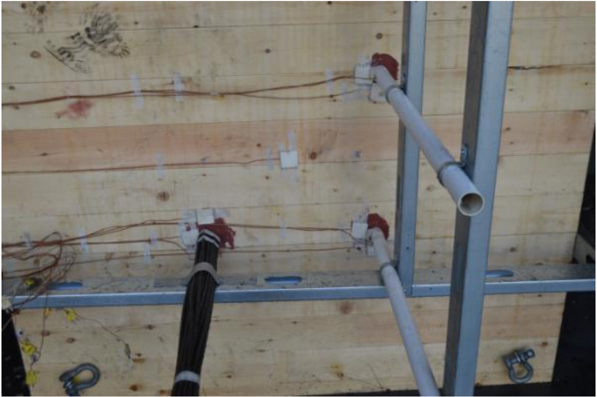
Figure B-5. Sample after Hose Stream Test.
