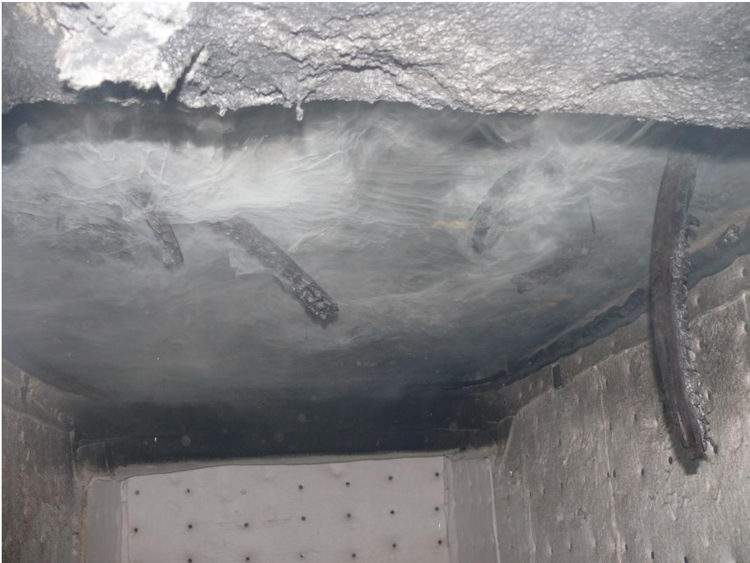
**Figure B-22. CLT #1 Test: Post-Test Picture of CLT Following Extinguishment.**
