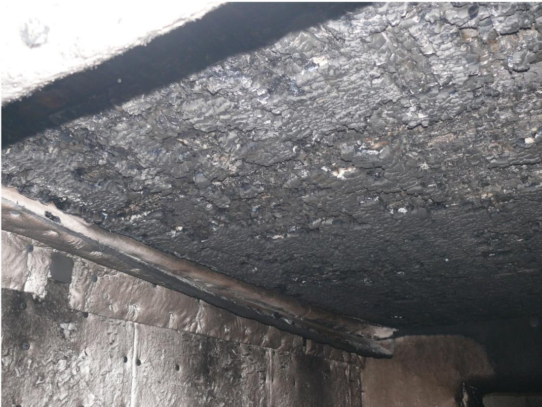
**Figure F-18. CLT #3 Test: Post-Test Picture of CLT Following Extinguishment.**
