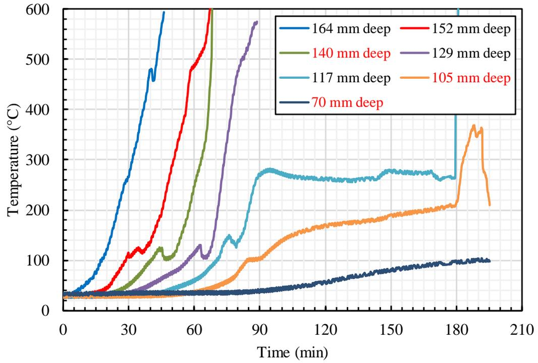
**Figure C-9. CLT #1 Test: Embedded TC Temperatures.**
