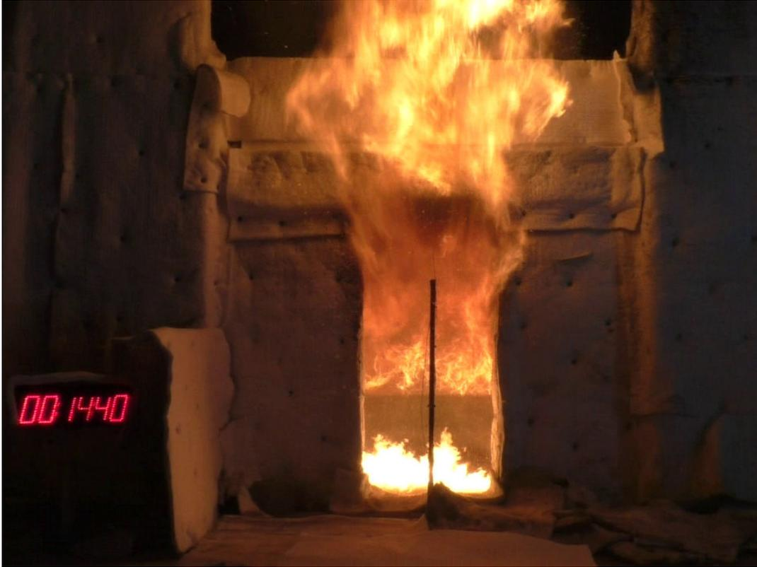
**Figure B-5. CLT #1 Test at 14 min 40 s: Flames on Floor Spread to Door.**
