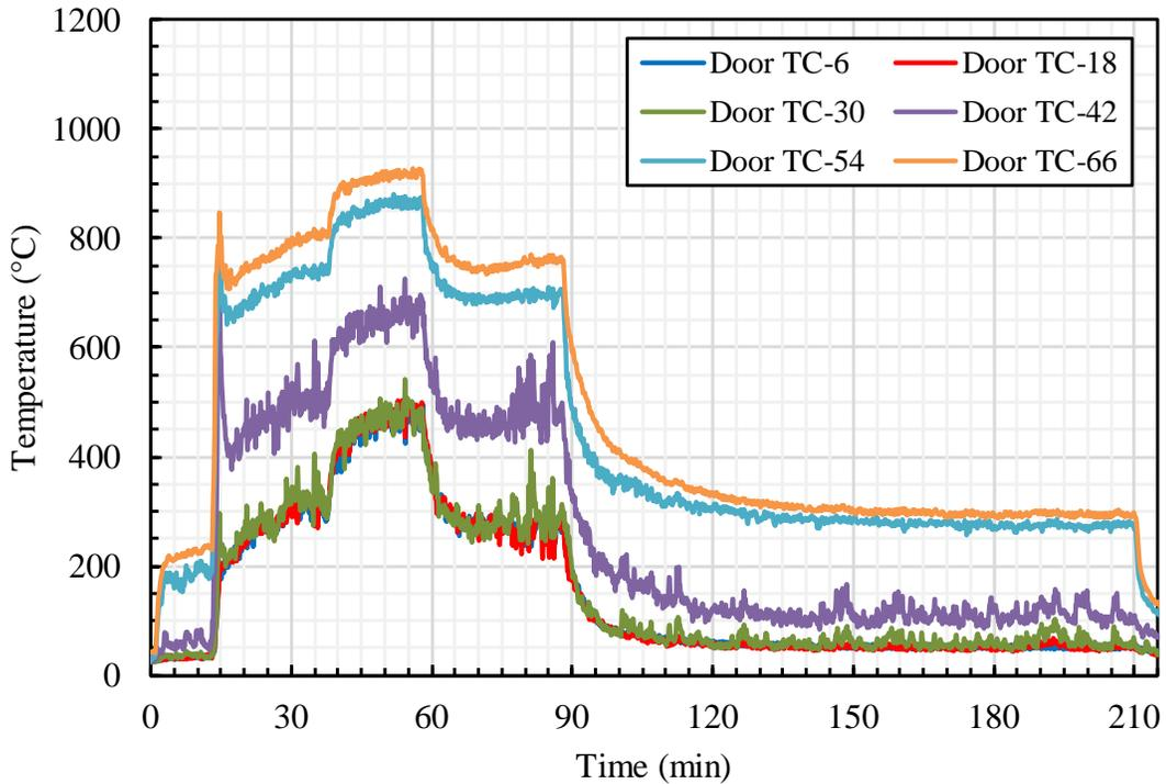
**Figure E-1. CLT #2 Test: Door TC Tree Temperatures.**
