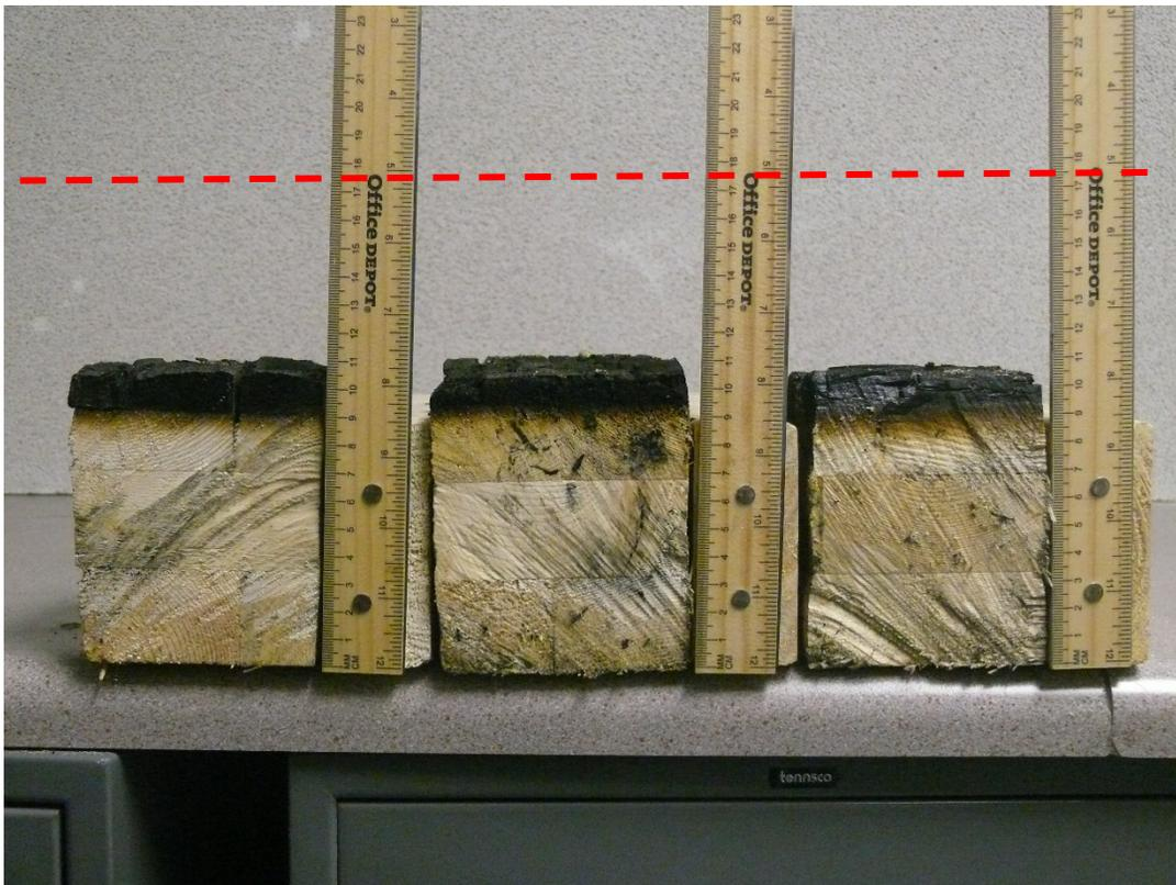
**Figure B- 26. CLT #1 Char Depth: Back Left – Ceiling Center – Back Right.**
