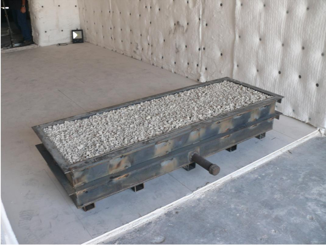
**Figure A-3. Gas Burner.**
