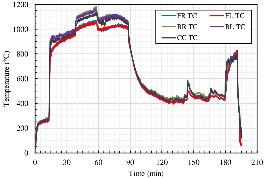
**Figure C-3. CLT #1 Test: Ceiling TC Temperatures.**
