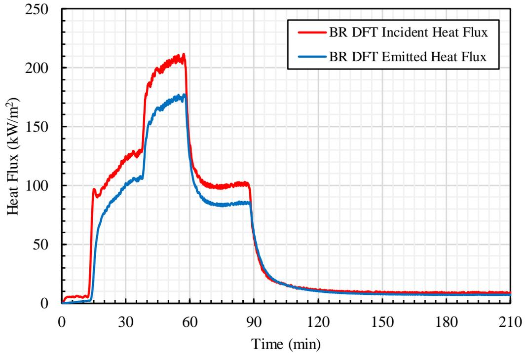
**Figure E-7. CLT #2 Test: Back Right DFT Heat Flux.**
