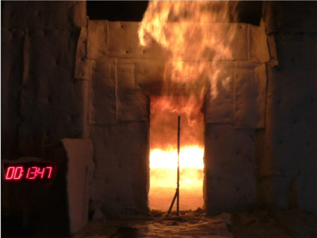
**Figure F-4. CLT #3 Test at 13 min 47 s: Ignition of Gypsum Board Paper at Burner.**
