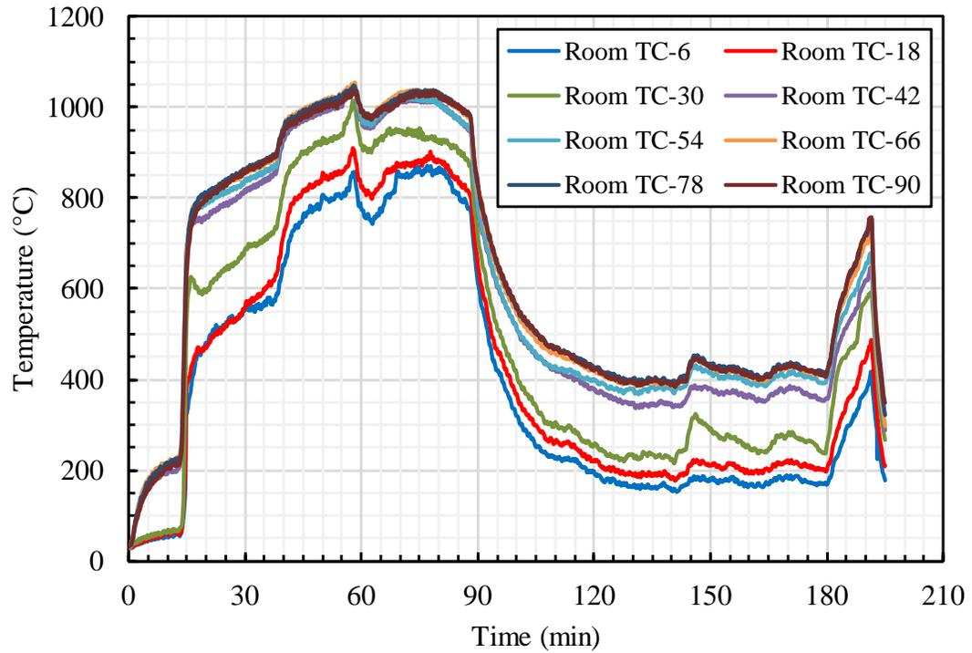
**Figure C-2. CLT #1 Test: Room TC Tree Temperatures.**
