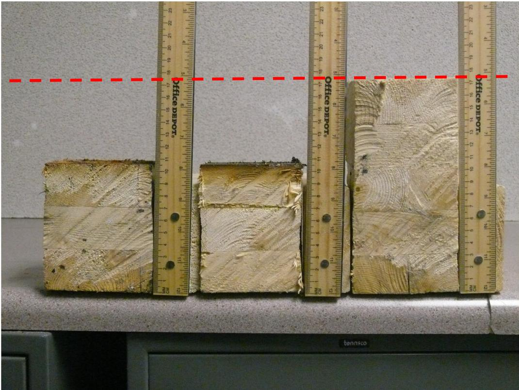
**Figure D-20. CLT #2 Char Depth: Front Left – Front Right - Original.**
