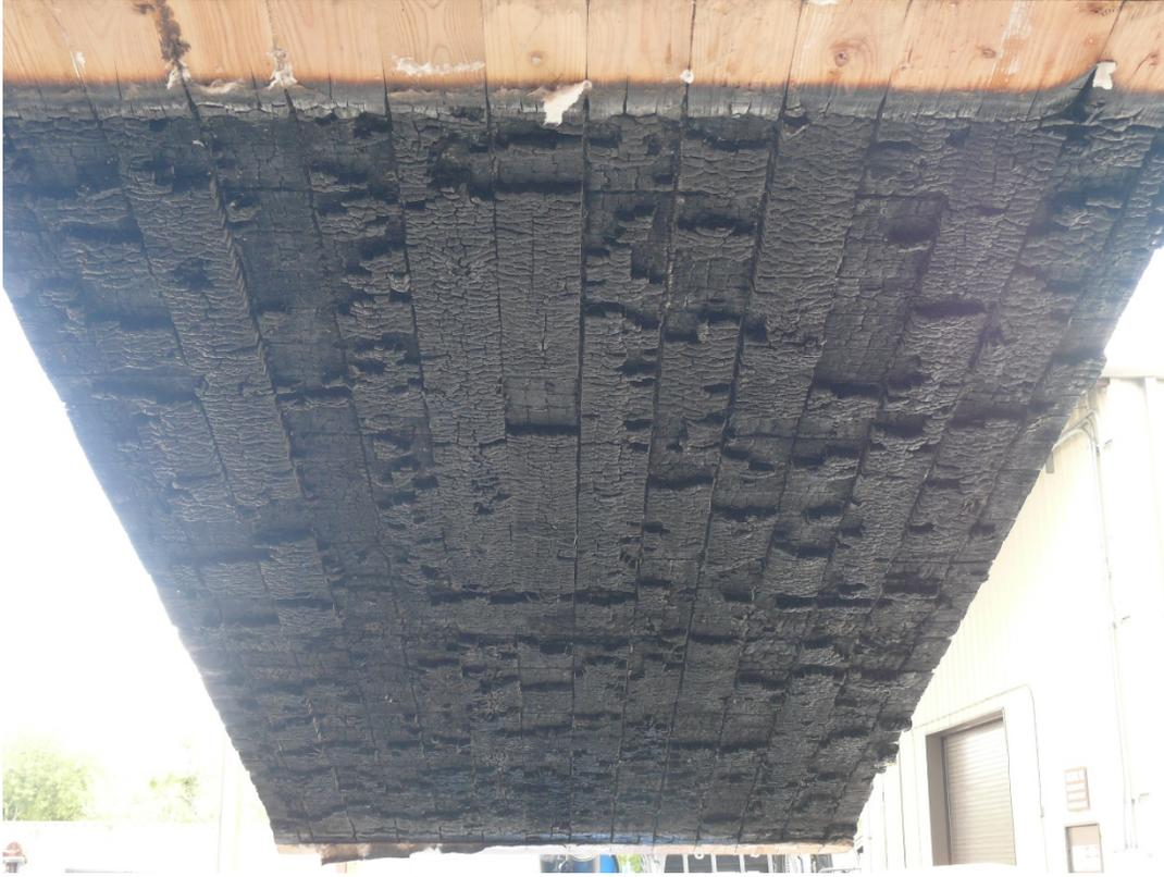
**Figure D-19. CLT #2 Test: Post-Test Picture of CLT Removed from Test Structure.**
