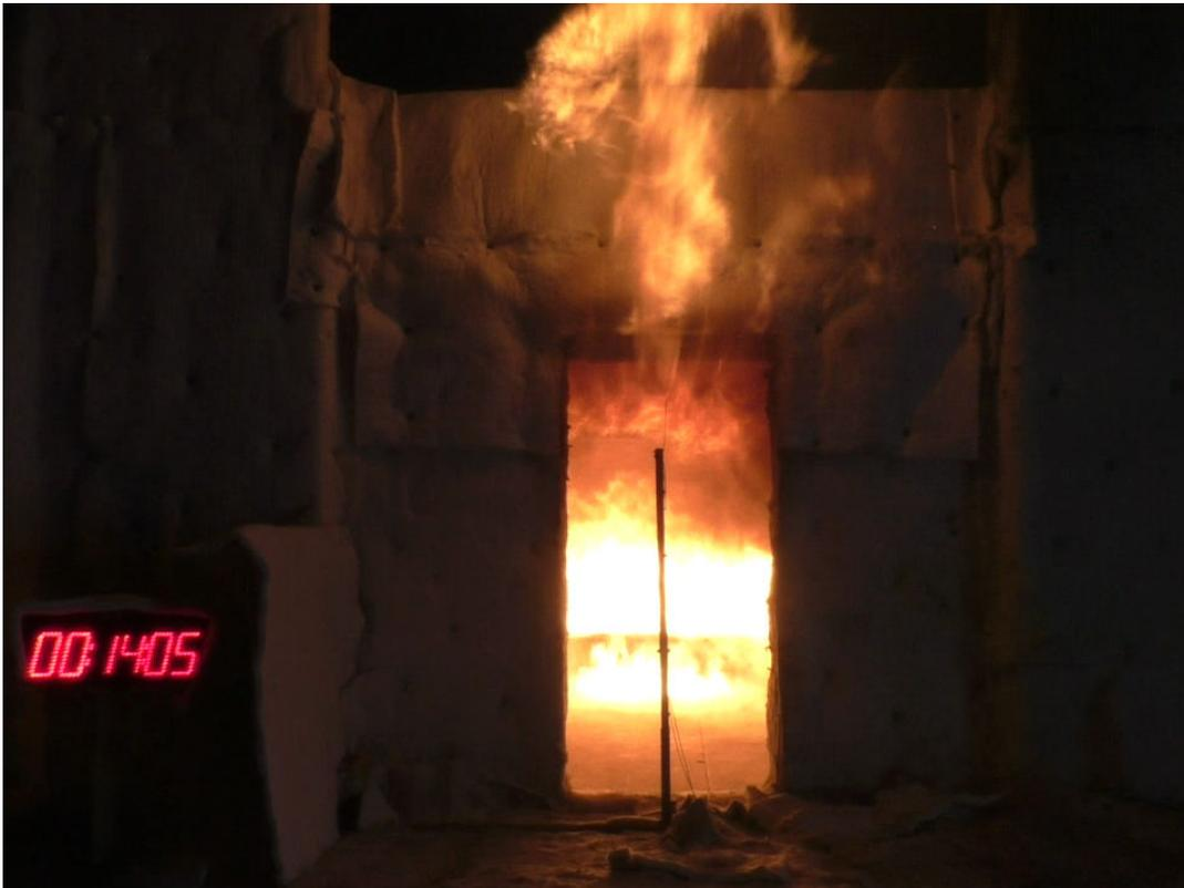
**Figure D-4. CLT #2 Test at 14 min 5 s: Ignition of Gypsum Board Paper at Burner.**
