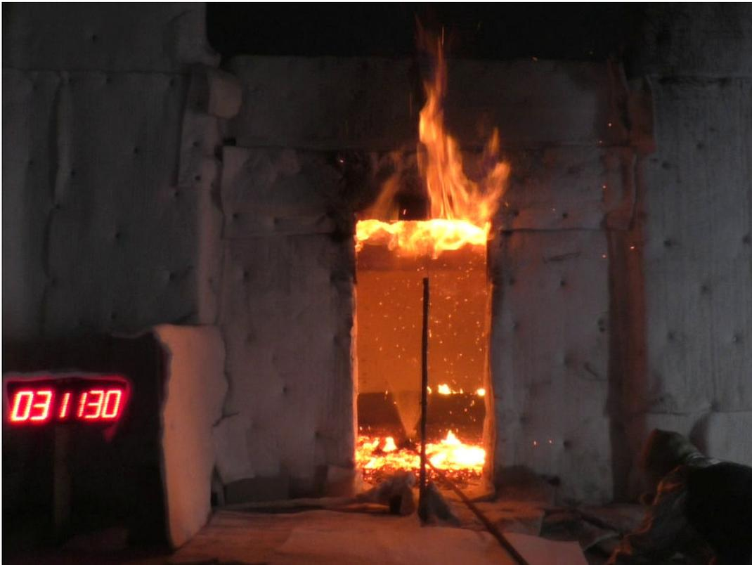
**Figure B-20. CLT #1 Test at 191 min 30 s: Start of Extinguishment.**
