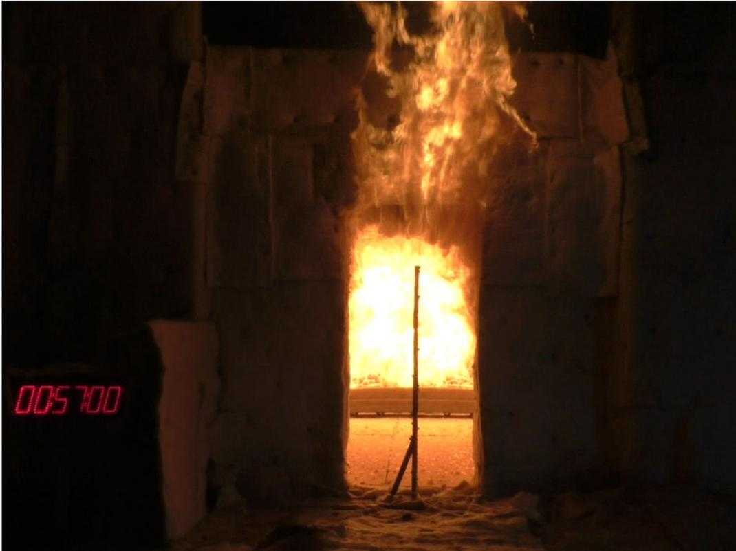
**Figure F-8. CLT #3 Test at 57 min.**
