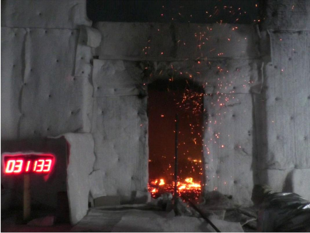
**Figure B-21. CLT #1 Test at 191 min 33 s: Ceiling Fire Extinguished.**
