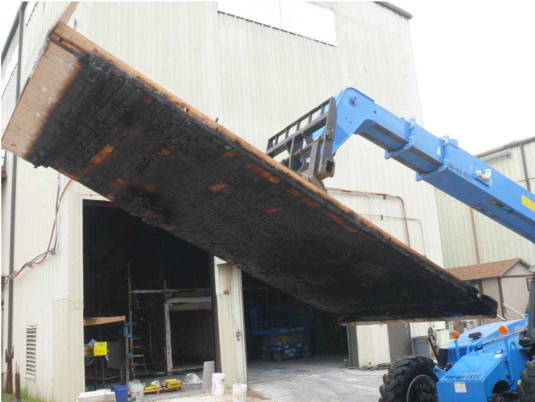
**Figure B- 24. CLT #1 Test: Post-Test Picture of CLT Removed from Test Structure.**
