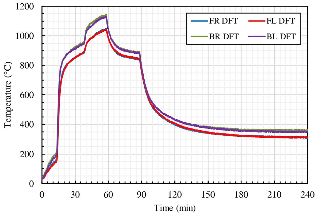
**Figure G-4. CLT #3 Test: DFT Exposed Plate Temperatures.**
