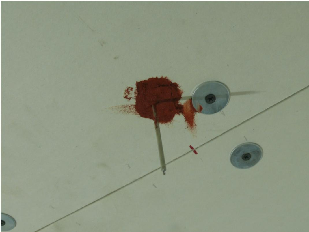
**Figure A-4. Hot Gas Layer Thermocouple.**
