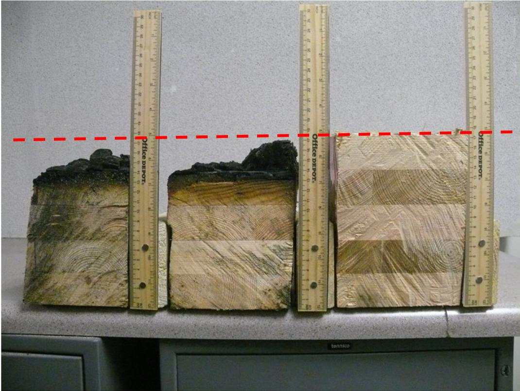
**Figure F-20. CLT #3 Char Depth: Front Left – Front Right - Original.**
