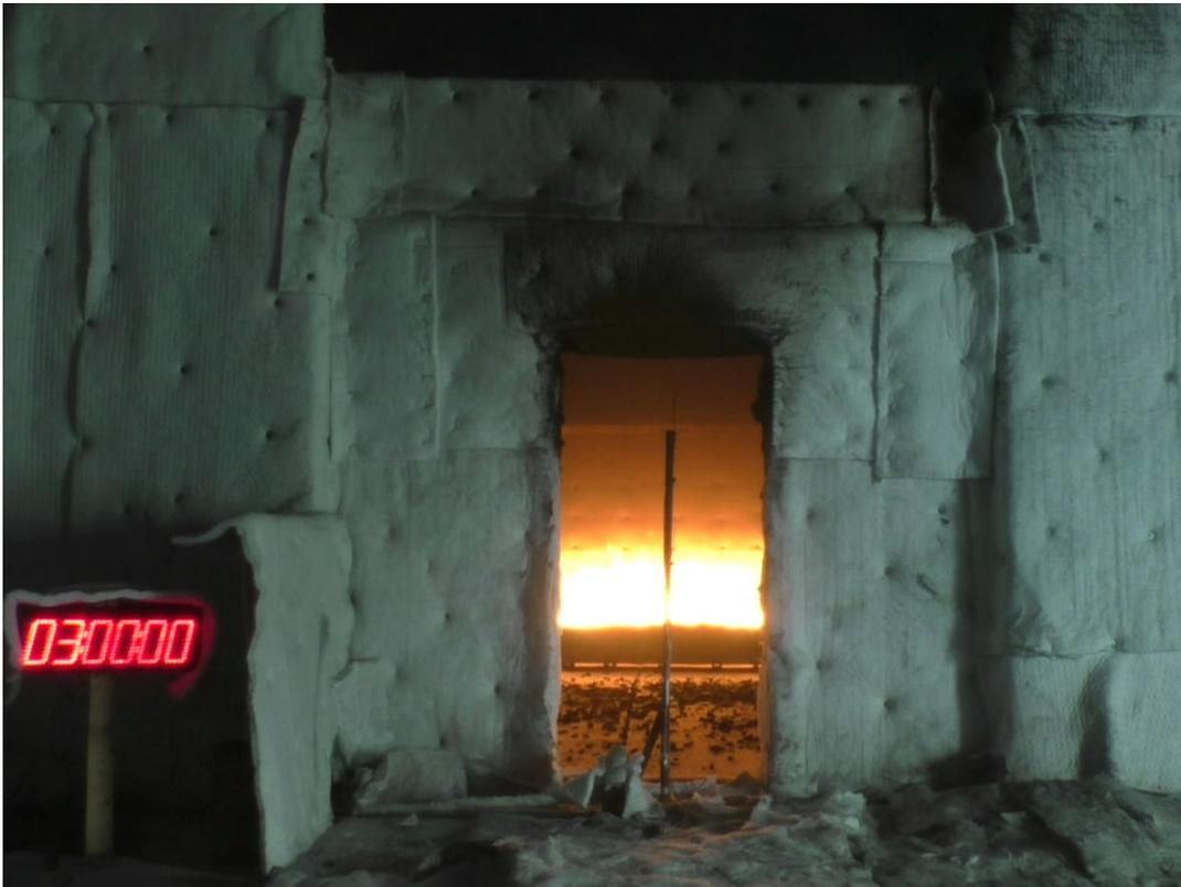
**Figure F-14. CLT #3 Test at 180 min.**
