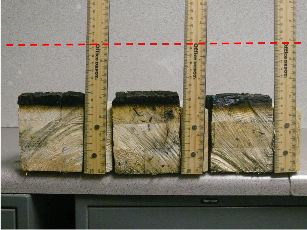
**Figure D-21. CLT #2 Char Depth: Back Left – Ceiling Center – Back Right.**
