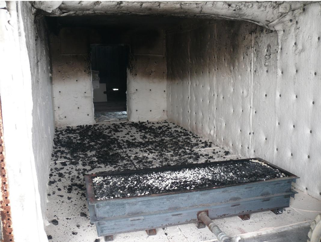
**Figure D-18. CLT #2 Test: Post-Test Picture of Charred Wood on Floor.**
