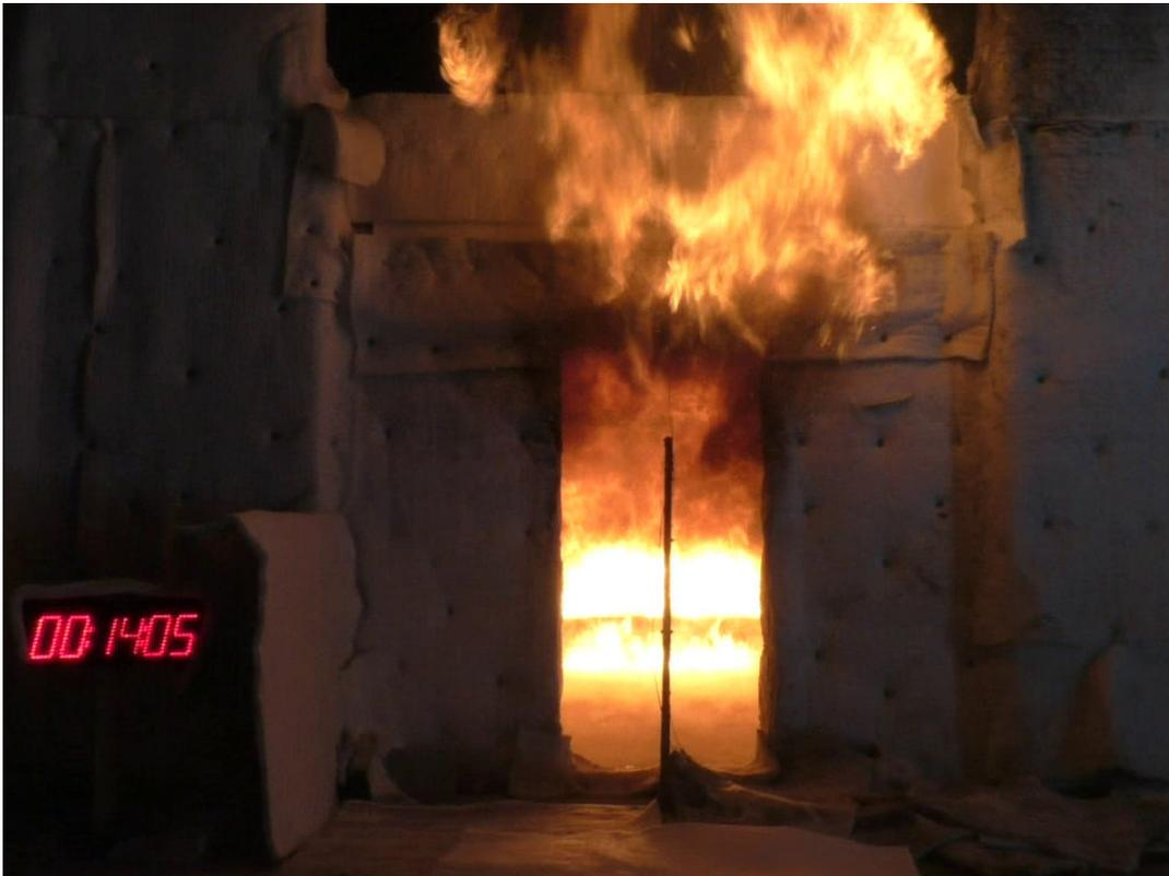
**Figure B-4. CLT #1 Test at 14 min 5 s: Ignition of Gypsum Board Paper at Burner.**
