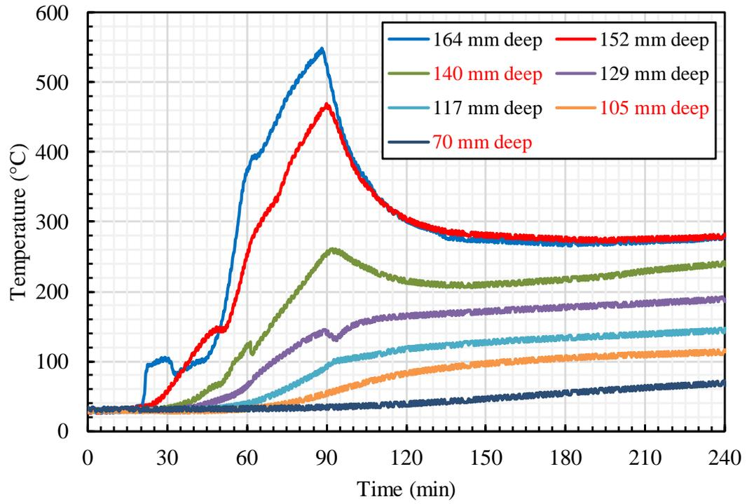
**Figure G-9. CLT #3 Test: Embedded TC Temperatures.**
