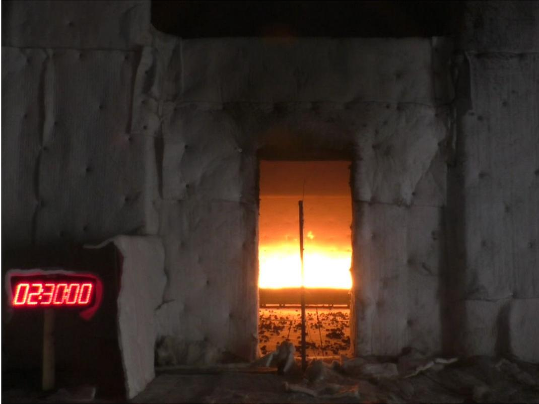
Figure D-13. CLT #2 Test at 150 min.
