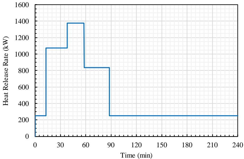
**Figure 2. Burner Heat Release Rate Profile.**
