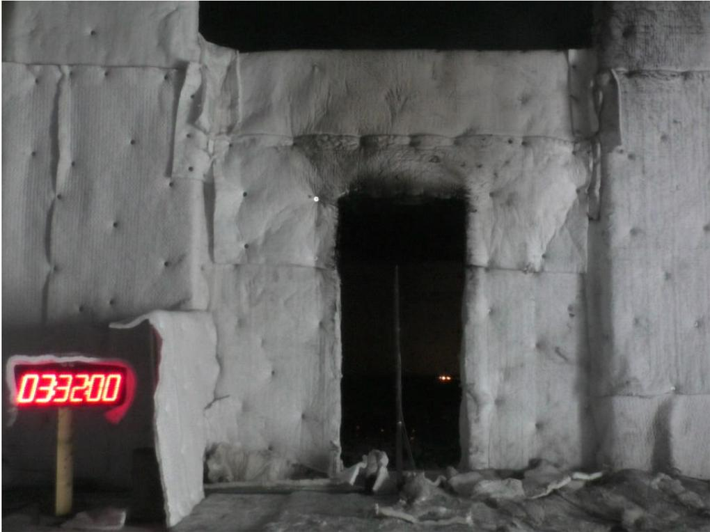
Figure D-16. End of CLT #2 Test at 212 min.
