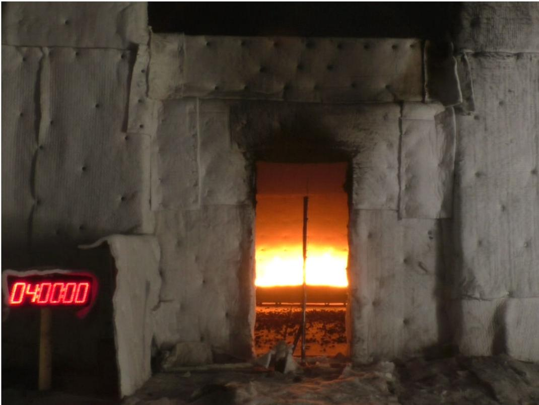
**Figure F-16. CLT #3 Test at 240 min**
