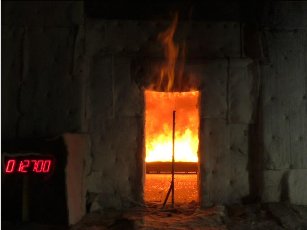
**Figure F-10. CLT #3 Test at 87 min.**
