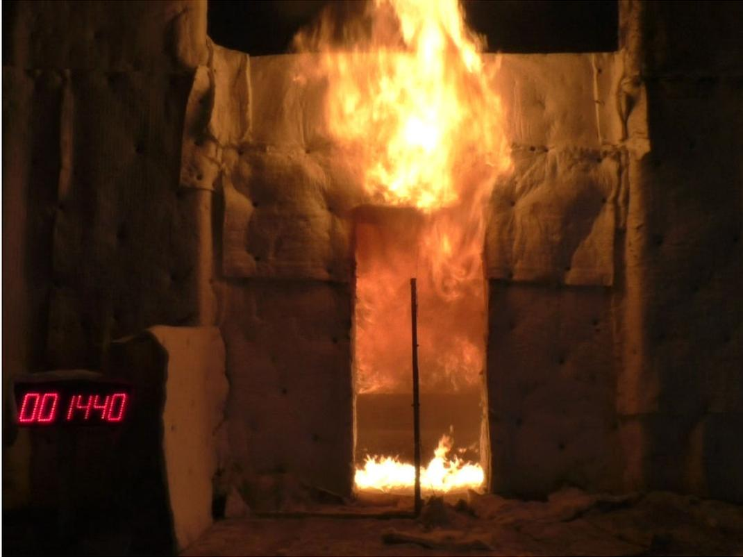
**Figure D-5. CLT #2 Test at 14 min 40 s: Flames on Floor Spread to Door.**
