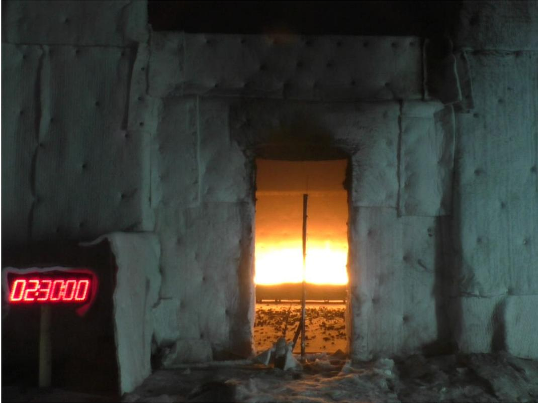
**Figure F-13. CLT #3 Test at 150 min.**
