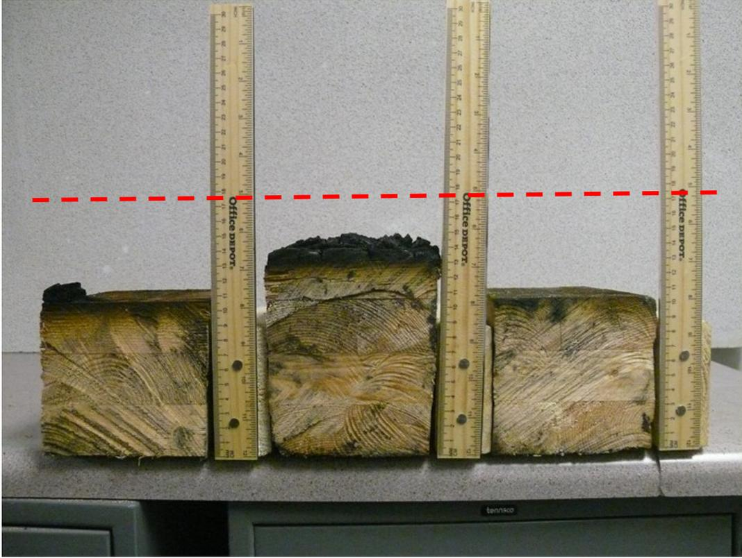
**Figure F-21. CLT #3 Char Depth: Back Left – Ceiling Center – Back Right.**
