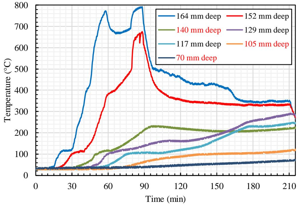
**Figure E-9. CLT #2 Test: Embedded TC Temperatures.**
