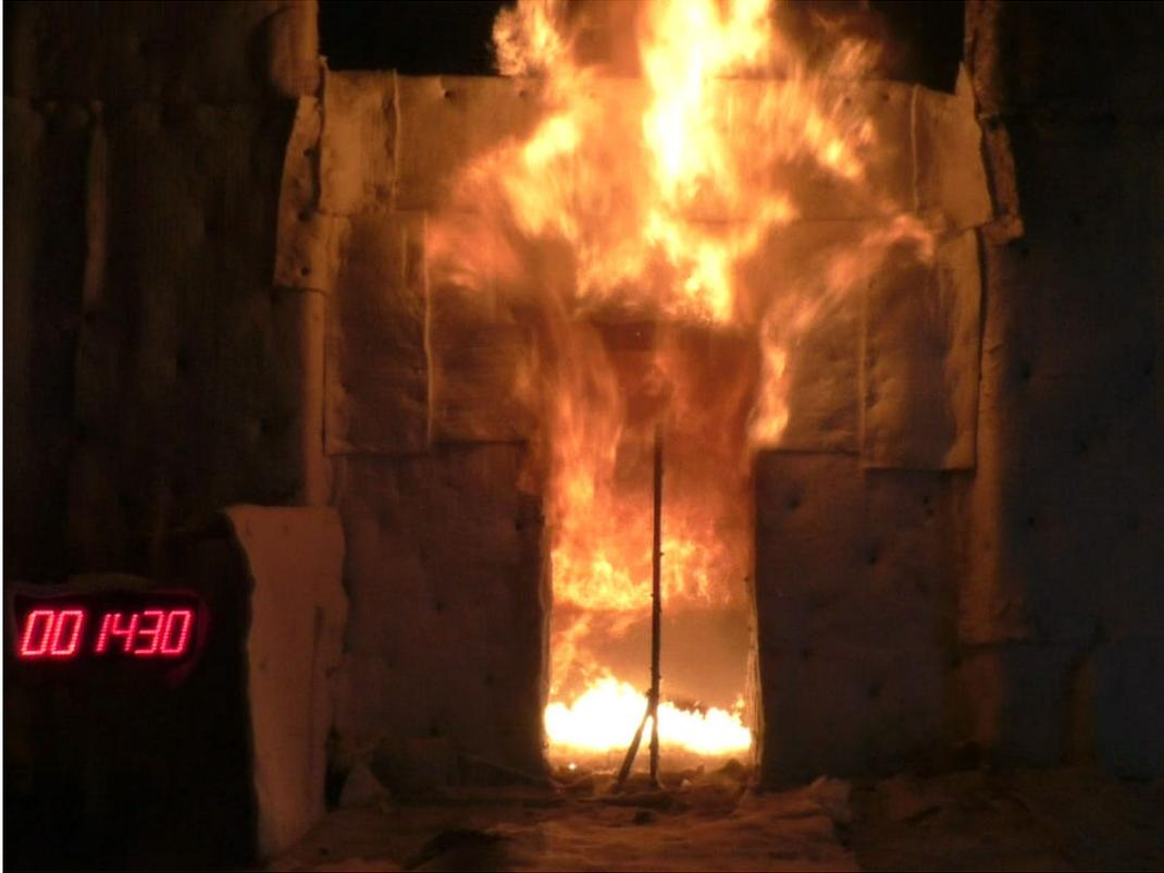
**Figure F-5. CLT #2 Test at 14 min 30 s: Flames on Floor Spread to Door.**
