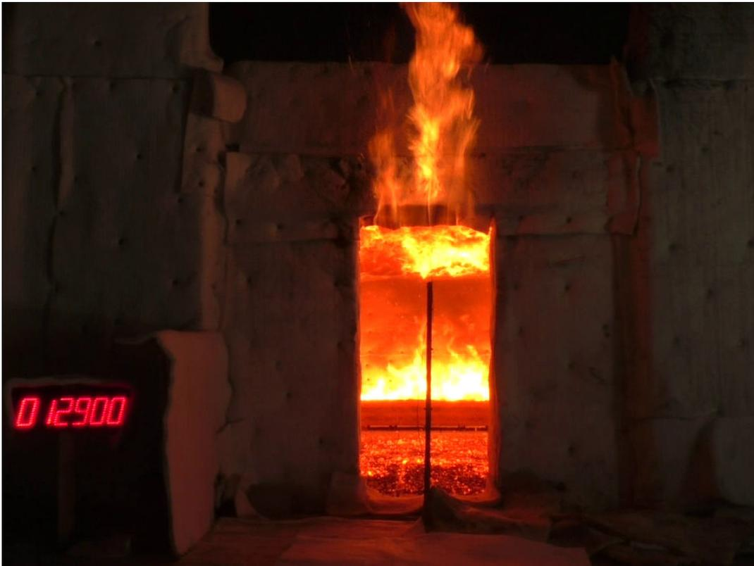
**Figure B- 12. CLT #1 Test at 89 min.**
