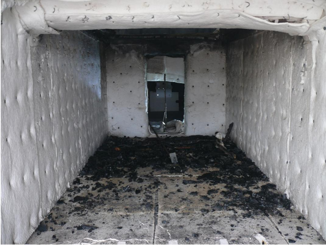
**Figure B-23. CLT #1 Test: Post-Test Picture of Charred Wood on Floor.**
