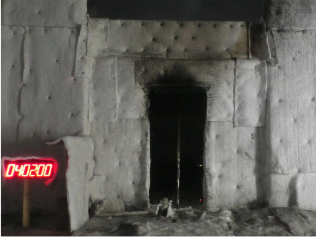
**Figure F-17. End of CLT #3 Test at 242 min.**
