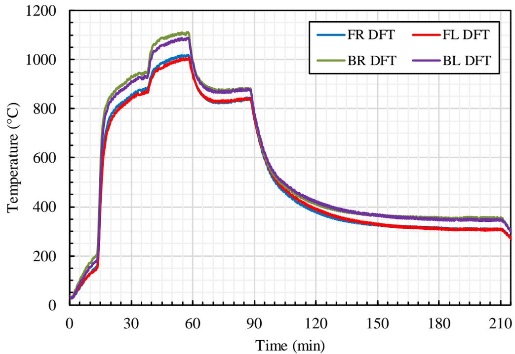
**Figure E-4. CLT #2 Test: DFT Exposed Plate Temperatures.**
