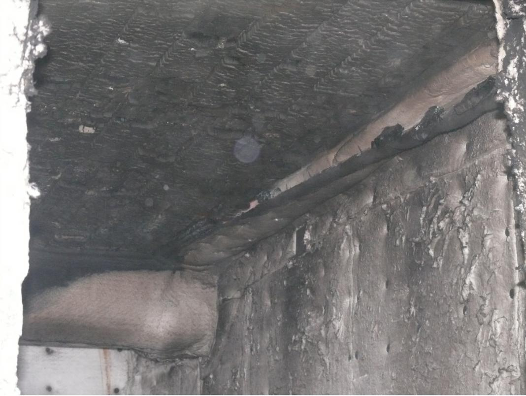
**Figure D-17. CLT #2 Test: Post-Test Picture of CLT Following Extinguishment.**
