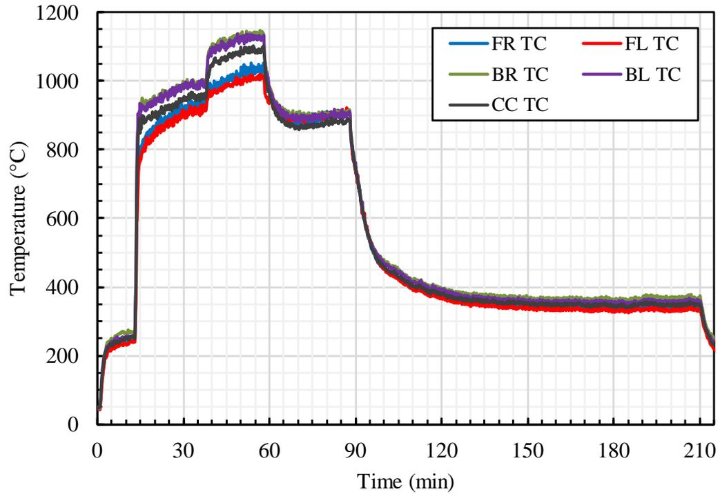
**Figure E-3. CLT #2 Test: Ceiling TC Temperatures.**
