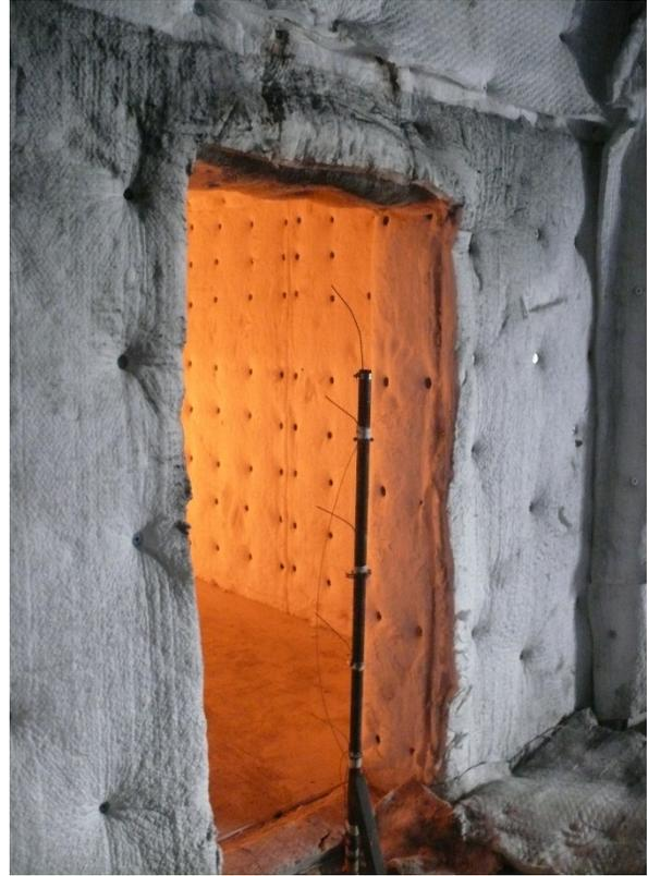
**Figure A-5. Door Thermocouple Tree**
