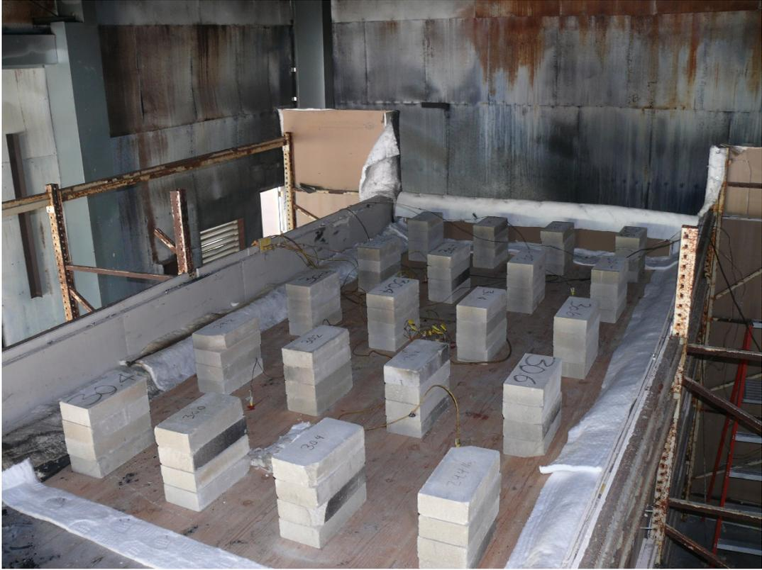
**Figure A-9. Applied Structural Load.**
