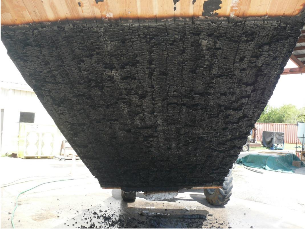
**Figure F-19. CLT #3 Test: Post-Test Picture of CLT Removed from Test Structure.**
