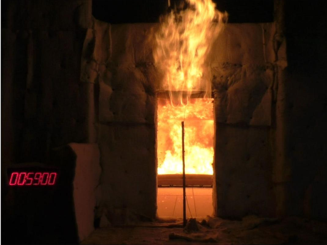
**Figure D-9. CLT #2 Test at 59 min.**
