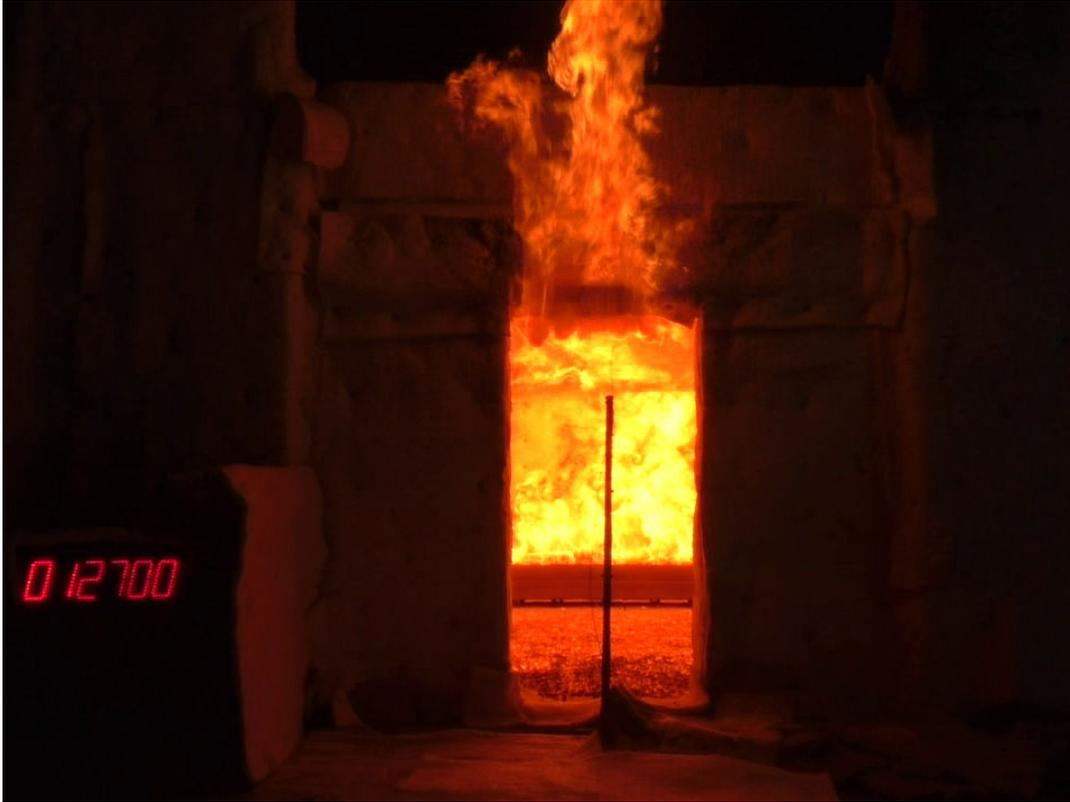
**Figure B- 11. CLT #1 Test at 87 min.**
