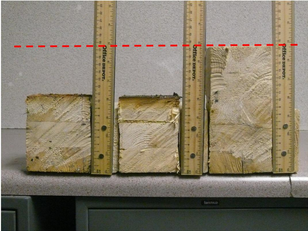
**Figure B- 25. CLT #1 Char Depth: Front Left – Front Right - Original.**
