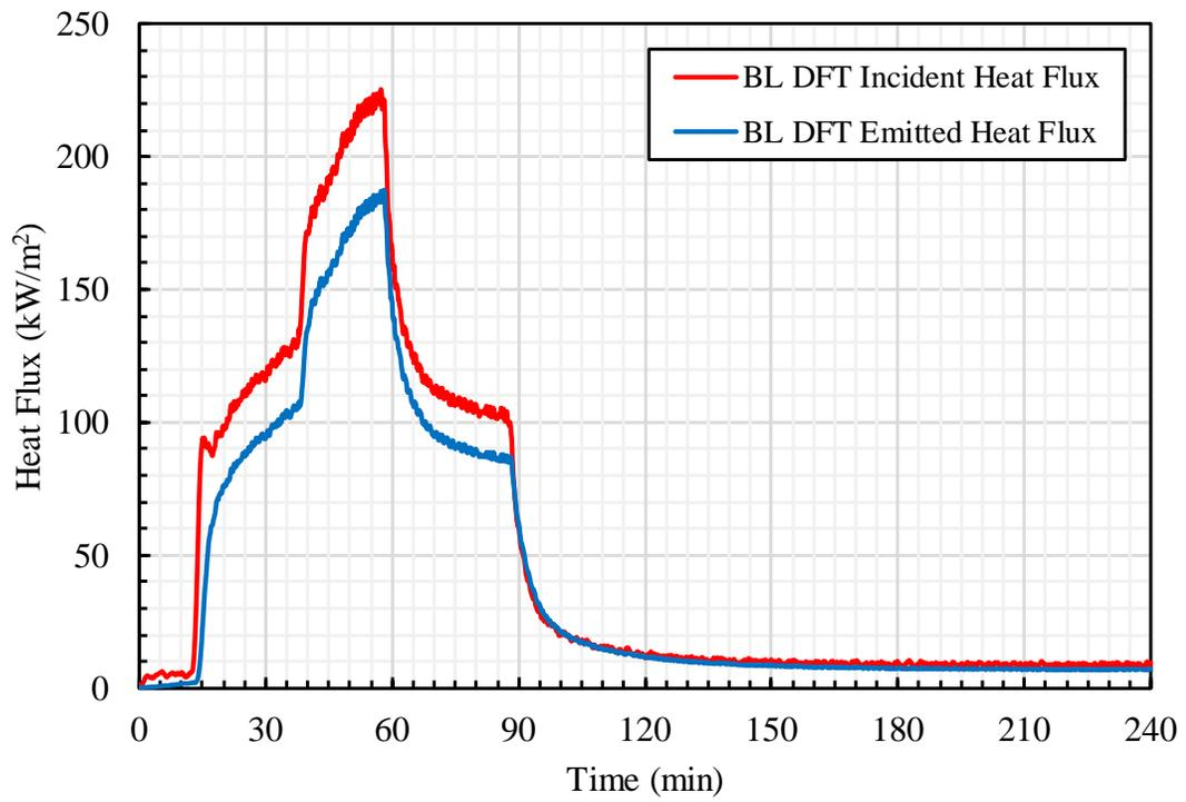
**Figure G-8. CLT #3 Test: Back Left DFT Heat Flux.**
