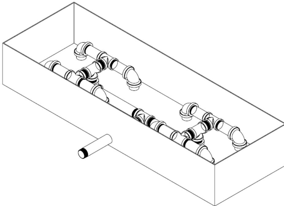
**Figure 1. Schematic of Burner Illustrating Distribution of Propane Flow.**
