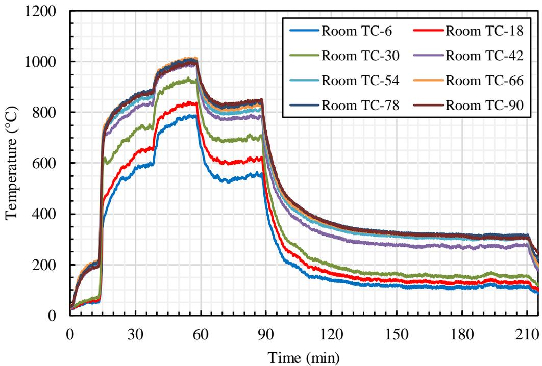
**Figure E-2. CLT #2 Test: Room TC Tree Temperatures.**
