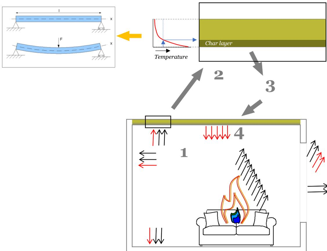
**Predictive method for fires in CLT and glulam structures –
