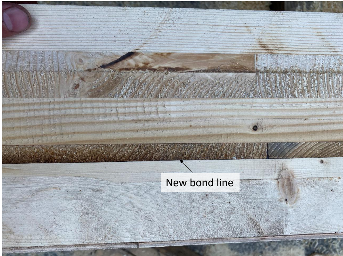
Figure 24: Photo of the longitudinal-section of the rehabilitated CLT member and an indication of the location of the PRF bond line
