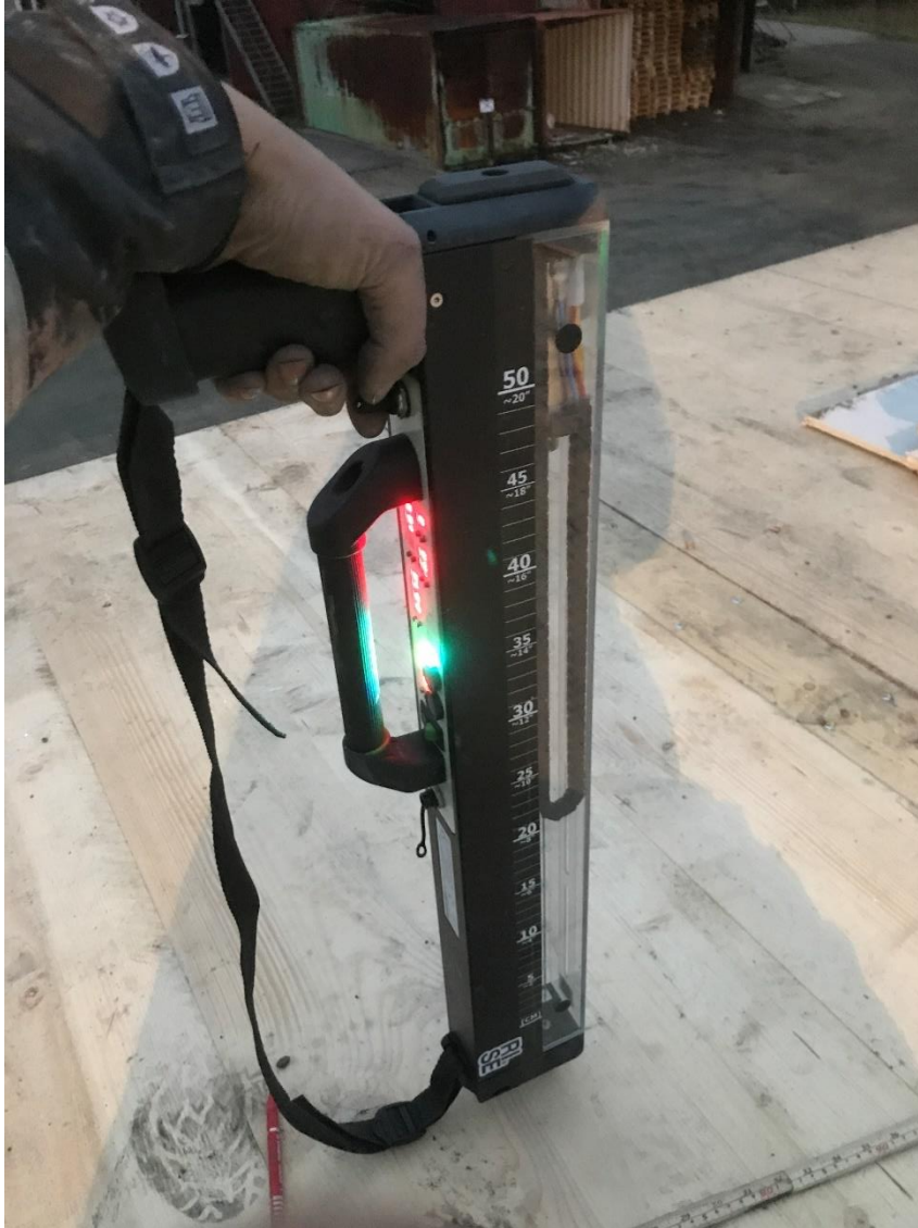
Figure 3: Resistograph, drilling with a thin long drill through the ceiling to identify the thickness of the residual cross section.
