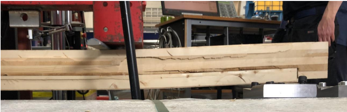
Figure 28: Repaired specimen tested to failure. Shear failure occurred in the cross layer.
