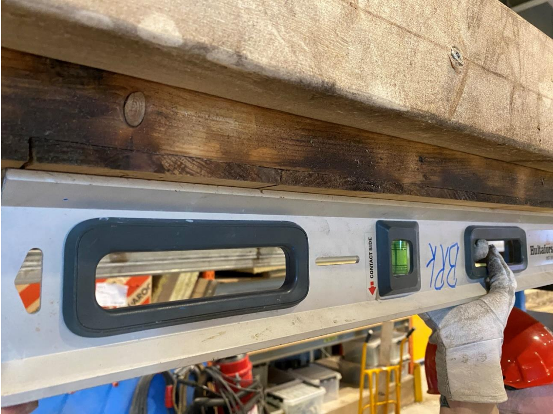
Figure 13: Checking the planeness of the surface
