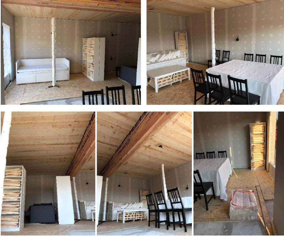
Figure 4. Photos from the interior of the compartment for test 1. Both white couches, the dining table and the wardrobes contained additional wood cribs within. The setup was replicated for all tests.
