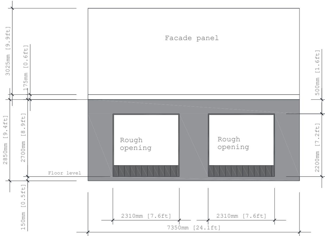
Figure A. 1: Front view of the compartments of Test 1, 2, 3 and 5
