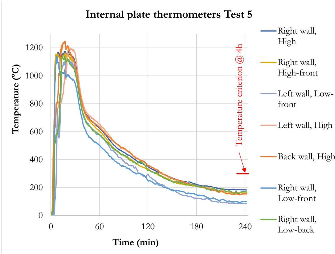
Figure 11: Internal plate thermometer measurements of Test 5
