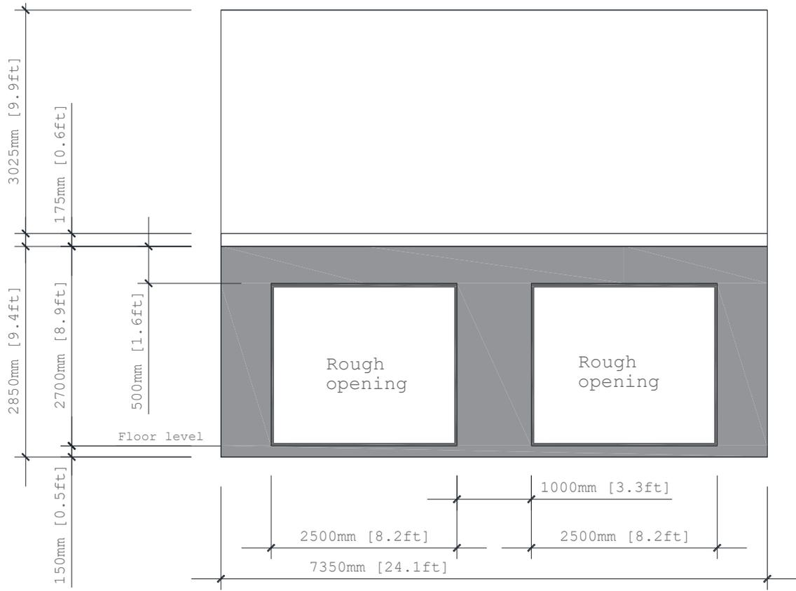
Figure A. 2: Front view of the compartment of Test 4
