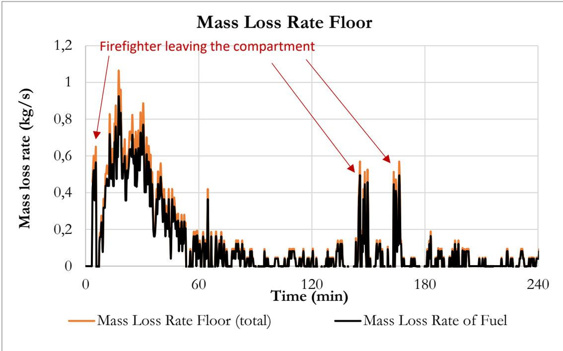
Figure D. 3: Mass loss rate of floor and mass loss rate of fuel of Test 2
