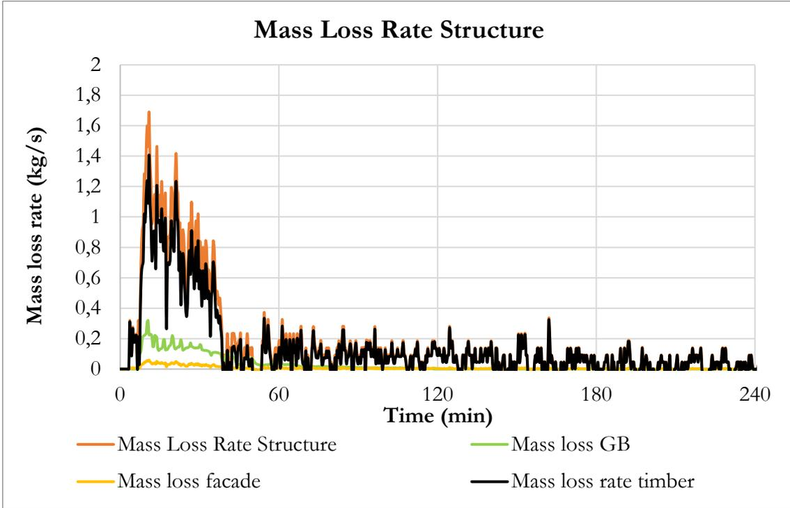
Figure D. 4: Mass loss rate of the structure (excluding floor), façade, gypsum boards and timber surfaces for Test 2.
