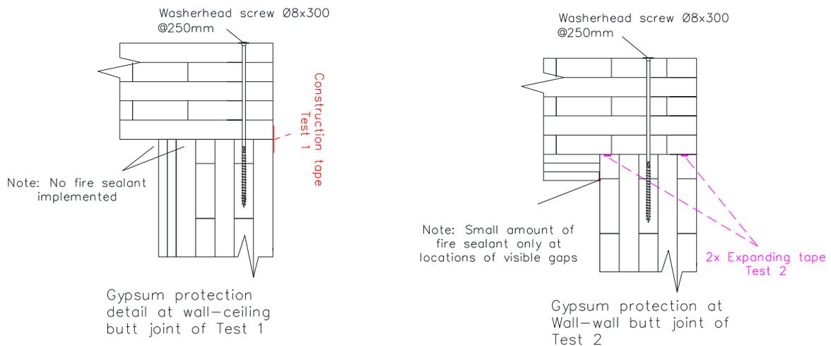
Figure 5: Variants of CLT intersections that only were implemented together with gypsum board protection.
