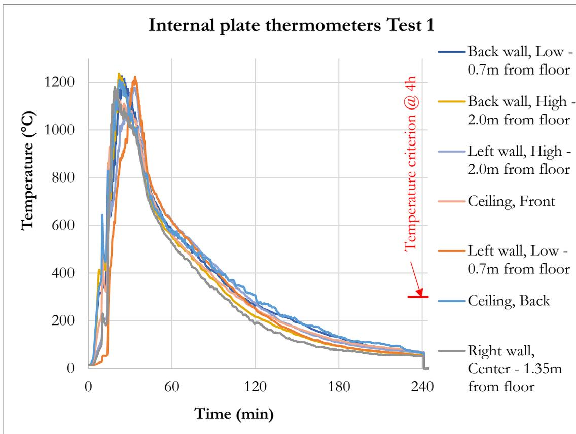
Figure 7: Internal plate thermometer measurements of Test 1
