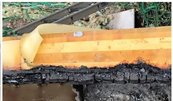
Figure 31: Top of the wall after removal of the ceiling. Typical location. Sealing method: construction tape and resilient profile (Test 2).
