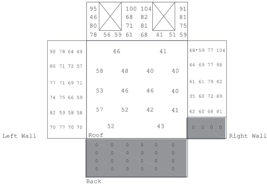
Figure 21: Char depths in mm measured after Test 3 (grey surfaces were protected)
