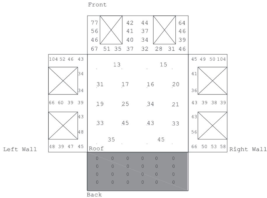
Figure 22: Char depths in mm measured after Test 4 (grey surfaces were protected)
