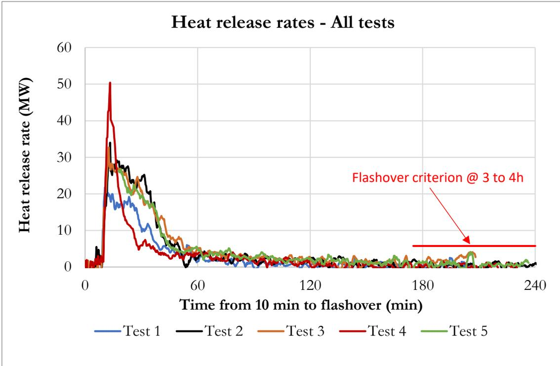
Figure 18: Heat release rates of all tests and the heat release rate flashover criterion of Chapter 3
