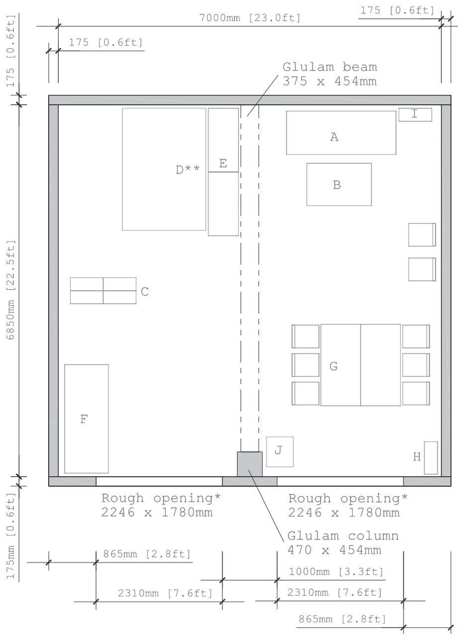
\*The sides of the opening are gypsum board protected. The opening dimensions after gypsum board installation are shown
