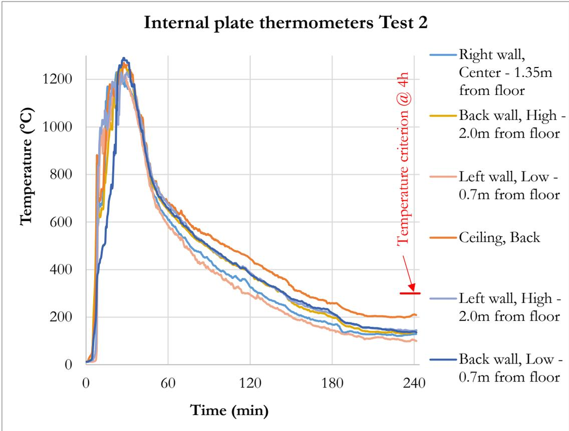
Figure 8: Internal plate thermometer measurements of Test 2
