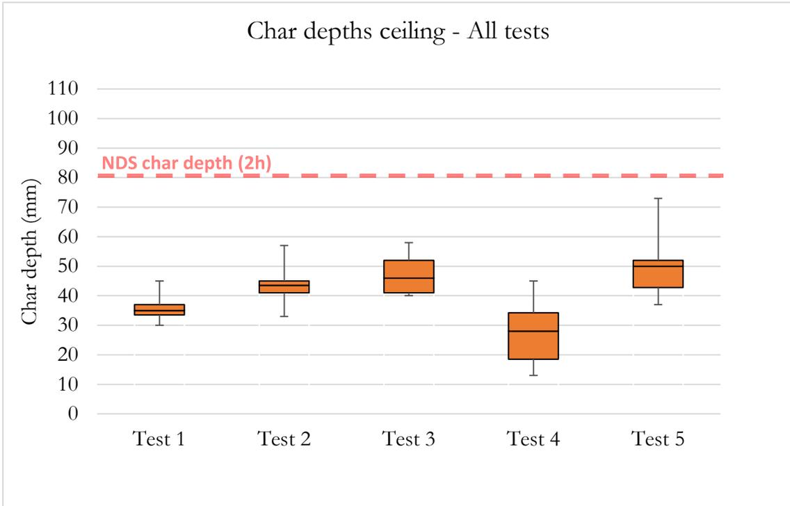
Figure 24: Box plots of char depths in the CLT surface of the ceiling
