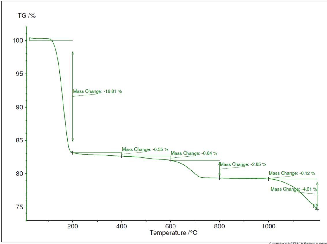
Figure D. 2: TGA results of Type X gypsum board conducted with a NETZSCH F3 Jupiter. Heating rate: 20°C/min from 20 °C to 1200 °C in an N<sub>2</sub> atmosphere.
