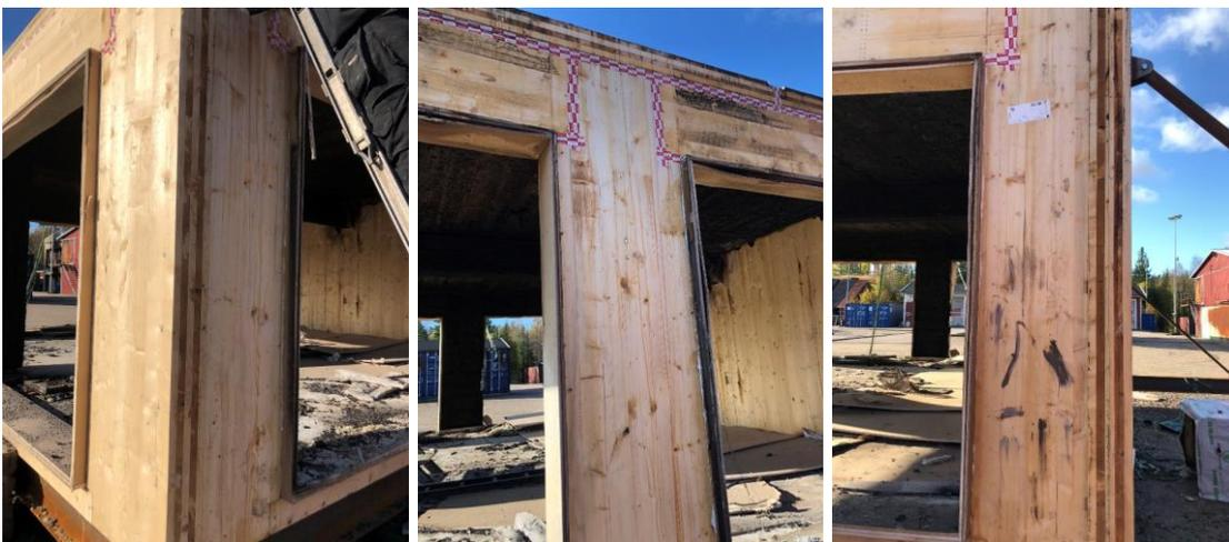
Figure F. 15. Test 4 – Right façade after removal of gypsum boards.
