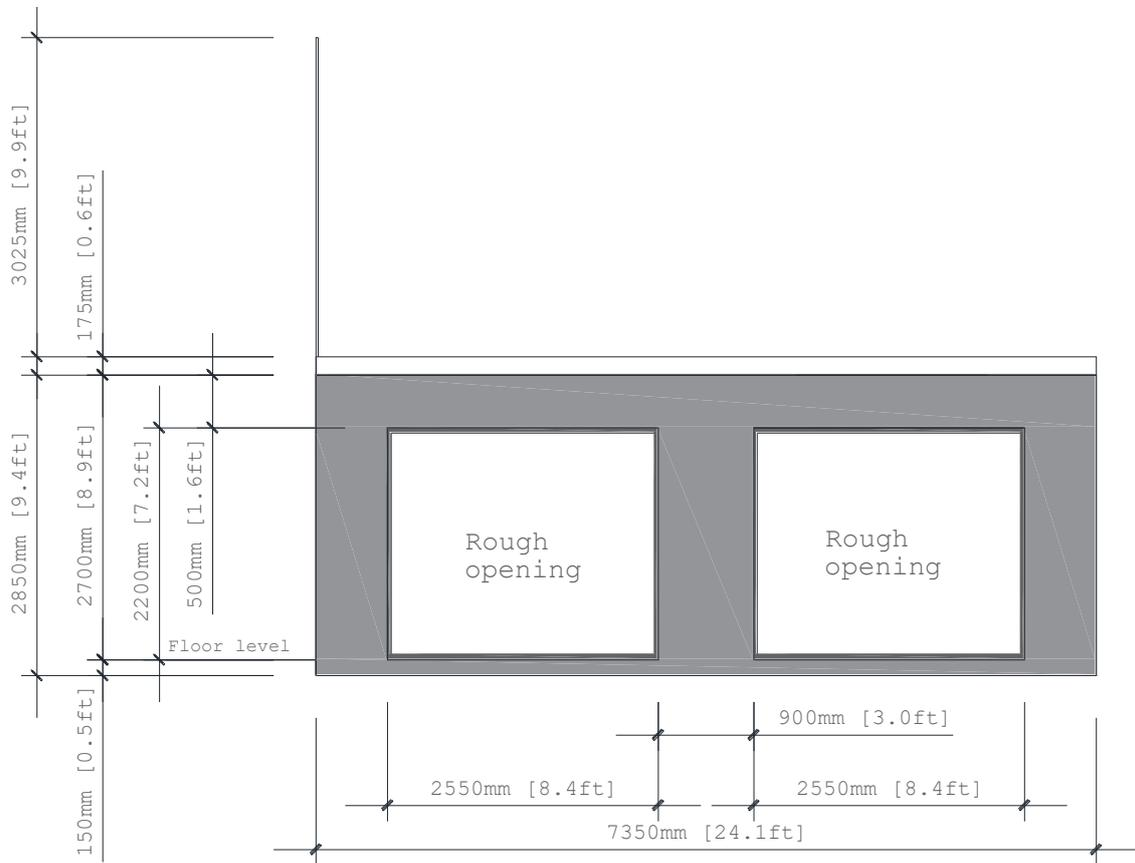
Figure A. 3: Side view of the compartment of Test 4
