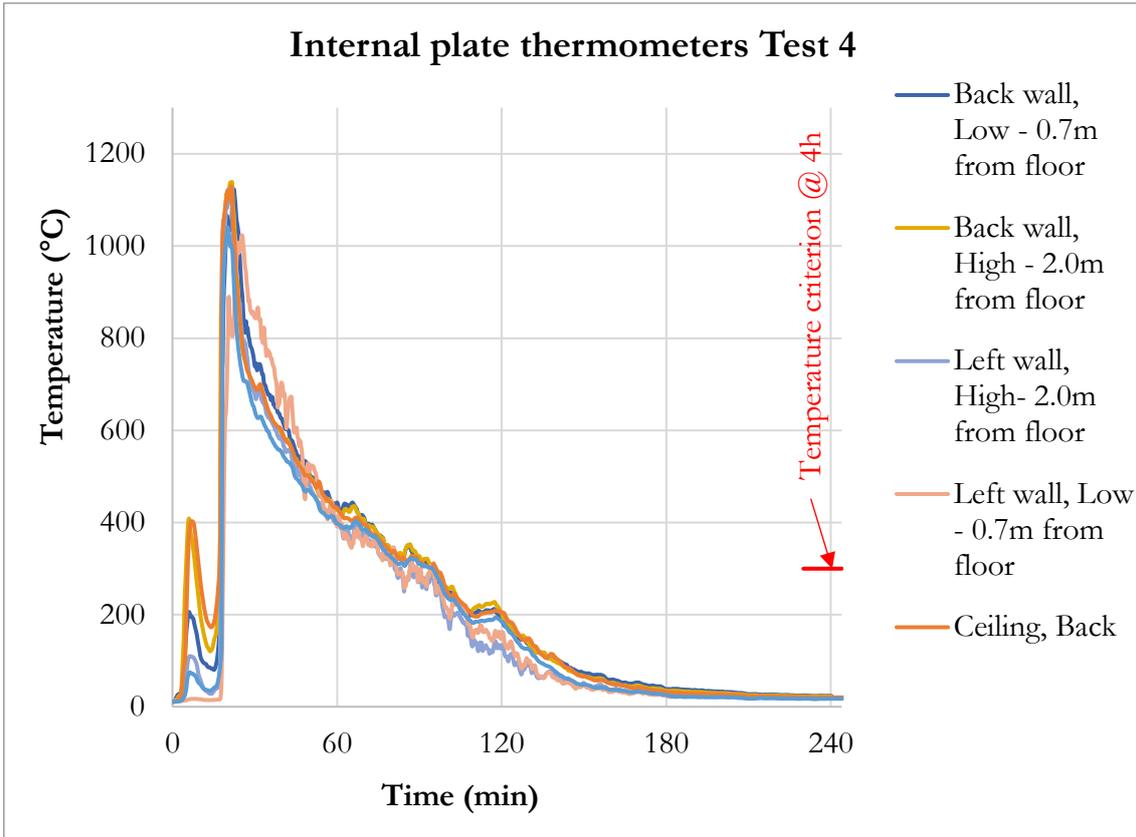
Figure 10: Internal plate thermometer measurements of Test 4
