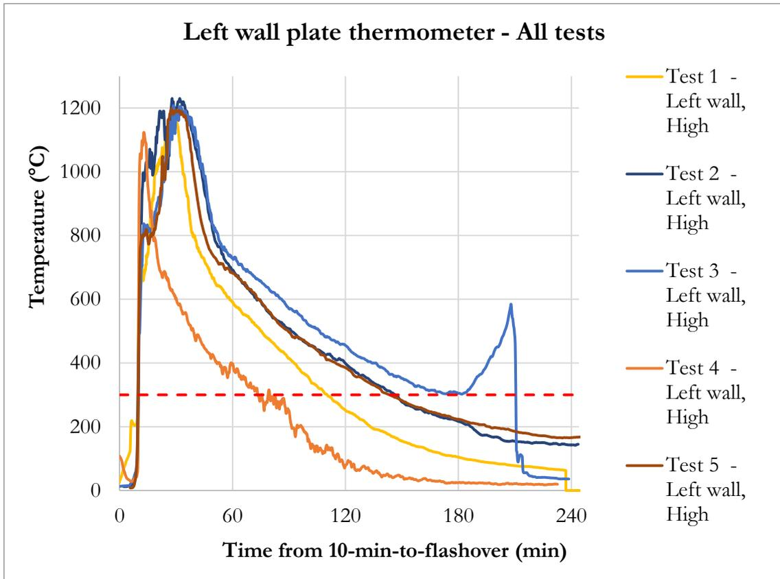
Figure 12: Left wall plate thermometer measurements at 2.0 meters (6.6ft) from the floor of all tests. The red dashed line indicates the 300 °C criterion at 4 hours.
