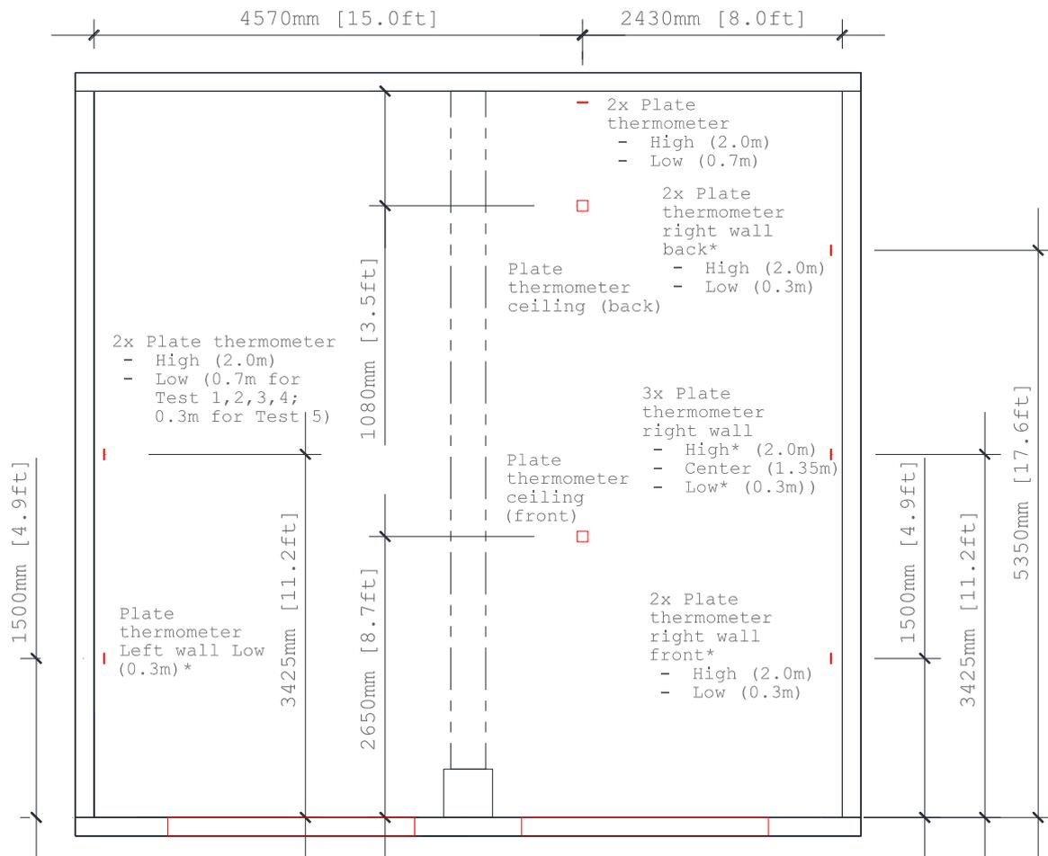
Figure 6: Locations of plate thermometers (includes only plates at surfaces that are directed away from the surface).
