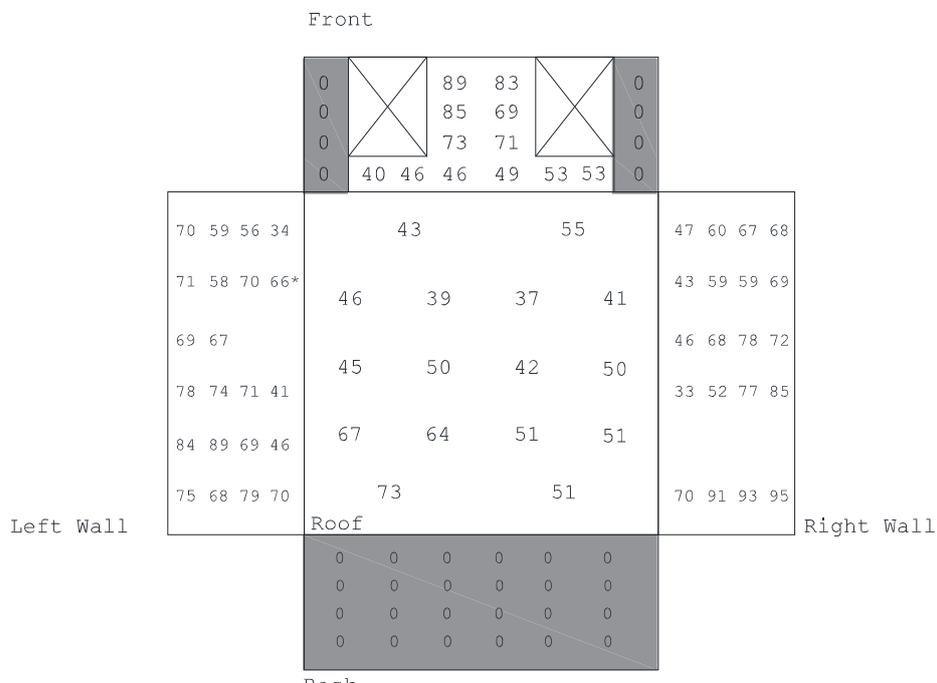
Figure 23: Char depths in mm measured after Test 5 (grey surfaces were protected)
