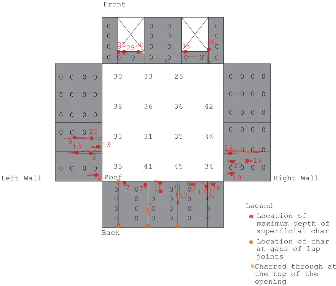
Figure 19: Char depths in mm measured after Test 1 (grey surfaces were protected)
