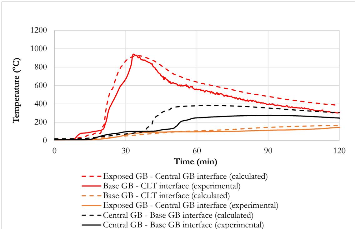
Figure D. 1: Measured and calculated temperatures at interfaces between gypsum boards (Example for Test 3).
