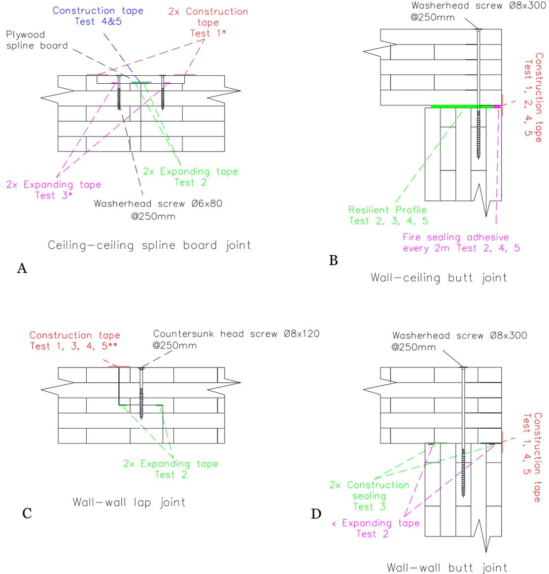
Figure 4: Variants of sealed CLT intersections and their sealing details (different colours represent different sealing types and/or locations)
