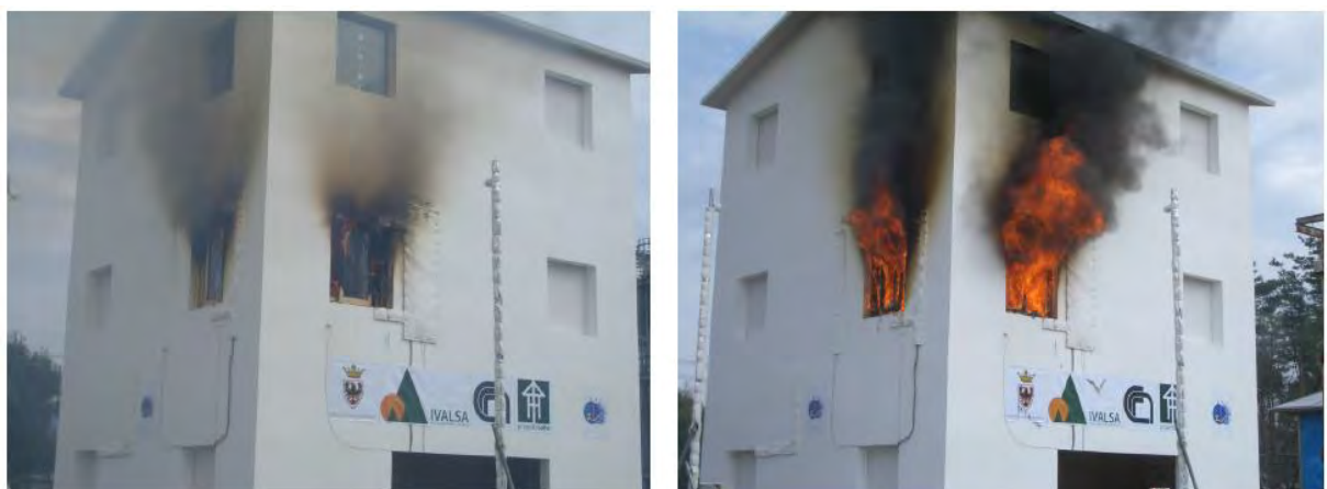
Figure 3: Fire after 32 minutes (left) and 40 minutes (right)
