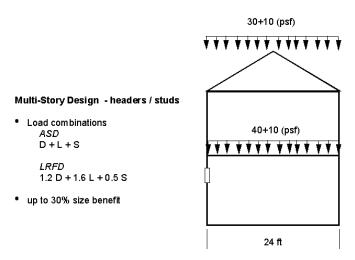
Figure 7 Case Study - headers for typical two-story structure
