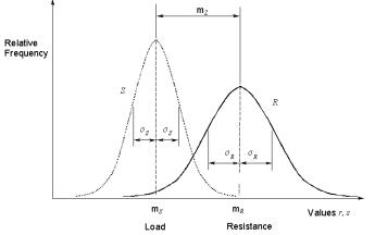
Figure 2 Sample distributions of load (S) and resistance (R)
