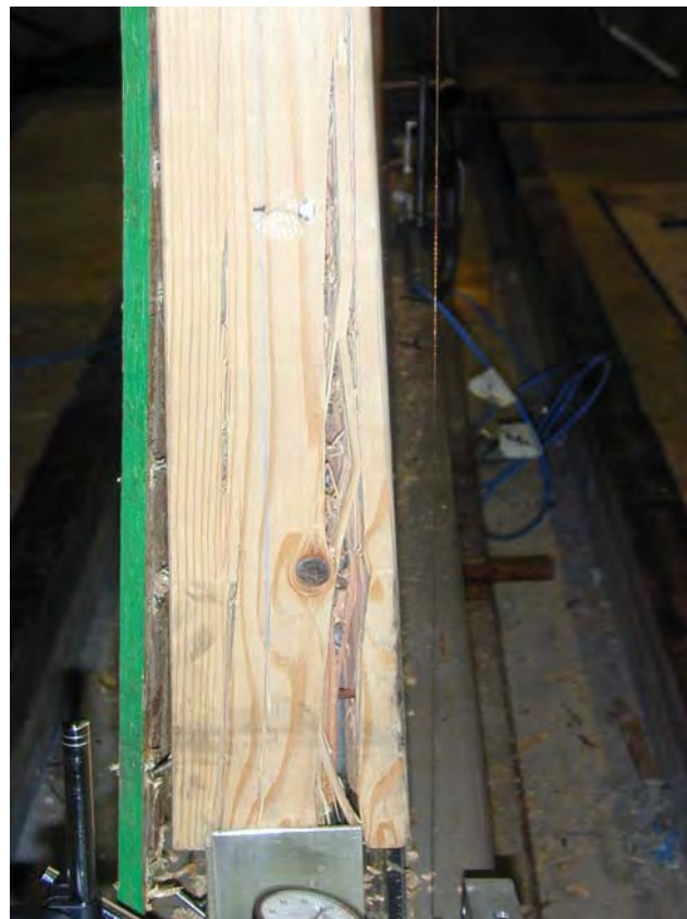
Figure 15. End stud failure (Specimen B1)
