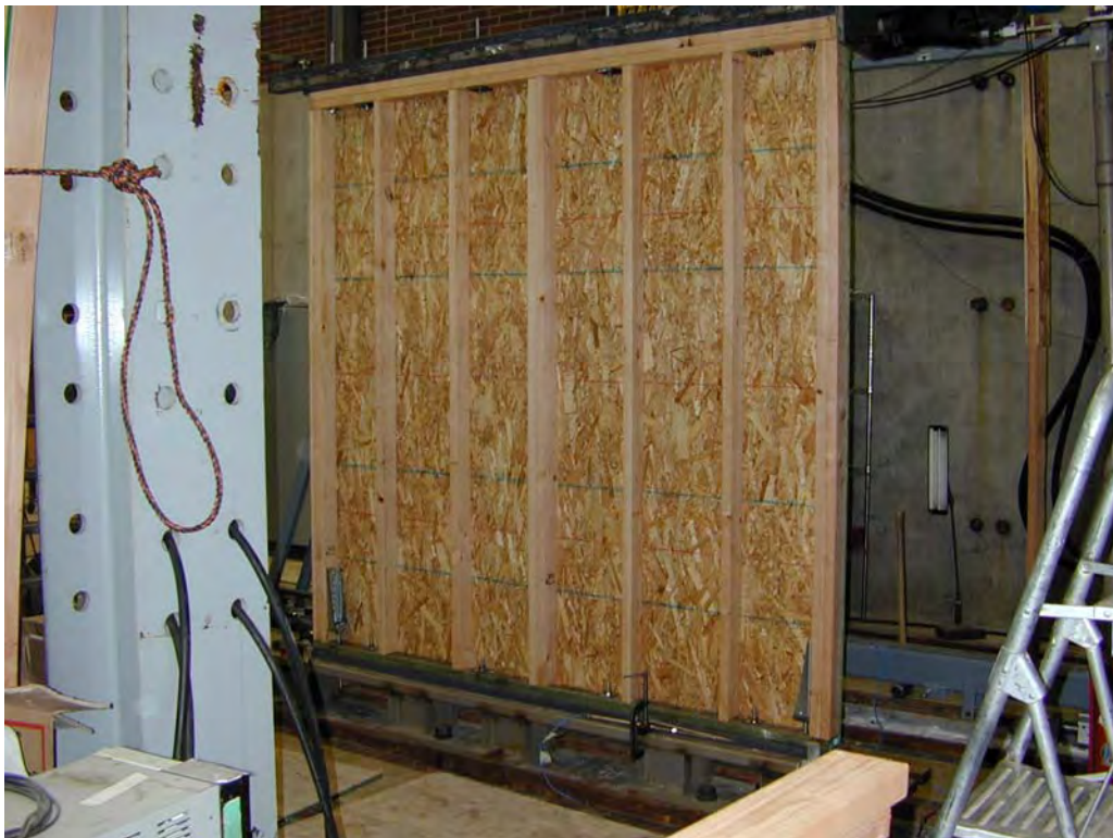
Figure 2. Shearwall assembly in test fixture
