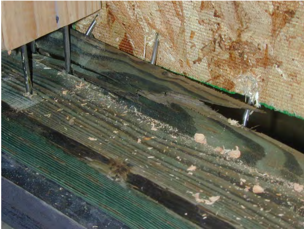
Figure 12. Close-up of sole plate splitting (Specimen A3)
