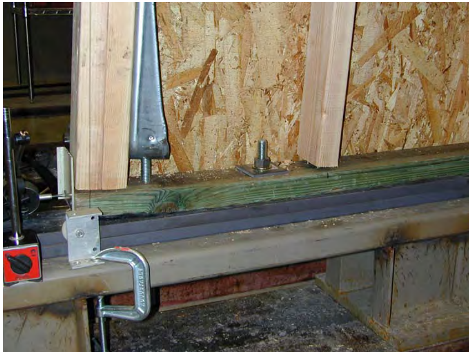
Figure 6. Uplift of sole plate at hold-down (Specimen A1)
