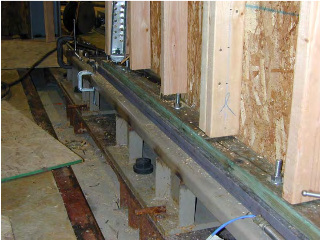
Figure 22. Sole plate split along its length (Specimen C1)
