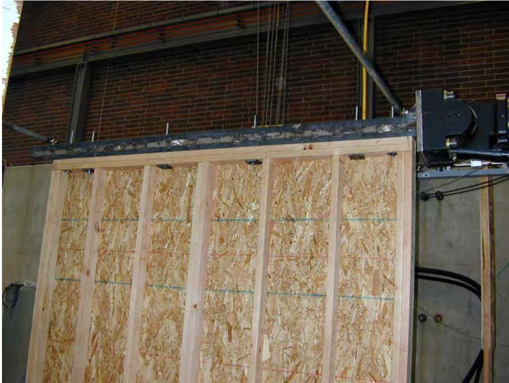
Figure 3. Shearwall assembly showing top loading beam and coupling to actuator
