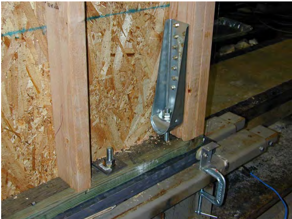
Figure 4. Hold-down in corner of shearwall
