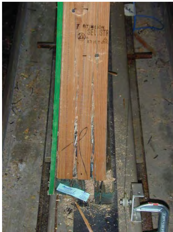
Figure 21. End stud and sole plate failures (Specimen C1)
