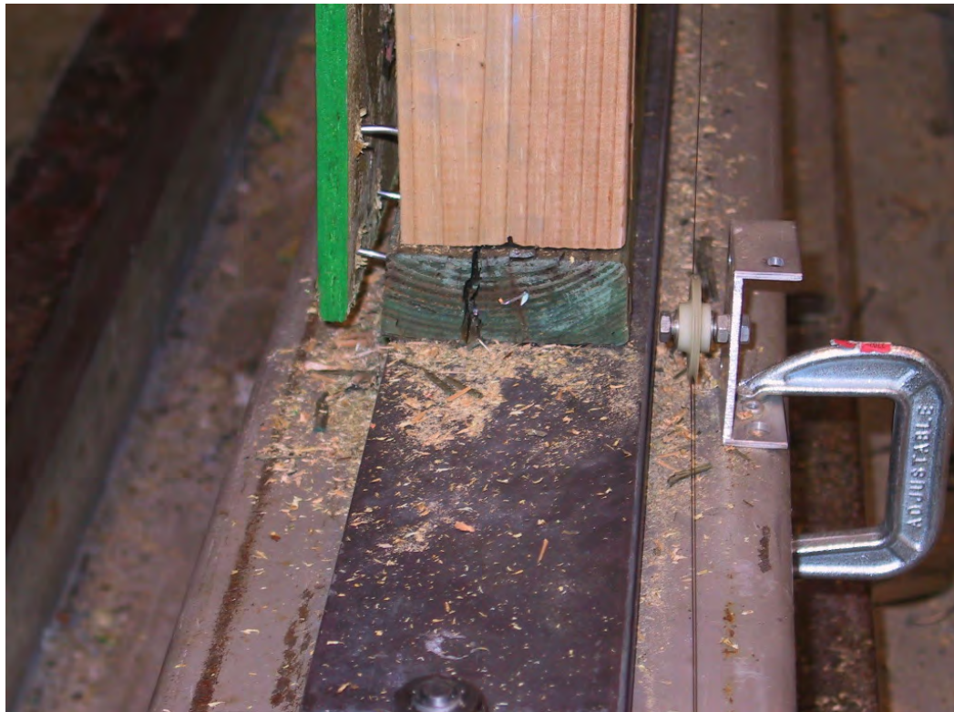
Figure 26. Failure at end of wall showing sole plate splitting (Specimen C2)
