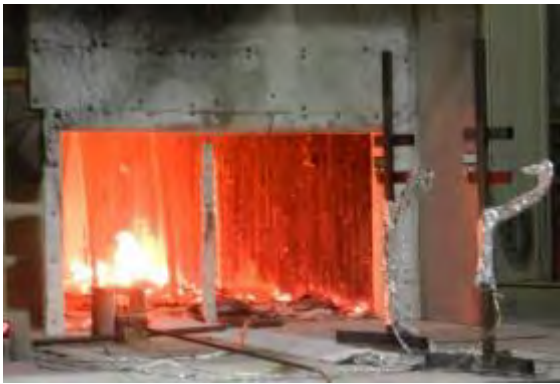
(c) exposed W1 at 48 min: charred, no visible flame
