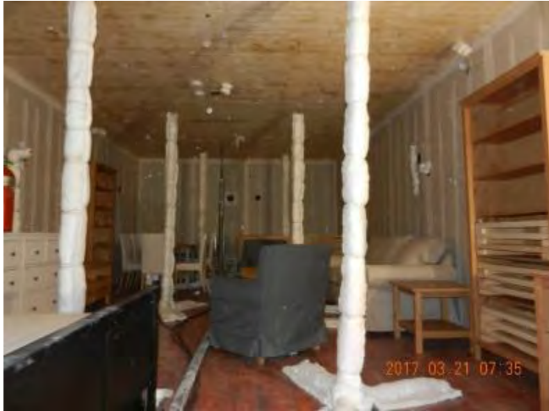
Figure 71. Photograph of CLT compartment with exposed ceiling for Test 1-4.
