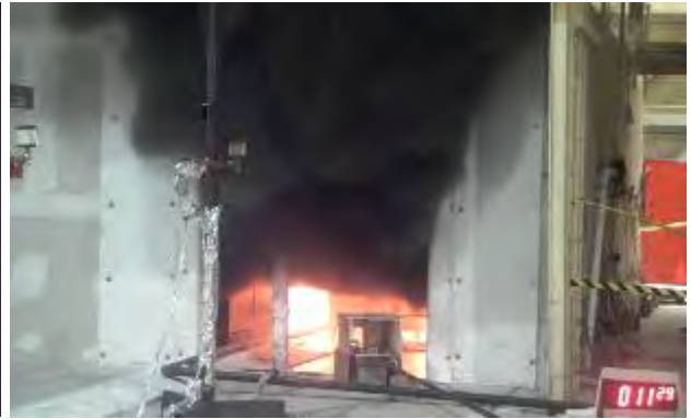
(b) just before flashover
