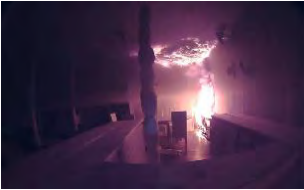
(a) ceiling ignited in corner
