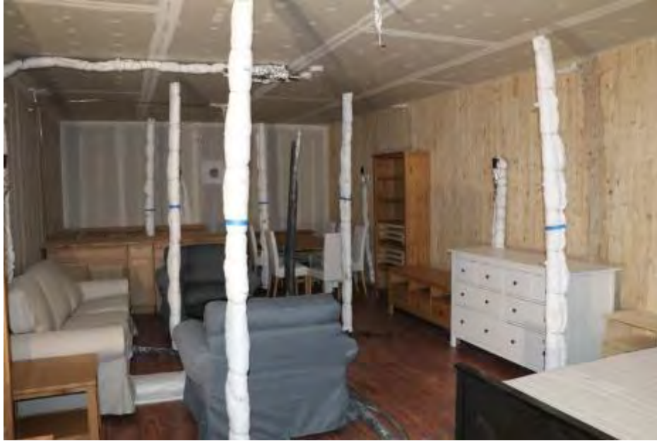
Figure 80. Photograph of CLT compartment with exposed W1 wall for Test 1-5.
