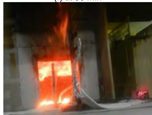
(h) at 151 min, second flashover
