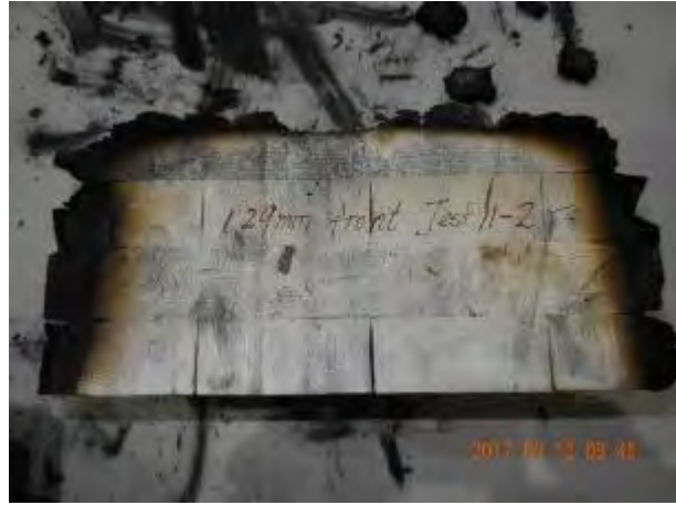
(b) front block near TC Tree 3 charred 46 mm
