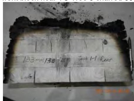
(d) rear block near TC Tree 4 charred 42 mm
