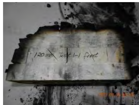
(b) front block near TC Tree 3 charred 55 mm
