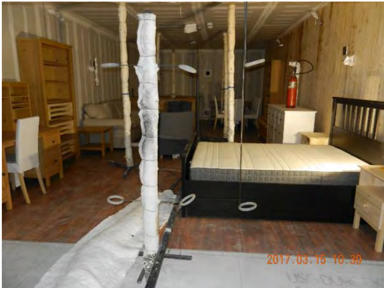
Figure 61. Photograph of CLT compartment with exposed W1 wall for Test 1-3.
