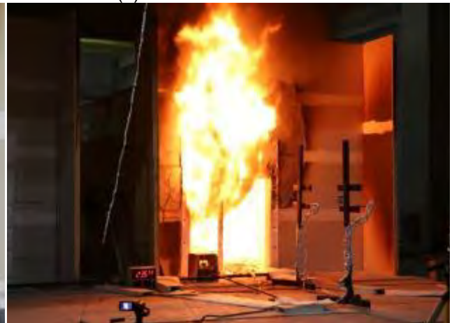
(f) second flashover at 155 min
