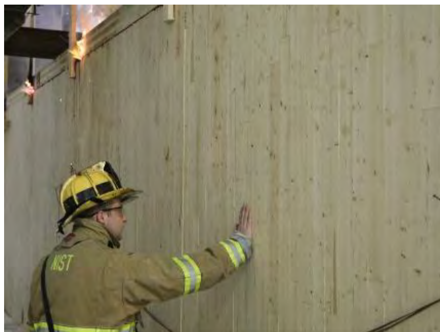
Figure 68. Exterior of the W1 wall at 198 min in Test 1-3.
