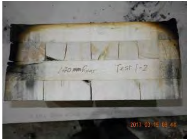
(d) rear block near TC Tree 4 charred 35 mm
