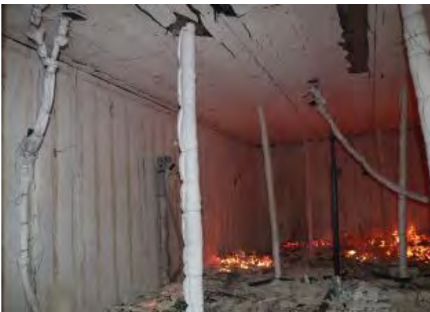
(e) at 130 min – near end of test, gypsum board remained: 2 layers on ceiling; 3 layers on walls
