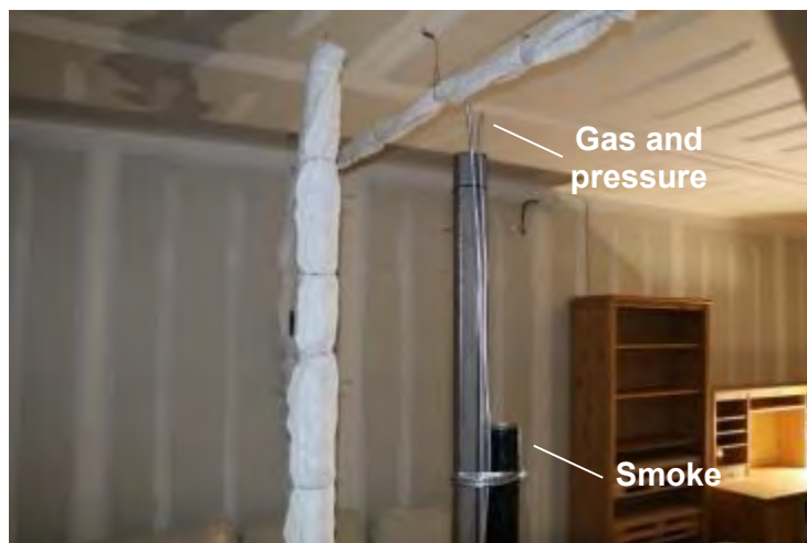
Figure 30. Photograph of stand with gas sampling tubes.
