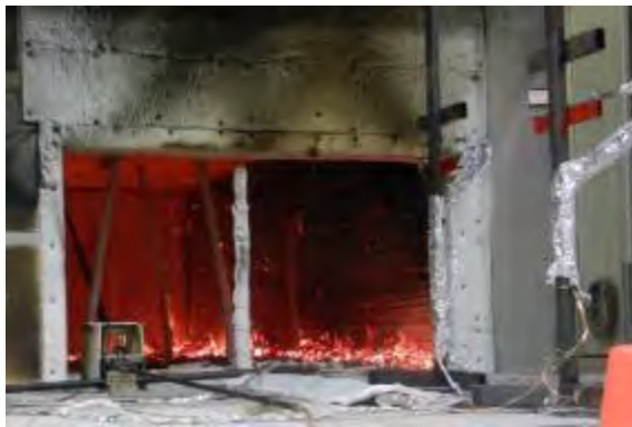
(e) exposed W1 at 120 min after 1 st ply falling off
