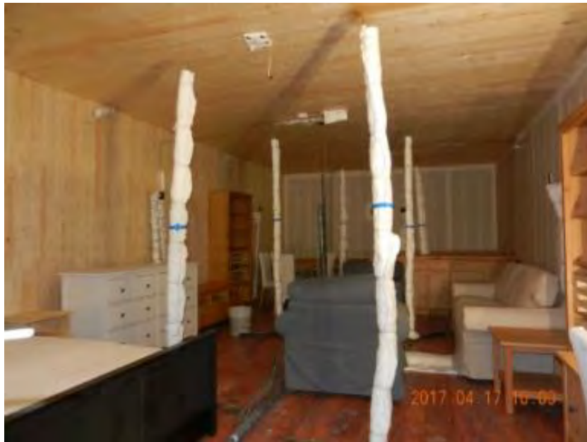
Figure 93. CLT compartment with exposed ceiling and W1 wall for Test 1-6.
