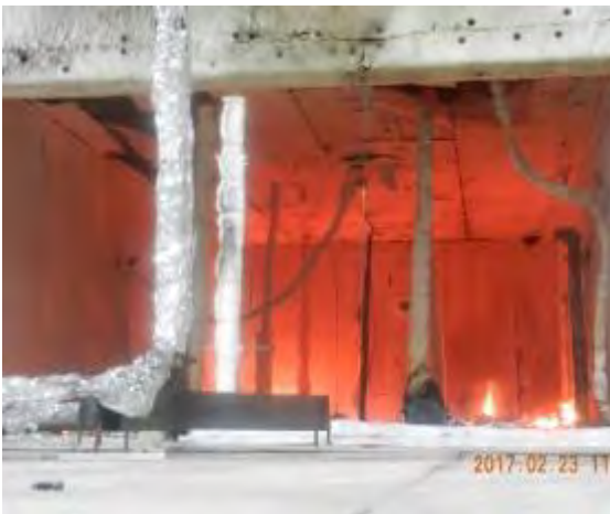
(e) at 100 min – near end of test, gypsum board remained: base layer on ceiling; 2 layers on walls
