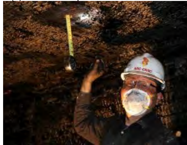
(d) char measurement by drilled holes
