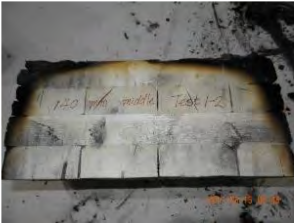
(c) middle block near TC Tree 6 charred 35 mm
