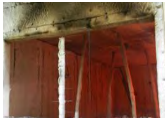
(h) two GB layers on ceiling and W3 and W4 at 240 min
