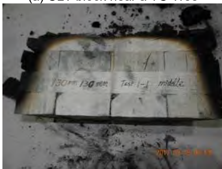
(c) middle block near TC Tree 6 charred 45 mm
