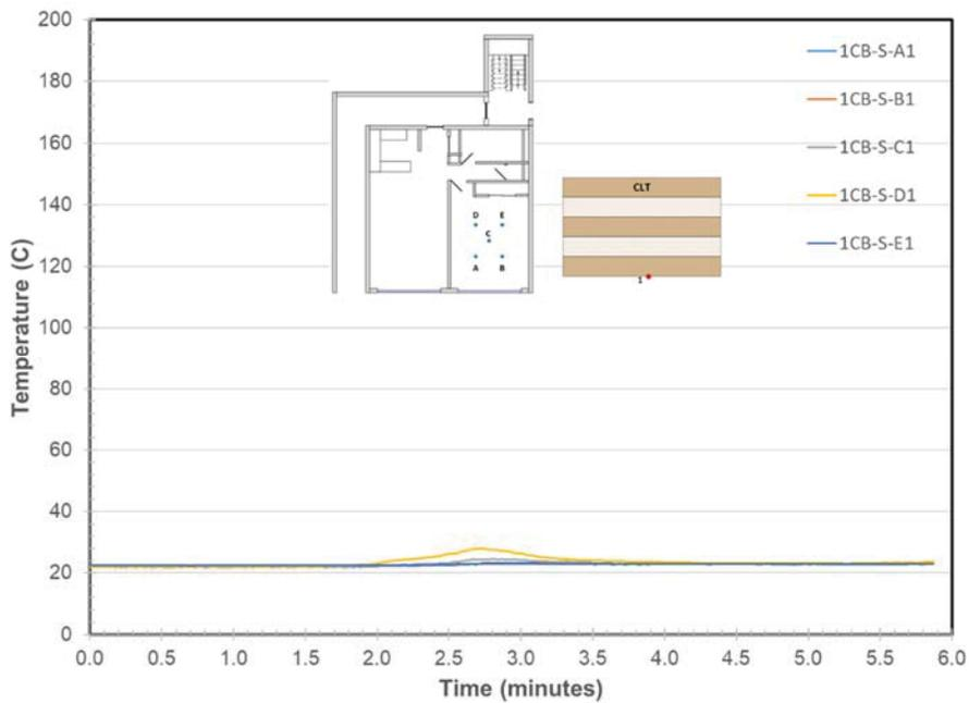
**Figure 241. Bedroom Ceiling Surface Temperatures at Locations A through E**
