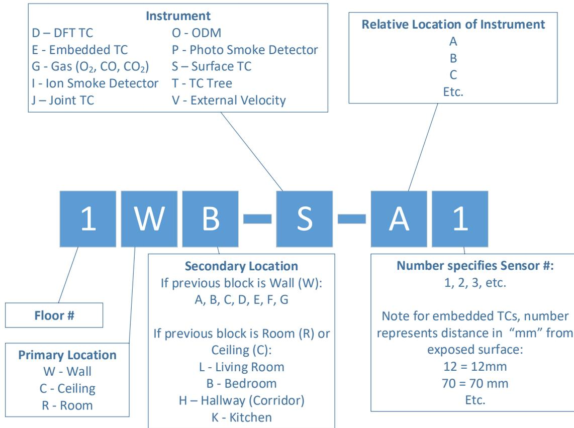
**Figure 1. Nomenclature of Instrumentation Location**
