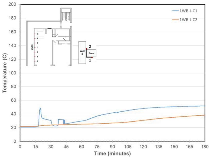
Figure 942. Wall B/Steel Angle Joint Temperatures at Location C
