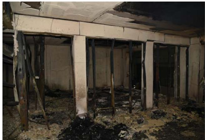
**Figure 59. Interior view of apartment after Test 2.**
