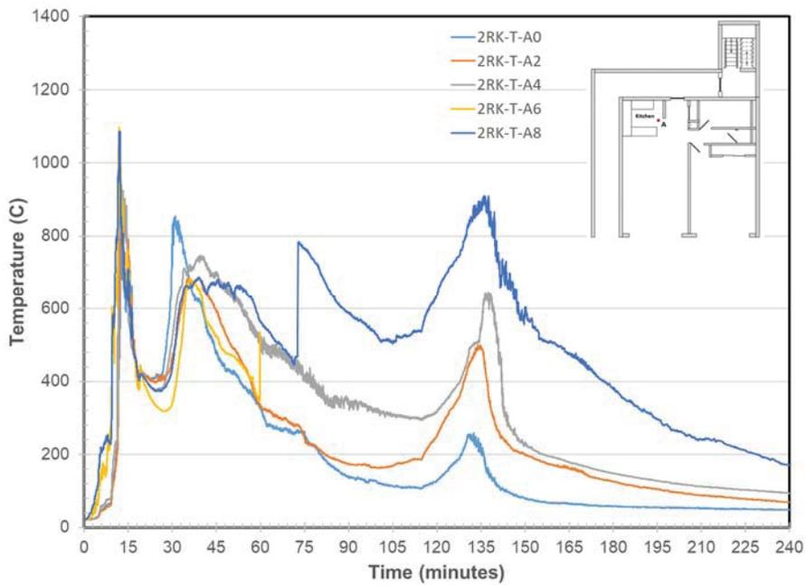
**Figure 13. Kitchen Temperatures at Location A**
