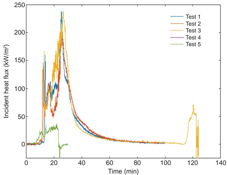
**Figure 110. Directional flame thermometer incident heat flux estimates in Wall B, location B, for each test.**
