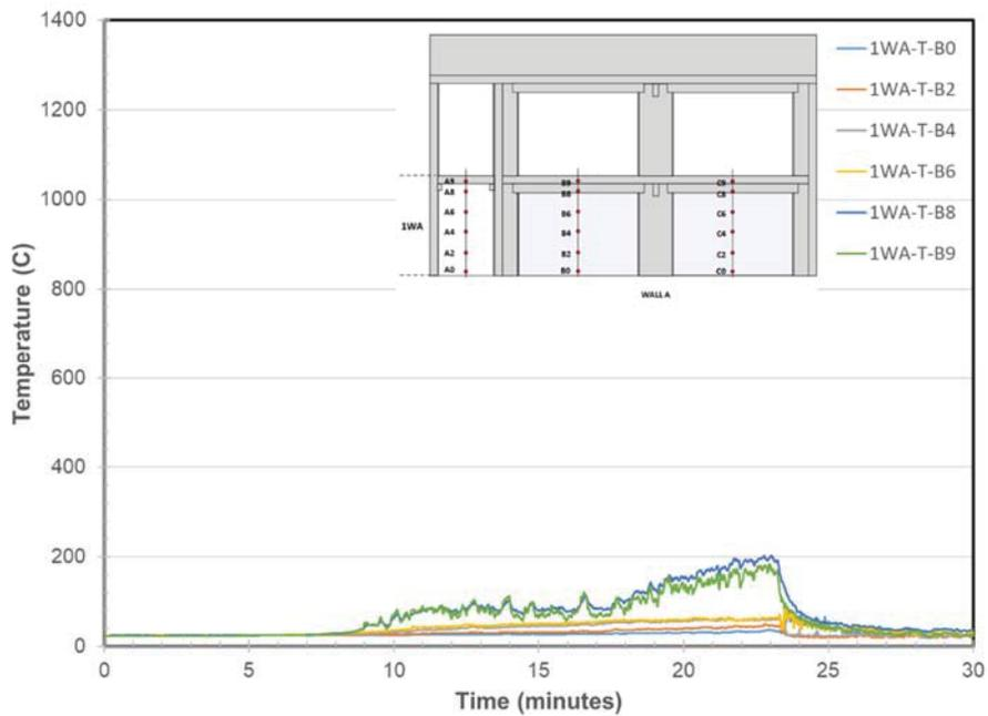
**Figure 18. Wall A Temperatures at Locations B**
