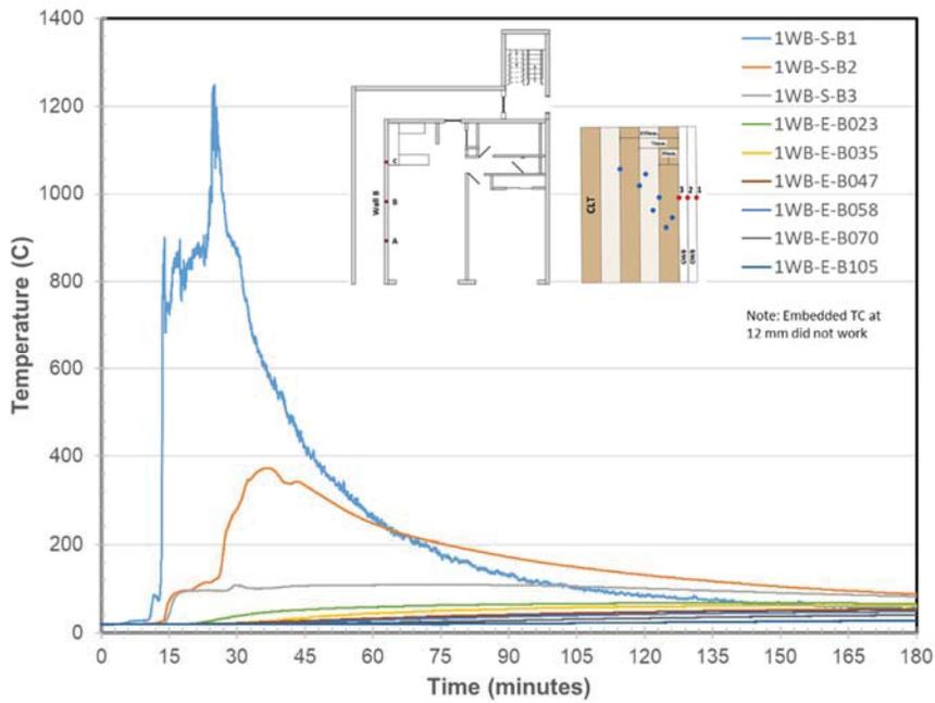
Figure 924. Wall B Embedded & Surface Temperatures at Location B
