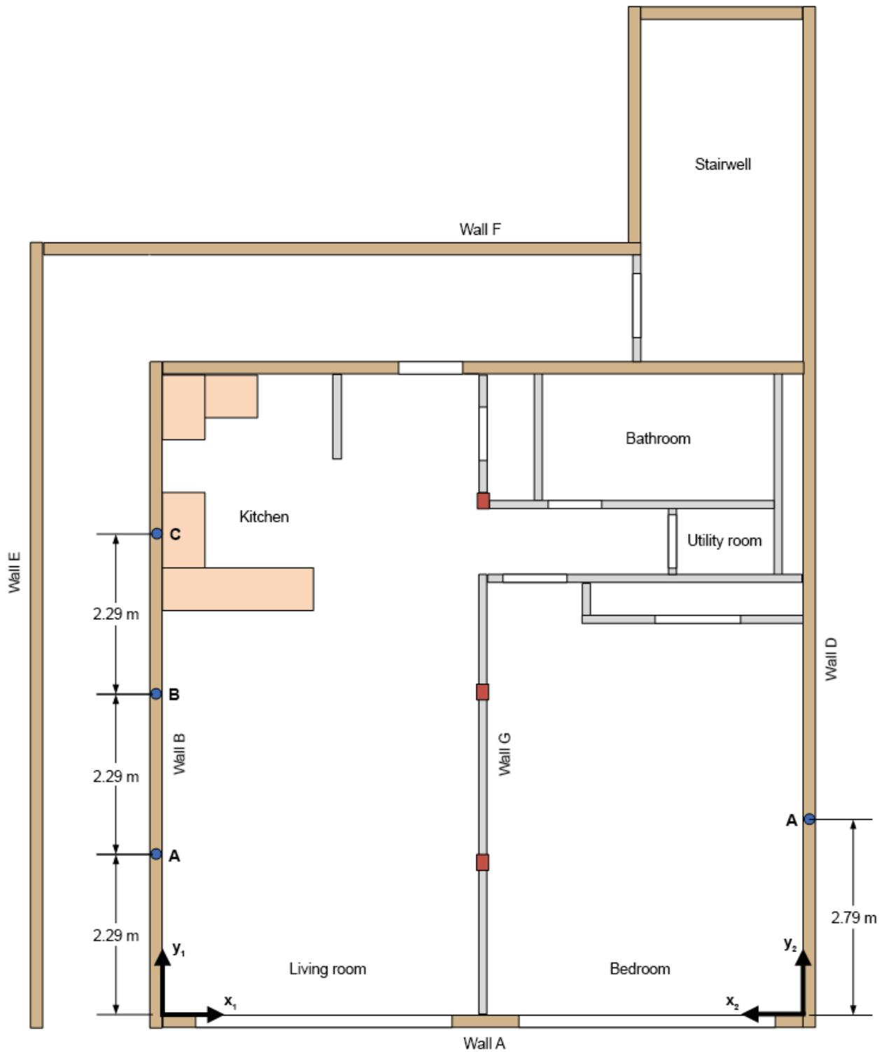
Figure 70. Location of embedded and surface wall thermocouples (blue circles) (thermocouples located 1.52 m above the finished floor).
