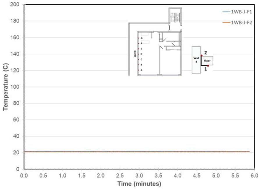
Figure 254. Wall B/Steel Angle Joint Temperatures at Location F
