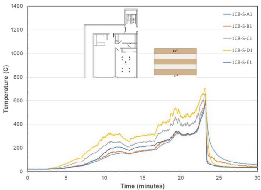
**Figure 12. Bedroom Ceiling Surface Temperatures at Locations A through E**
