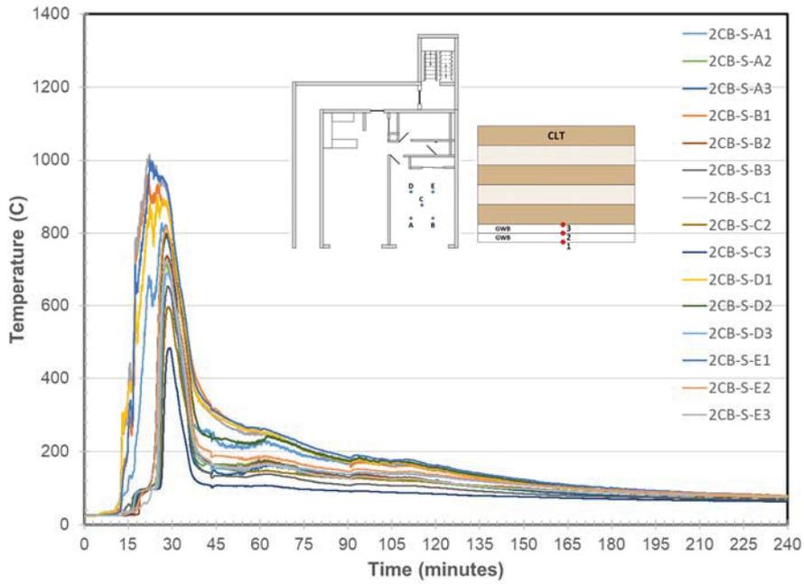
Figure 217. Bedroom Ceiling Surface Temperatures at Locations A through E
