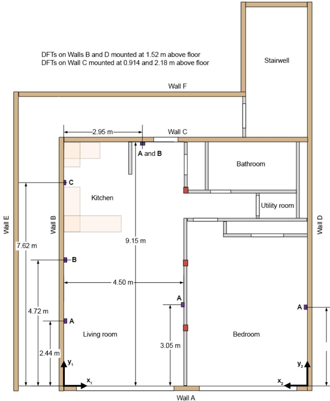
Figure 85. Location of directional flame thermometers (DFTs) on interior walls (purple rectangles).
