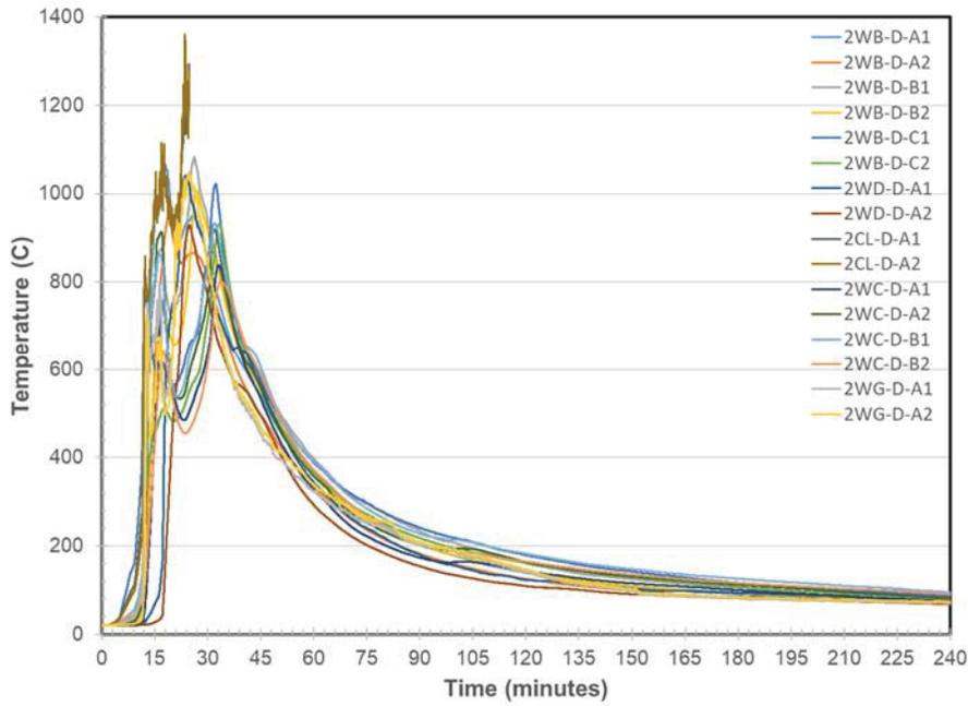
**Figure 32. DFT Temperatures at each Location**
