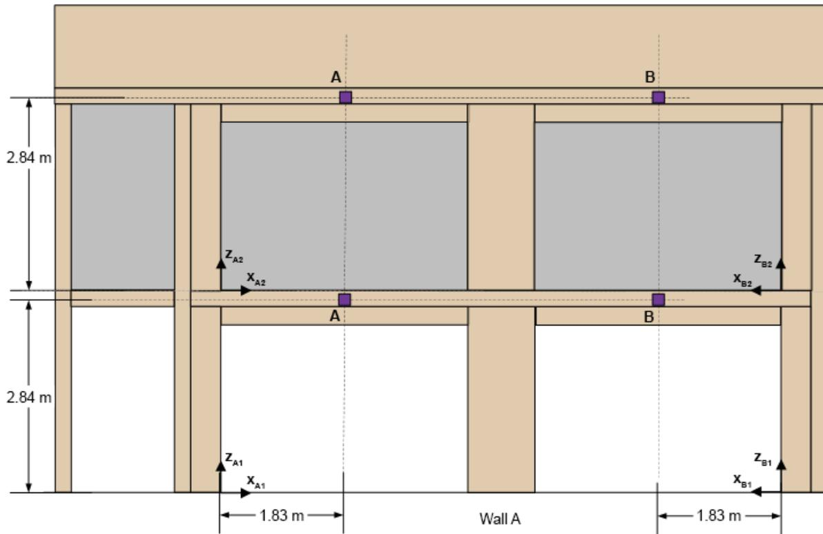
Figure 89. Location of directional flame thermometers on Wall A (purple squares) (see also photograph in Fig. 52).
