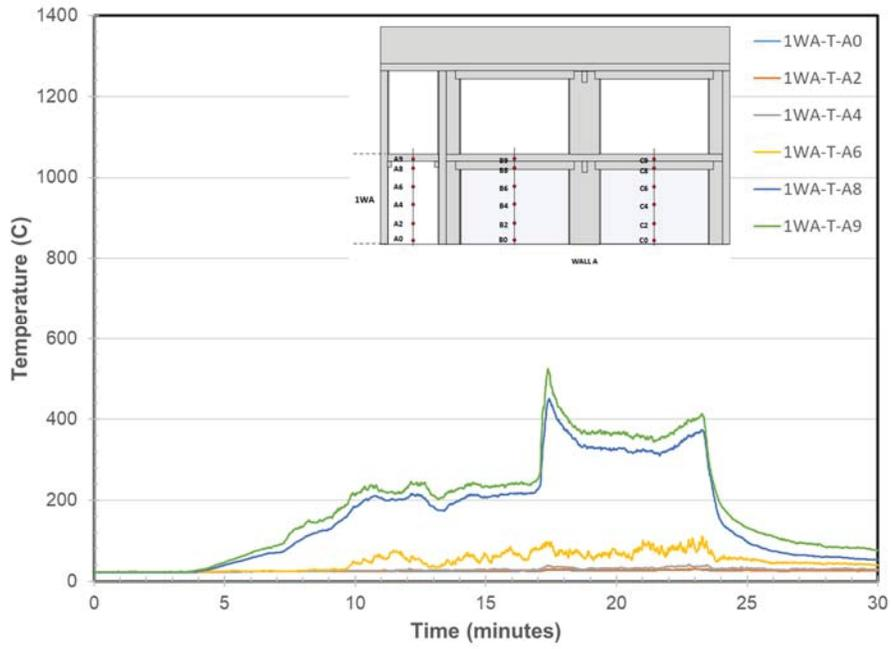
**Figure 17. Wall A Temperatures at Location A**
