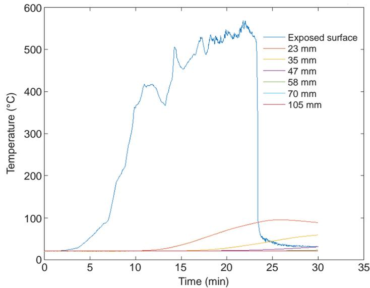
**Figure 108. Embedded thermocouple temperatures in living room wall at Location B for Test 5.**
