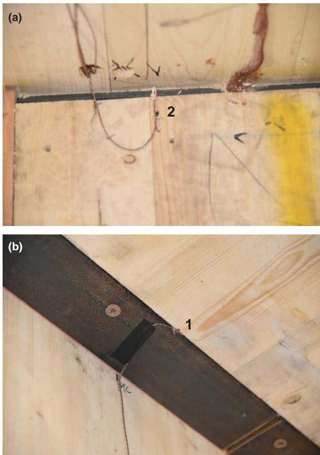
**Figure 72. Thermocouples placed between the steel angle and the cross-laminated timber floor assembly to measure the joint temperatures: (a) top view; (b) bottom view (numbers correspond to locations shown in Fig. 71).**
