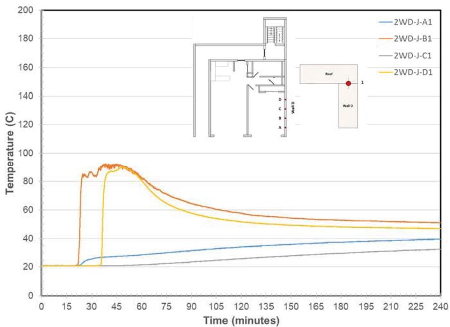
Figure 31. Ceiling/Wall B Joint Temperatures at Locations A-D
