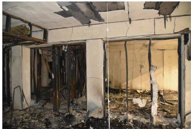
**Figure 58. Interior view of apartment after Test 1.**
