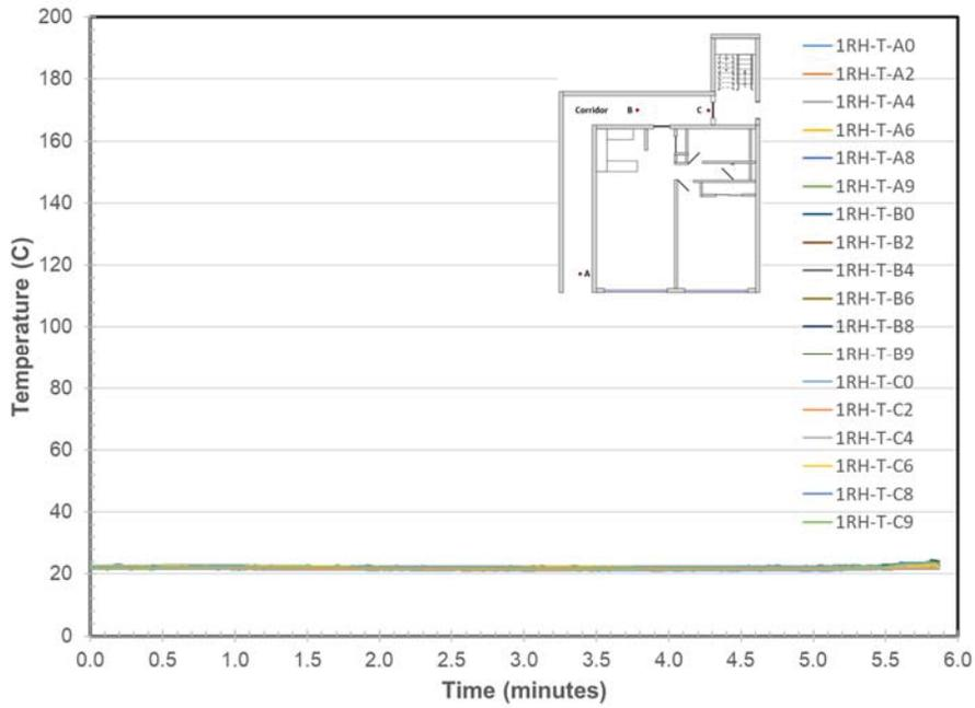
Figure 244. Corridor Temperatures at Locations A, B, & C
