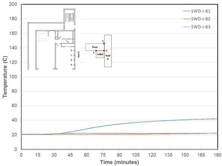
**Figure 948. Wall D/Ledger Joint Temperatures at Location B**
