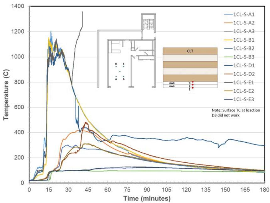
Figure 930. Living Room Ceiling Surface Temperatures at Location A, B, D, & E
