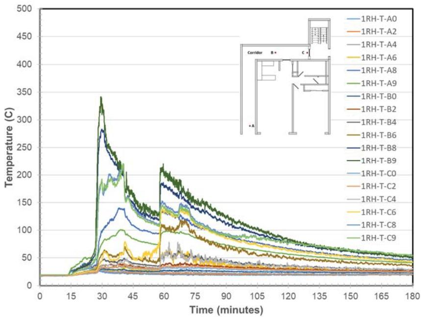
Figure 936. Corridor Temperatures at Locations A, B, & C
