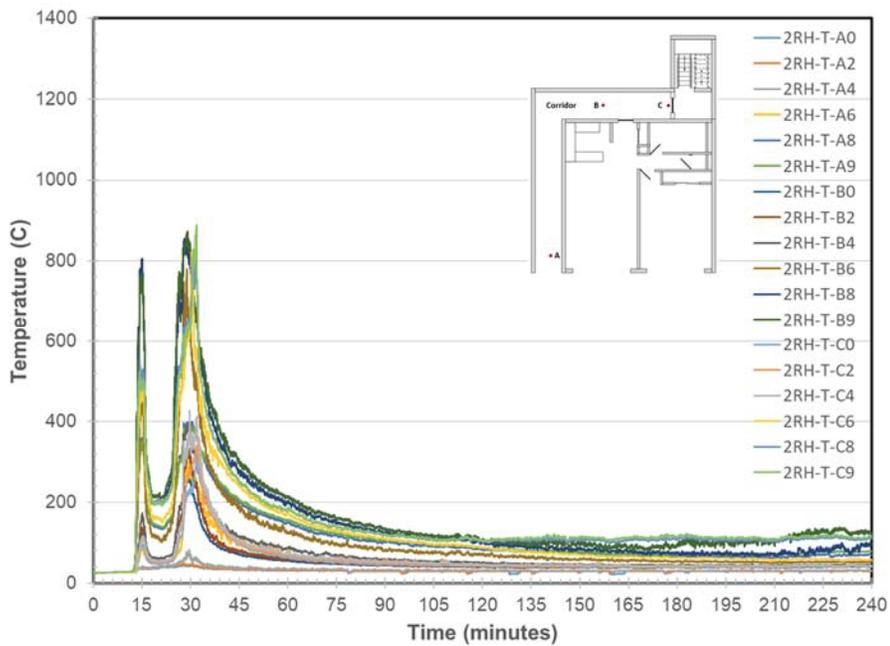
Figure 220. Corridor Temperatures at Locations A, B, & C
