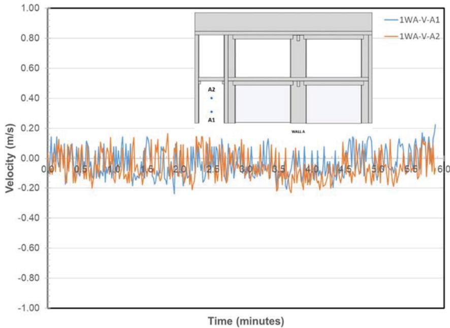
**Figure 263. Velocity at Location A on Wall A**
