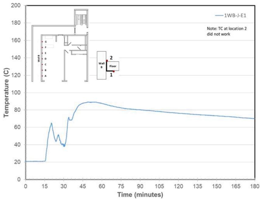
Figure 944. Wall B/Steel Angle Joint Temperatures at Location E
