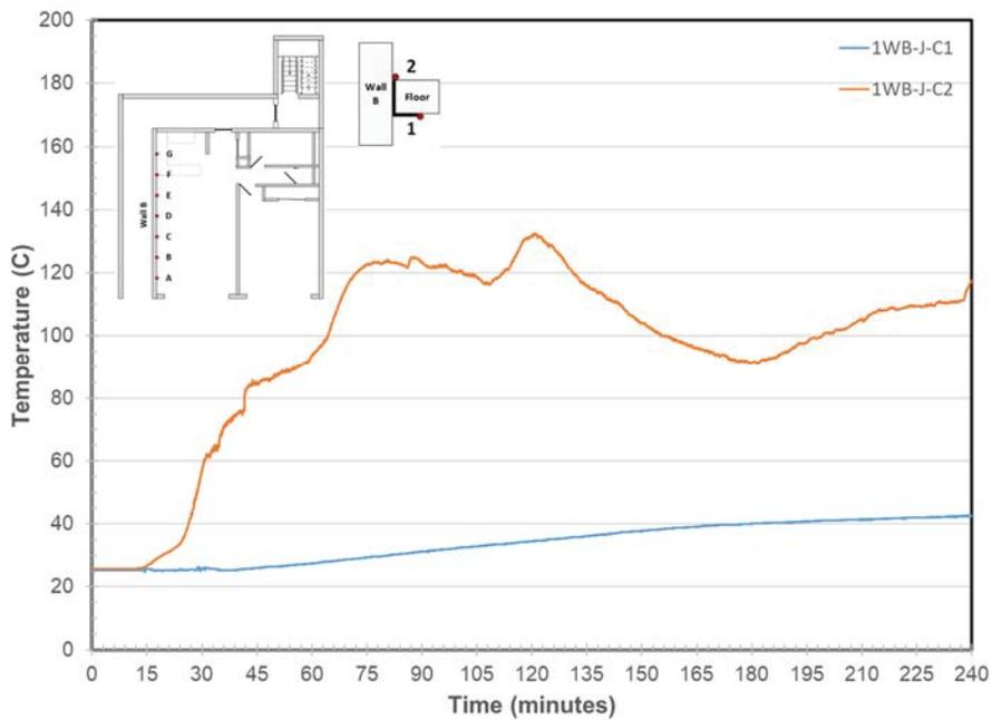
Figure 226. Wall B/Steel Angle Joint Temperatures at Location C
