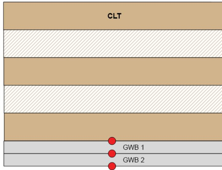
Figure 68. Additional surface thermocouples when the cross-laminated timber (CLT) was encapsulated (GWB, gypsum wallboard).
