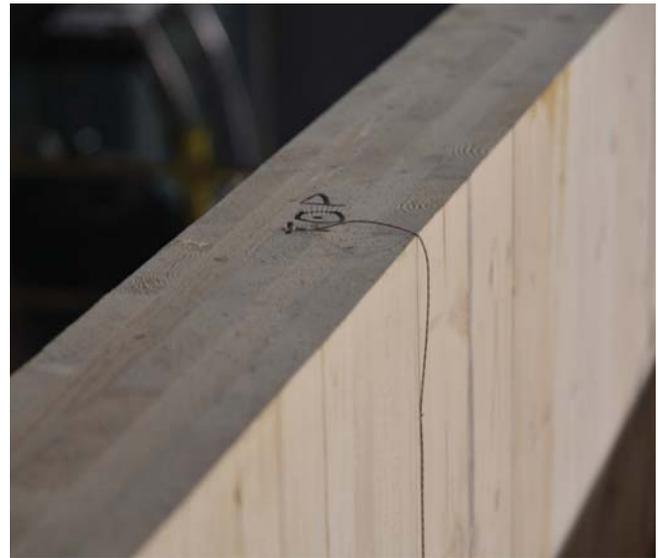
**Figure 76. Thermocouple placed on wall to measure temperature at ceiling–wall joint interface on the second floor.**
