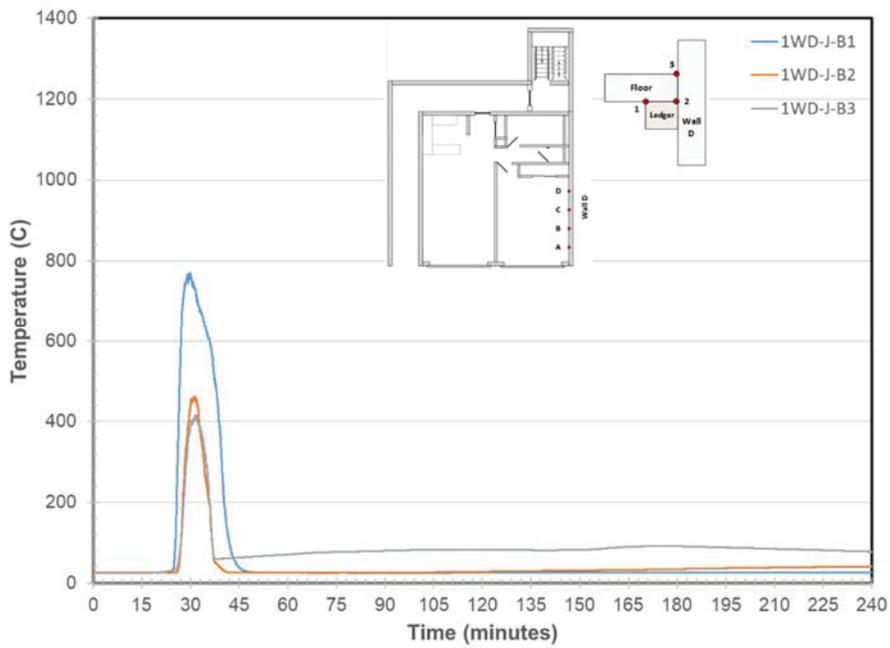
Figure 232. Wall D/Ledger Joint Temperatures at Location B
