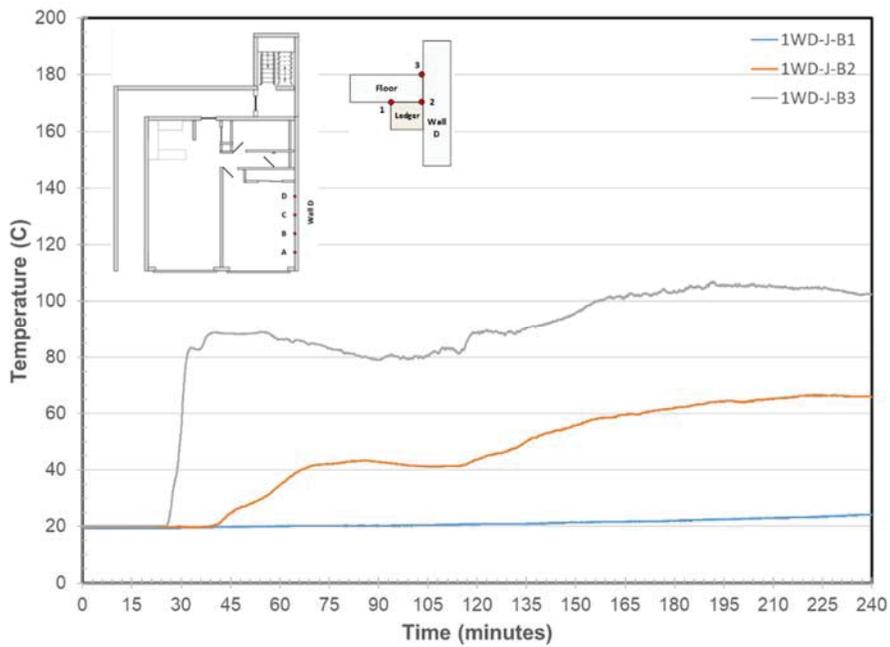
Figure 27. Wall D/Ledger Joint Temperatures at Location B
