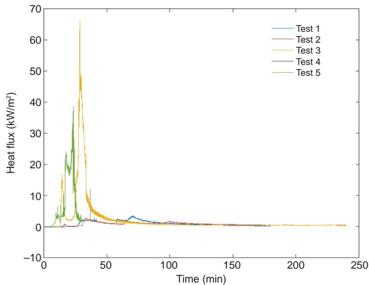
**Figure 109. Heat flux in Wall F across from apartment door for each test.**
