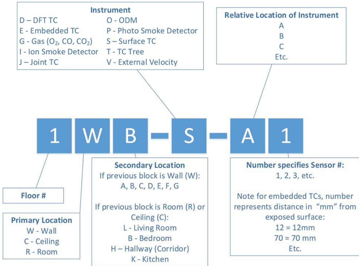
**Figure 1. Nomenclature of Instrumentation Location**
