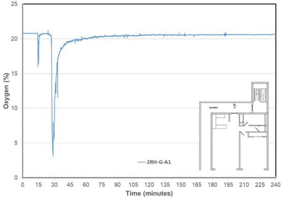
**Figure 247. Oxygen Concentration in the Corridor**
