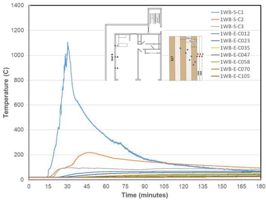
Figure 925. Wall B Embedded & Surface Temperatures at Location C
