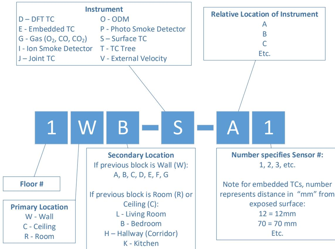
**Figure 1. Nomenclature of Instrumentation Location**
