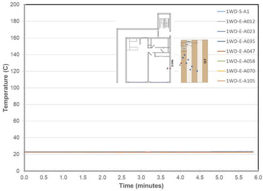
Figure 234. Wall D Embedded & Surface Temperatures at Location A
