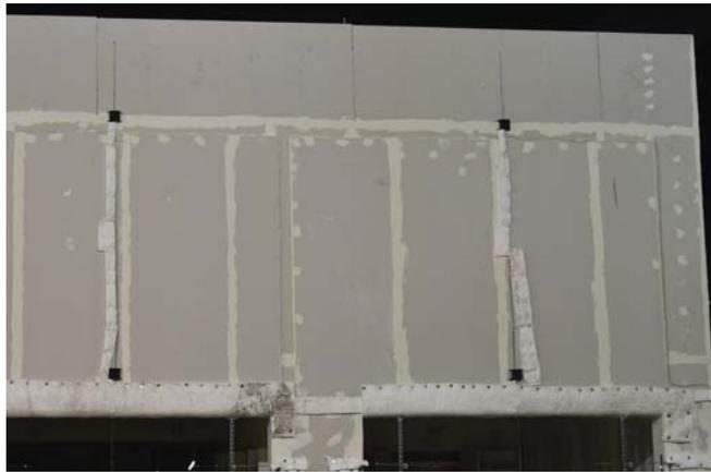
Figure 88. Directional flame thermometers mounted on the exterior of Wall A.
