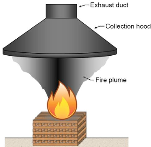
**Figure 95. Schematic of a fire product collector.**
