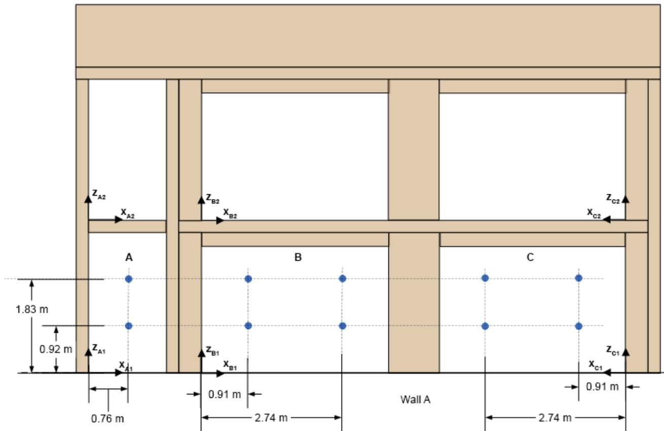
Figure 81. Location of bidirectional probes (blue circles).
