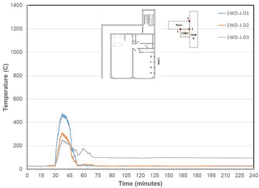
Figure 234. Wall D/Ledger Joint Temperatures at Location D
