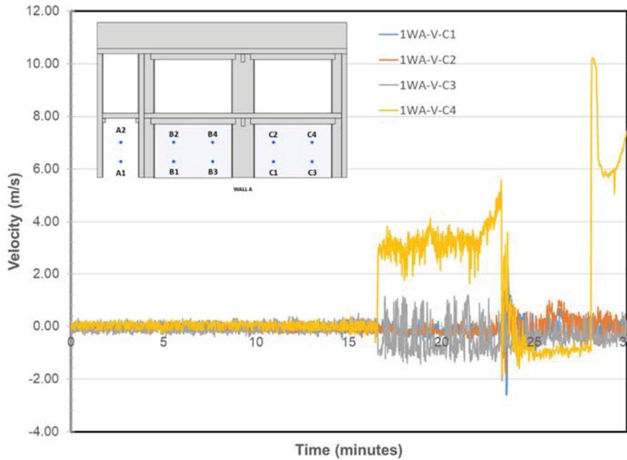
Figure 36. Velocity at Location C on Wall A
