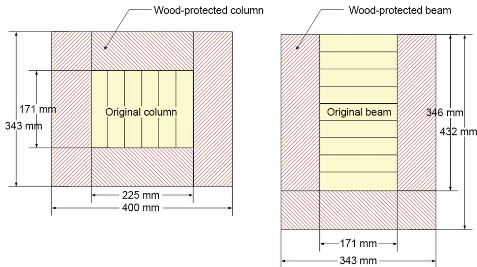
Figure 15. Cross-sectional view of a support column and midspan beam illustrating the wood protection added to achieve a 2-h fire resistance rating.
