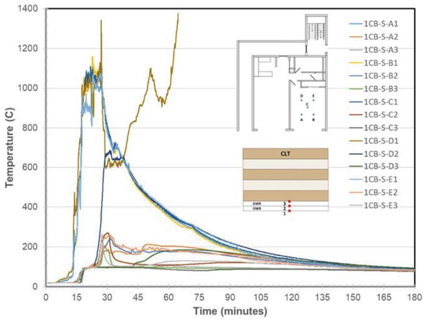
Figure 933. Bedroom Ceiling Surface Temperatures at Locations A through E
