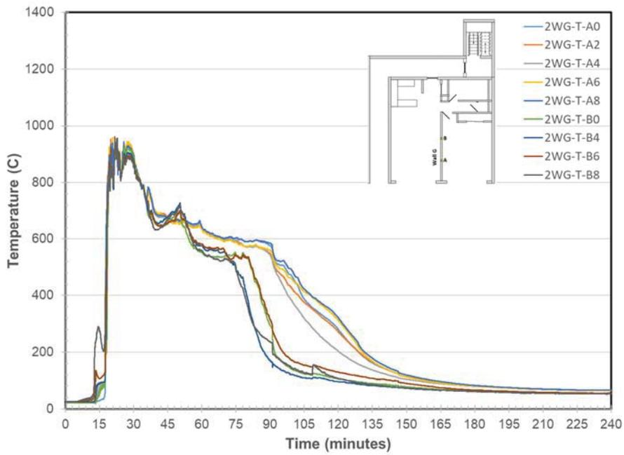
Figure 219. Wall G Temperatures at Locations A & B
