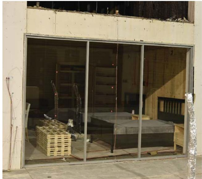
Figure 27. Window installed in Wall A for Tests 4 and 5.
