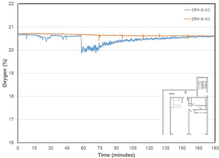
**Figure 964. Oxygen Concentration in the Corridor on each Floor**
