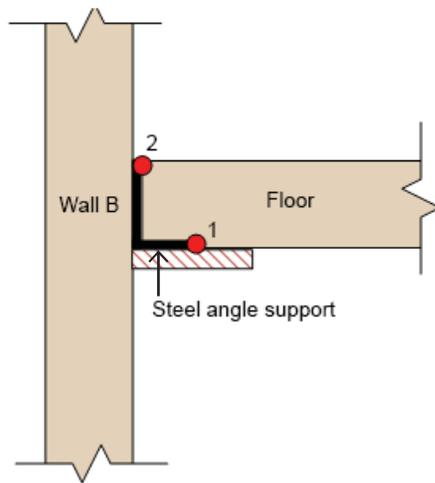
**Figure 71. Joint temperature measurement at the steel angle–floor interface.**
