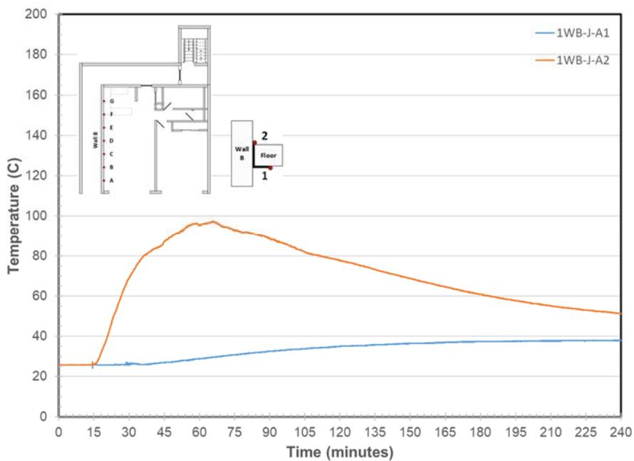
Figure 224. Wall B/Steel Angle Joint Temperatures at Location A
