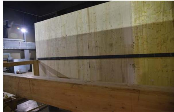
Figure 7. Steel angle located on Wall B to support the second-level floor in the apartment.
