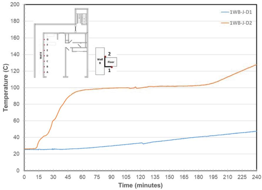
Figure 227. Wall B/Steel Angle Joint Temperatures at Location D
