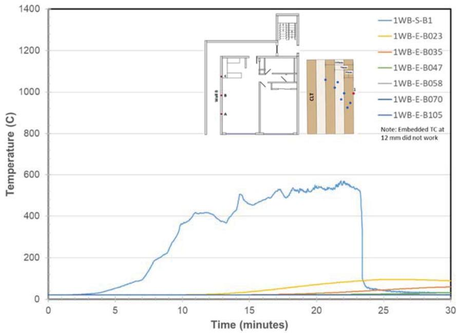
Figure 3. Wall B Embedded & Surface Temperatures at Location B
