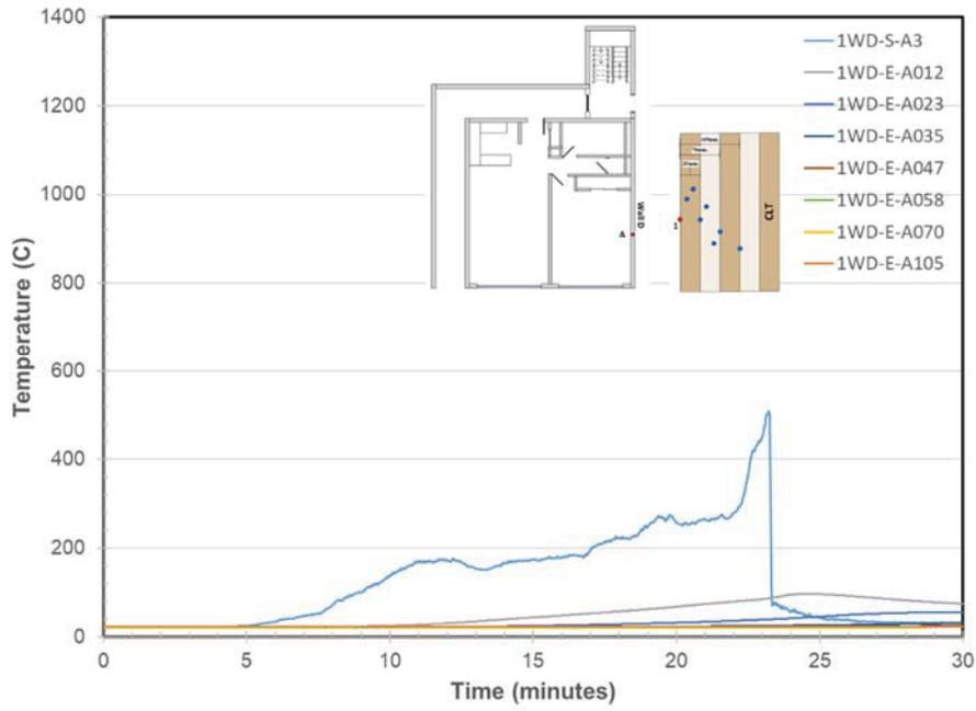
Figure 5. Wall D Embedded & Surface Temperatures at Location A
