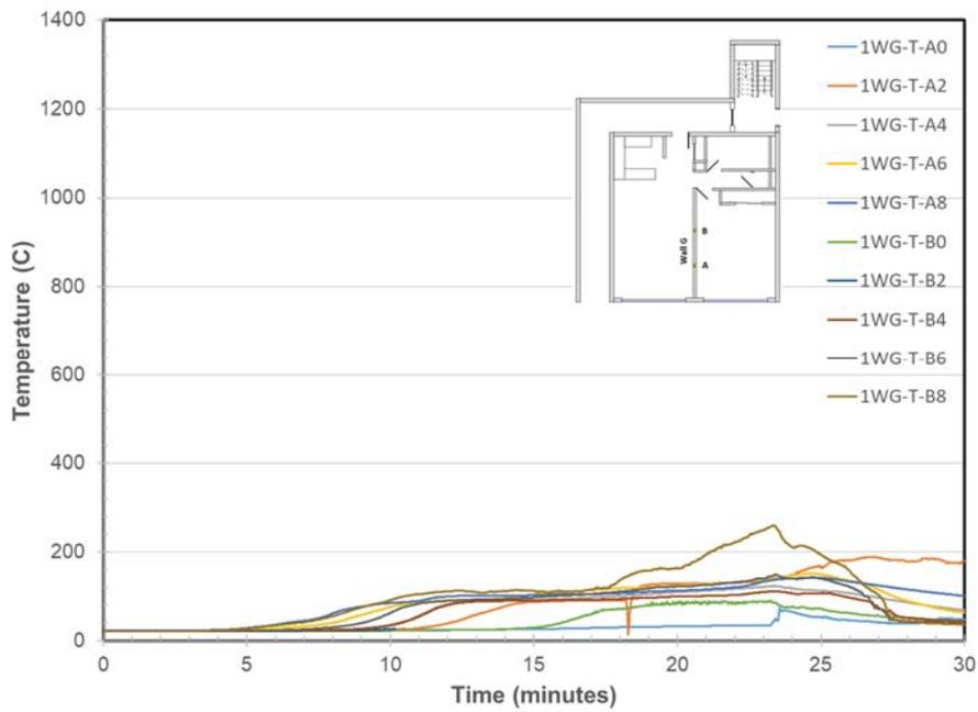
**Figure 14. Wall G Temperatures at Locations A & B**
