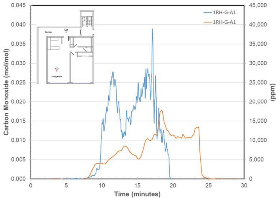
**Figure 44. Carbon Monoxide Concentrations in the Corridor and Living Room**
