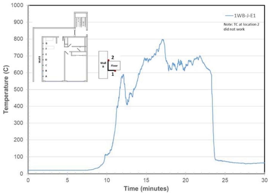
Figure 24. Wall B/Steel Angle Joint Temperatures at Location E
