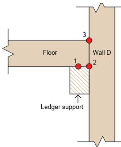
**Figure 73. Ledger–floor joint temperature measurement locations.**
