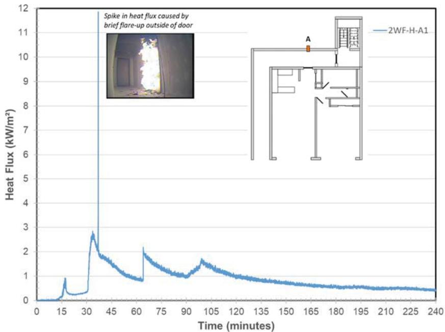
Figure 37. Heat Flux on Wall F across from Apartment Door
