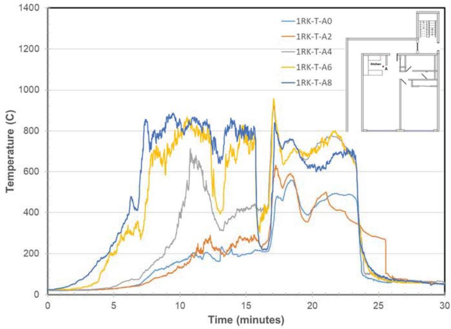
**Figure 13. Kitchen Temperatures at Location A**
