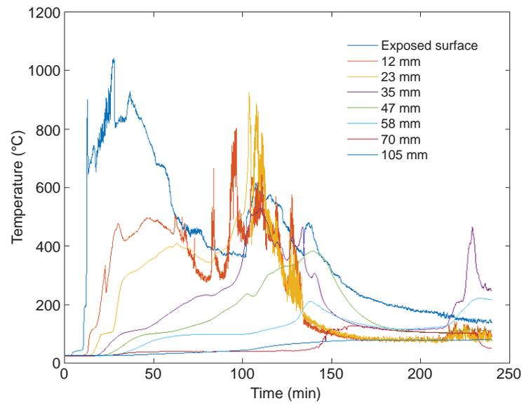
**Figure 106. Embedded thermocouple temperatures in living room wall at location B for Test 3.**
