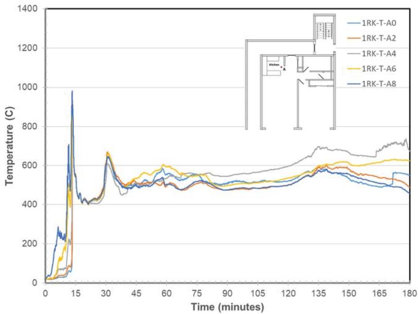
Figure 934. Kitchen Temperatures at Location A
