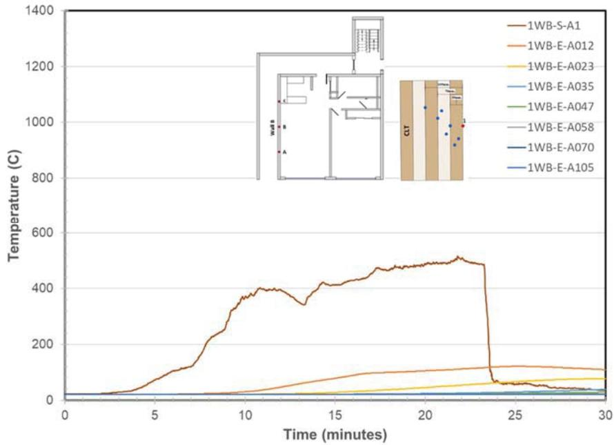
**Figure 2. Wall B Embedded & Surface Temperatures at Location A**
