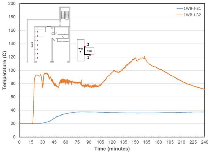
Figure 20. Wall B/Steel Angle Joint Temperatures at Location B
