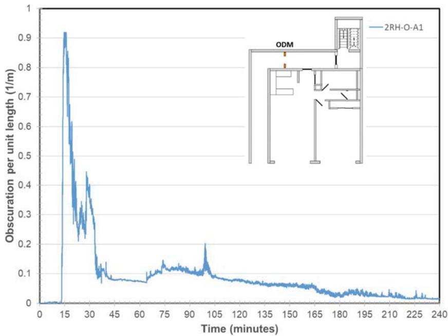
**Figure 39. Obscuration per unit Length in Corridor**
