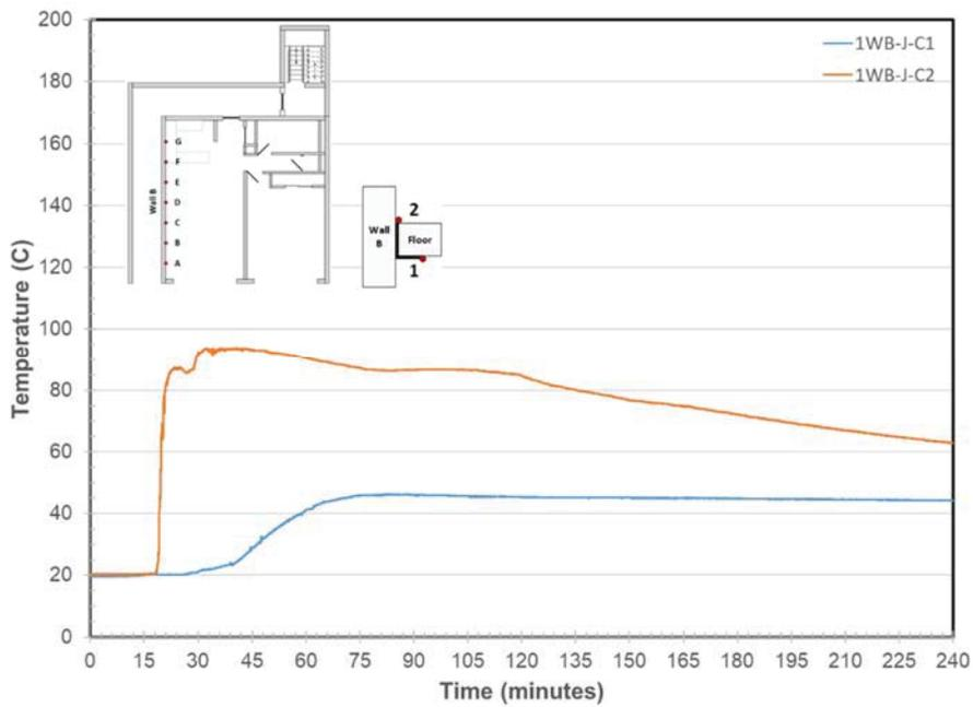
Figure 21. Wall B/Steel Angle Joint Temperatures at Location C
