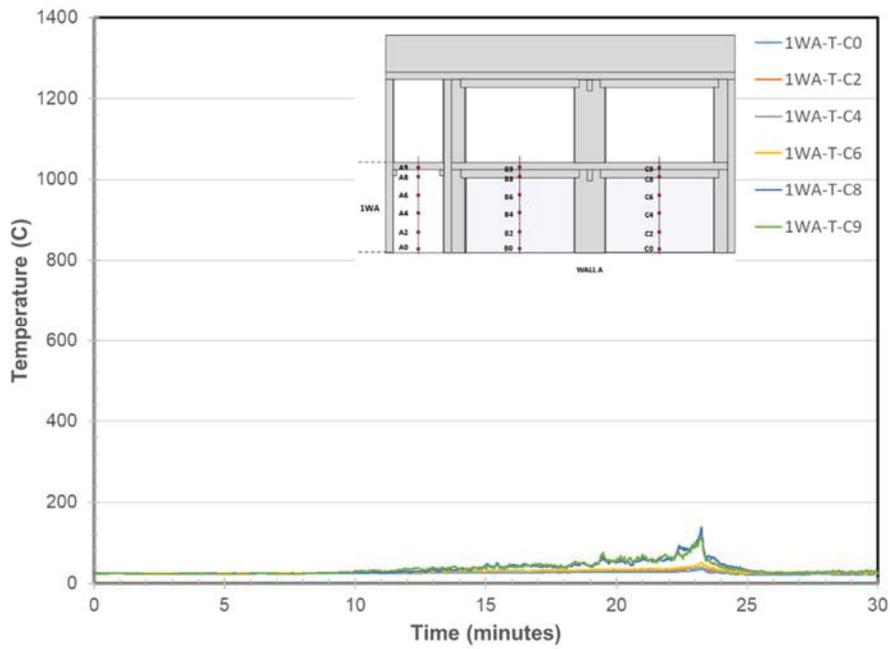
Figure 19. Wall A Temperatures at Locations C
