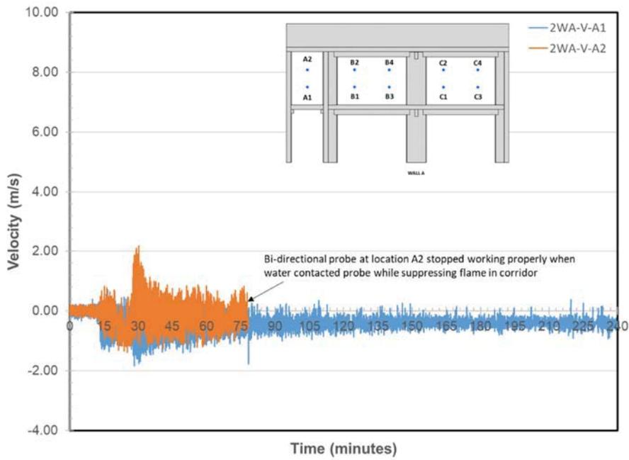
**Figure 238. Velocity at Location A on Wall A**
