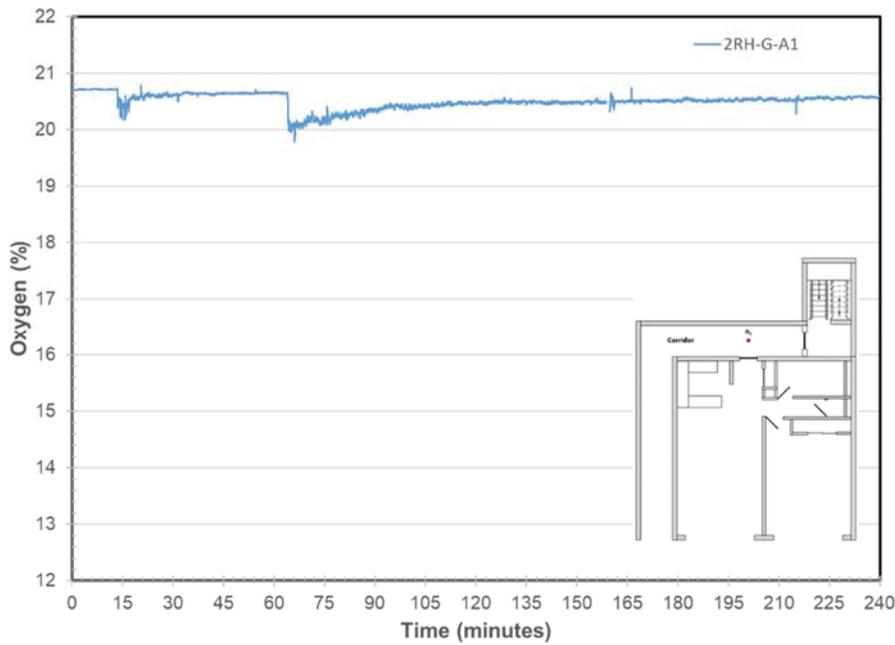
**Figure 42. Oxygen Concentration in the Corridor**
