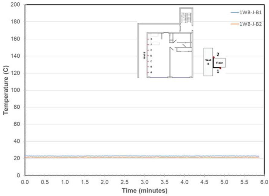
Figure 250. Wall B/Steel Angle Joint Temperatures at Location B
