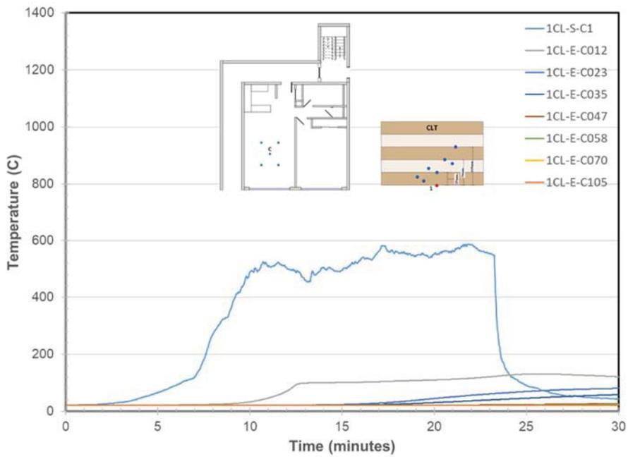
Figure 6. Living Room Ceiling Embedded & Surface Temperatures at Location C
