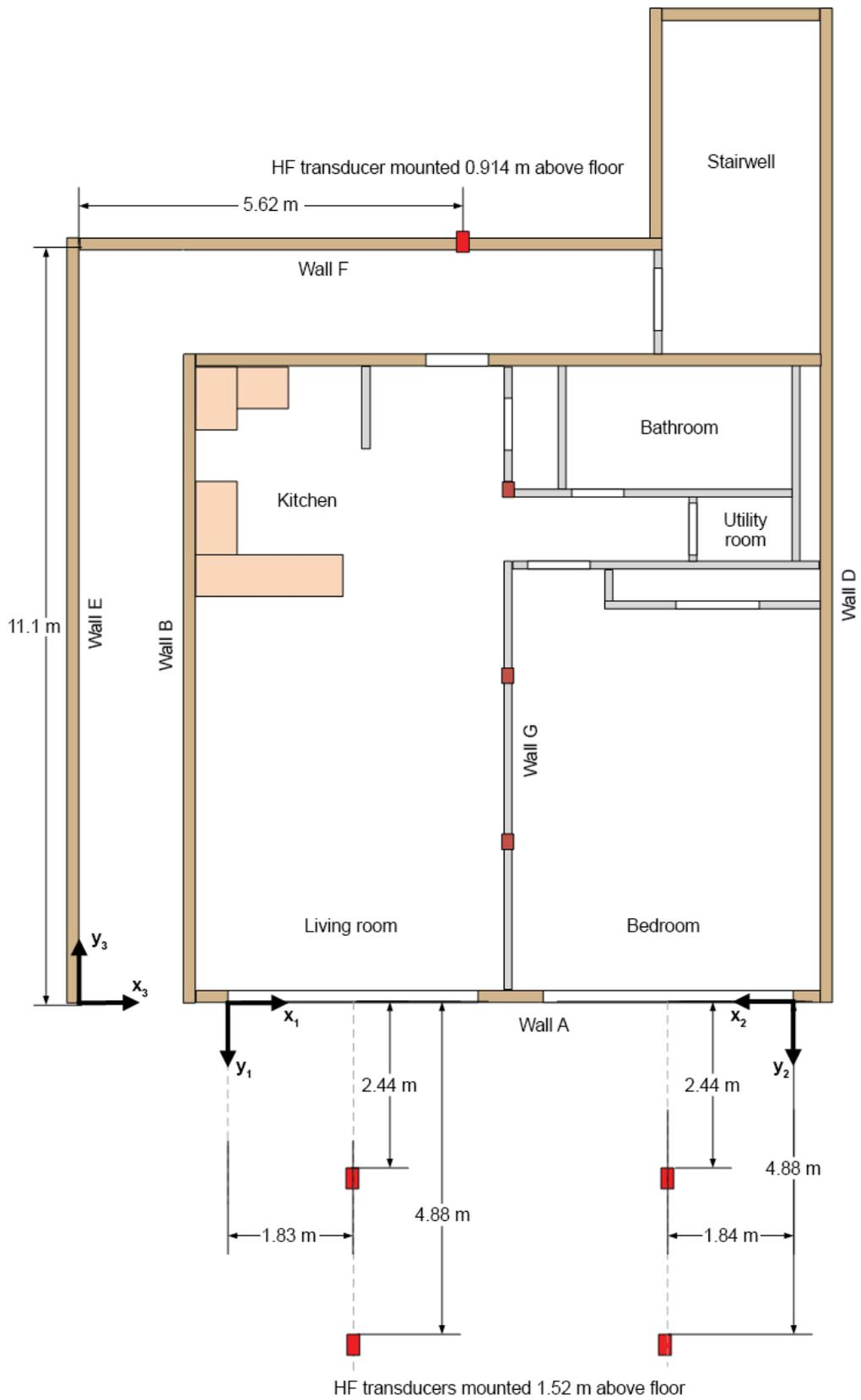
Figure 83. Location of heat flux (HF) transducers (red rectangles).
