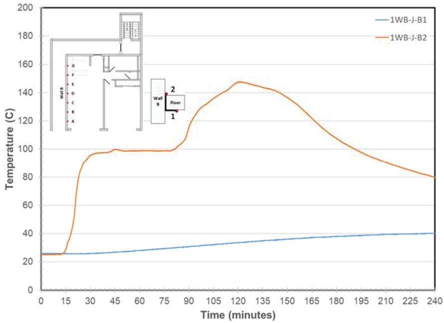
Figure 225. Wall B/Steel Angle Joint Temperatures at Location B
