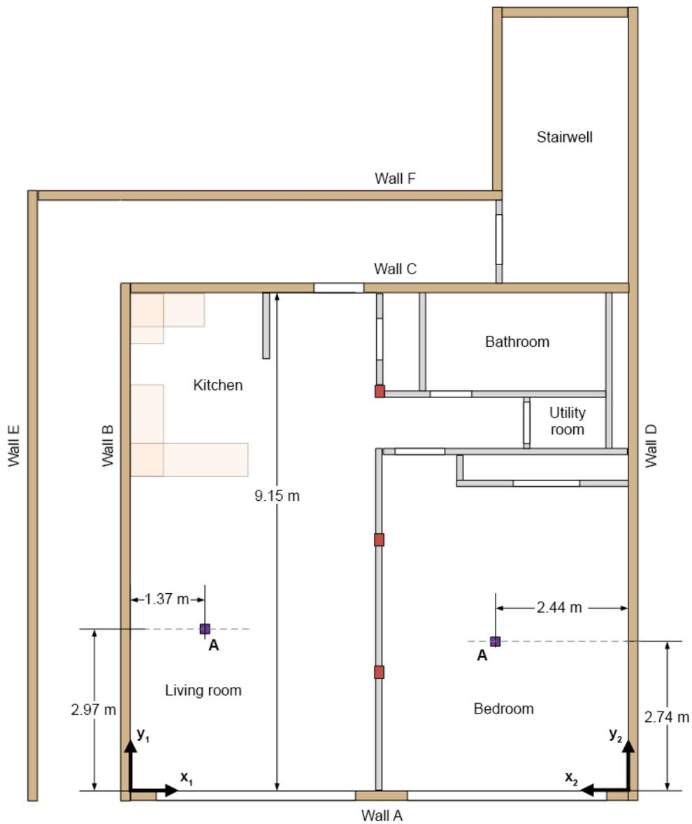
Figure 87. Location of directional flame thermometers on ceilings (purple squares).
