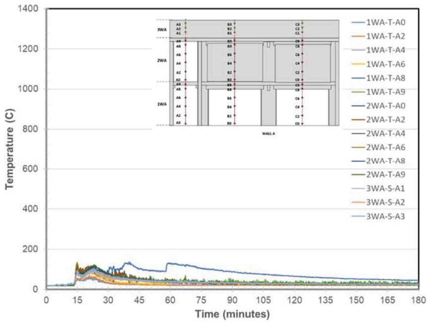
Figure 937. Wall A Temperatures at Location A
