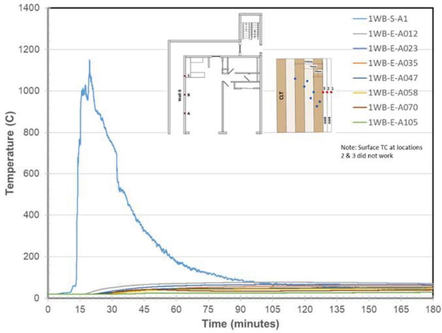
Figure 923. Wall B Embedded & Surface Temperatures at Location A
