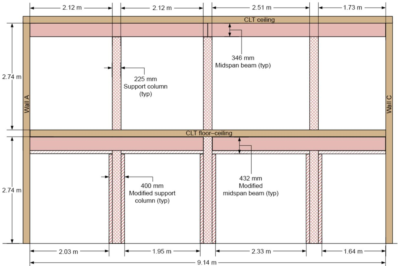
Figure 14. Cross-sectional view of apartment showing locations of support columns.
