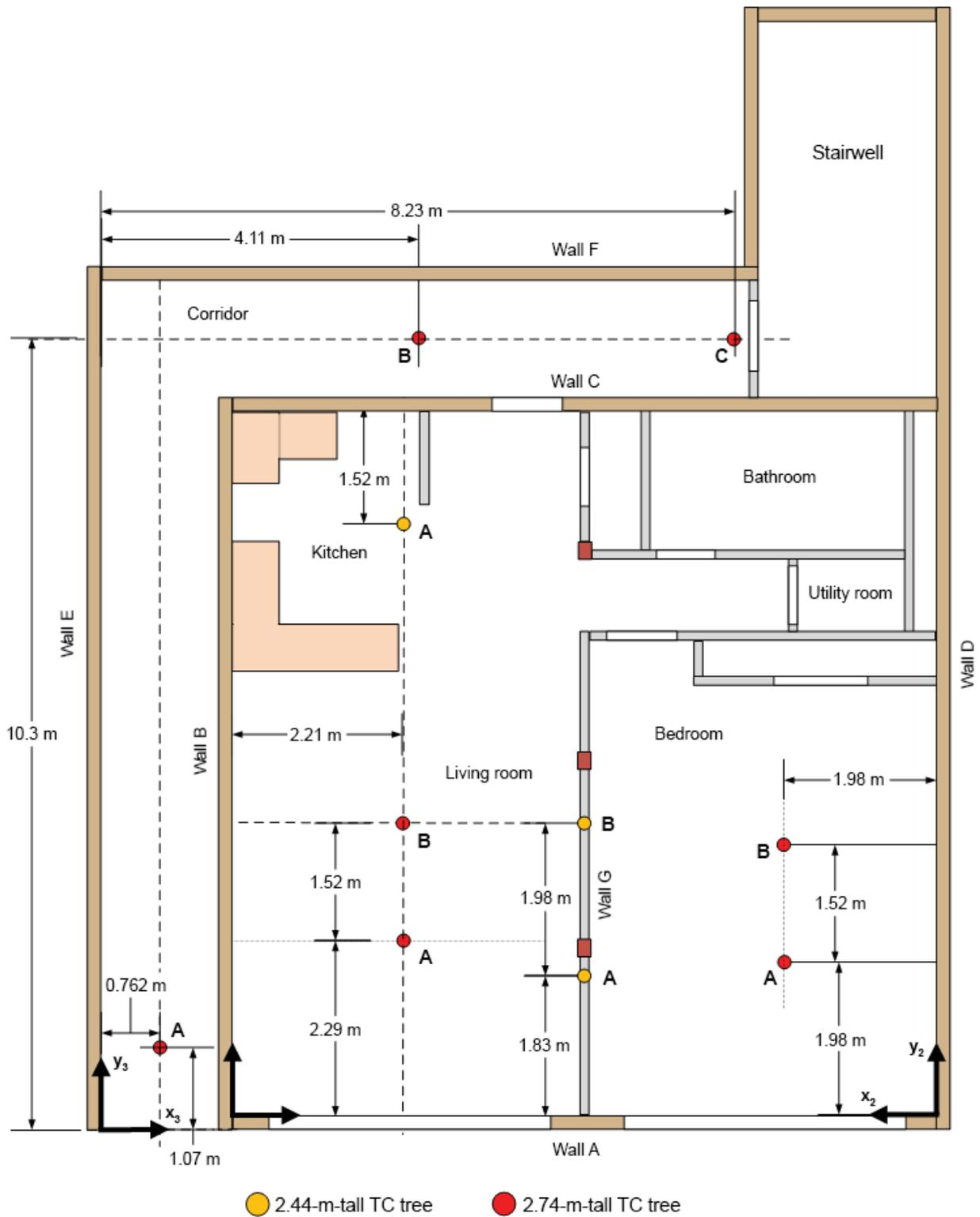
Figure 66. Location of thermocouple (TC) trees.
