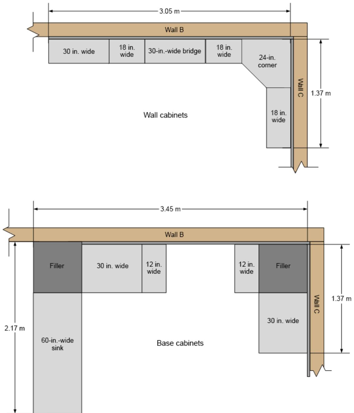
Figure 45. Plan view of wall cabinets and base cabinets in kitchen.
