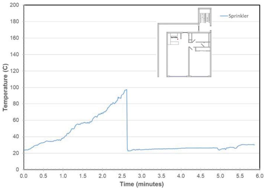
Figure 245. Sprinkler Head Temperature in Kitchen
