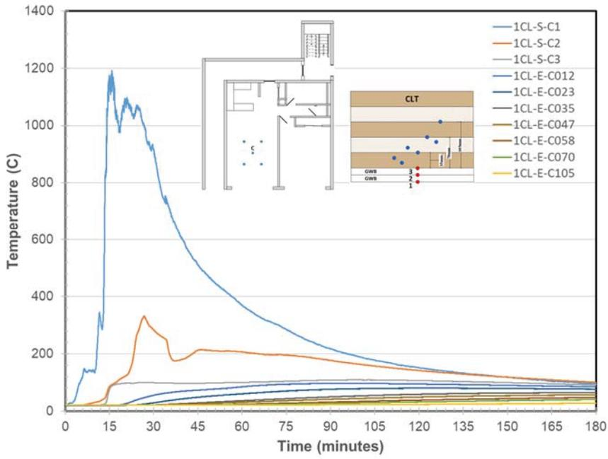
Figure 927. Living Room Ceiling Embedded & Surface Temperatures at Location C
