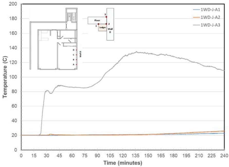
Figure 26. Wall D/Ledger Joint Temperatures at Location A
