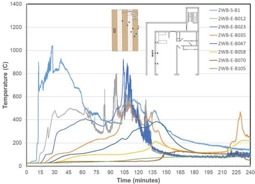
**Figure 208. Wall B Embedded & Surface Temperatures at Location B**
