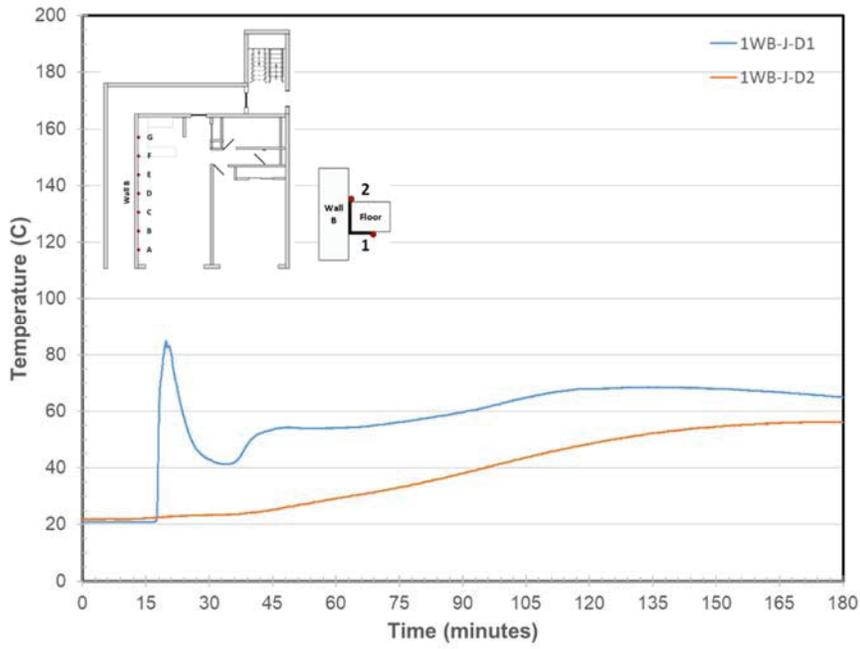
Figure 943. Wall B/Steel Angle Joint Temperatures at Location D
