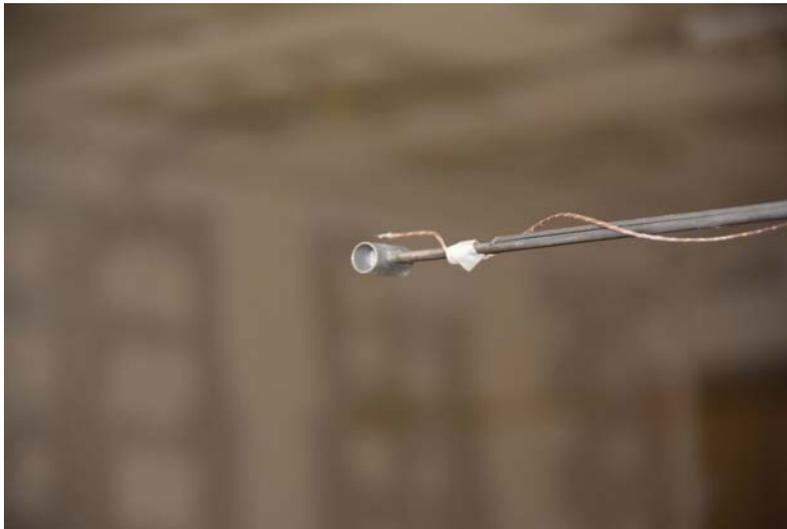
Figure 80. Bidirectional probe.
