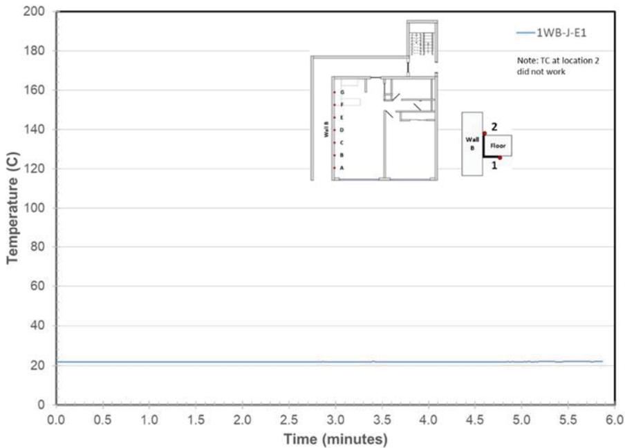
Figure 253. Wall B/Steel Angle Joint Temperatures at Location E
