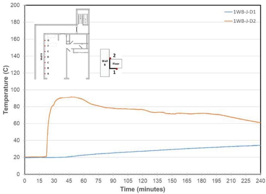
Figure 22. Wall B/Steel Angle Joint Temperatures at Location D
