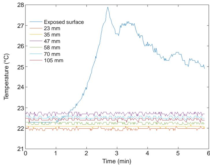
**Figure 107. Embedded thermocouple temperatures in living room wall at Location B for Test 4.**
