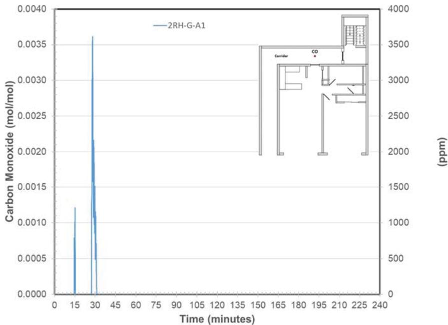
**Figure 248. Carbon Monoxide Concentration in the Corridor**
