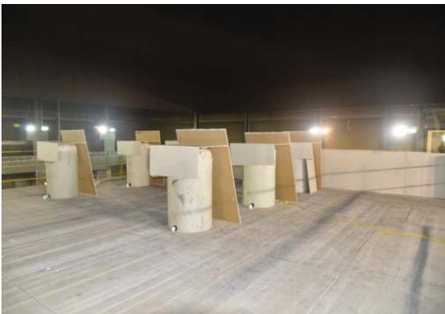
Figure 54. Water tanks on top of the second-level ceiling panels for Tests 2 and 3.
