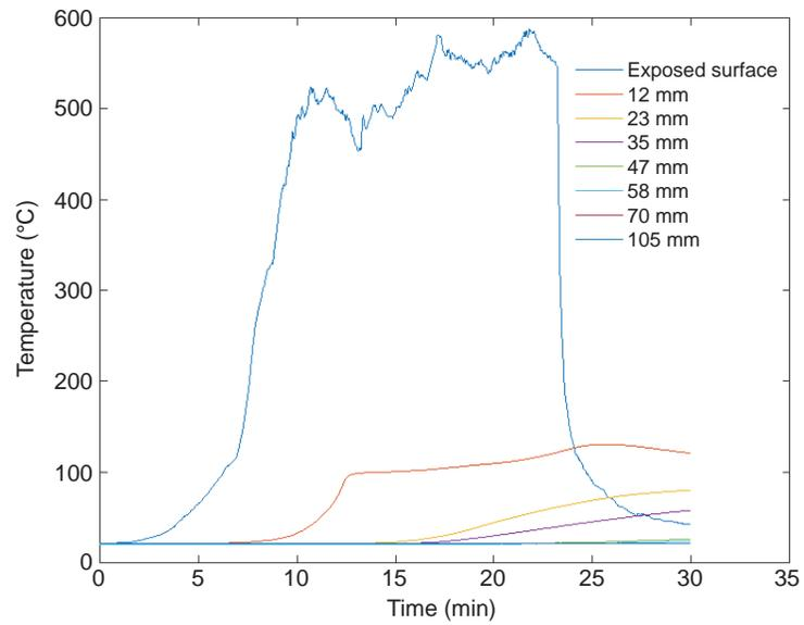
**Figure 105. Embedded thermocouple temperatures in living room ceiling for Test 5.**
