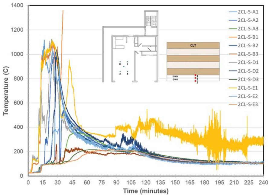
**Figure 214. Living Room Ceiling Surface Temperatures at Location A, B, D, & E**
