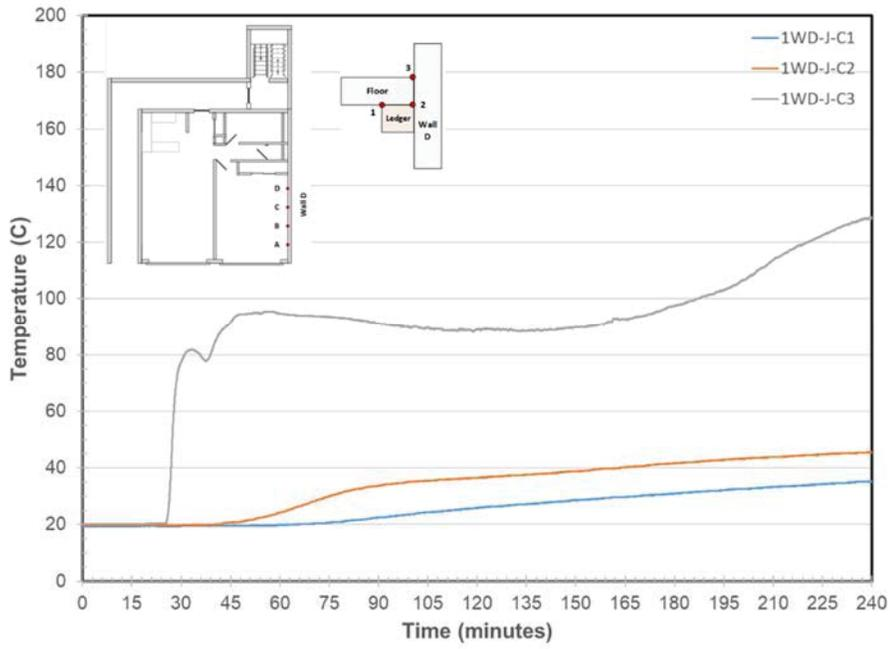
Figure 28. Wall D/Ledger Joint Temperatures at Location C
