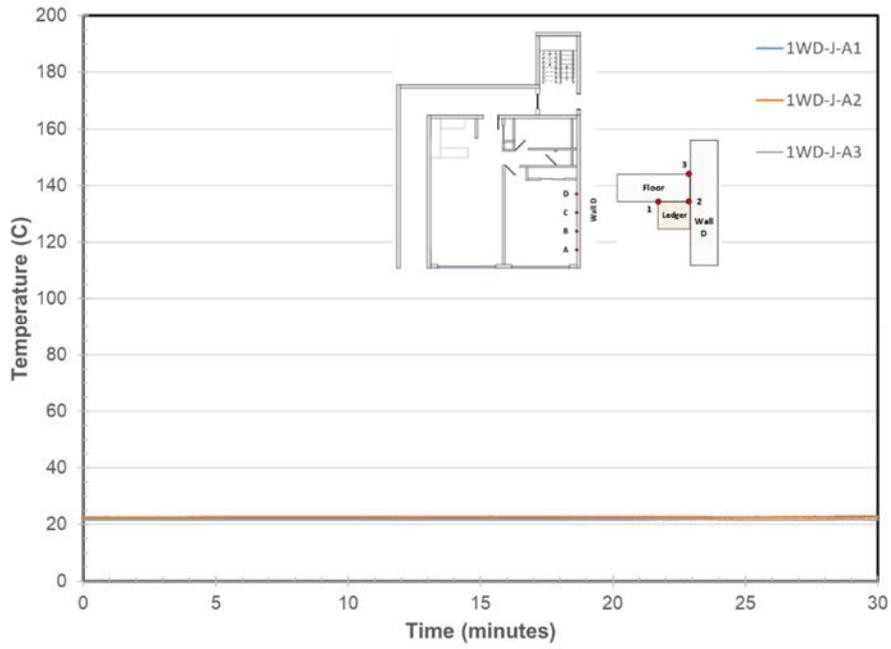
**Figure 27. Wall D/Ledger Joint Temperatures at Location A**
