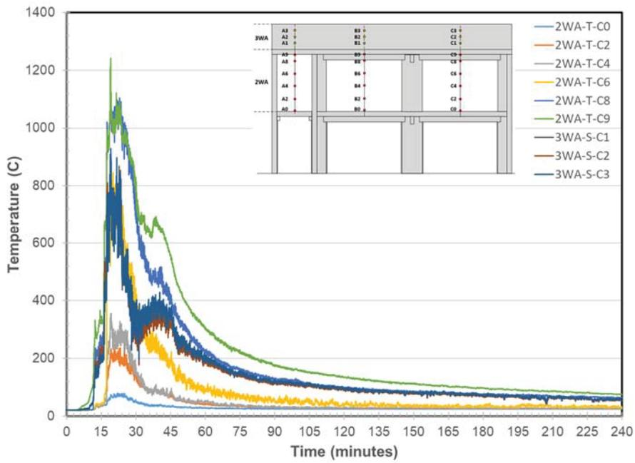
Figure 18. Wall A Temperatures at Locations C
