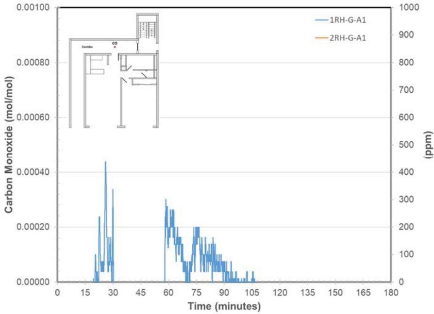
**Figure 965. Carbon Monoxide Concentrations in the Corridor on each Floor**
