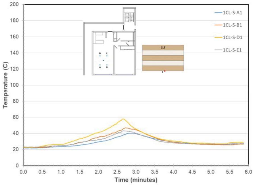
Figure 238. Living Room Ceiling Surface Temperatures at Location A, B, D, & E
