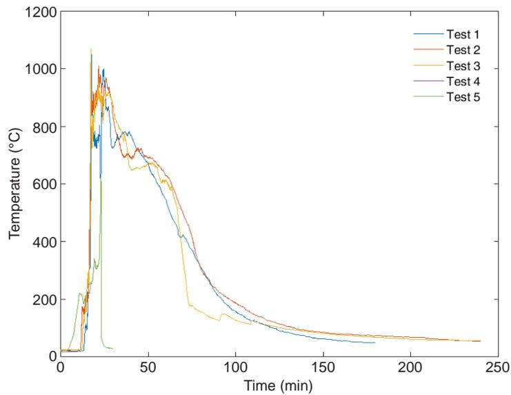
**Figure 101. Bedroom air temperature at 1.83 m above finished floor at location B for each test.**
