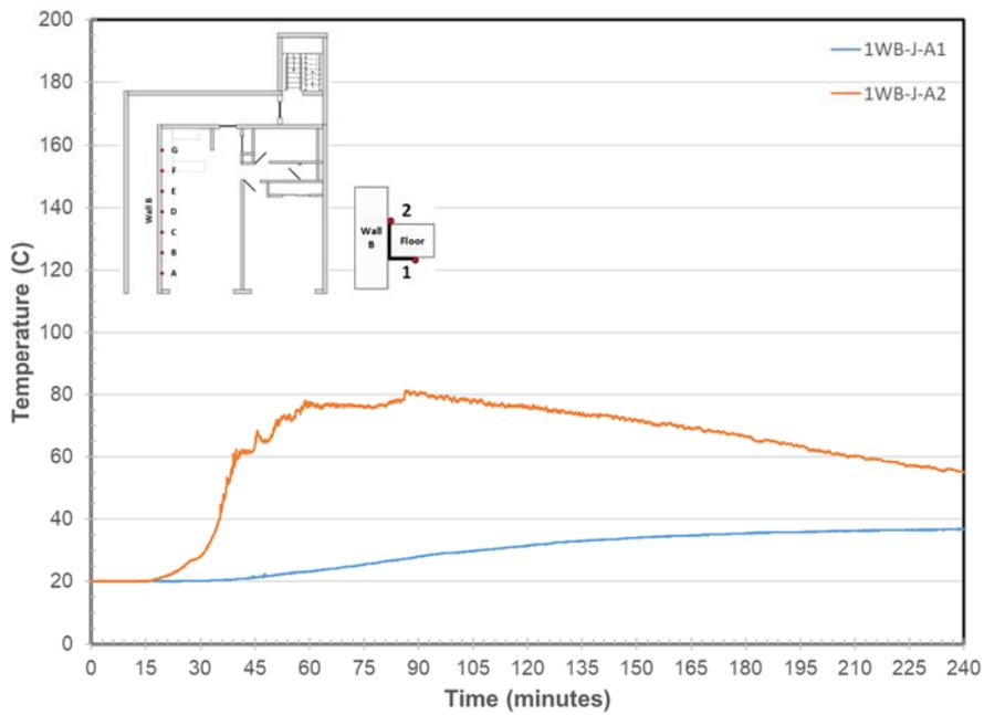
Figure 19. Wall B/Steel Angle Joint Temperatures at Location A
