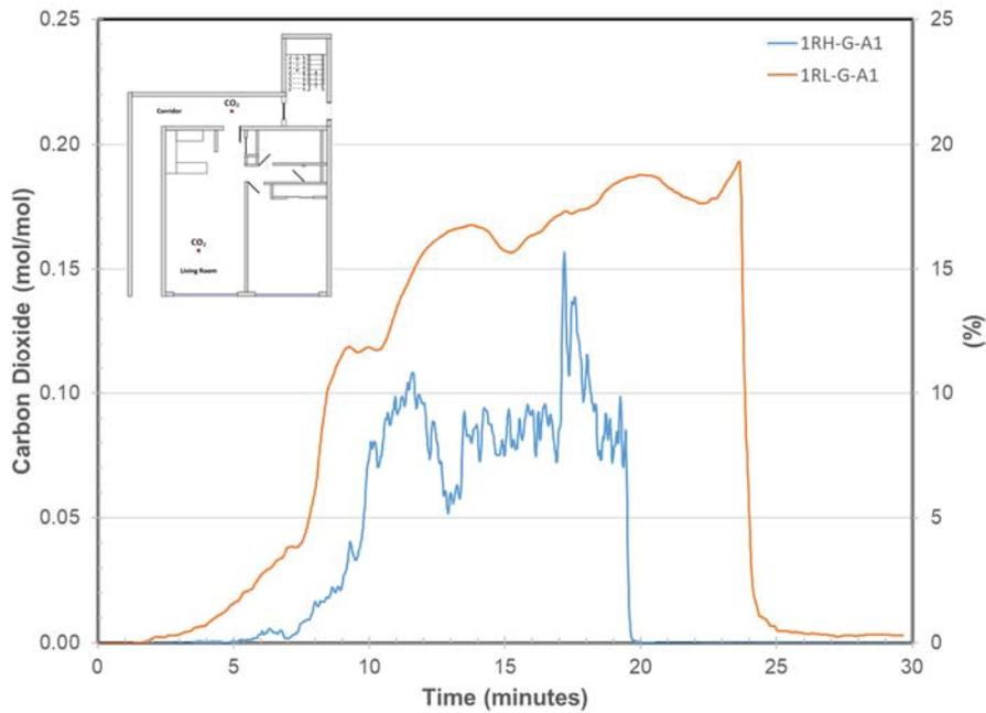
Figure 45. Carbon Dioxide Concentrations in the Corridor and Living Room
