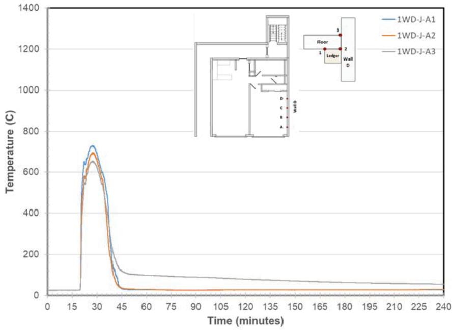
Figure 231. Wall D/Ledger Joint Temperatures at Location A
