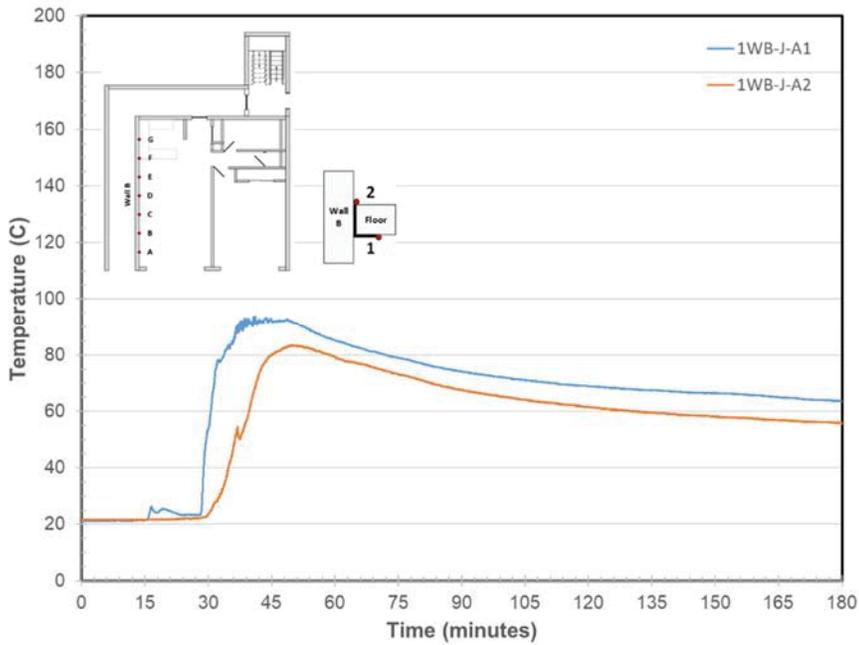
Figure 940. Wall B/Steel Angle Joint Temperatures at Location A
