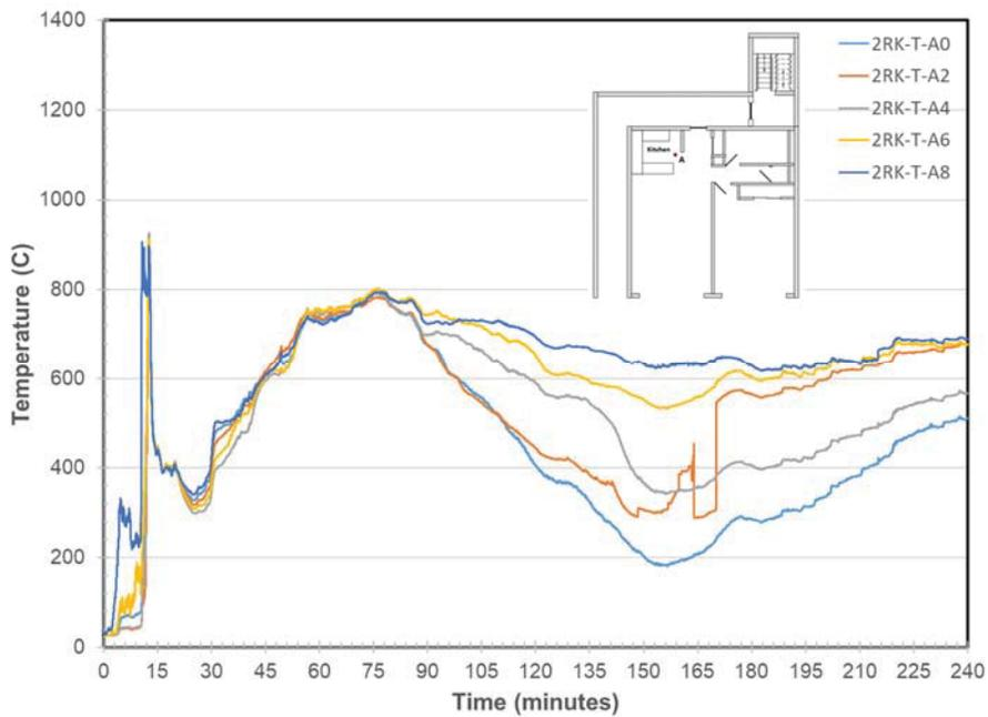
Figure 218. Kitchen Temperatures at Location A
