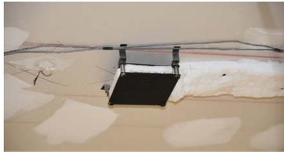
Figure 84. Directional flame thermometer mounted on ceiling.
