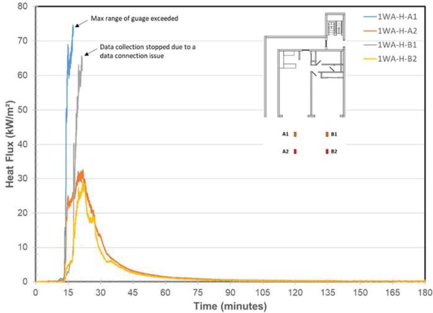
**Figure 958. Heat Flux in Front of Wall A**
