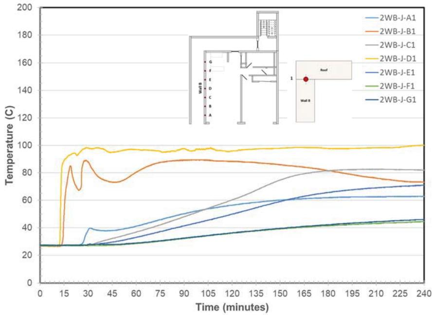
Figure 235. Ceiling/Wall B Joint Temperatures at Locations A-G
