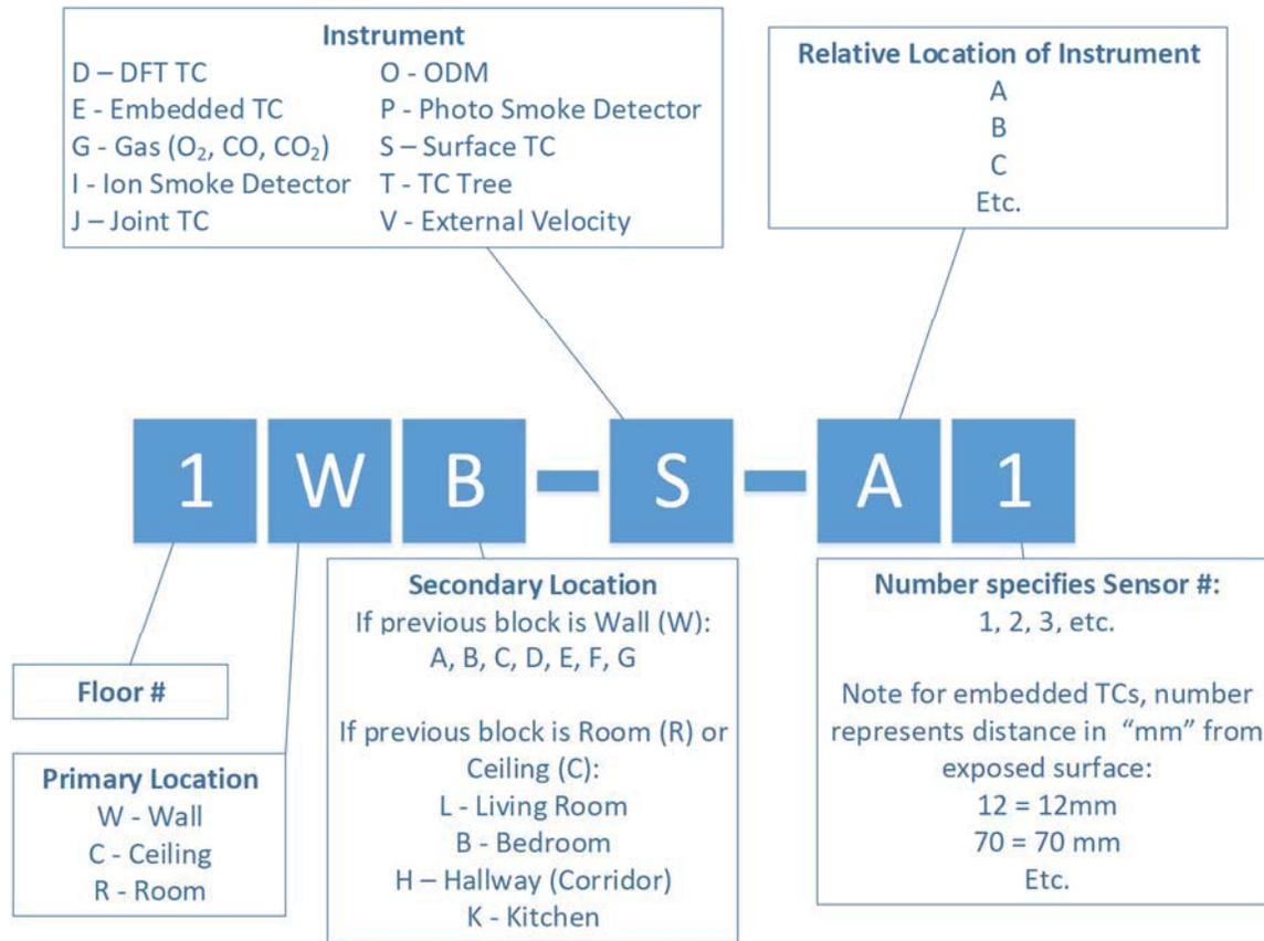
**Figure 1. Nomenclature of Instrumentation Location**
