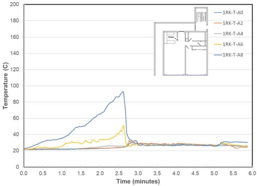
**Figure 242. Kitchen Temperatures at Location A**
