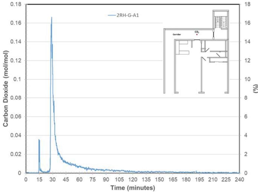
**Figure 249. Carbon Dioxide Concentration in the Corridor**
