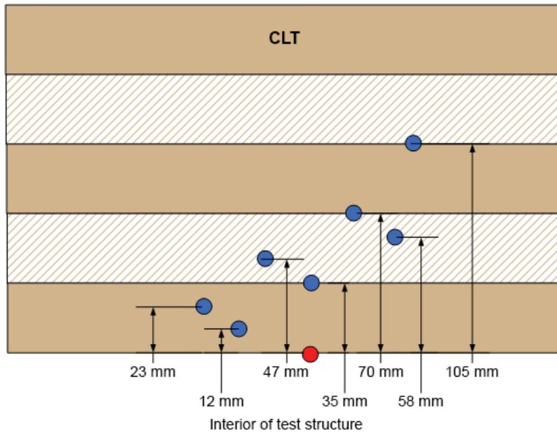
Figure 69. Location of embedded thermocouples in the cross-laminated timber (CLT).
