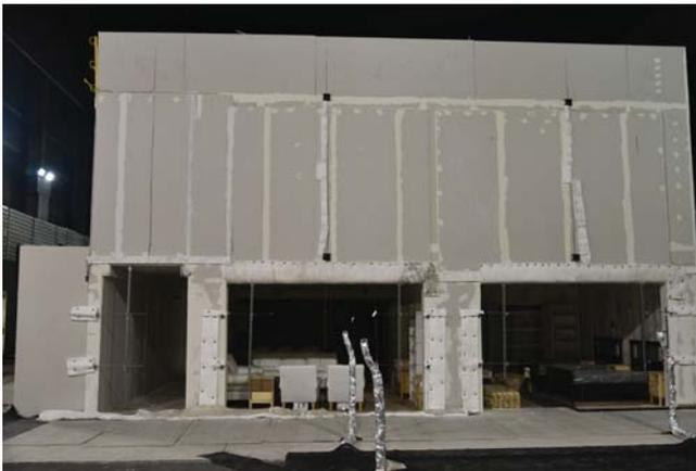
**Figure 52. Second-level openings on Wall A covered with Type X wallboard for Test 1.**
