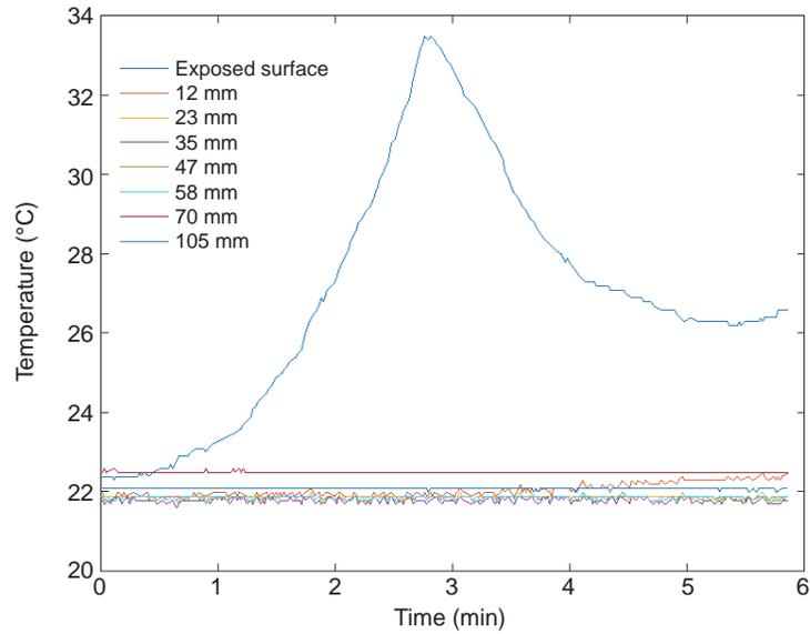
**Figure 104. Embedded thermocouple temperatures in living room ceiling for Test 2.**
