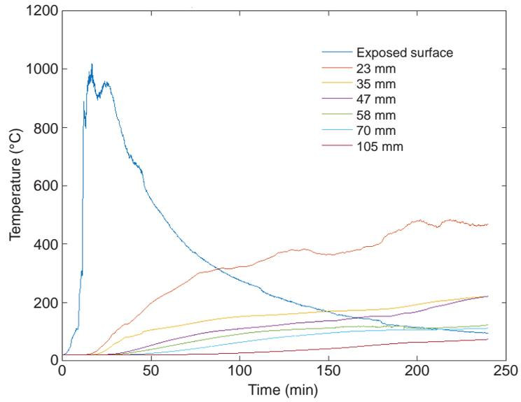
**Figure 103. Embedded thermocouple temperatures in exposed cross-laminated timber portion of living room for Test 2.**
