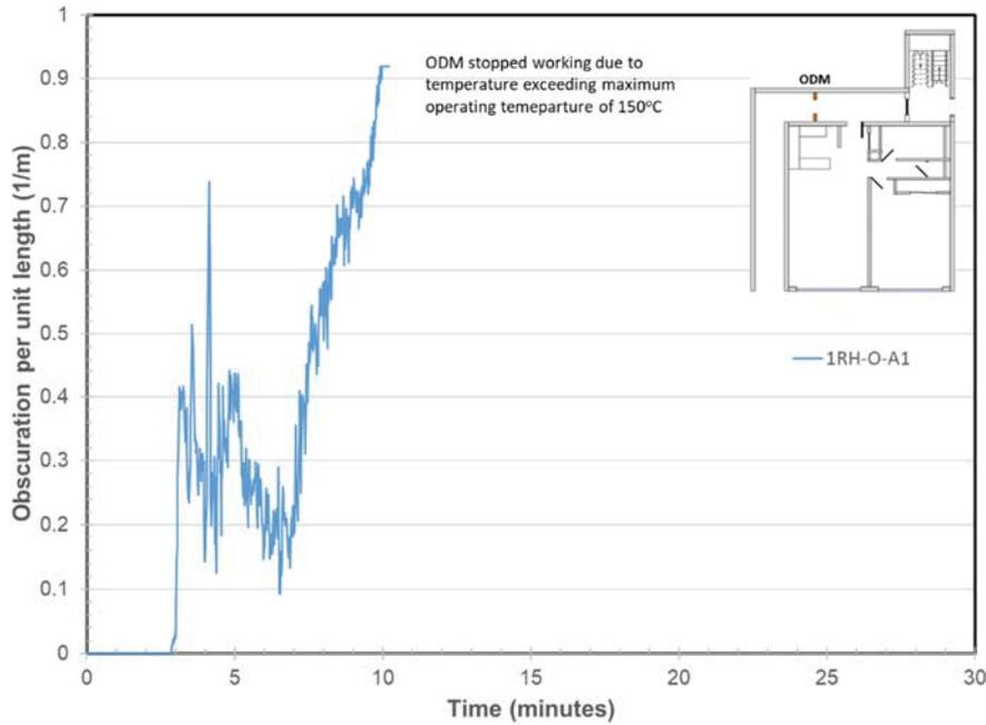
**Figure 40. Obscuration per unit Length in Corridor**
