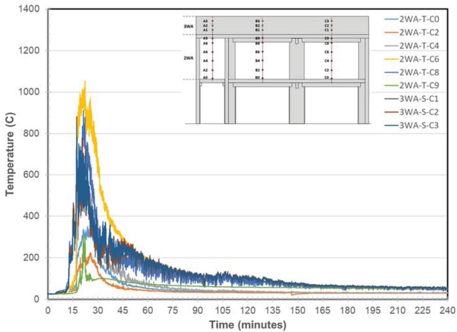
Figure 223. Wall A Temperatures at Locations C
