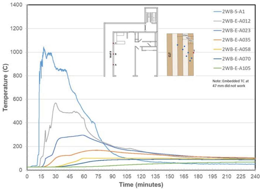
**Figure 207. Wall B Embedded & Surface Temperatures at Location A**
