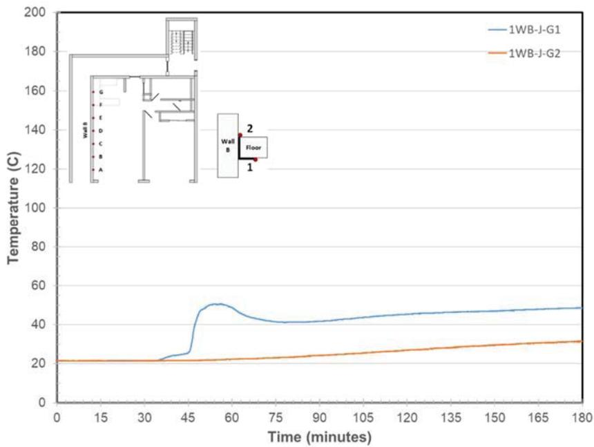
Figure 946. Wall B/Steel Angle Joint Temperatures at Location G
