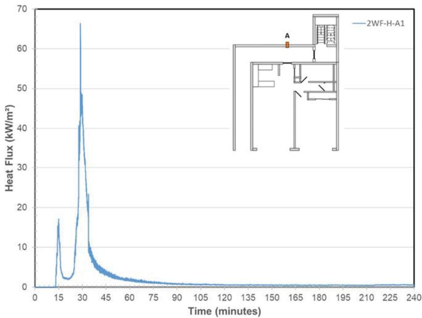
Figure 242. Heat Flux on Wall F across from Apartment Door
