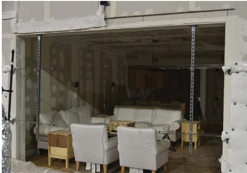
Figure 82. Bidirectional probes mounted at the opening in Wall A.
