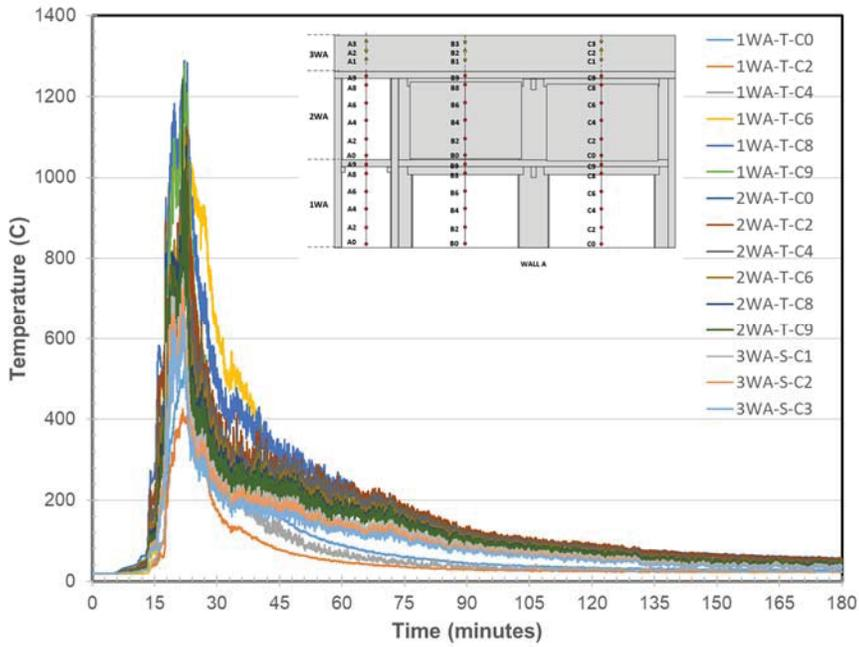
Figure 939. Wall A Temperatures at Locations C
