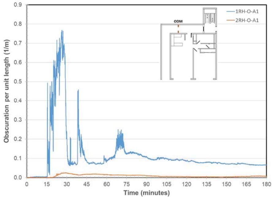
**Figure 961. Obscuration per unit Length in Corridor**
