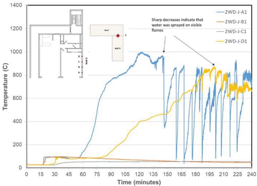
Figure 236. Ceiling/Wall B Joint Temperatures at Locations A-D
