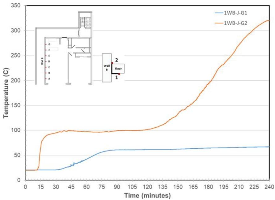
Figure 25. Wall B/Steel Angle Joint Temperatures at Location G
