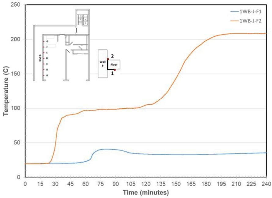
Figure 24. Wall B/Steel Angle Joint Temperatures at Location F
