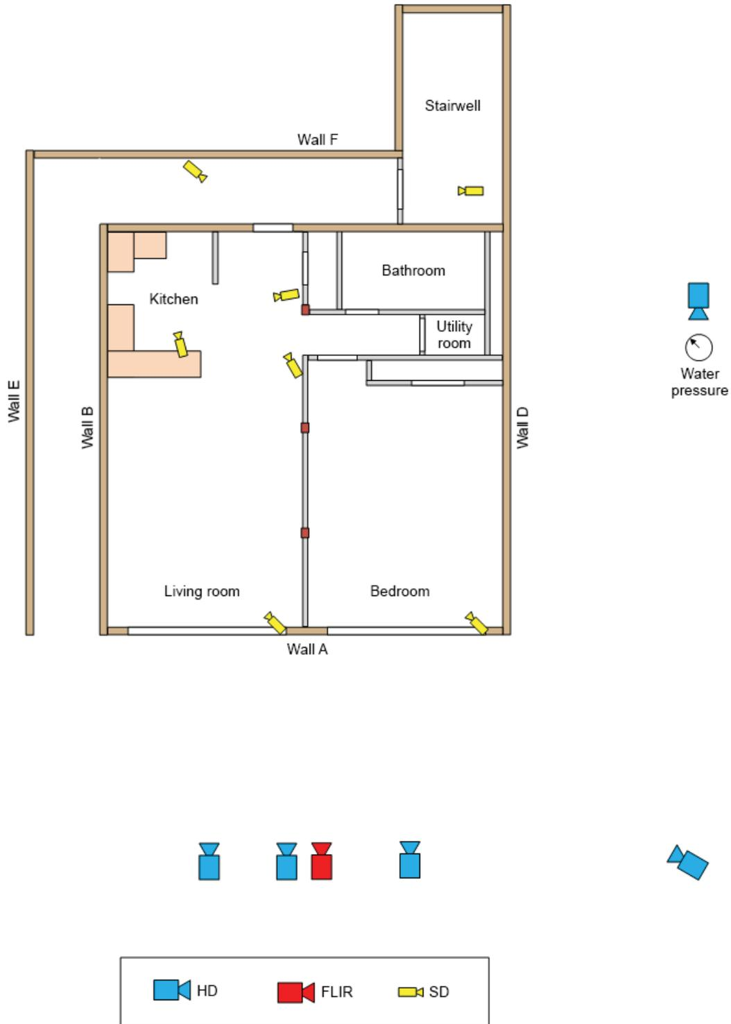
Figure 97. Layout of video cameras (HD, high definition; FLIR, forward looking infrared radiometer; SD, standard definition).
