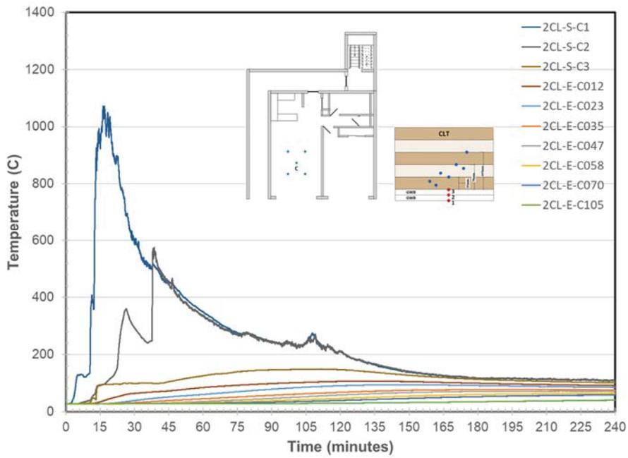
**Figure 211. Living Room Ceiling Embedded & Surface Temperatures at Location C**
