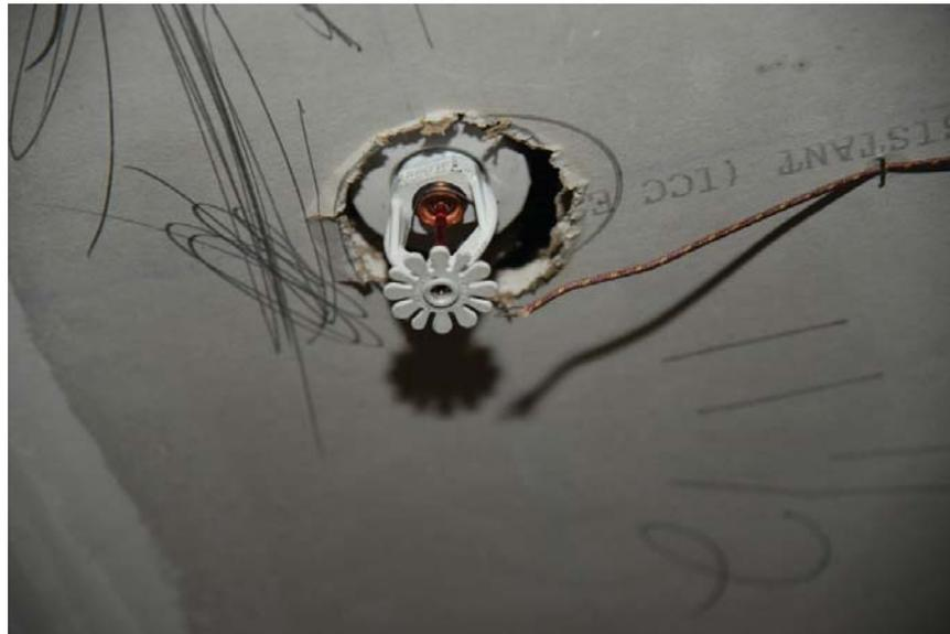
Figure 79. Thermocouple placed near sprinkler head in kitchen for Test 4.
