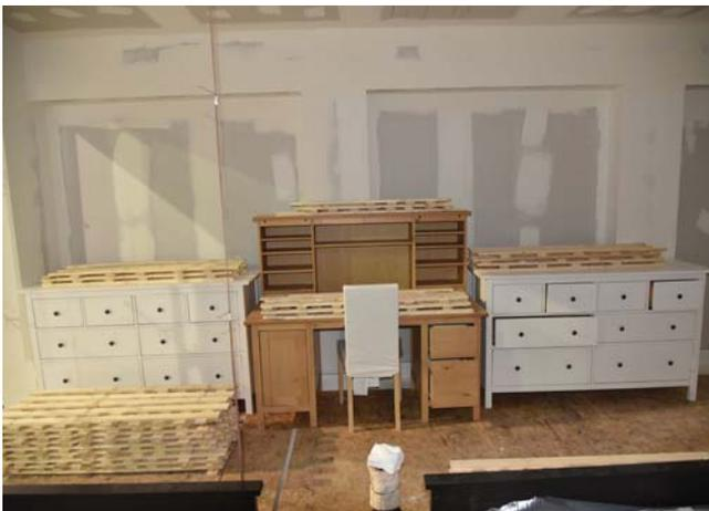
Figure 47. Wood cribs and oriented strandboard added in the bedroom.
