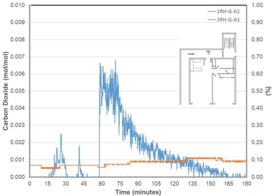
**Figure 966. Carbon Dioxide Concentrations in the corridor on each Floor**
