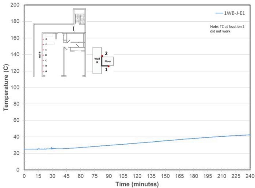
Figure 228. Wall B/Steel Angle Joint Temperatures at Location E
