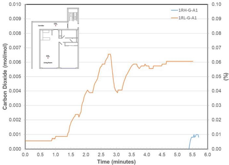
**Figure 272. Carbon Dioxide Concentration in the Corridor and Living Room**
