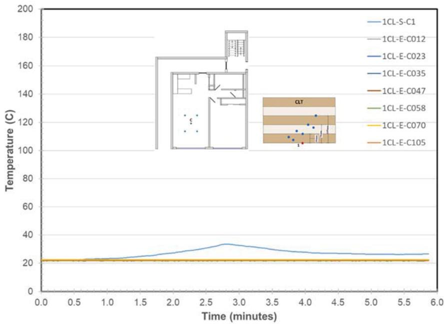
Figure 235. Living Room Ceiling Embedded & Surface Temperatures at Location C
