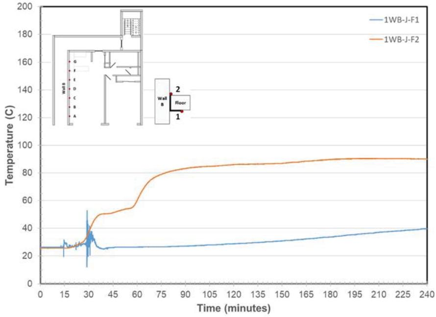
Figure 229. Wall B/Steel Angle Joint Temperatures at Location F
