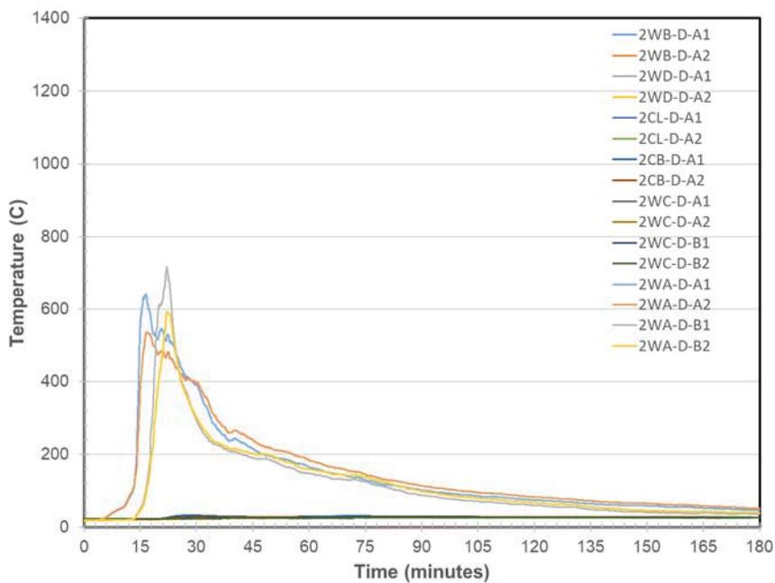
Figure 954. DFT Temperatures at each Location on 2<sup>nd</sup> floor
