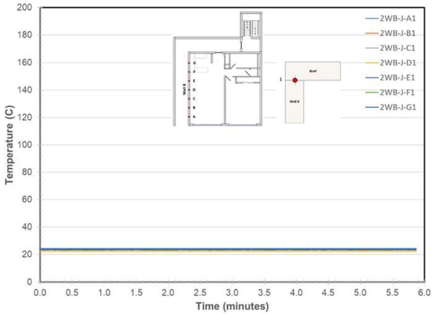
Figure 260. Ceiling/Wall B Joint Temperatures at Locations A-G
