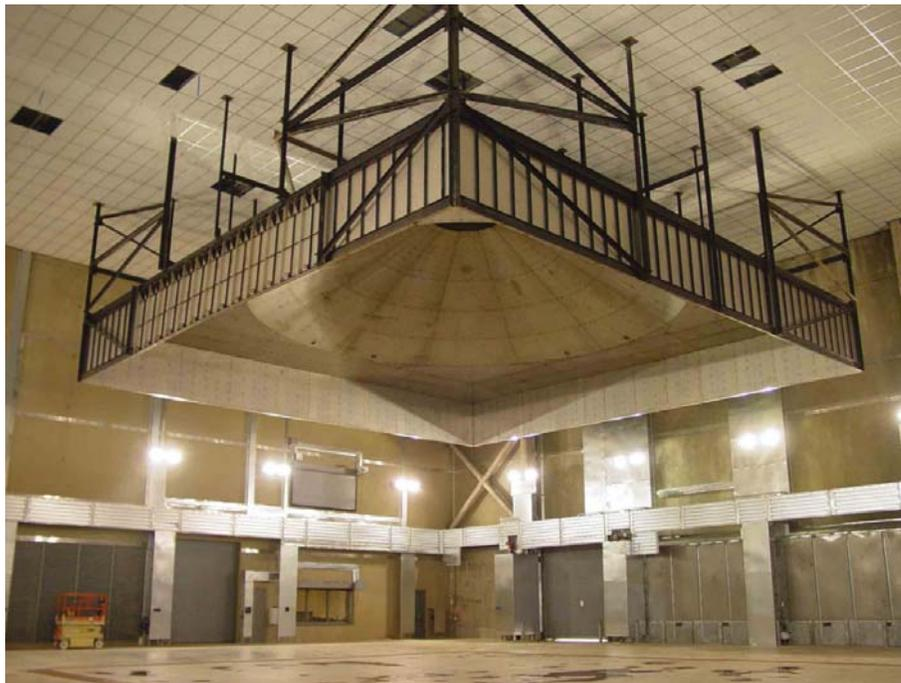
**Figure 96. 14-MW fire product collector at the Bureau of Alcohol, Tobacco, Firearms and Explosives (ATF) Fire Research Laboratory.**
