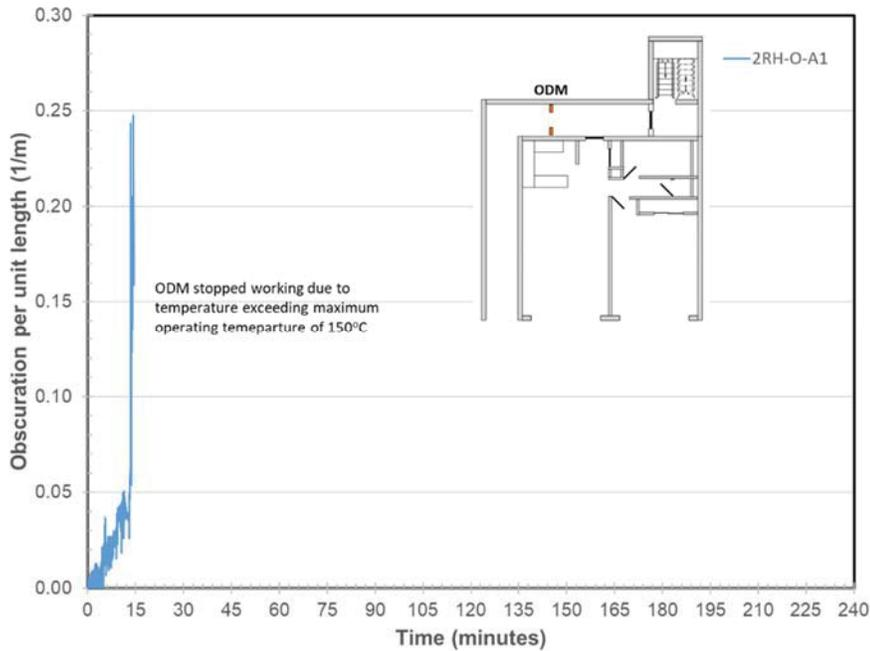
**Figure 244. Obscuration per unit Length in Corridor**
