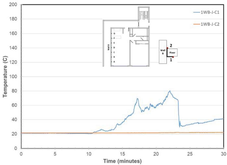
**Figure 22. Wall B/Steel Angle Joint Temperatures at Location C**
