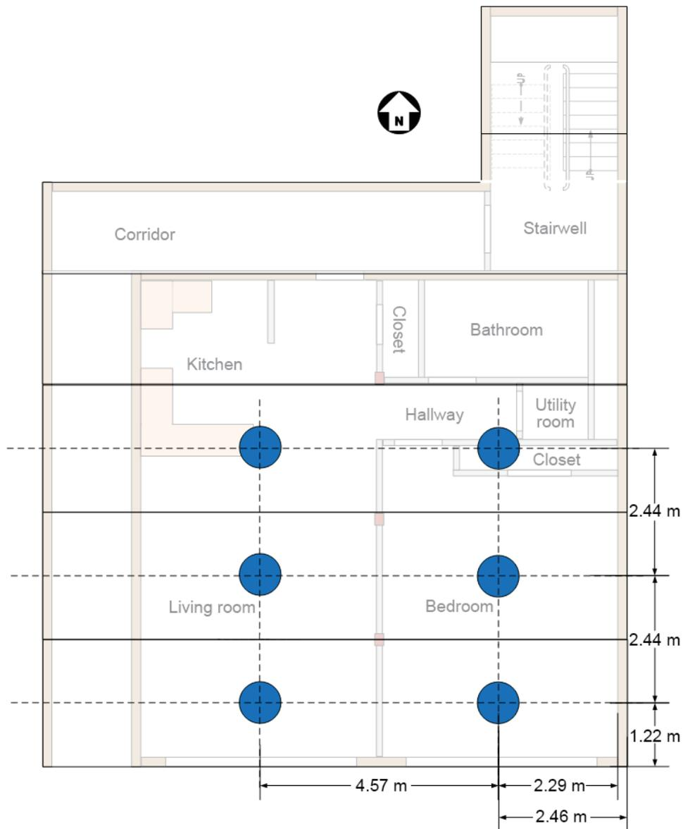
Figure 53. Location of water tanks on the second-level ceiling panel during Tests 2 and 3.
