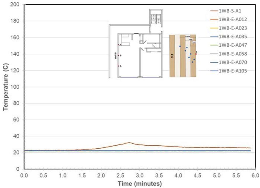
**Figure 231. Wall B Embedded & Surface Temperatures at Location A**
