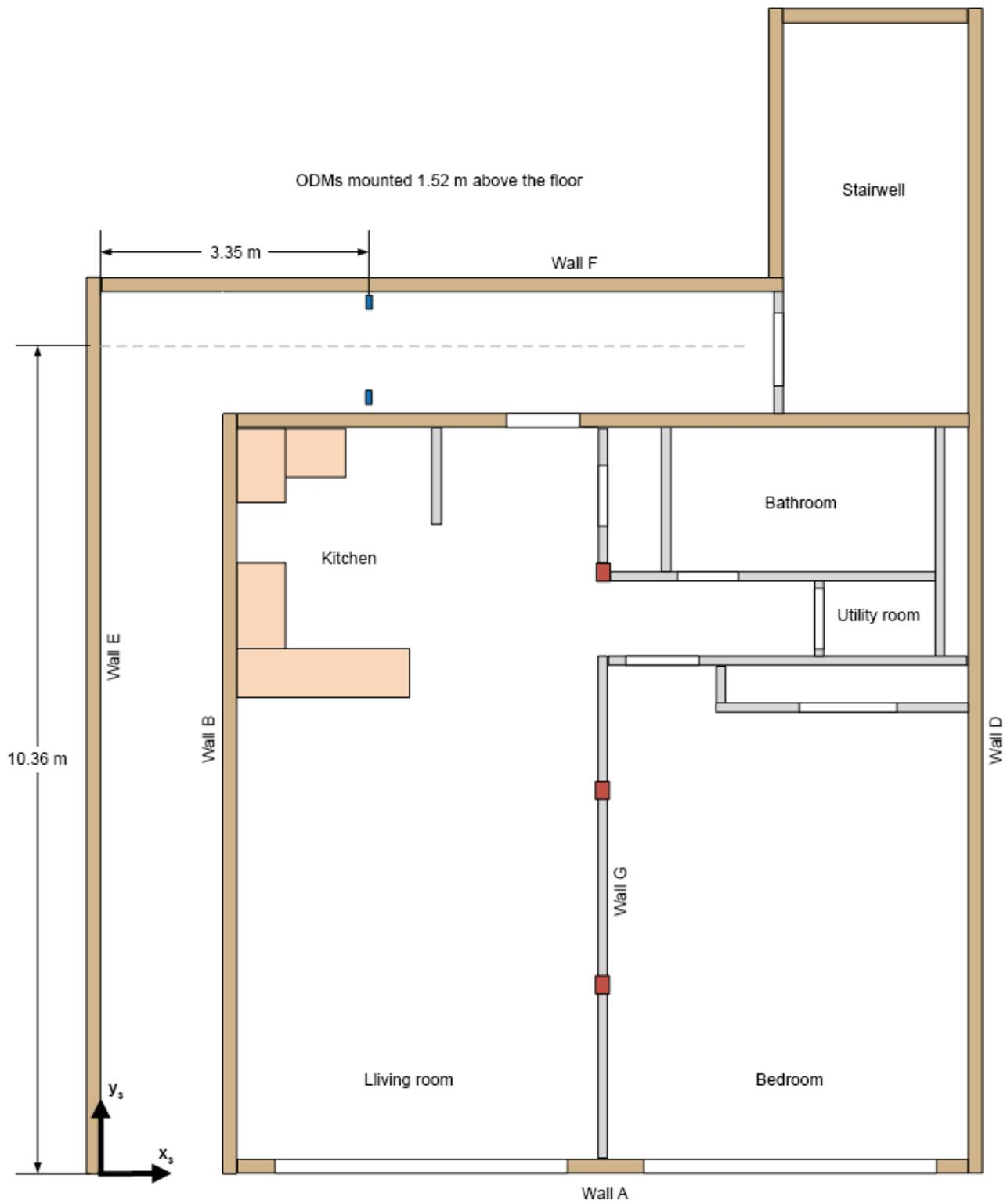
Figure 91. Location of optical density meters (ODMs) (blue rectangles).
