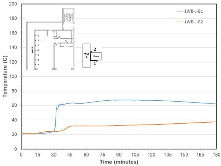
Figure 941. Wall B/Steel Angle Joint Temperatures at Location B
