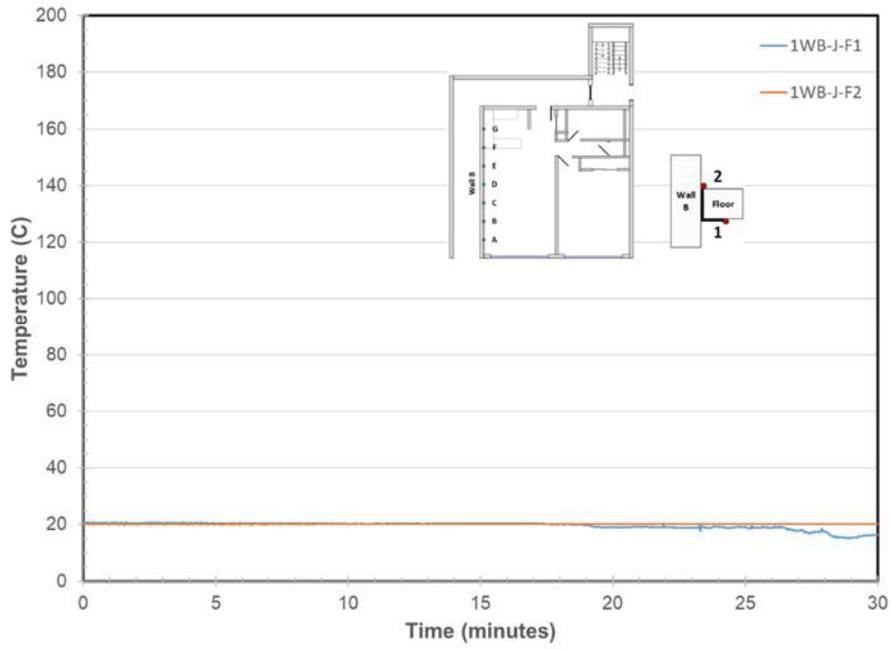
Figure 25. Wall B/Steel Angle Joint Temperatures at Location F
