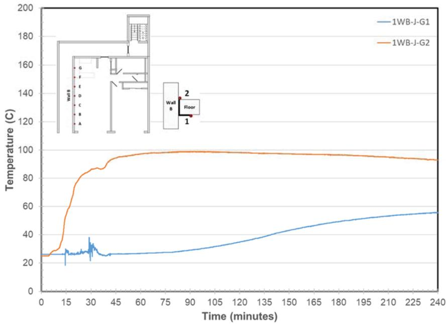
Figure 230. Wall B/Steel Angle Joint Temperatures at Location G
