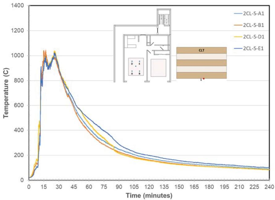
**Figure 9. Living Room Ceiling Surface Temperatures at Location A, B, D, & E**
