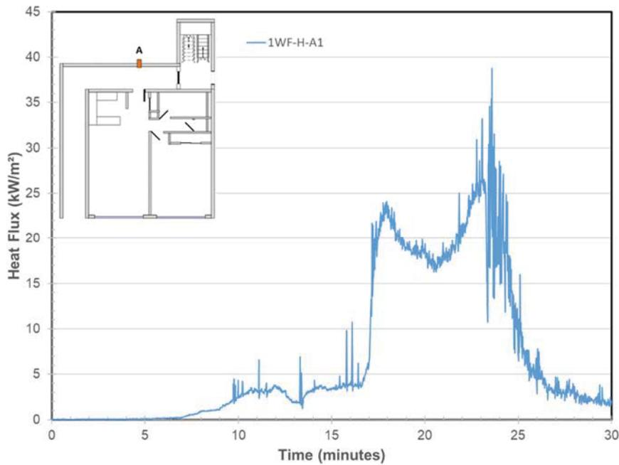
**Figure 38. Heat Flux on Wall F across from Apartment Door**
