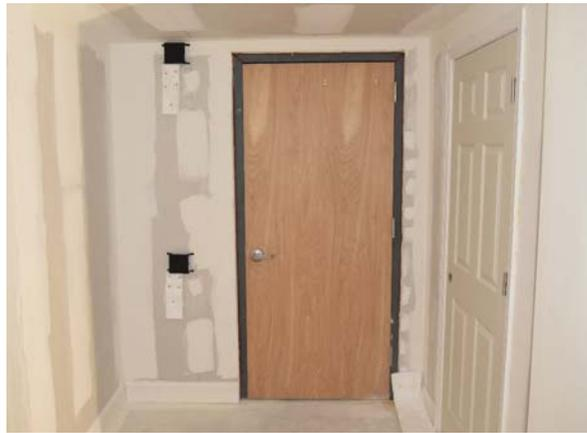
Figure 86. Directional flame thermometers mounted on Wall C near the apartment door.
