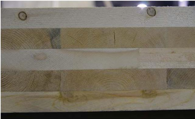
Figure 5. Cross section of the five-ply cross-laminated timber panel.
