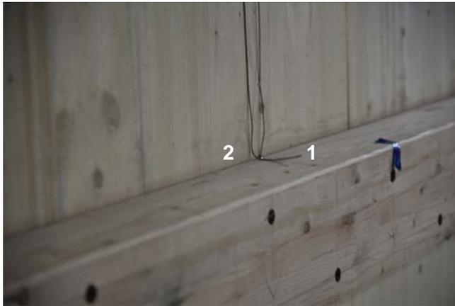
**Figure 74. Thermocouples placed on the ledger to measure the temperature at the ledger–floor interface (numbers correspond to locations shown in Fig. 73).**
