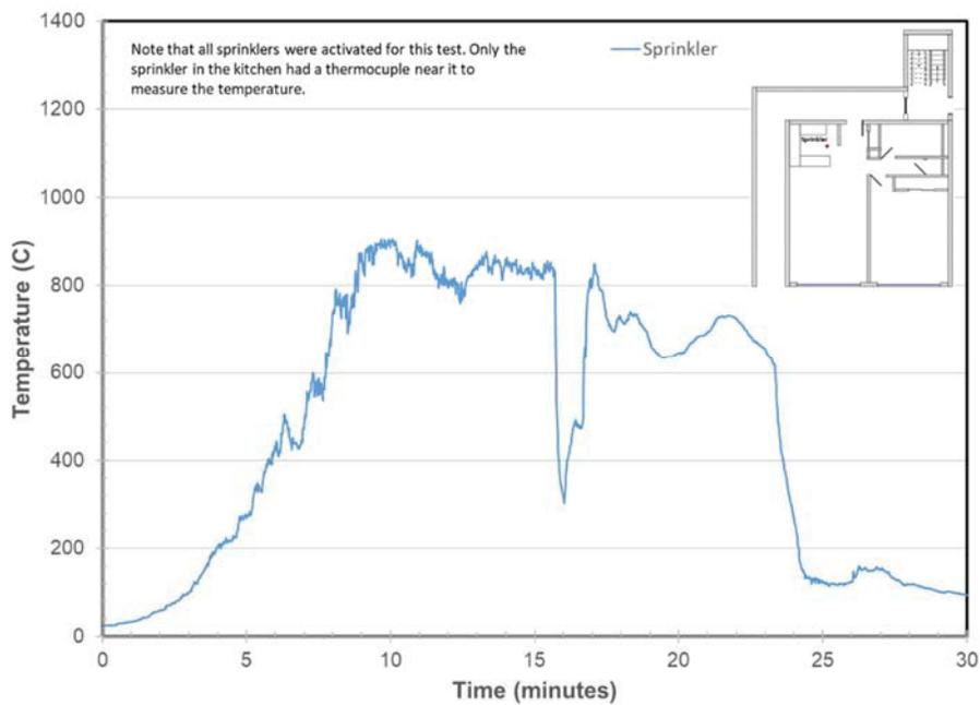
**Figure 16. Sprinkler Head Temperature in Kitchen**
