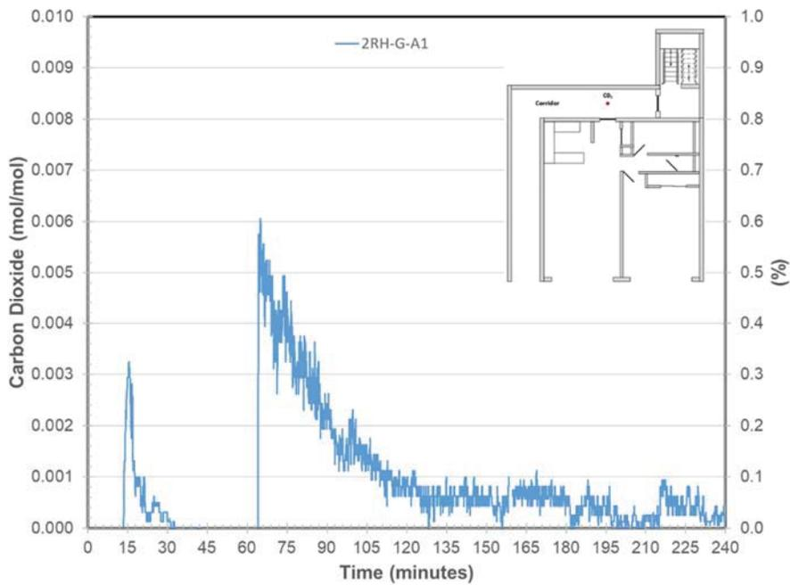
Figure 44. Carbon Dioxide Concentration in the Corridor
