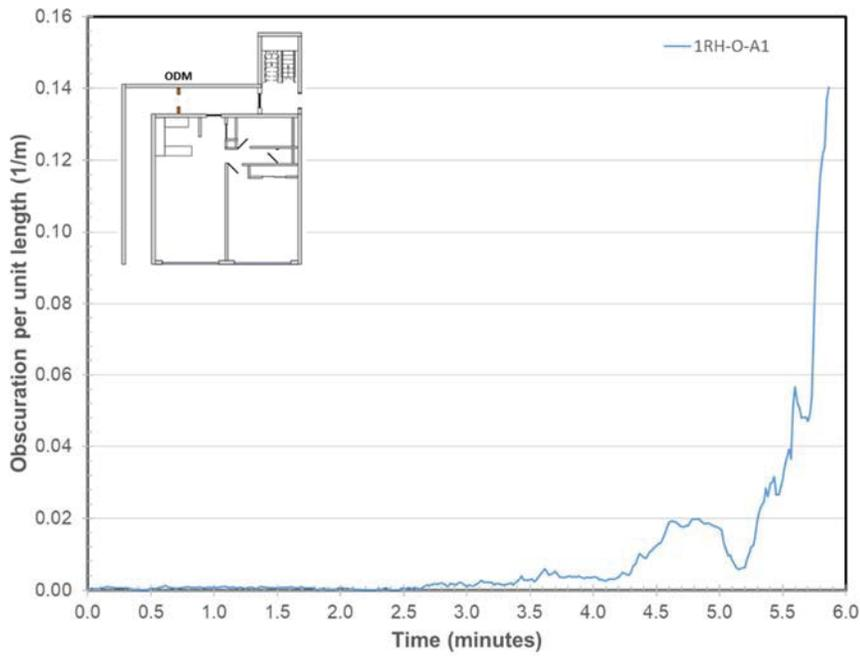
Figure 267. Obscuration per unit Length in Corridor
