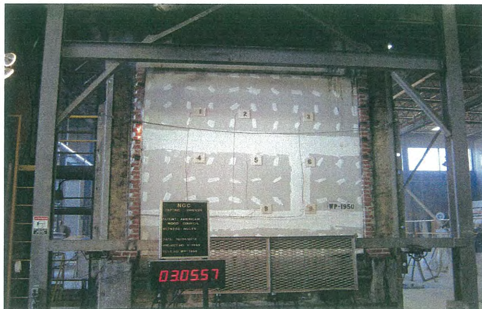
Unexposed Side – Flaming at Wall Assembly Perimeter
