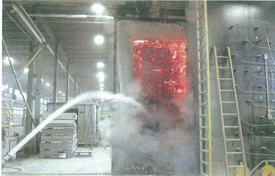
Exposed Side – End of Test (Removing from Furnace)
