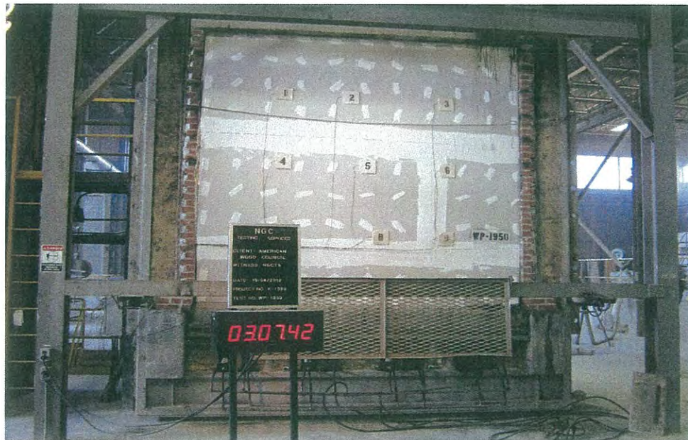
Unexposed Side – Test Termination
