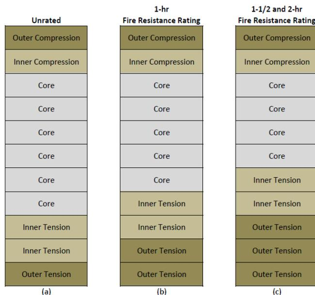
**Figure C16B Typical Balanced Beam Layup**
