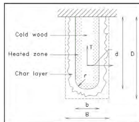
**Figure 9: Heavy Timber Member Exposed to Fire**
