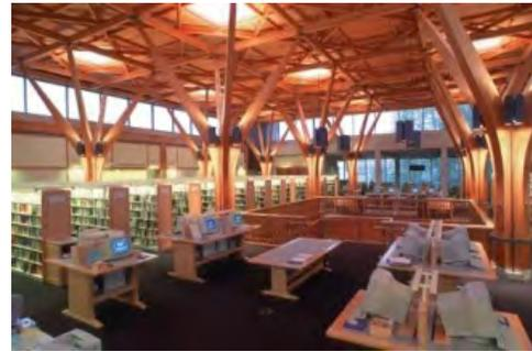
Figure 4: Type IV Construction
