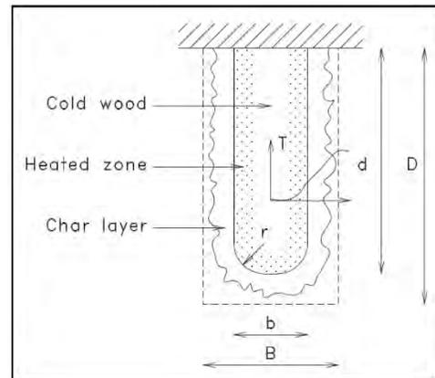
Figure 8: Heavy Timber Member Exposed to Fire
