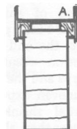
Figure 10-12.--A good metal flashing cap design. This cap channels water runoff away from the sides of the beam. Air space, as shown in (A), could further improve the design.
